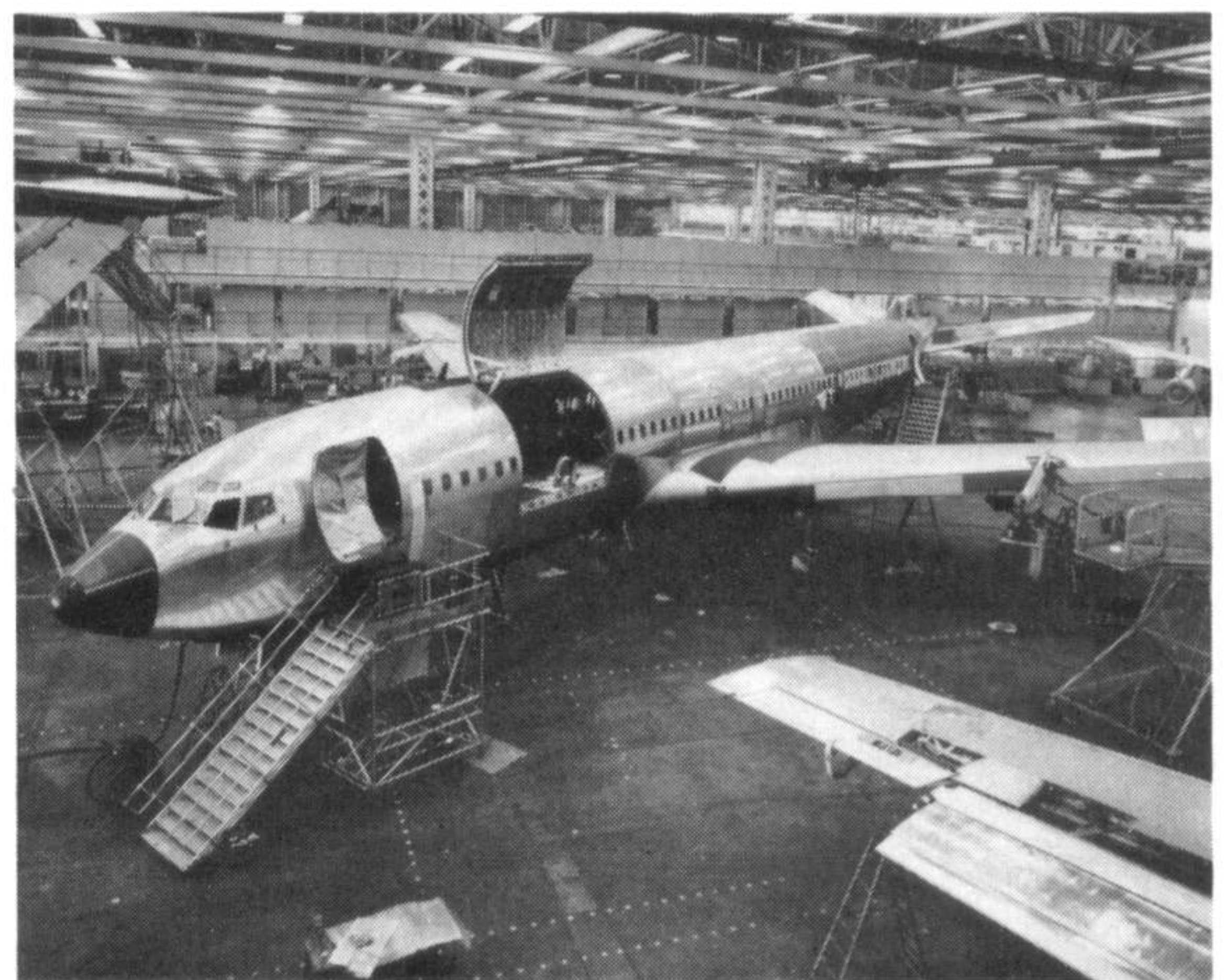
A 707-320C beginning to take shape; the fin and engines have still to be fitted.
