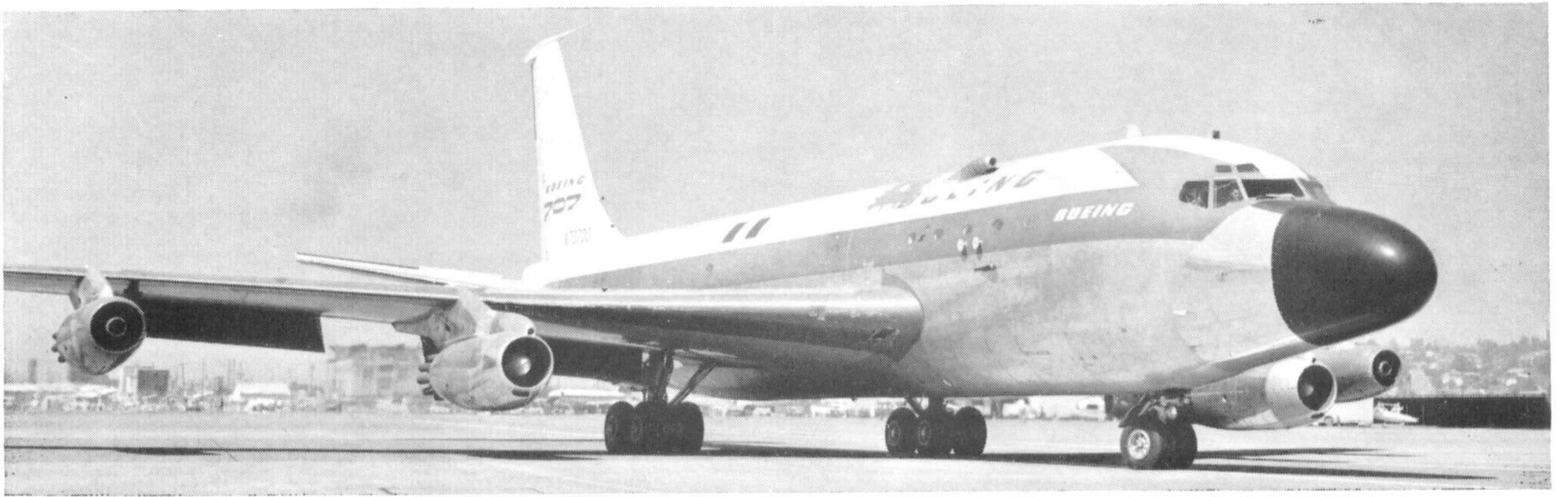
(Above) When fitted with the Bendix AN/AMQ-15 weather radar, the nose of the "Dash Eighty" assumed a new shape. At the time this photo was taken engine tests were also in progress. The outboard engines were JT-3's, No. 2 was a J 75 and No. 3 was a J 57.
