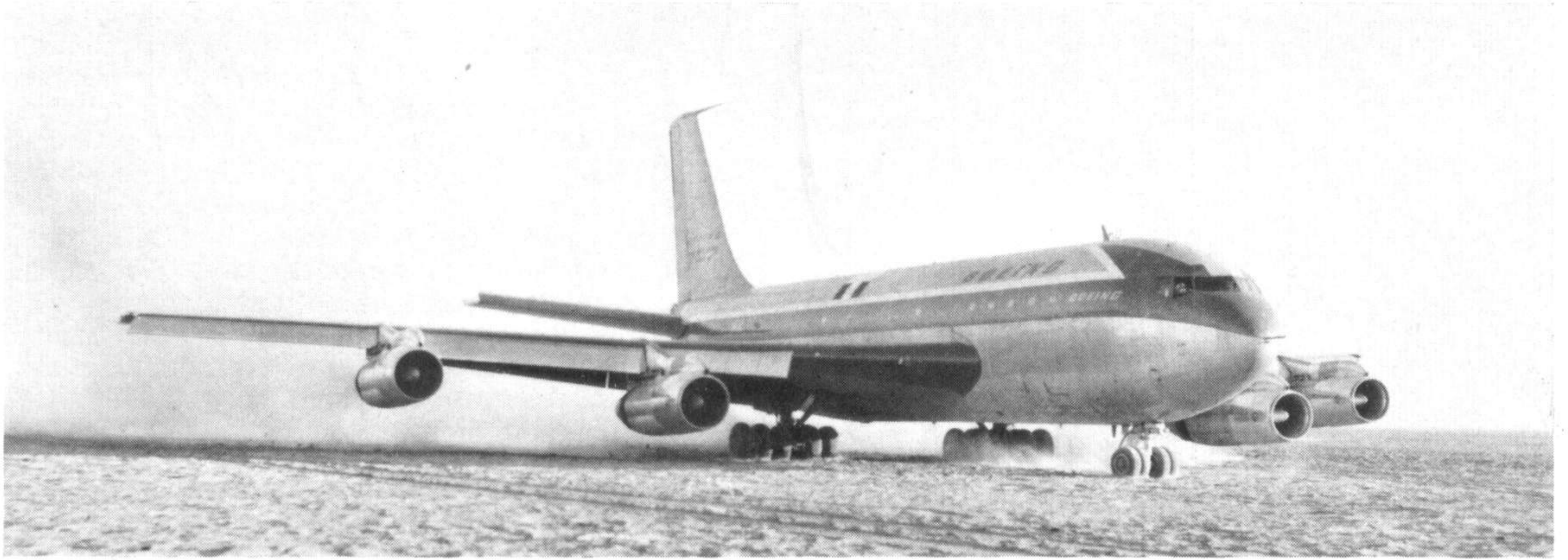
(Above) Modified still further with a twenty-wheel rough field landing gear, the "Dash Eighty" made a series of landings and take-offs from the untreated sand and mud surface of Harper Dry Lake, California.
