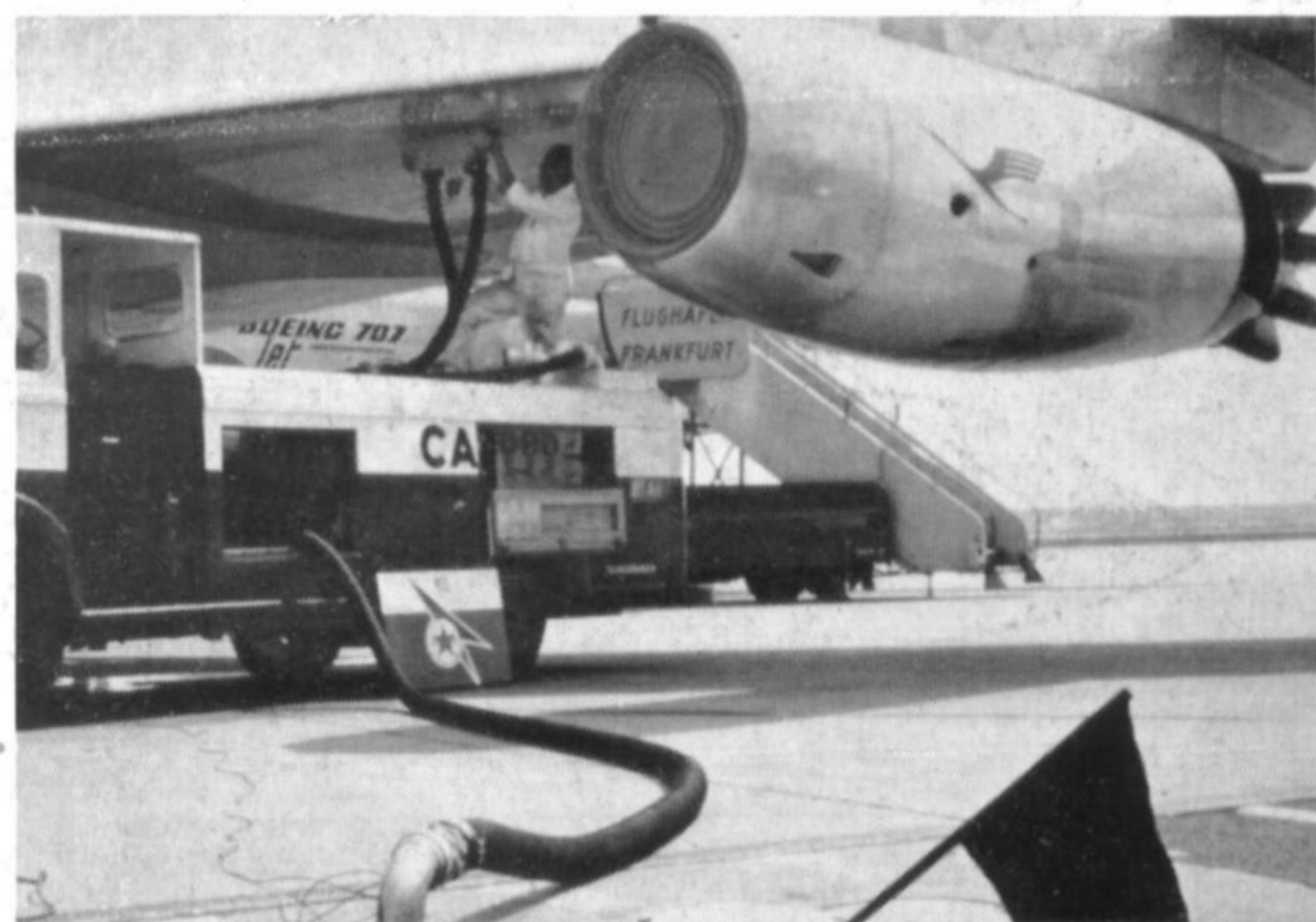
Pressure refuelling a Lufthansa 707 at Frankfurt International Airport. (Photo: Lufthansa)
