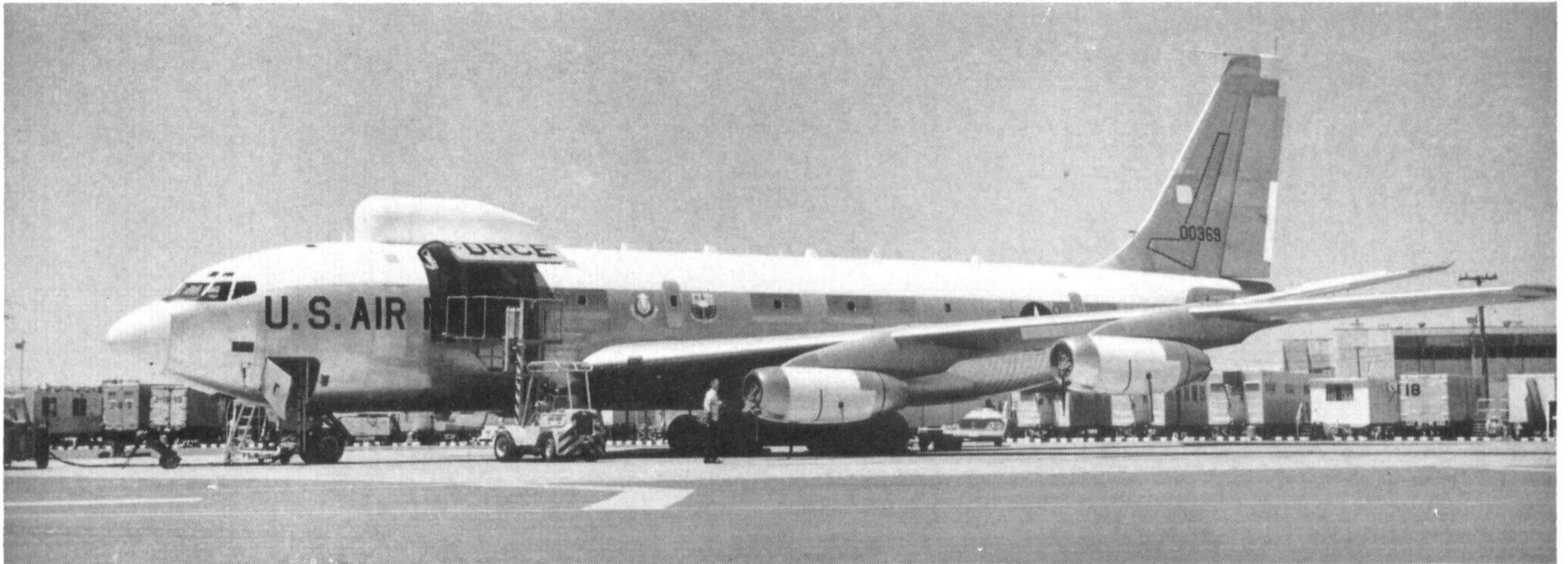
These hump backed NKC-135A's carry infra red, ultra violet and optical scanning equipment for data collection during nuclear tests. Note the unusual sensor built into the starboard wing. These aircraft fly clockwise round the explosion while collecting their information, and therefore have all markings on the starboard side painted out to avoid flash burns. On their port sides these aircraft carry the normal markings. The badges on the fuselage are those of the Air Force Systems Command and the A.F. Special Weapons Centre. Two NKC-135A's were built with sensors looking out to starboard, one with sensors looking out to port.
