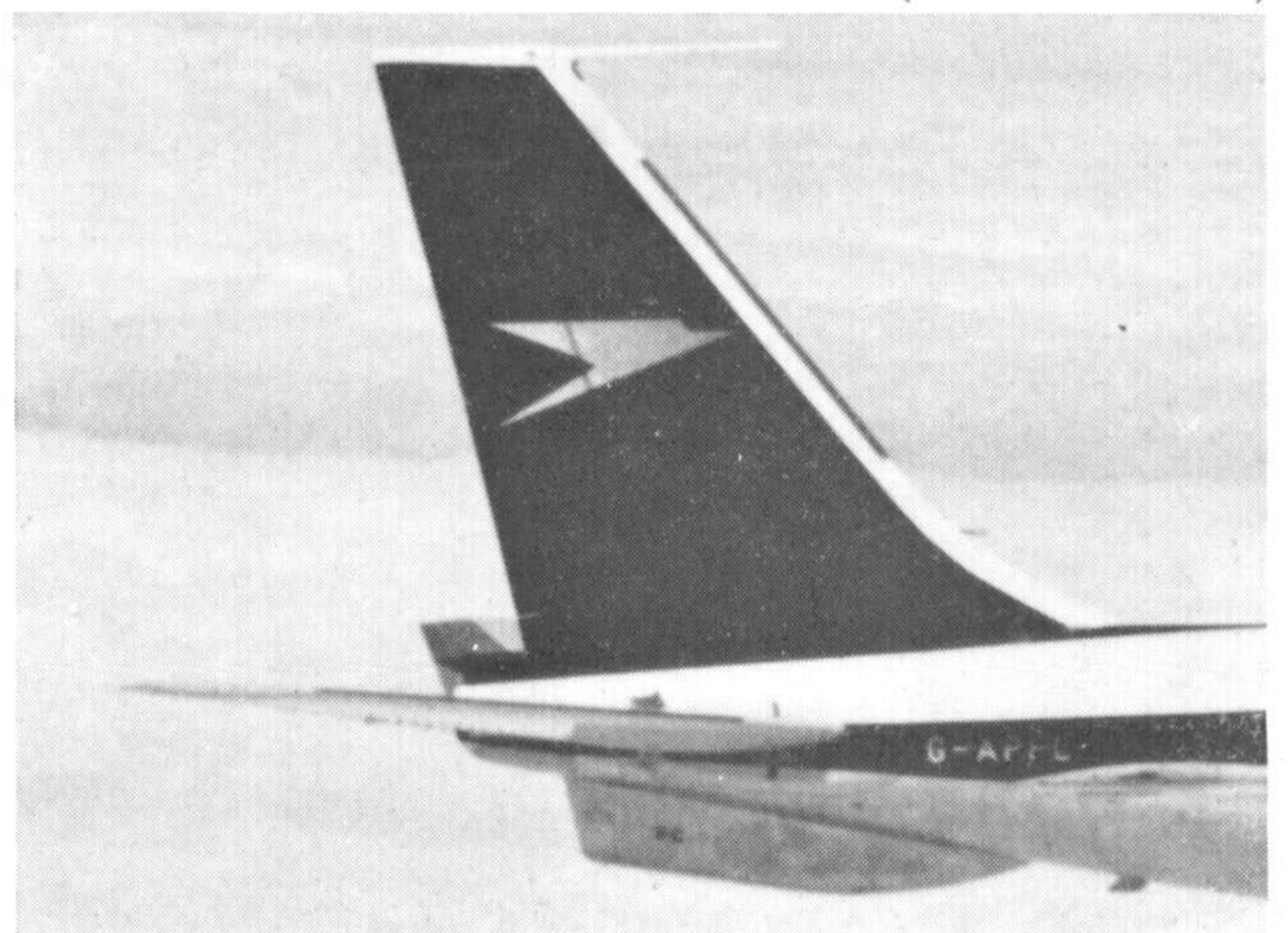
Boeing 707 tails: (below) the original short fin, as fitted to the early models; and (right) the modified fin with an extra 2 ft. 11 in. at the top to improve directional stability. The under fin, fitted to some 707's, provides warning of an excessive nose-up attitude during take-off. (Photo: B.O.A.C.)
