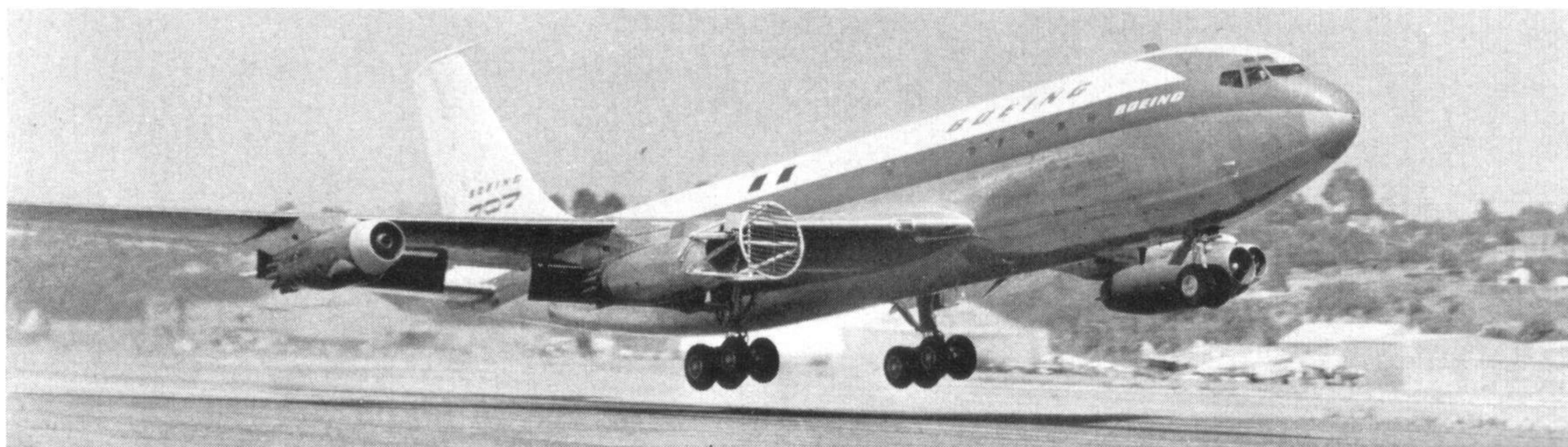
The "Dash Eighty" taking off. At the time this picture was taken the aircraft was fitted with a water spray rig for icing tests of the J 57 fitted in the starboard inner position.
