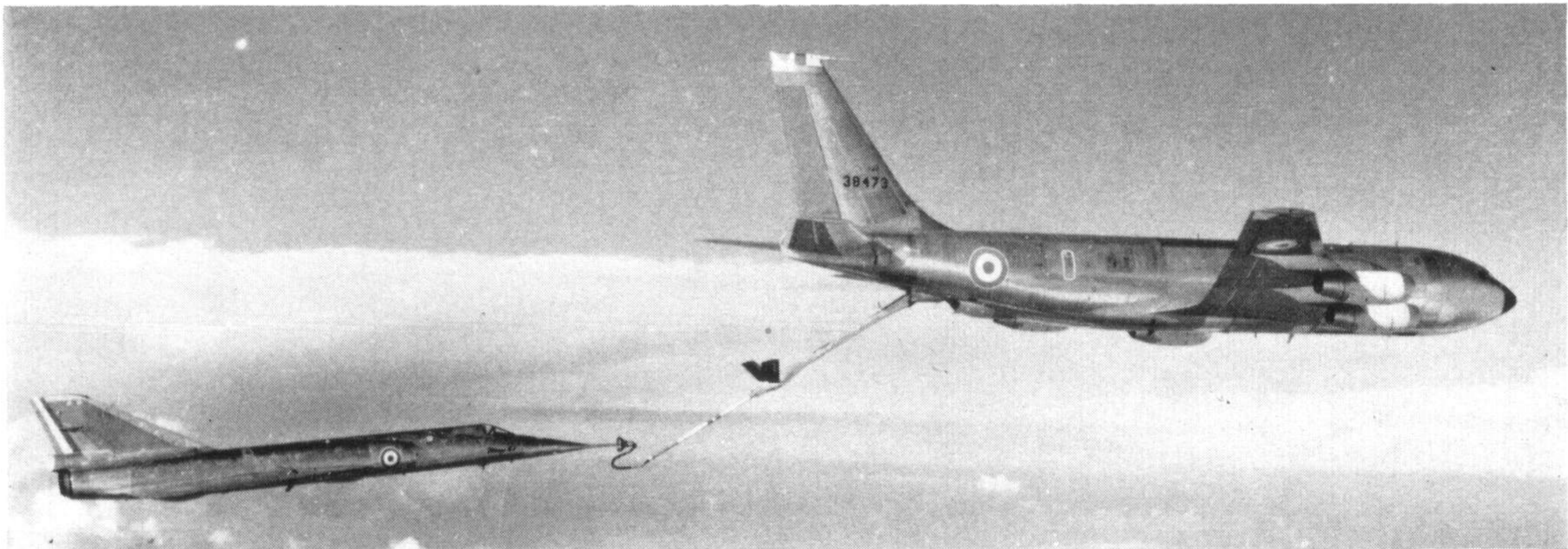
A C-135F (the "K" prefix is not applied to these aircraft) of the French Air Force refuels a Mirage IV. Note the adaptor to enable the boom to be used for the probe and drogue refuelling method. Because of its appearance as it hangs from the rear of the tanker, while the latter is on the ground, the adaptor is widely known as "The Limp Dick". (Photo: French Air Force)
