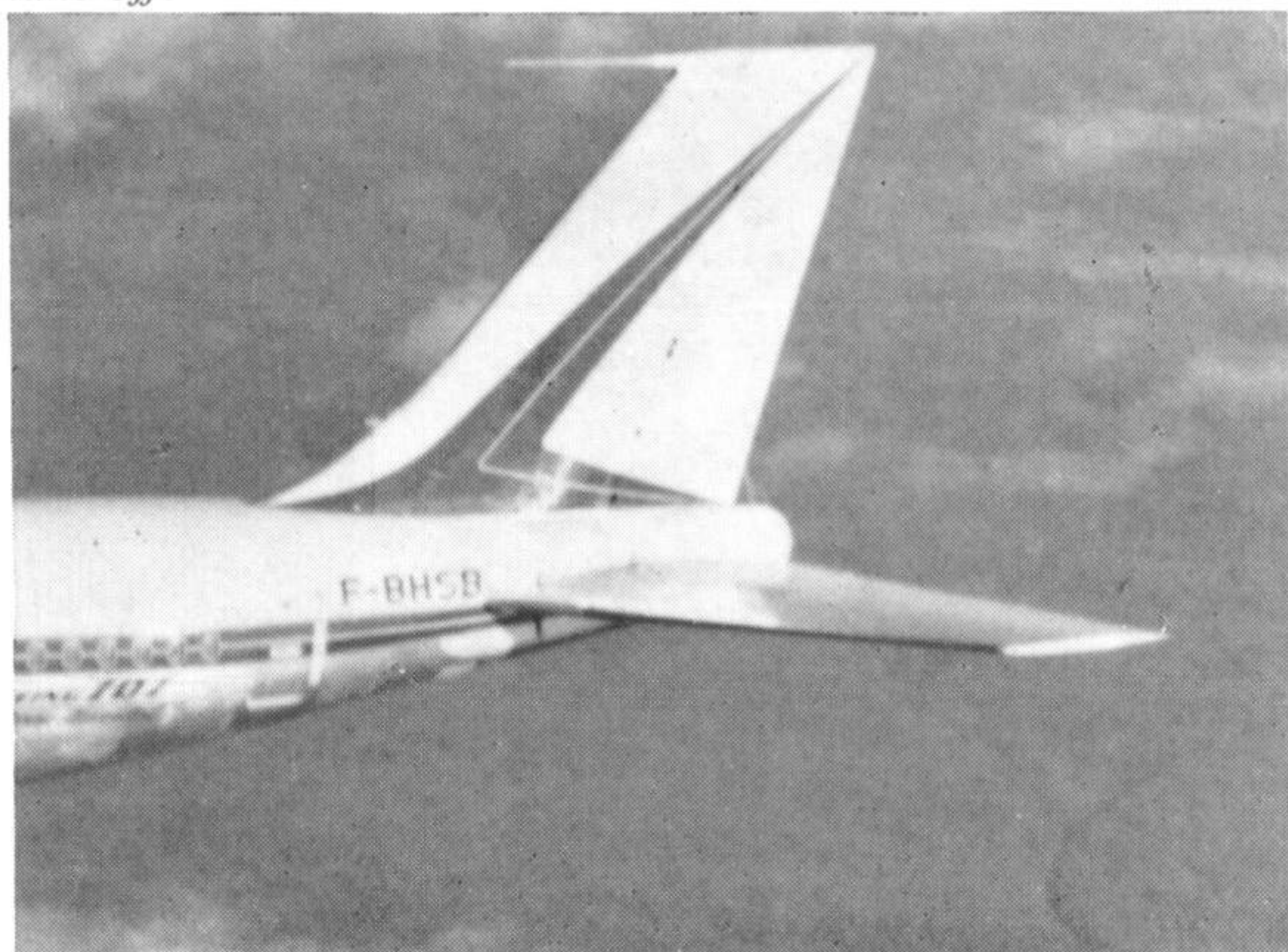
Boeing 707 tails: (below) the original short fin, as fitted to the early models; and (right) the modified fin with an extra 2 ft. 11 in. at the top to improve directional stability. The under fin, fitted to some 707's, provides warning of an excessive nose-up attitude during take-off. (Photo: B.O.A.C.)
