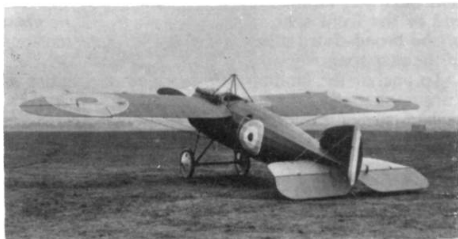
(Left) The first Bristol M.1B, A5139, had its clear-view panel in the starboard wing root covered with transparent material. This view shows clearly the Vickers gun mounted on the port upper longeron and the white guide line between the upper and lower foot-holds in the fuselage side. (Right) This frontal view of A5141 in Palestine shows the Clerget engine, small frontal opening in the spinner, and position of the Vickers gun. (Photo: John H. Blake)
