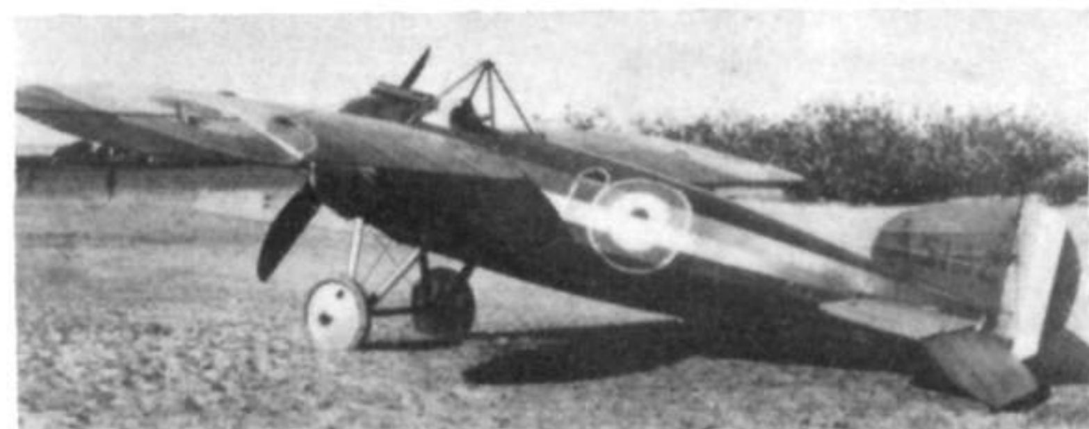
(Left) The fourth M.1B, A5142, with its Vickers gun installed centrally on top of the fuselage. (Photo: I.W.M. H(AM) 1469) (Right) The first production M.1C, C4901, together with another M.1C and an Avro 504A, photographed in Egypt. The absence of armament indicates that the Bristols were used for training purposes.
