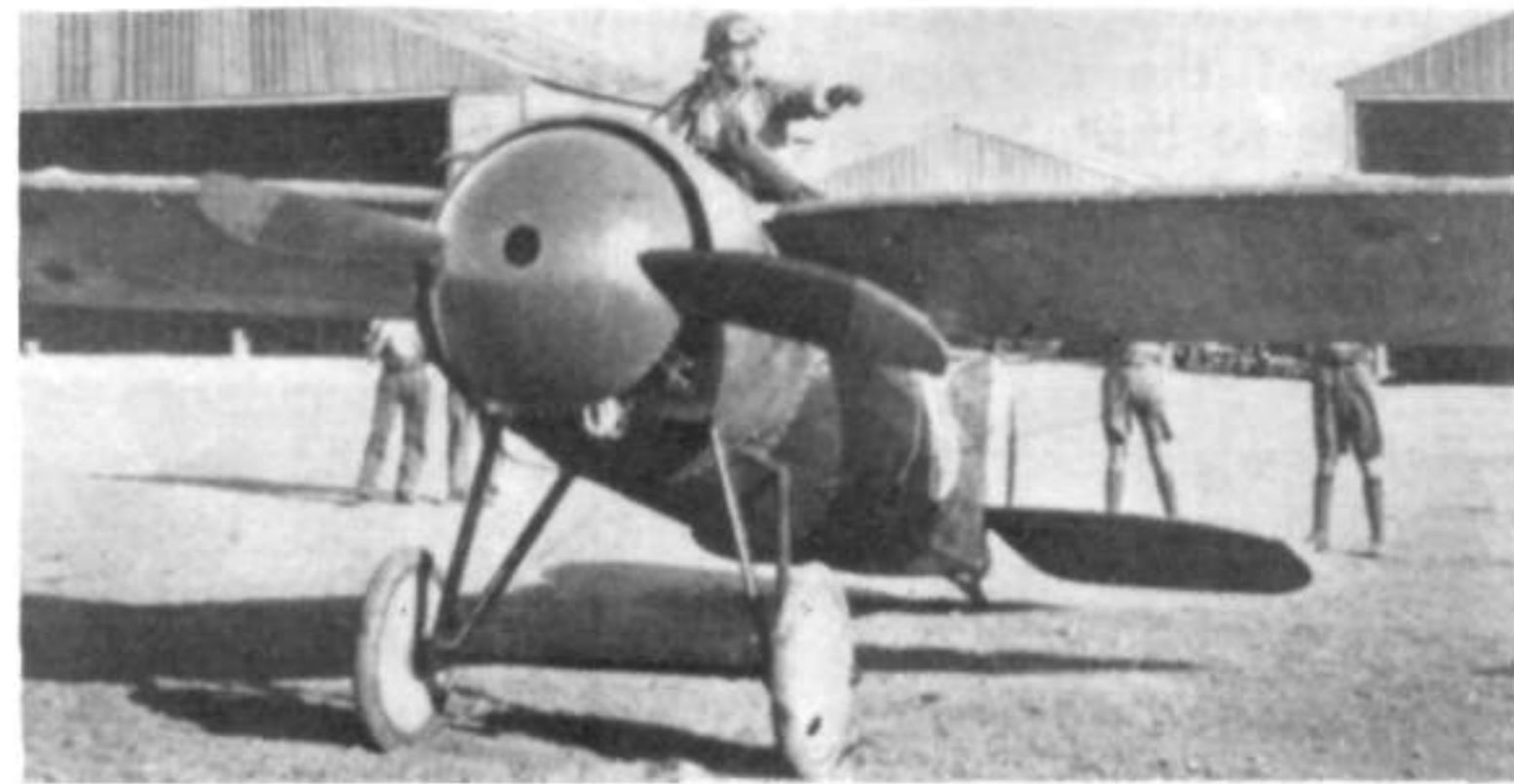
(Left) The first Bristol M.1B, A5139, had its clear-view panel in the starboard wing root covered with transparent material. This view shows clearly the Vickers gun mounted on the port upper longeron and the white guide line between the upper and lower foot-holds in the fuselage side. (Right) This frontal view of A5141 in Palestine shows the Clerget engine, small frontal opening in the spinner, and position of the Vickers gun. (Photo: John H. Blake)
