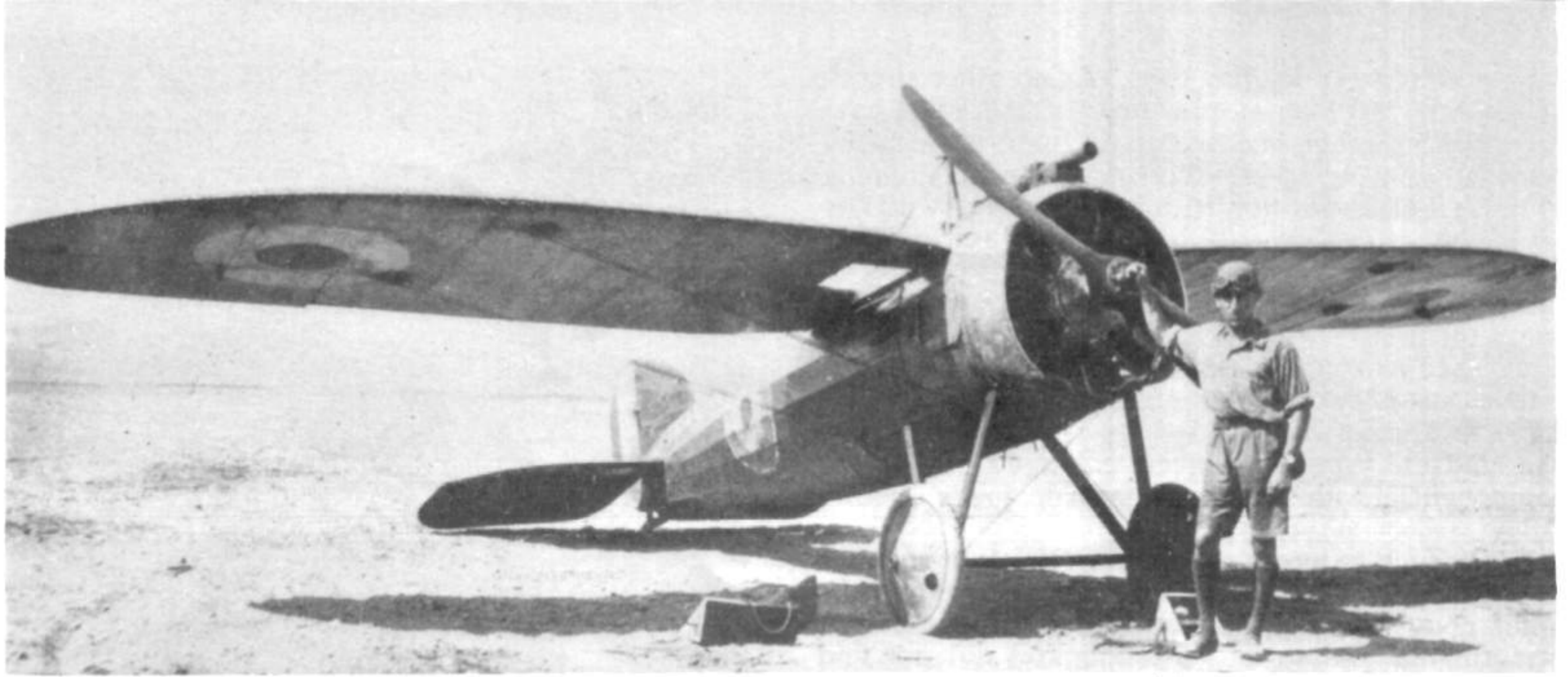
Another M.1C with spinner removed out of consideration for its Le Rhône engine. It is believed that this photograph was taken at Heliopolis; certainly the fitting of a camera gun indicates that this Bristol was used for training purposes.
