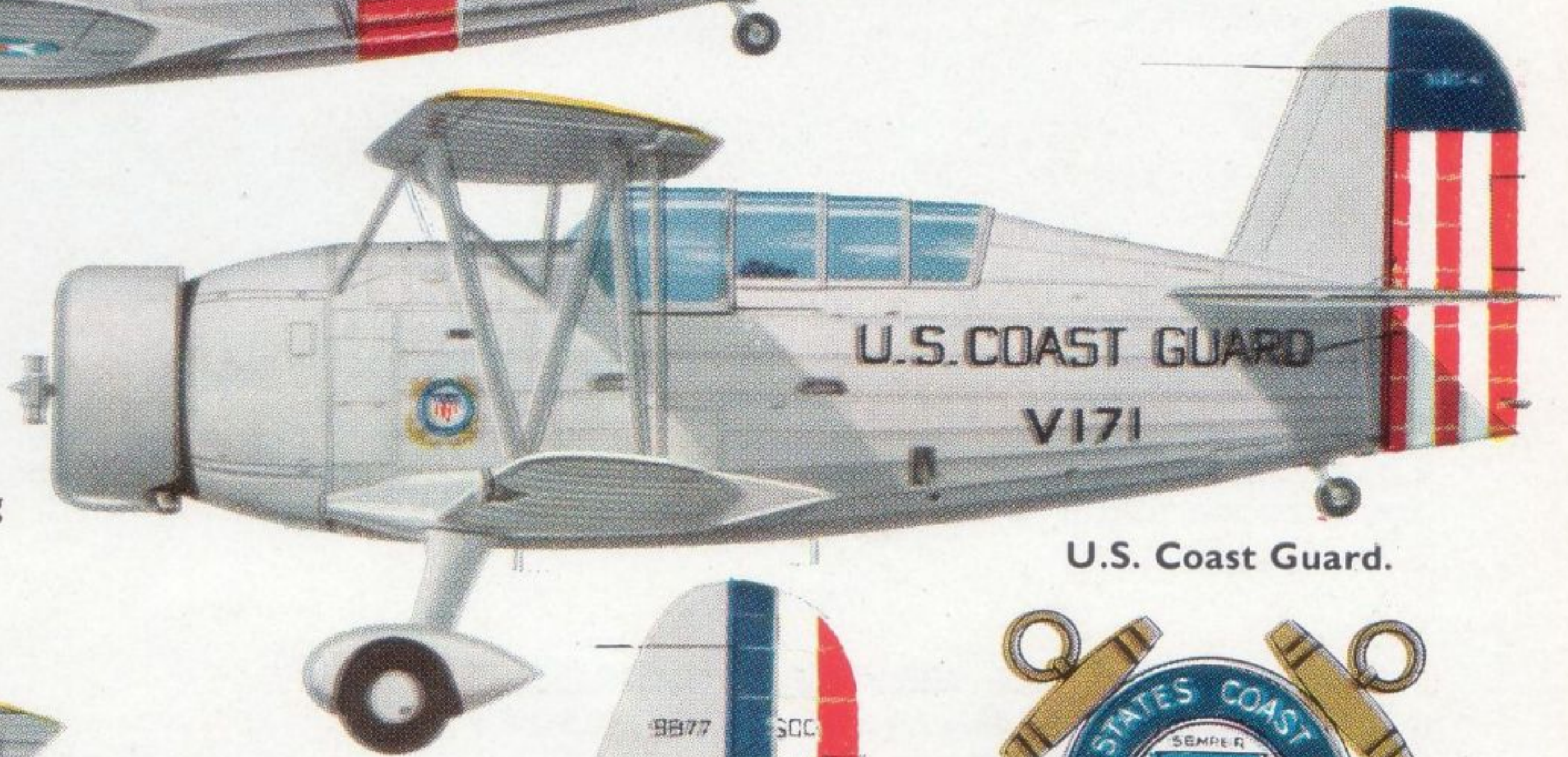
SOC-4 of U.S. Coast Guard; this aircraft also operated on floats from the Coast Guard cutter Bibby in 1938-39. Silver finish overall, yellow top wing upper surfaces.
