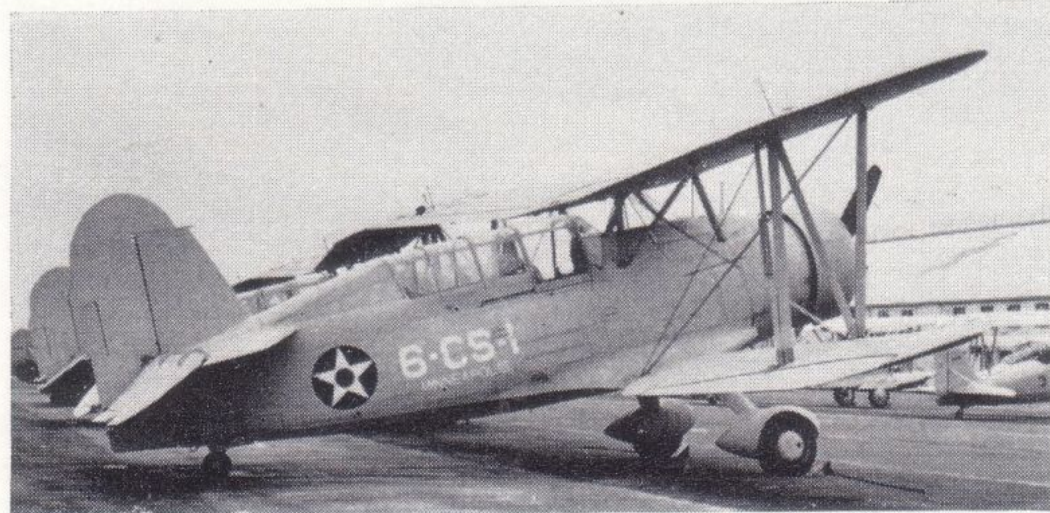
(Left) Starting in March 1941 the colourful squadron markings were replaced with a dull overall grey. The national insignia was placed on both sides of the fuselage but removed from the top and lower left wings. The squadron designation and ship name, in white, was retained until after 7th December, 1941. (Photo: the author). (Right) One of the main advantages of the SOC over the previous Vought observation types was that its wings would fold to give a total width of only 12 feet 6 inches. Some Second World War cruisers had hangers above or below deck for repair work. (Photo: the author)
