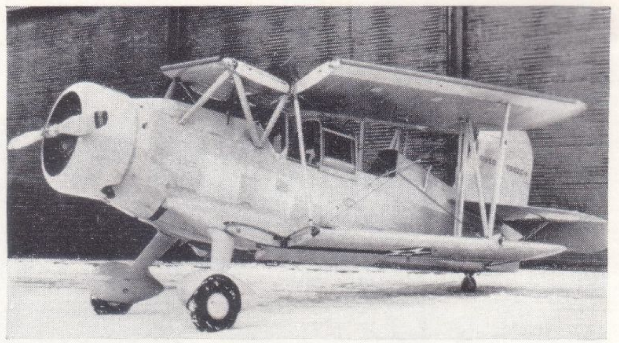
(Left) The Naval Aircraft Factory at Philadelphia built 44 duplicates of the SOC-3 as the model SON-1. Number 1166, shown here, was operating with VO-3 aboard the battleship U.S.S. Mississippi. (Photo the author). (Right) A January 1937 photo of the XS02C-1 which had flaps on both upper and lower wings and a minor engine change; one only was built. (Photo: Curtiss neg. no. SF-10024)
