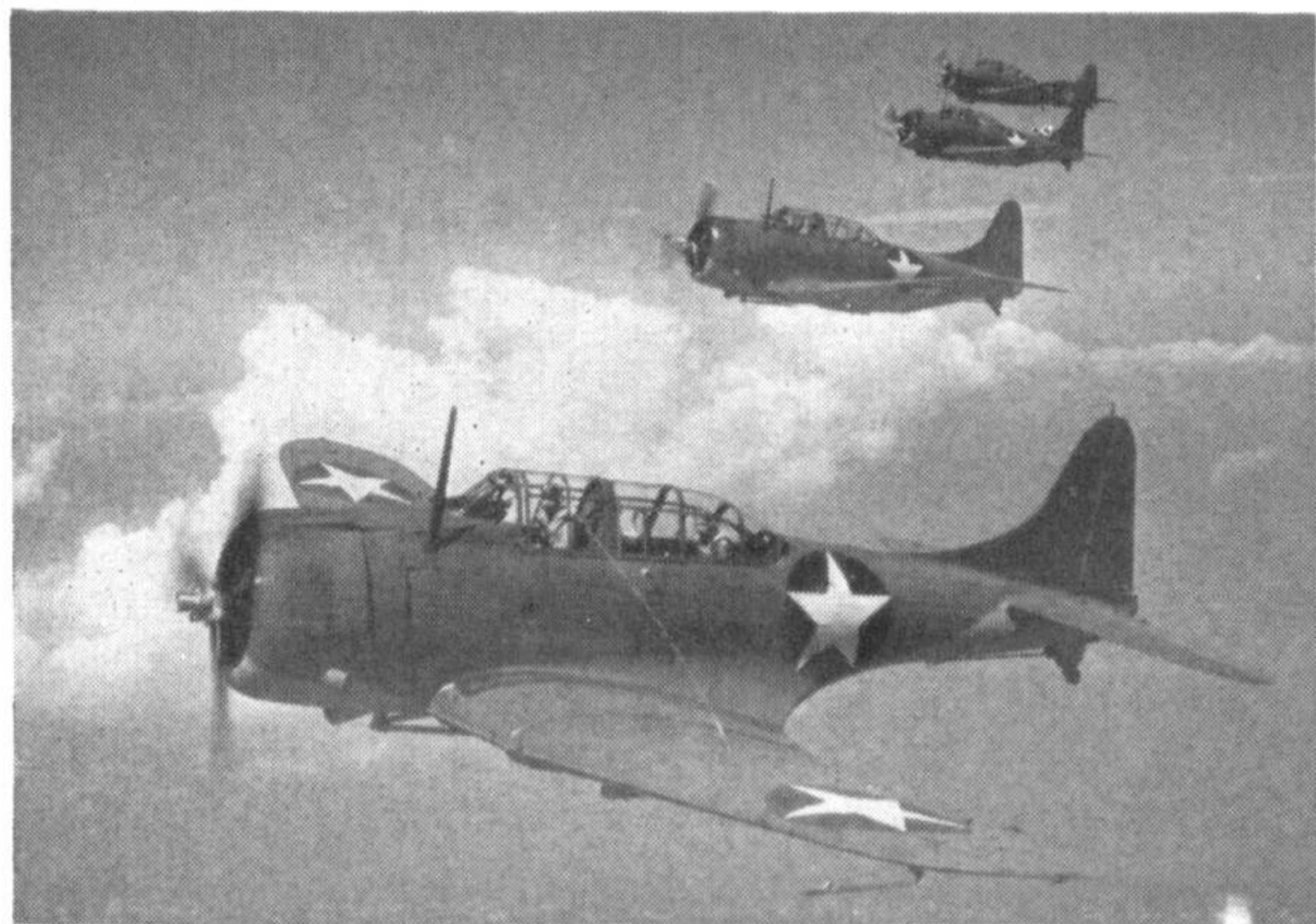
A formation of early SBD-3's; a second rear gun, improved armour and self-sealing fuel tanks carried the top weight to 6,350 lbs. (Photo: U.S. Navy Official via W. T. Larkins)
