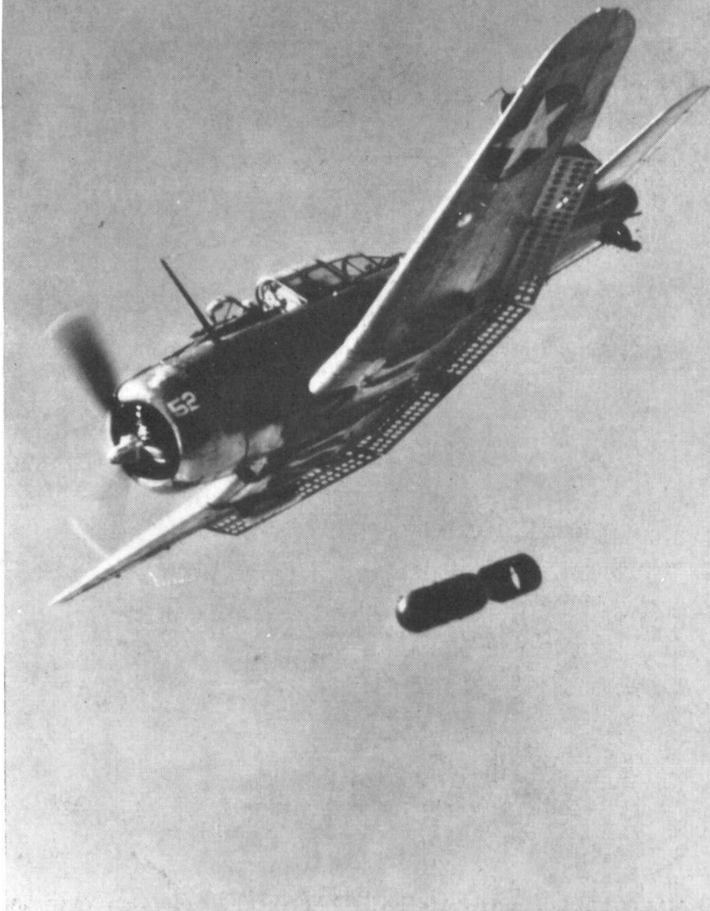
A classic view of the SBD Dauntless, which shows the characteristic pierced flaps to advantage.
