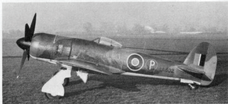
The first Tempest II prototype, LA602, with Centaurus IV and Typhoon tail unit.
