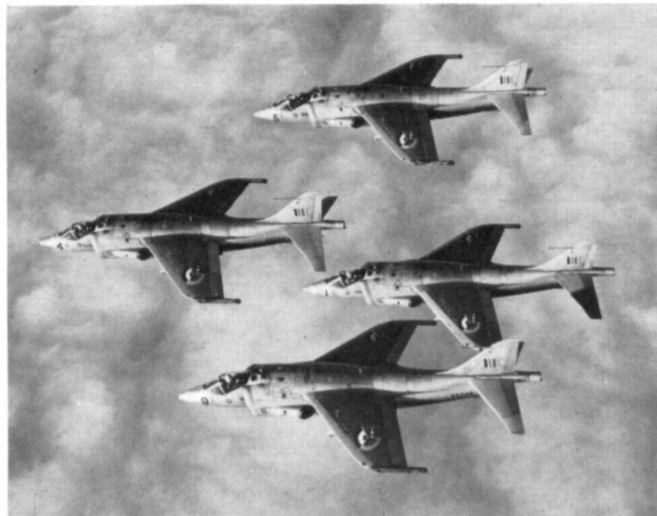
Curiously suggestive of a shoal of porpoises, four Kestrels of the West Raynham squadron in vic formation with "one in the box". The corrected wing markings (i.e. not mirrored) are evident. Also well illustrated are the extended tailplanes. (Neg. No. 687/261)
