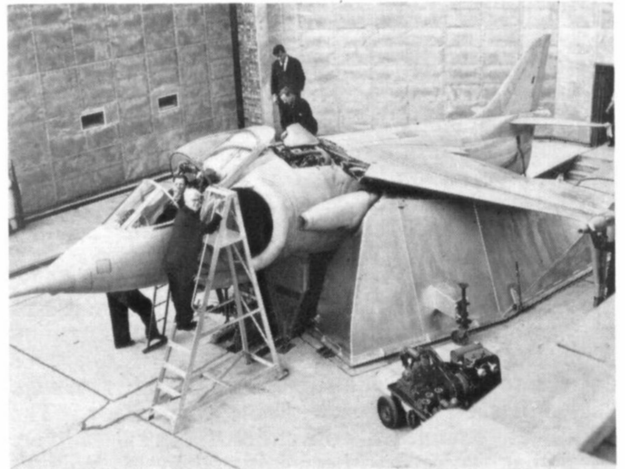
Preparations being made for engine running prior to the first flight. In the cockpit is Bill Bedford, beside him Frank Cross, head of the Experimental Design Office. The large sheet metal shrouds were designed to allow both horizontal and vertical nozzle positions during engine running. (Neg. No. EXP256/60)
