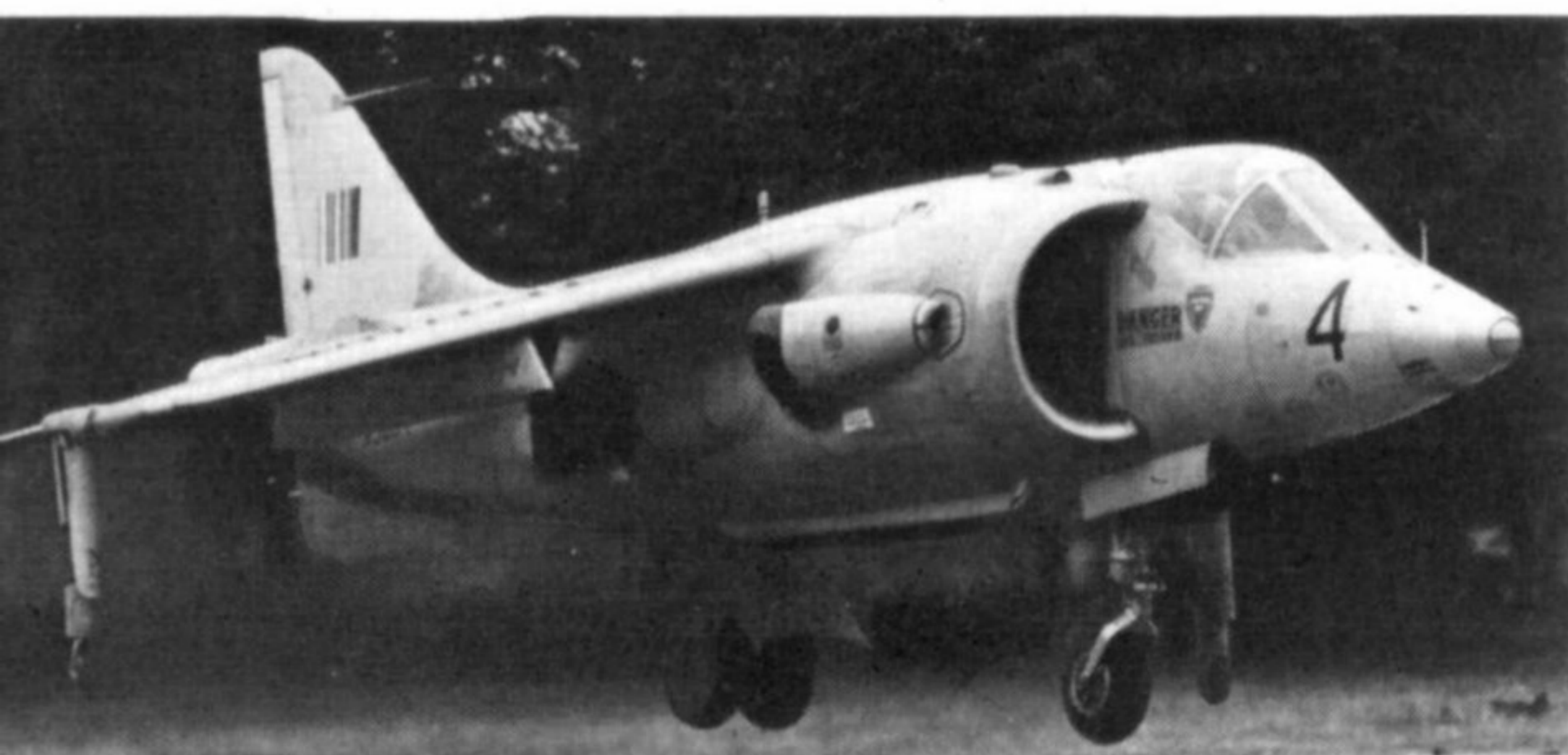
Emphasising the independence of obstacle-free airfields and runways, these pictures show Kestrels dispersed and operating among heavily wooded sites in the neighbourhood of West Raynham, Norfolk. The take-off photo illustrates one of several types of transportable operating platforms tested. Note the addition of wing pylons.
