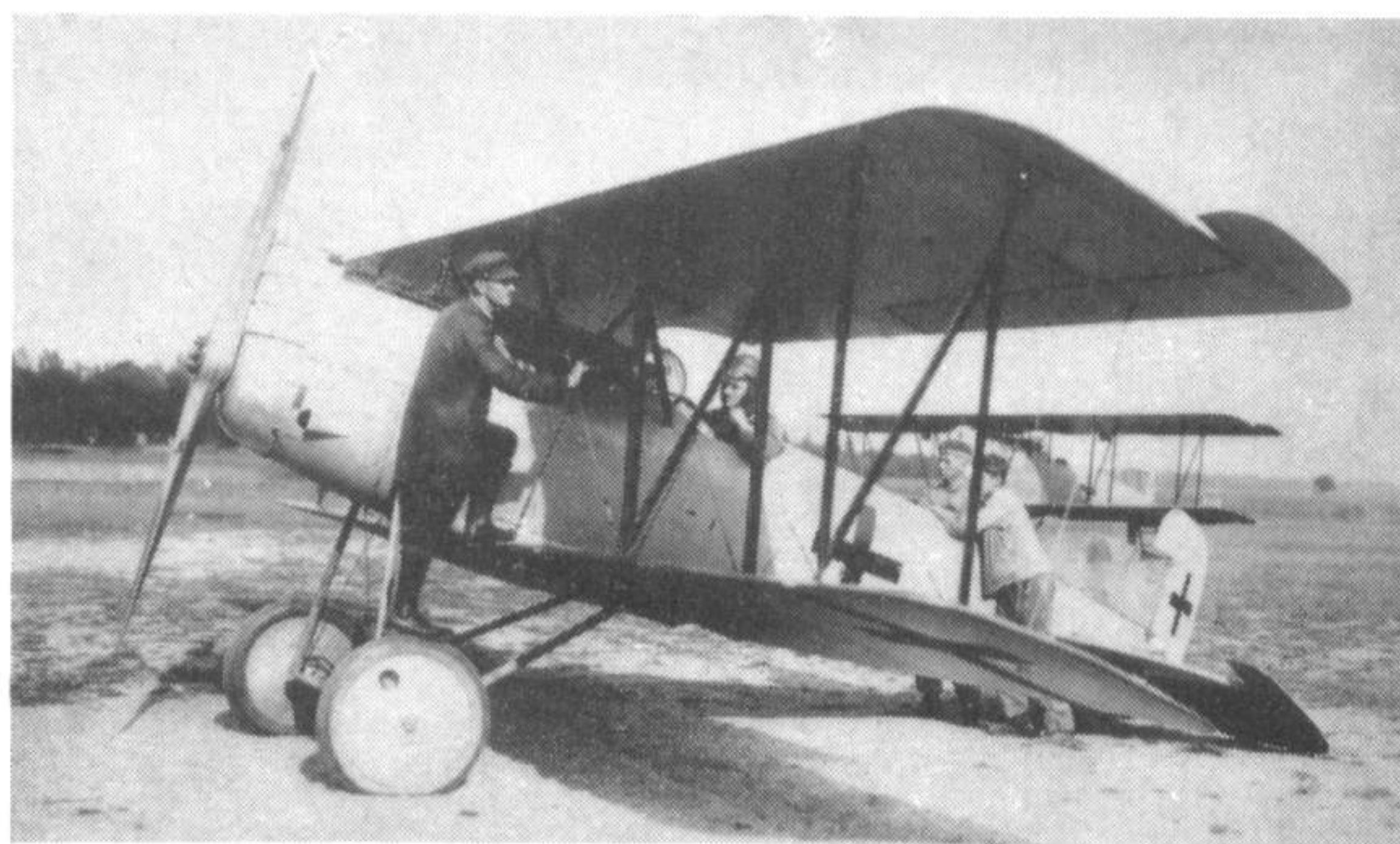
An early production D.XII, with rectangular tail, being readied for a test flight; in the cockpit is Pfalz test pilot Otto Augst.
