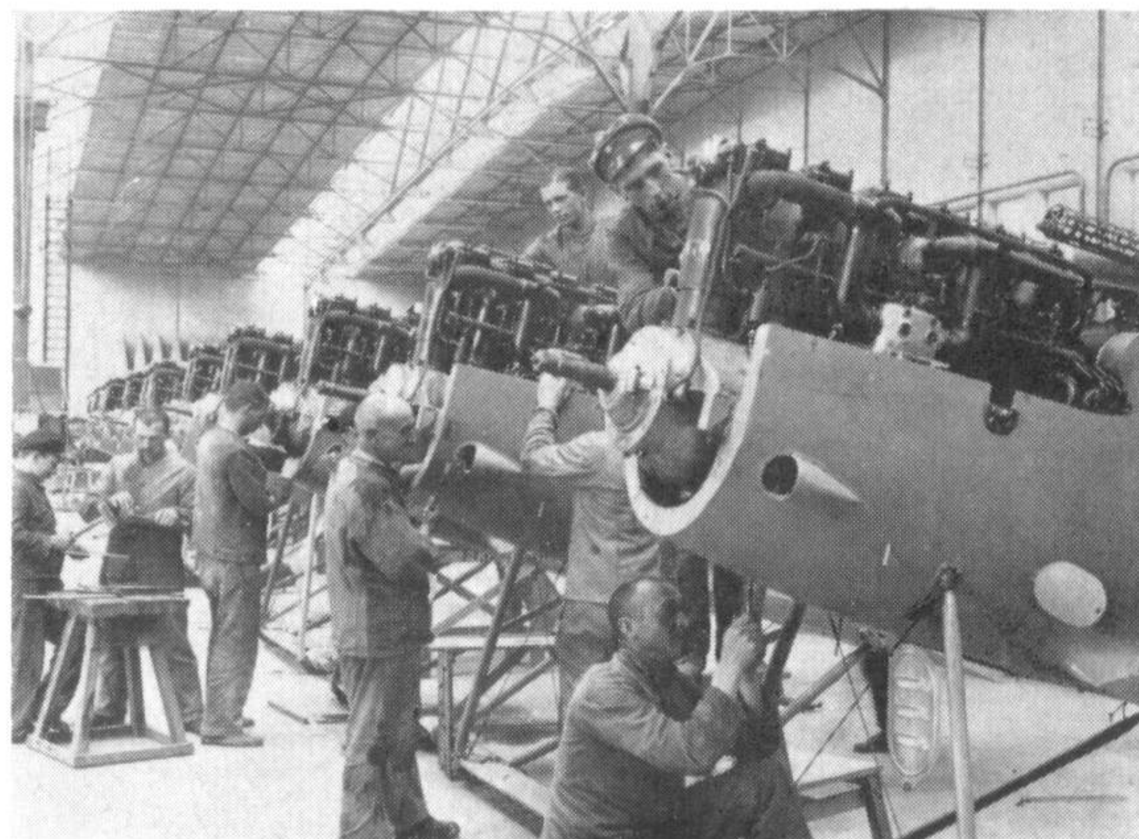
(Left), assembling the lower wing on a D.XII; note lozenge pattern showing through the light blue underside paint. (Right), installing engine components; the worker in uniform is a specialist released from Army service.
