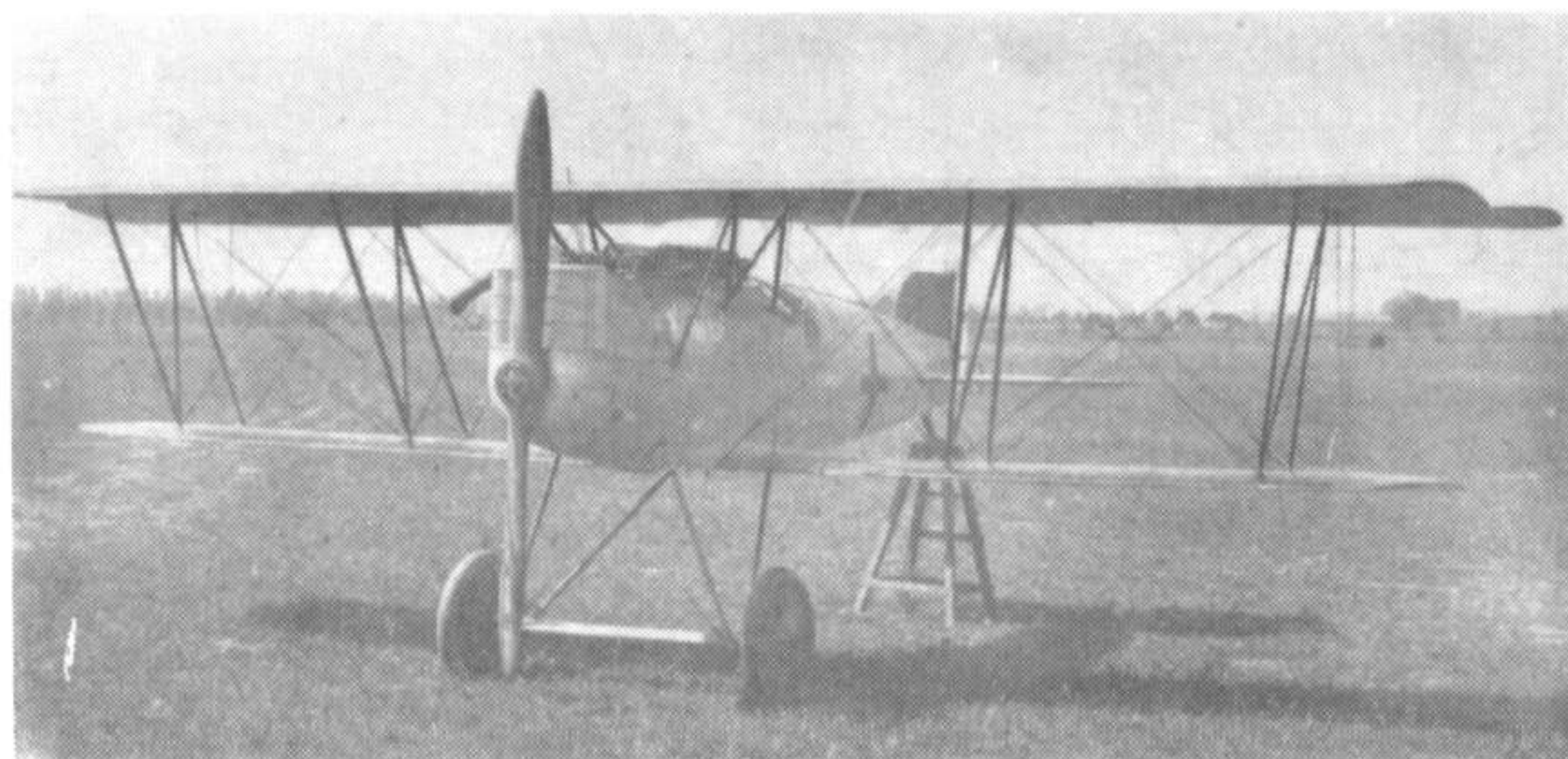
Another early D.XII, without slipstream deflector on radiator; this was fitted to later models to improve cooling efficiency.
