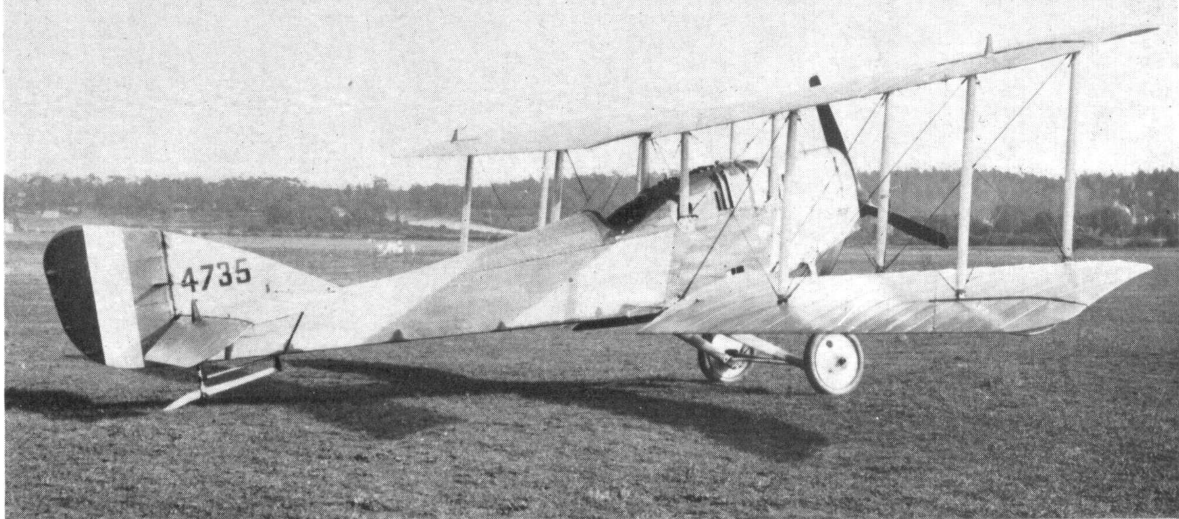
The prototype Martinsyde G.100, 4735, photographed at Brooklands. The original long tail-skid can be seen clearly. (Photo: Imperial War Museum Q57642)
