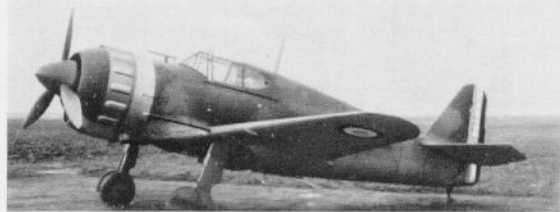
Bloch 152 No. 320 during manufacturers' trials; note absence of armour behind pilot's seat. (Photo: via M. Cristesco)
