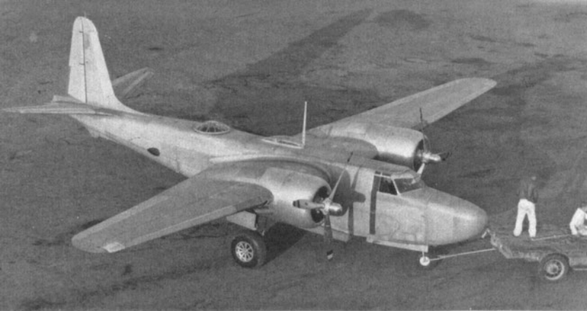
The 7B after the first flight, showing new tail layout; the plexiglass housing aft of the cockpit is an antenna fairing. (Photo via the author)
