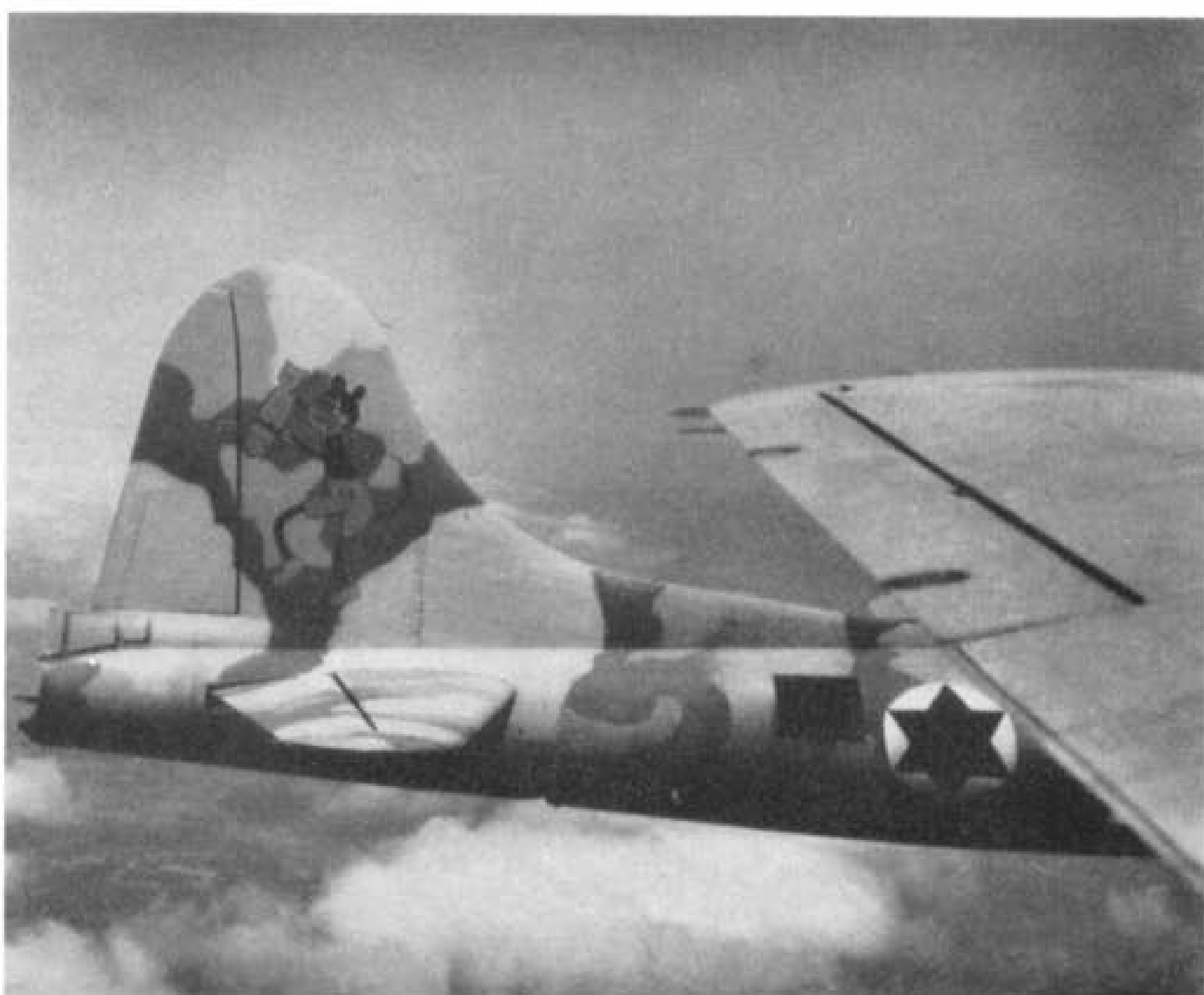
Three B-17Gs were the main long-range bombing arm of the Israel Defence Forces/Air Forces in the 1950s. The Mickey Mouse contrasts with the extensive camouflage. Note the modified tail gun position. (Photos: I.D.F./A.F. viz C. W. Cain)
