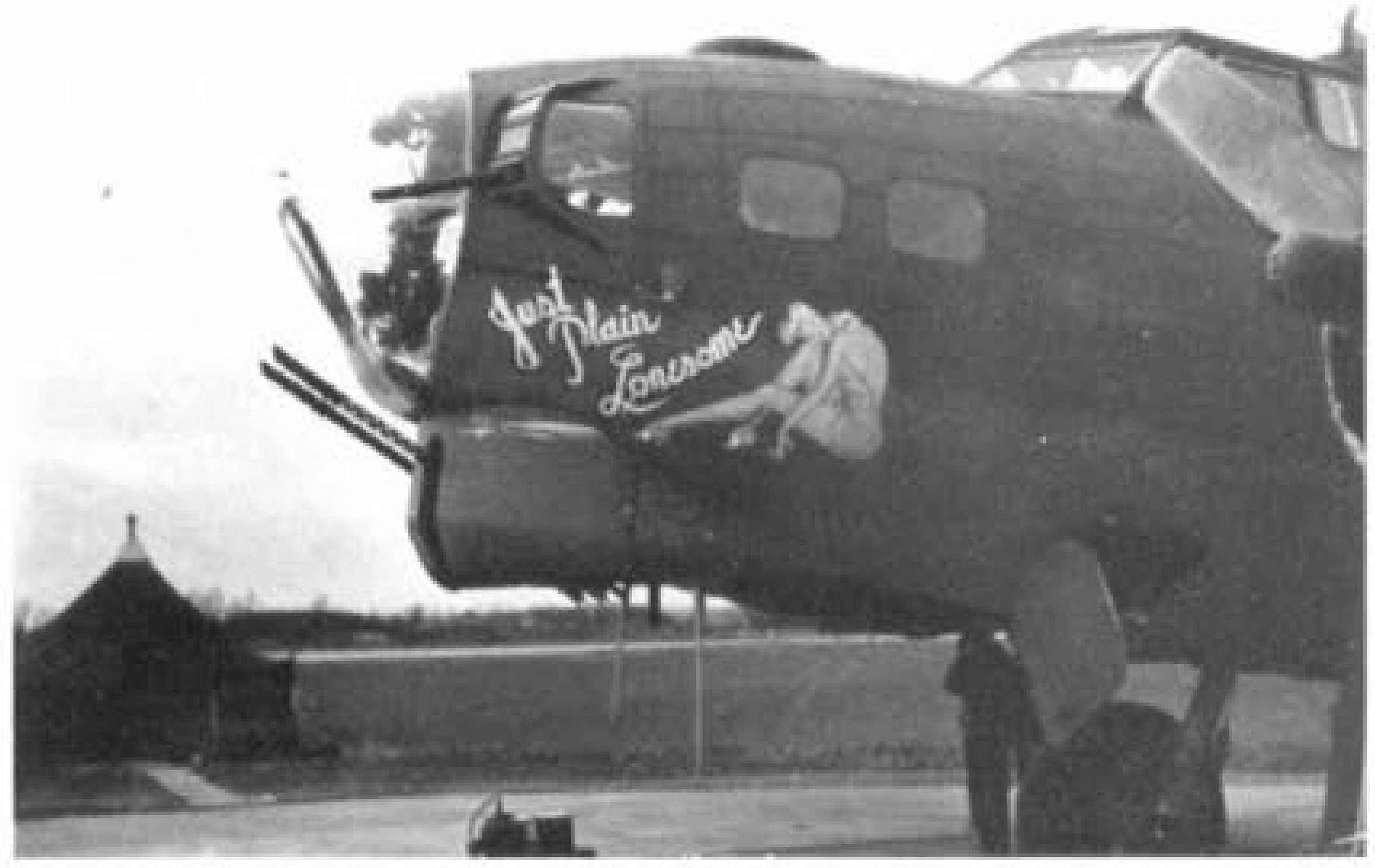
The 91st BG's Pist'l Packin' Mama and Just Plain Lonesome offer comparison between the long and short nose pieces (Douglas and Vega respectively) with the famed Norden bombsight exposed.
