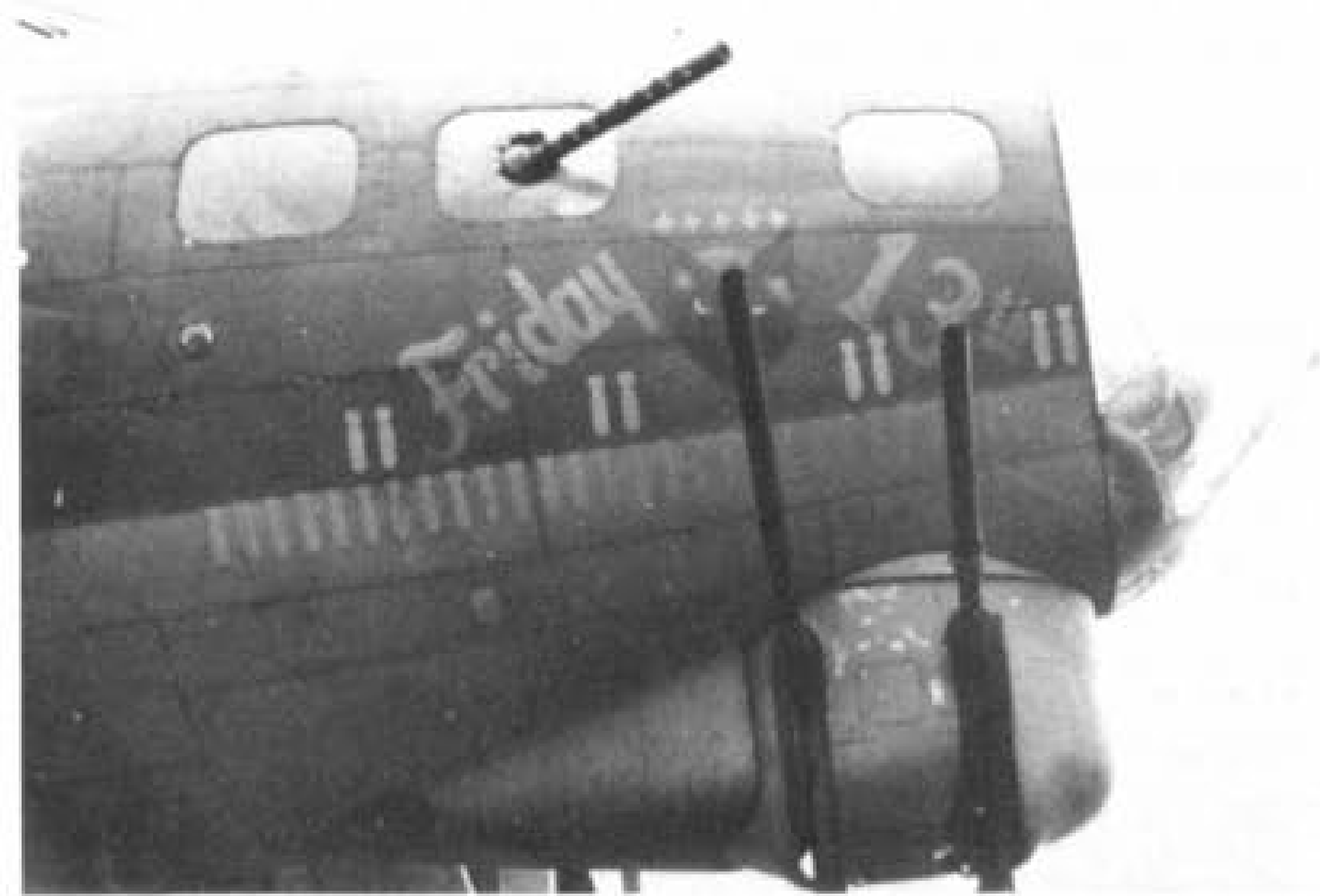
Early Douglas-built B-17Gs, like the 388th BG's Little Willie, were hurried into operational service without cheek guns which left scope for unit improvisation as shown with the 94th BG's Friday 13th.
