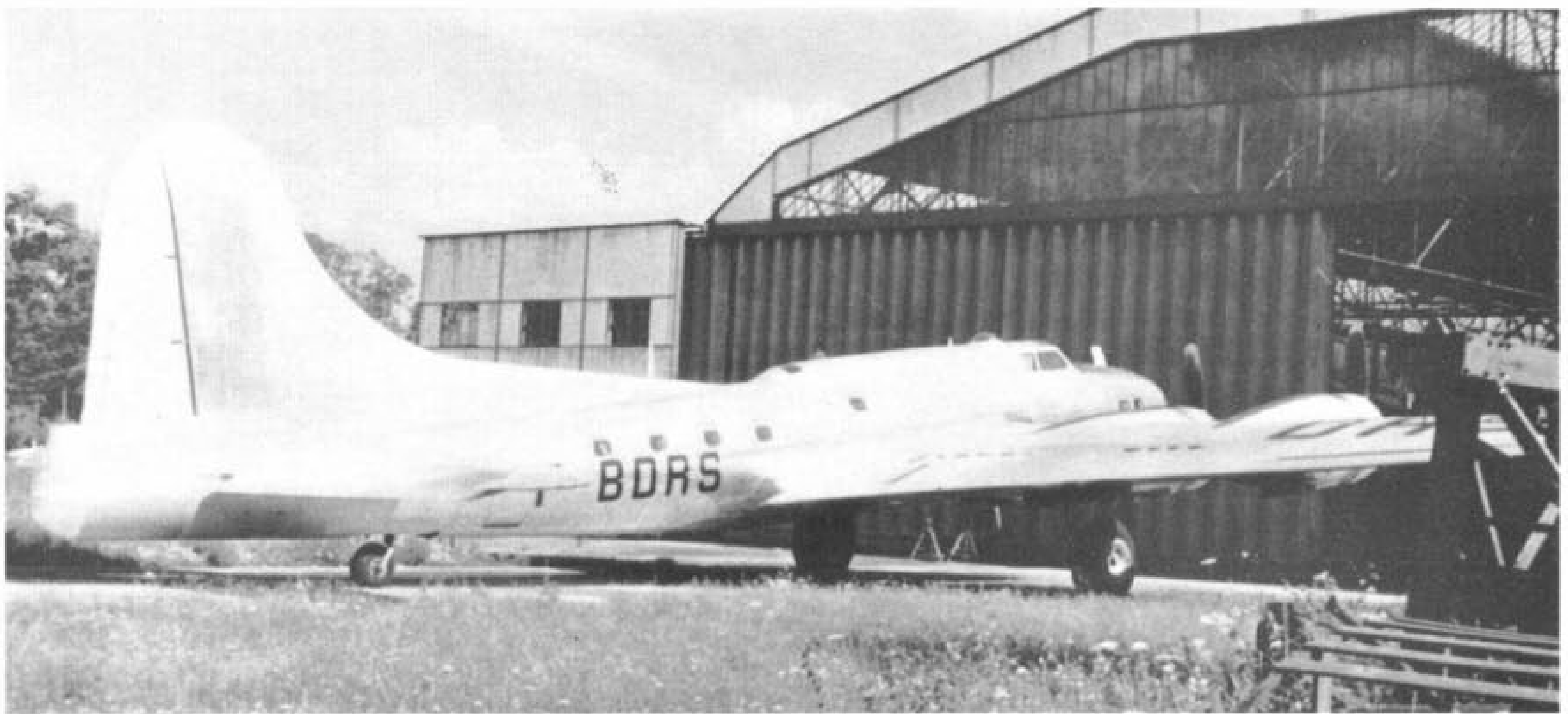
A modified B-17G-95-DL (formerly 44-83735) used by IGN. Tail and waist gun positions have been sealed and extra windows made in the fuselage. (Photo: G. Dufton)
