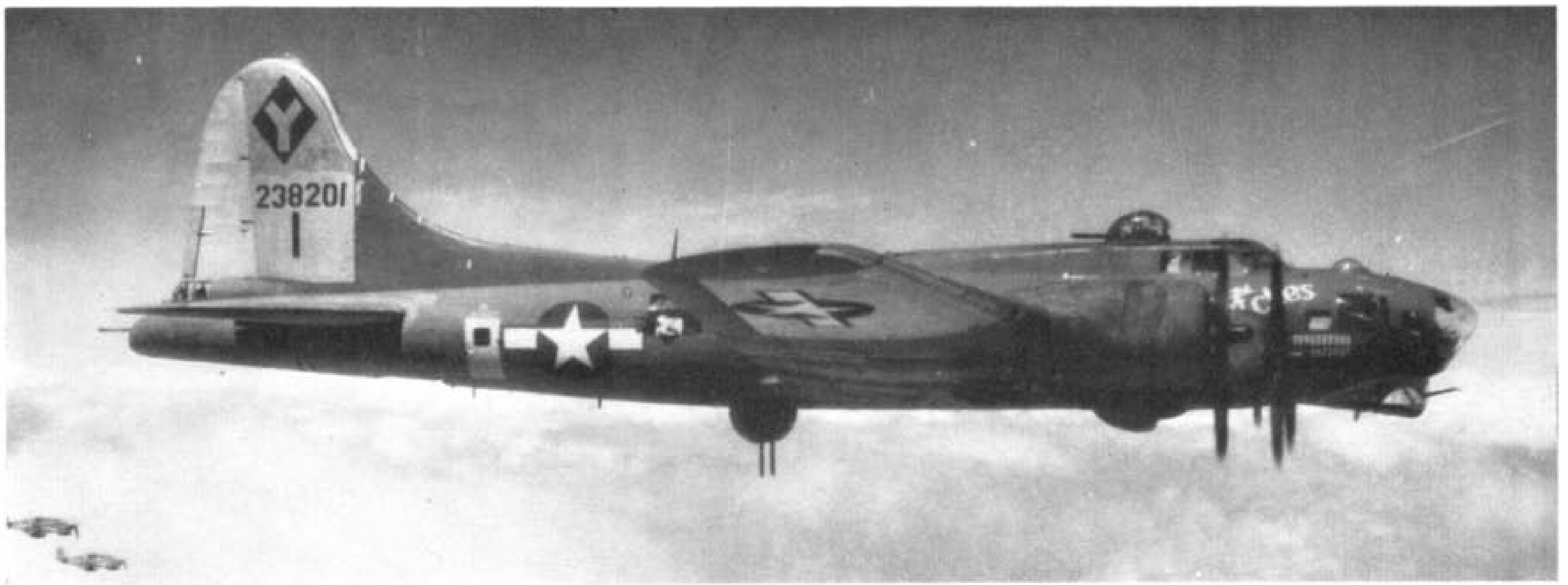
A B-17G of the 346th Bombardment Squadron, 99th BG dubbed 2nd Patches, on route to the U.S.S.R. from Italy during the first Fifteenth Air Force shuttle mission in June 1944. Largest patches are a new "silver finish" fin and rudder and outer wing panel. Note the red and white shark's mouth around the chin turret. (Photo: U.S.A.F.)
