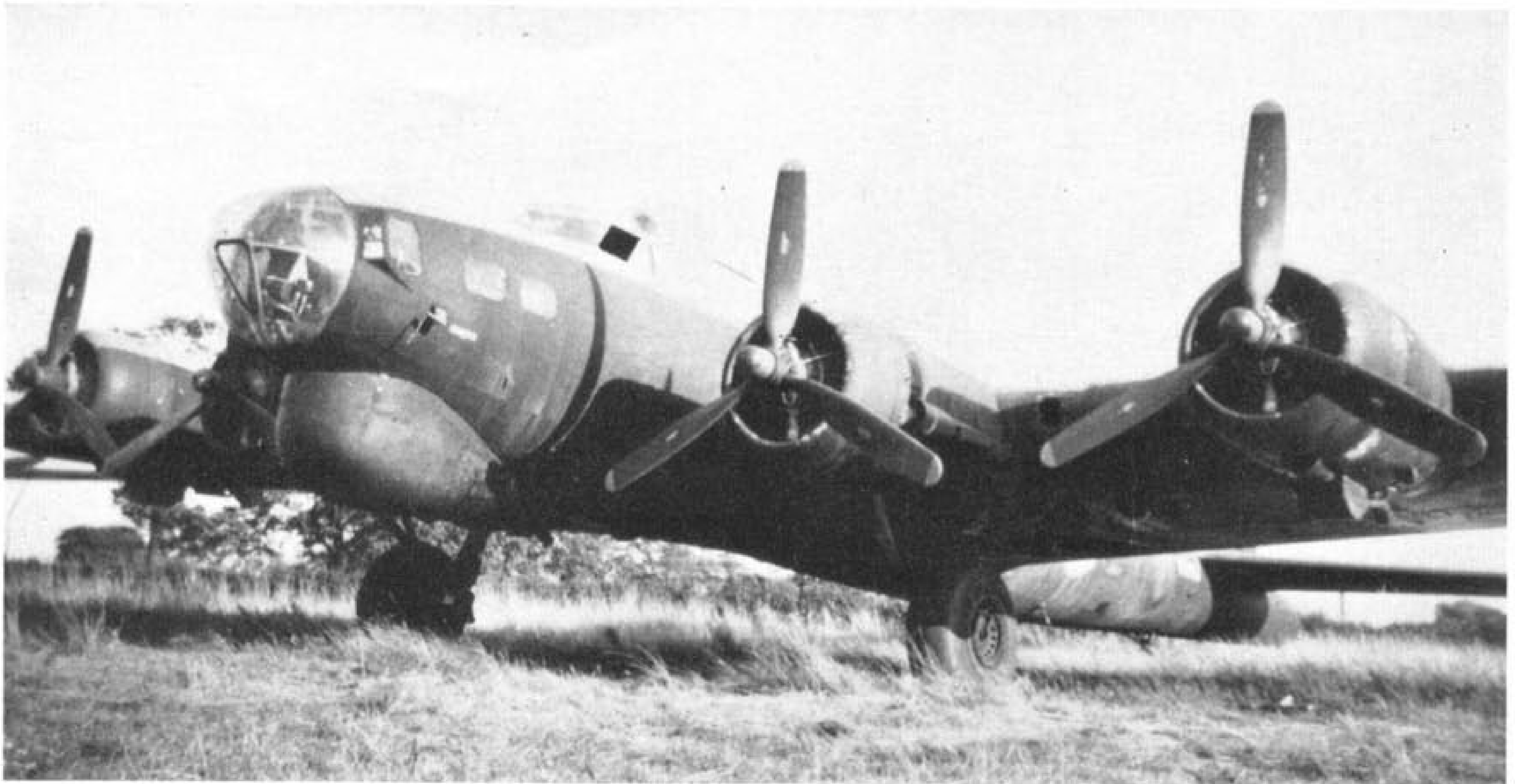
An R.A.F. Fortress III with chin turret replaced by H2S radome. This particular B-17G is believed to have served with No. 214 Squadron in Bomber Command's 100 Group in an RCM (Radio Counter Measures) rôle. (Photo: J. R. Rabbets)
