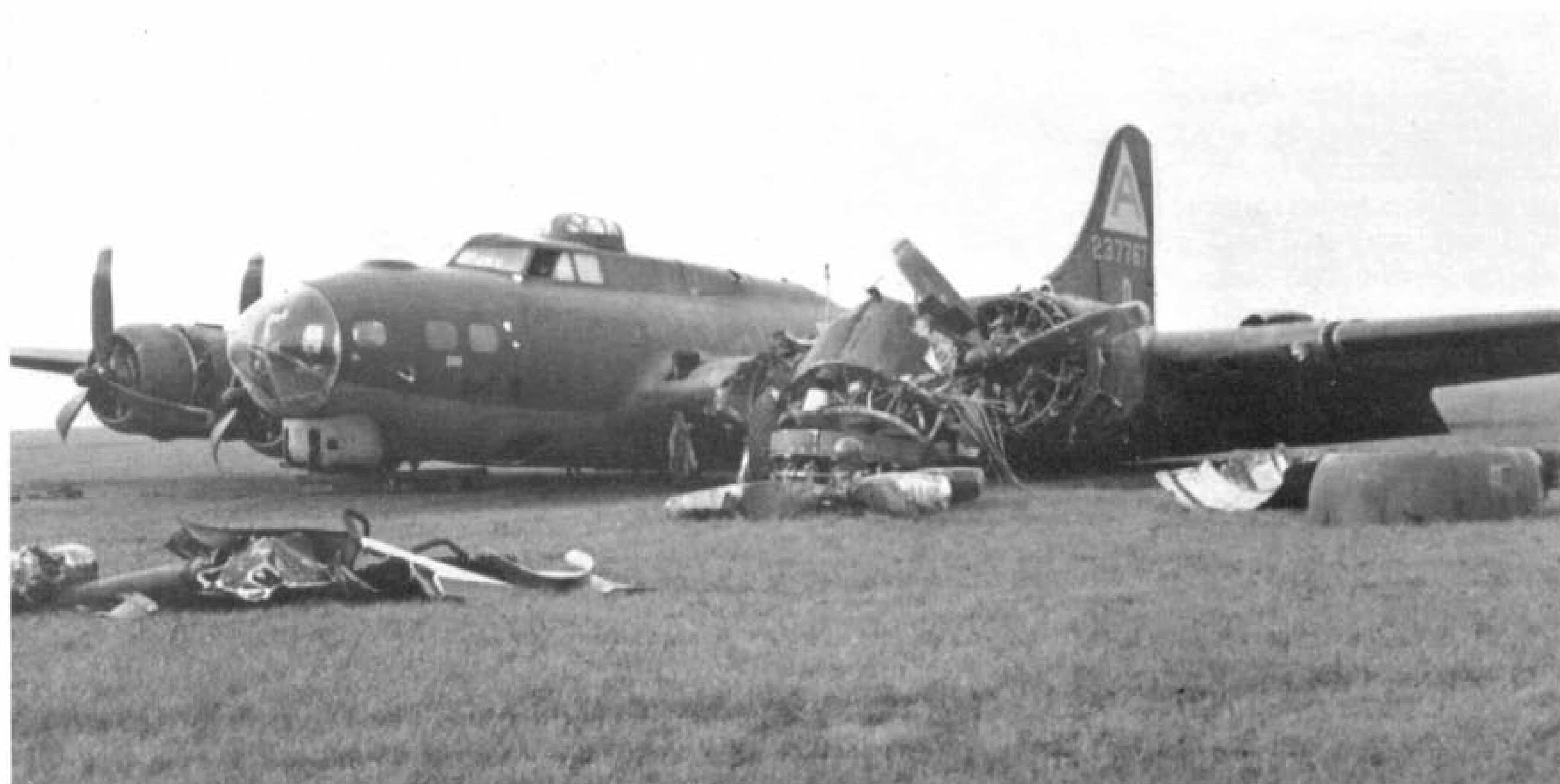
This 91st Bomb Group B-17G (serial 42-37767; code letters LL:D) was classified a total wreck after a wheels-up emergency landing at Cambridge Airport (England) on the afternoon of December 21, 1943. (Photo: U.S.A.F.)
