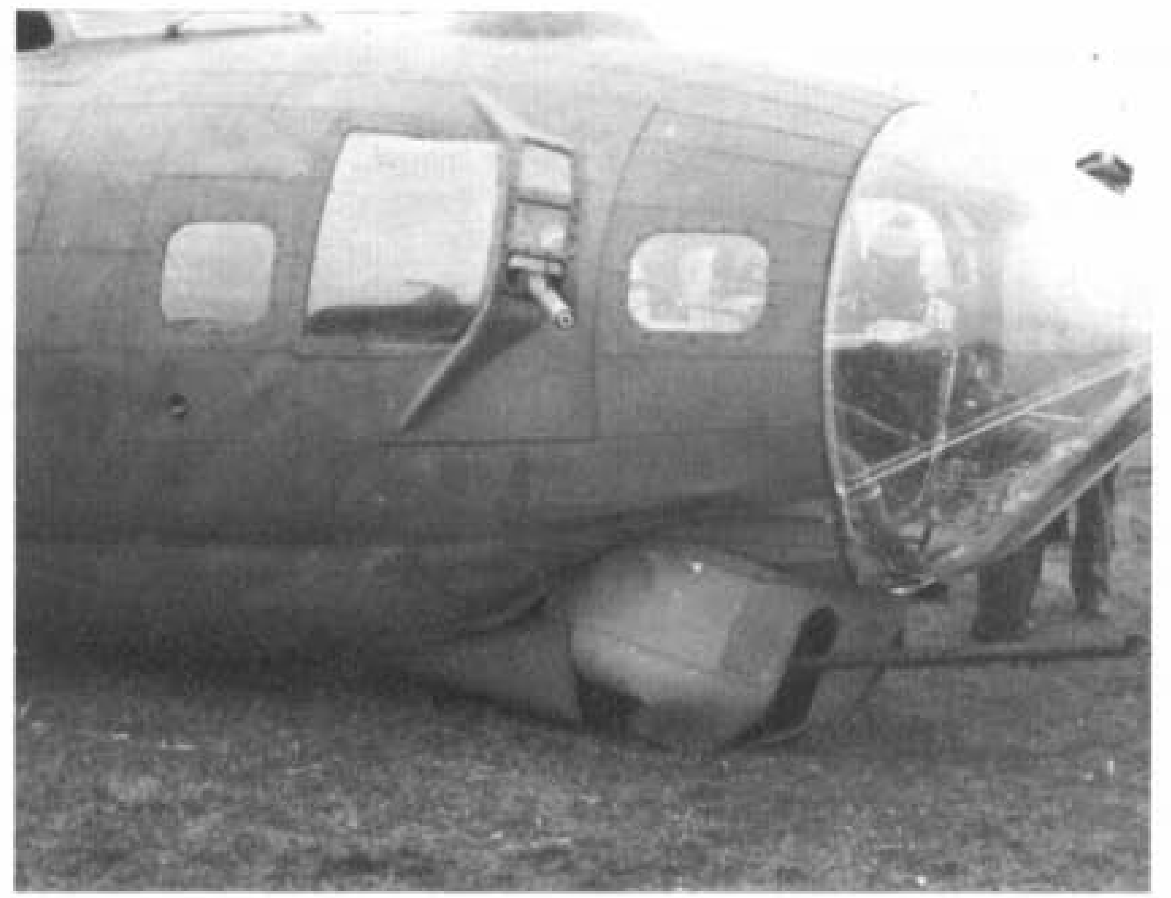
This 447th BG Flying Fortress Hey Mabel! proves the point that a wheels-up landing usually resulted in the chin turret buckling the nose section. (Photo: U.S.A.F.)
