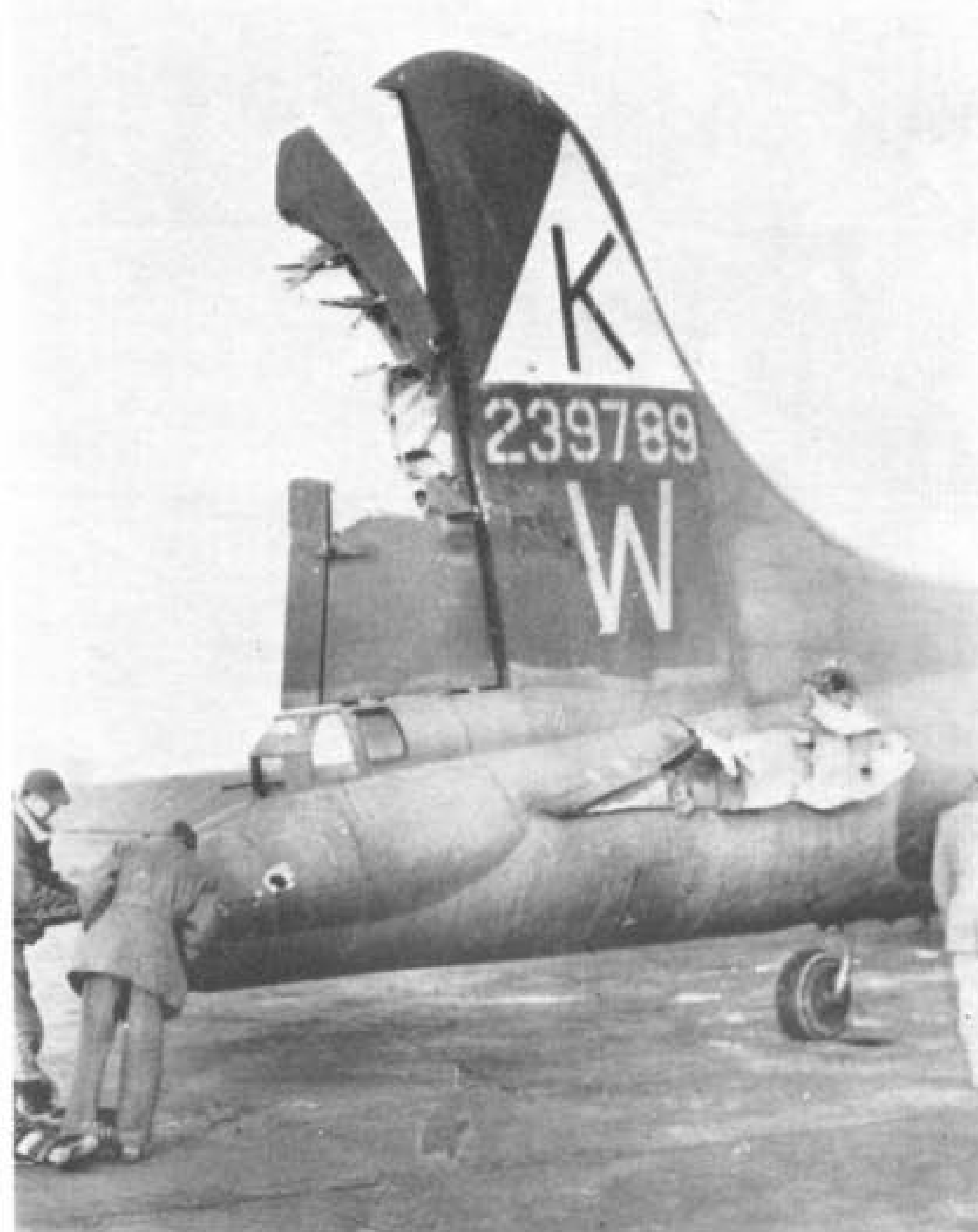
A rocket projectile tore a large hole from the turret of yet another B-17G yet, miraculously, neither the gunner nor the pilots were harmed. (Photo: R. Barnes)
