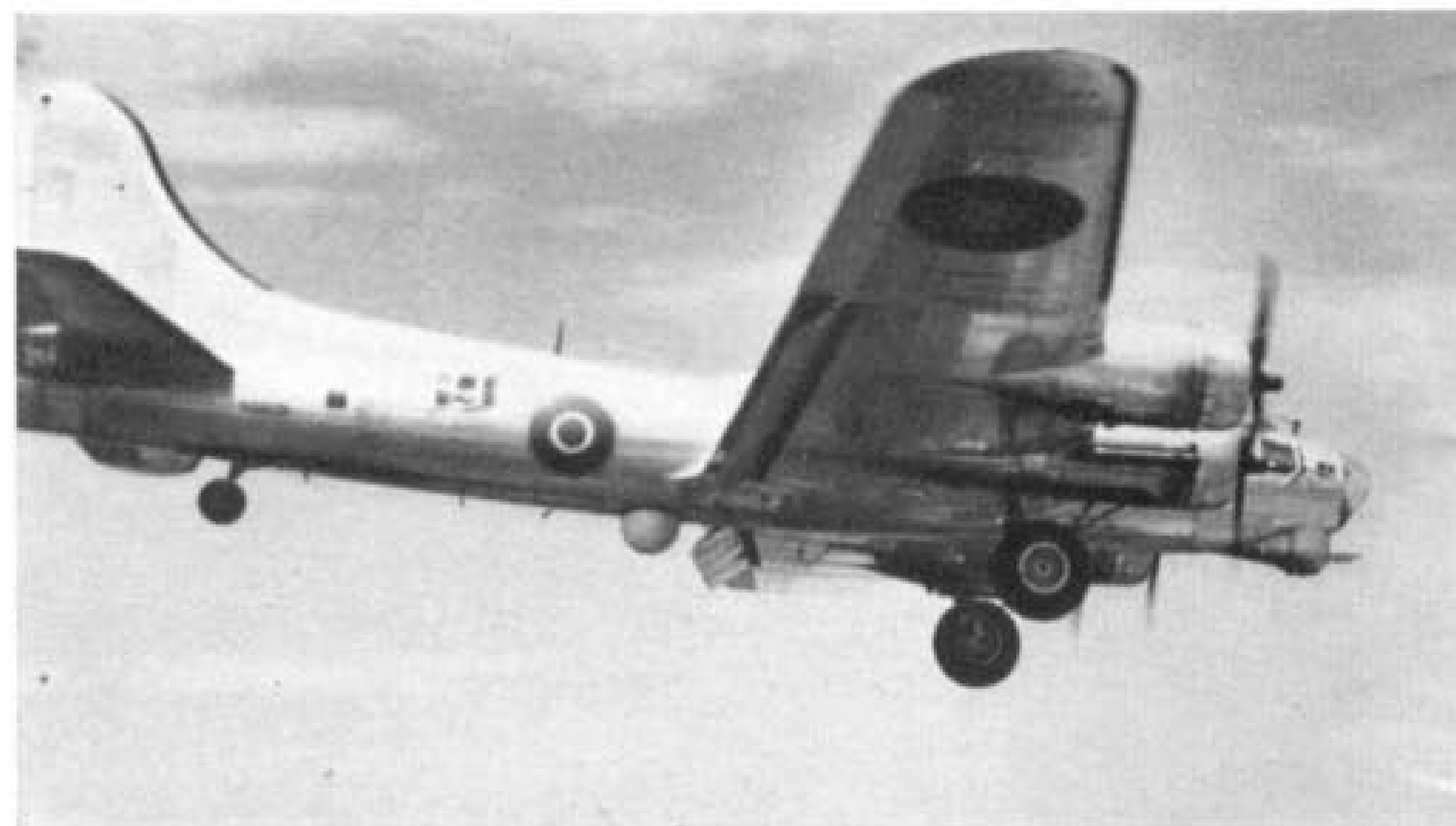
A Lockheed-Vega B-17G-VE about to land at Denver (Colorado, U.S.A.) prior to delivery to R.A.F. Bomber Command (serial HB 809). Noteworthy are the retracted H2X radome and the "barred"-type waist window. (Photo: W. T. Larkins, A.A.H.S.)
