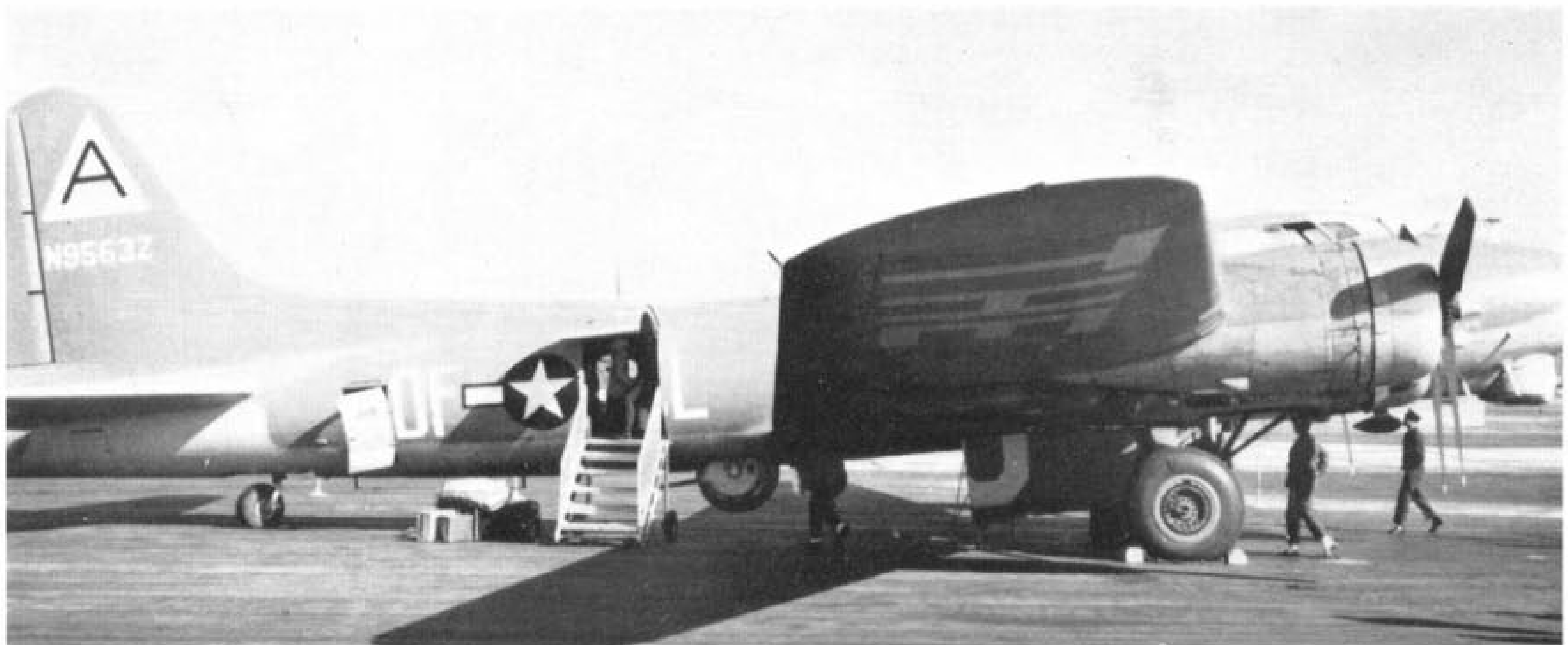
Civil B-17G N9563Z (formerly 44-83563) returned to the U.S., retaining its warpaint for some weeks to advertise the film. Normally used for freight, this aircraft had a special door at the point where the right waist window was once situated. (Photo: R. C. Mikesh)
