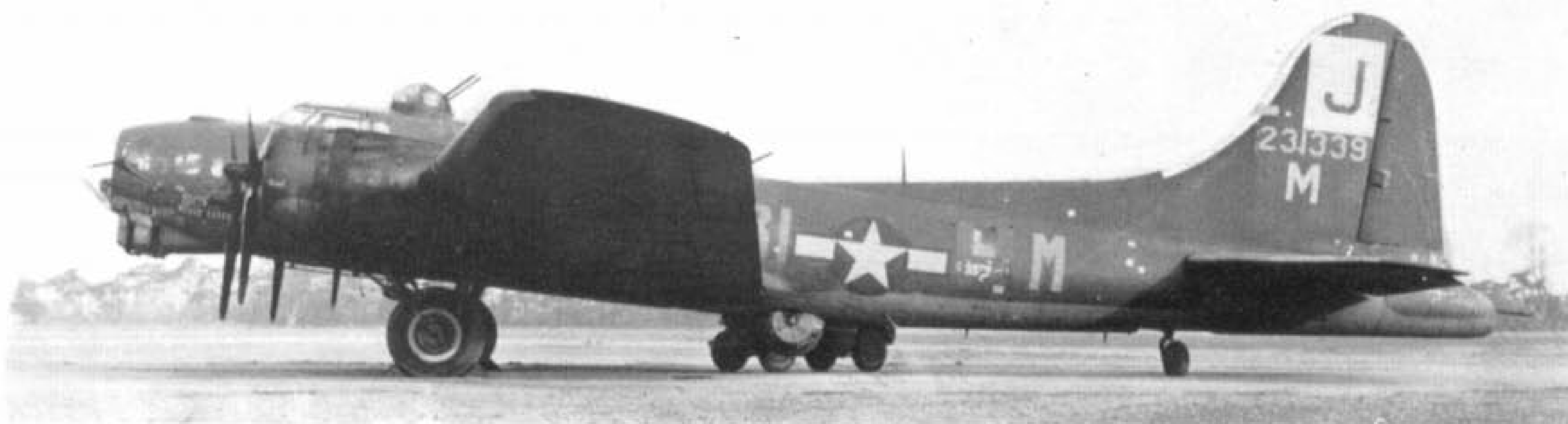
Compare two types of tail gun installations. Above: A 390th Bomb Group B-17G-15-BO and (below) a 96th BG B-17G-30-DL. The "Cheyenne" gun position in 42-38133 was one of the earliest of this experimental installation. (Photos: U.S.A.F.)
