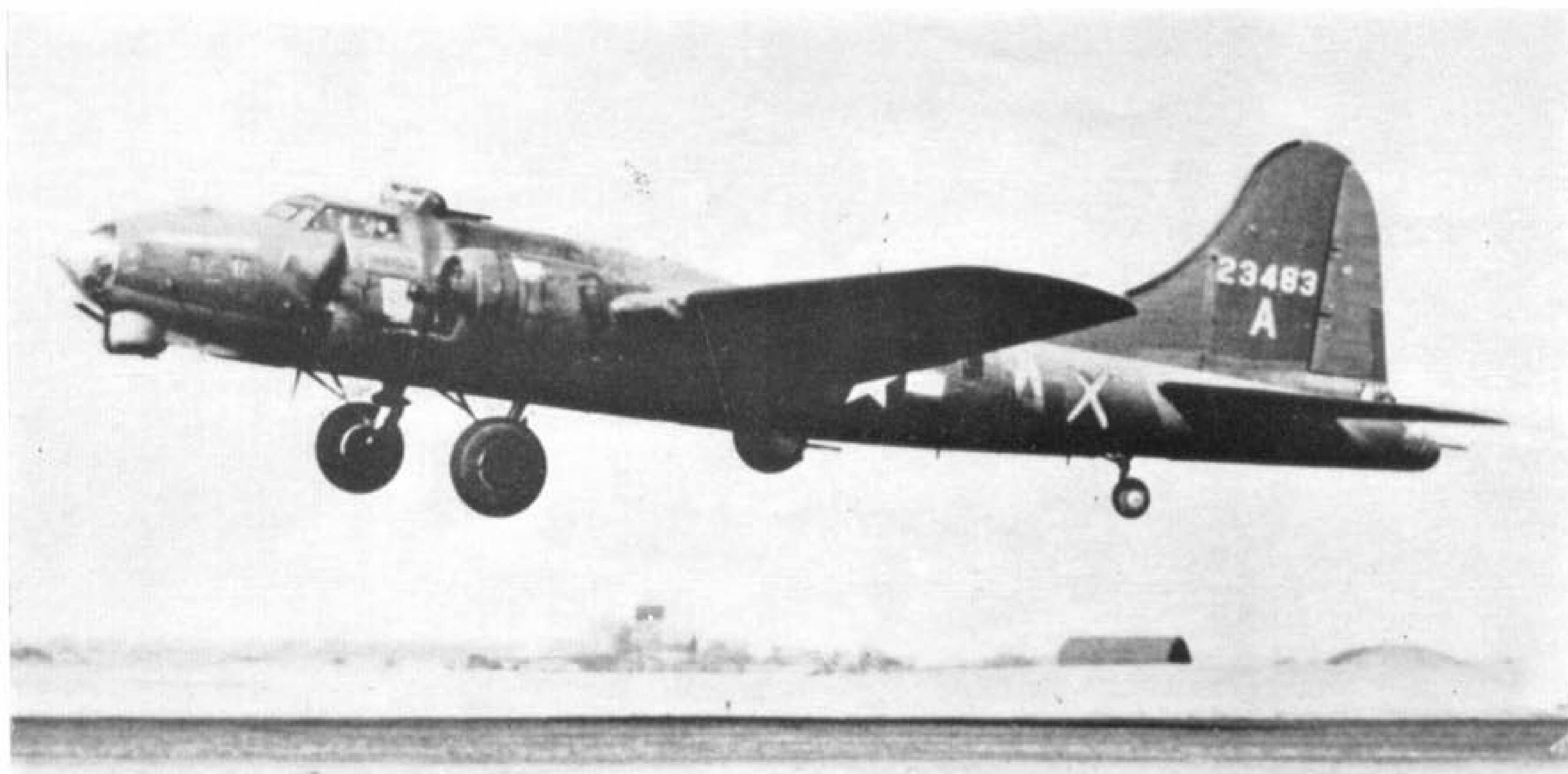
The first Douglas (-DL) series-production Flying Fortress (B-17F-70-DL) to have the distinctive "chin" turret takes-off from an English airfield Spring 1944. (Photo: U.S.A.F.)
