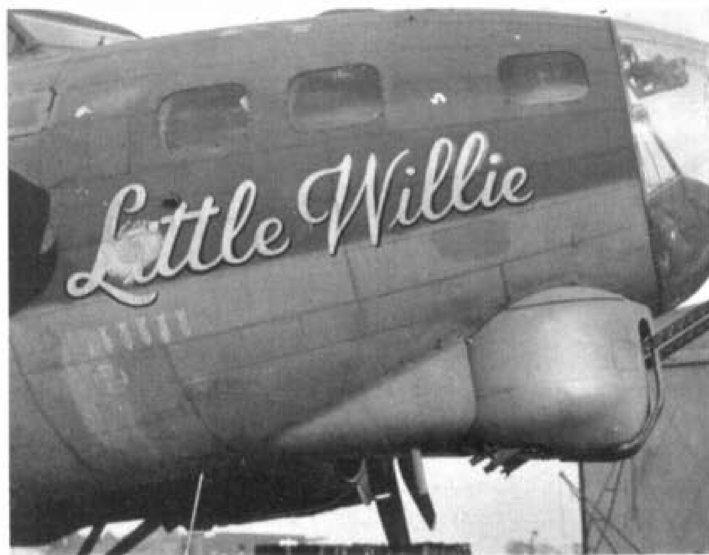
Early Douglas-built B-17Gs, like the 388th BG's Little Willie, were hurried into operational service without cheek guns which left scope for unit improvisation as shown with the 94th BG's Friday 13th.
