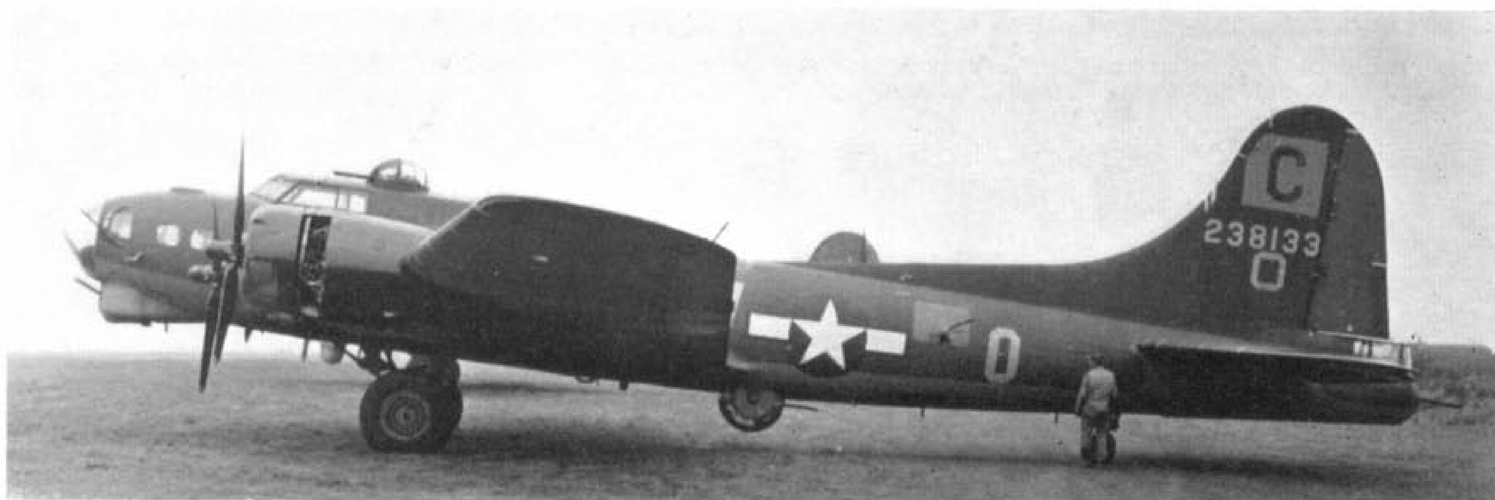
Compare two types of tail gun installations. Above: A 390th Bomb Group B-17G-15-BO and (below) a 96th BG B-17G-30-DL. The "Cheyenne" gun position in 42-38133 was one of the earliest of this experimental installation. (Photos: U.S.A.F.)
