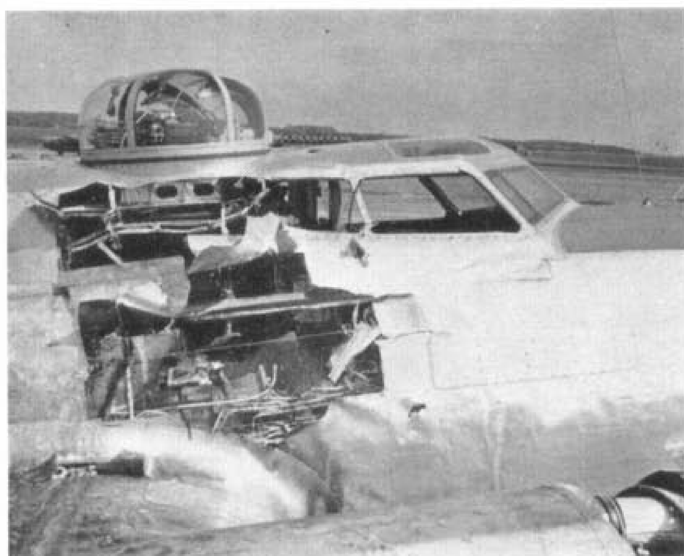
A rocket projectile tore a large hole from the turret of yet another B-17G yet, miraculously, neither the gunner nor the pilots were harmed. (Photo: R. Barnes)
