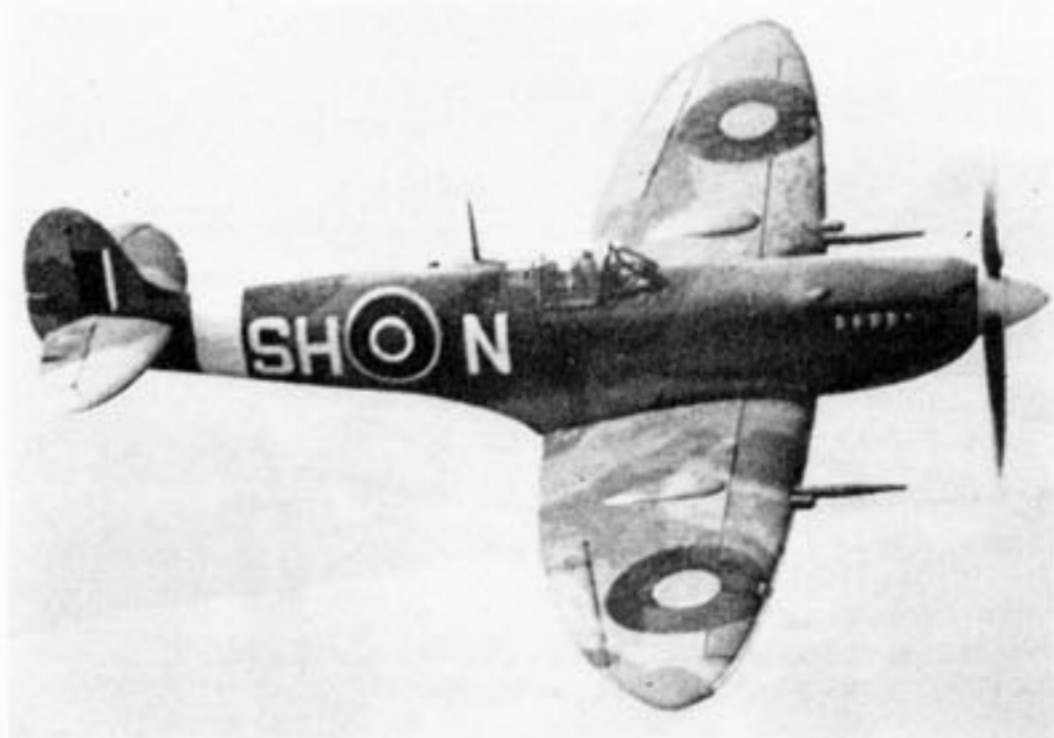
This photograph of July 1942 shows an example of an F. Mk. IX C of No. 64 Squadron—the first unit to receive Mk. IXs. Along each outboard wing leading-edge is the yellow strip which was adopted (like the yellow-tipped propeller blades) to assist ground crews when working around Spitfires in the pre-dawn darkness. Note also the larger cannon blisters in place of the more familiar narrow-chord, tear-drop blisters. (Photo: via M. Garbutt)
