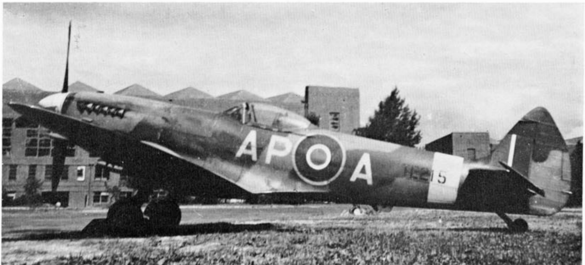
S/Ldr. G. R. S. McKay's Spitfire Mk. IX E (TE215) of No. 130 Squadron at Odiham in 1946. AP-A was one of the few Mk. IXs to have the tear-drop cockpit canopy fitted.
