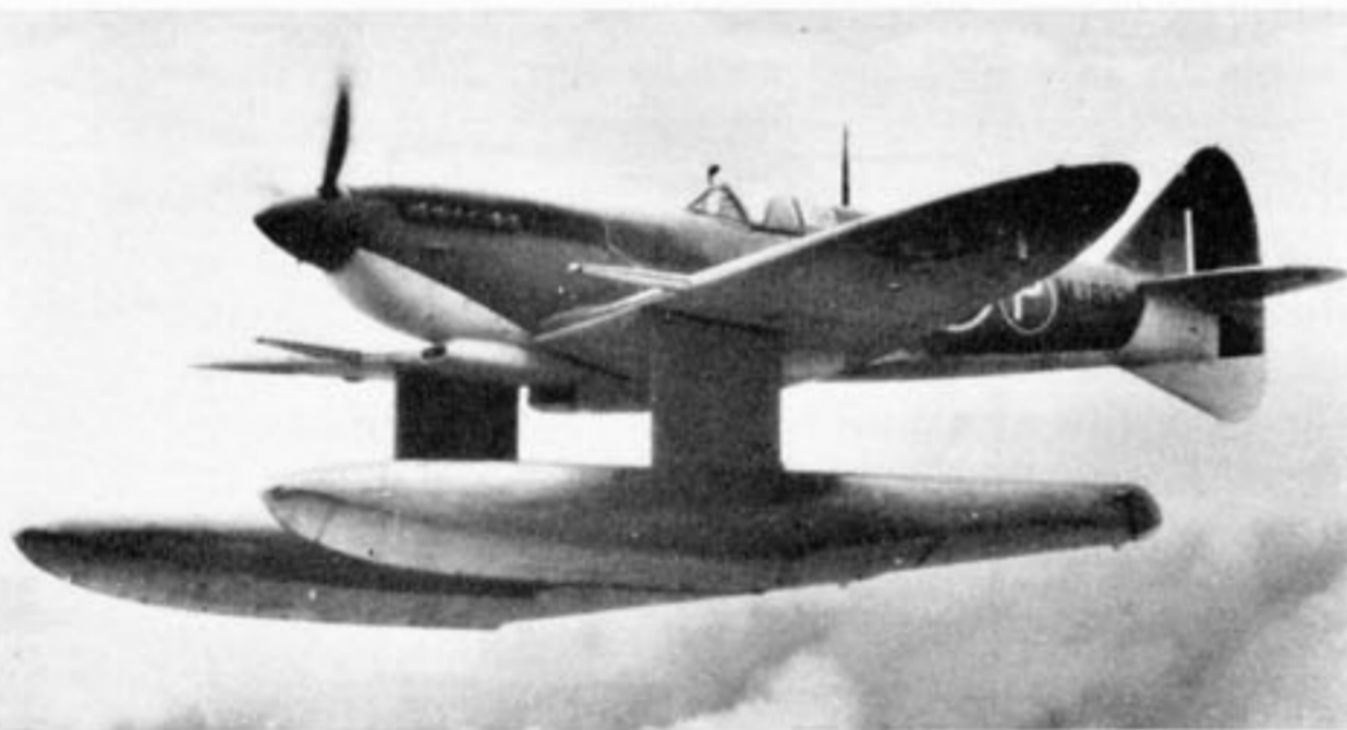
The experimental floatplane Mk. IX B (MJ892) on a flight from Hamble in 1943. Note revised tail unit. (Photo: via Bruce Robertson)
