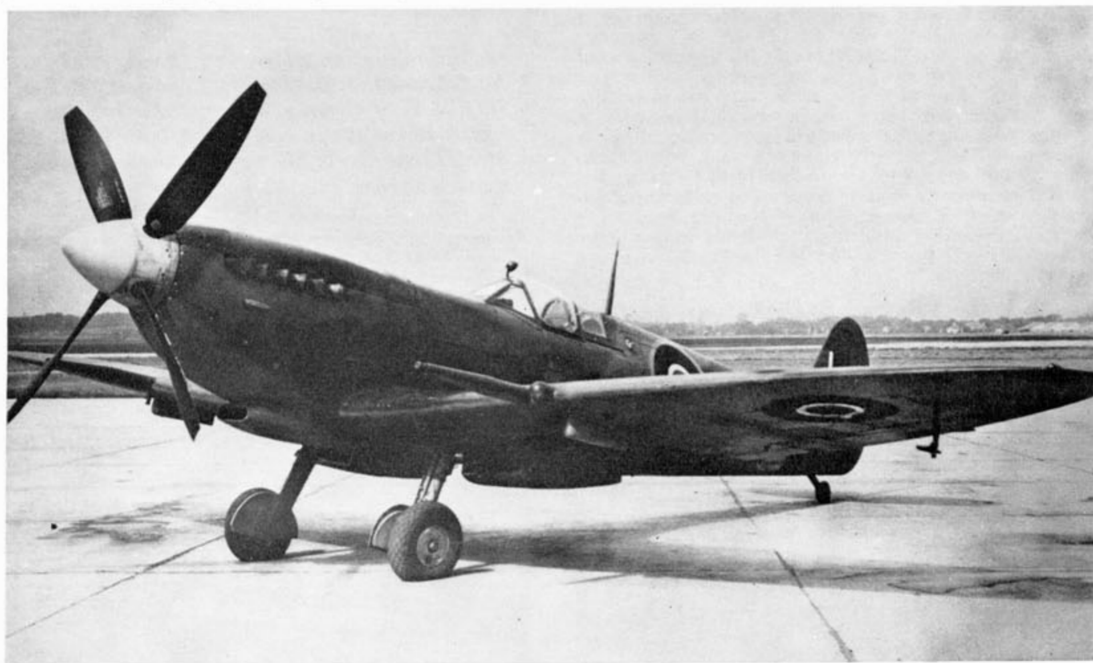
The experimental Spitfire Mk. IXC (MK210) at Wright Field, U.S.A., between May and June 1944, showing the underwing carriers for tests on auxiliary drop-tanks to improve range. (Photo: via E. N. Hooten)
