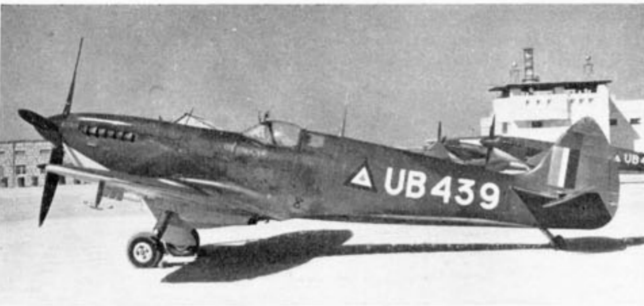
Ex-I.D.F./A.F. Spitfire Mk. IX Es of the Union of Burma Air Force with rocket launch points—three to each wing. Period early 1955. (Photo: Capt. A. P. Bishop)
