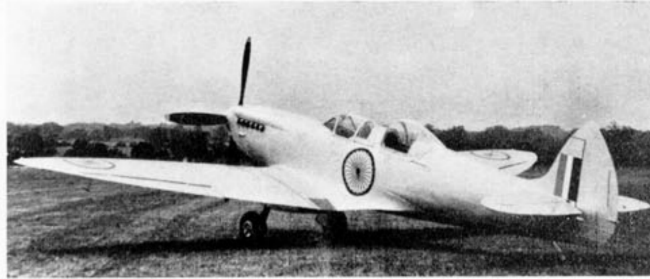
One of ten Spitfire Mk. IX two-seat trainers sold to the Indian Air Force circa 1946. (Photo: Hawker Siddeley)
