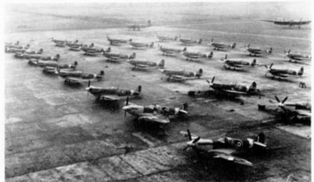
Spitfire Mk. IX Es awaiting collection at the Castle Bromwich factory in 1944. Aircraft in the front row include (right to left): NH432, NH311, NH419, NH45 and NH425. Some cowlings, wing fillets, ailerons and tailplanes require final camouflage. (Photo: via Bruce Robertson)
