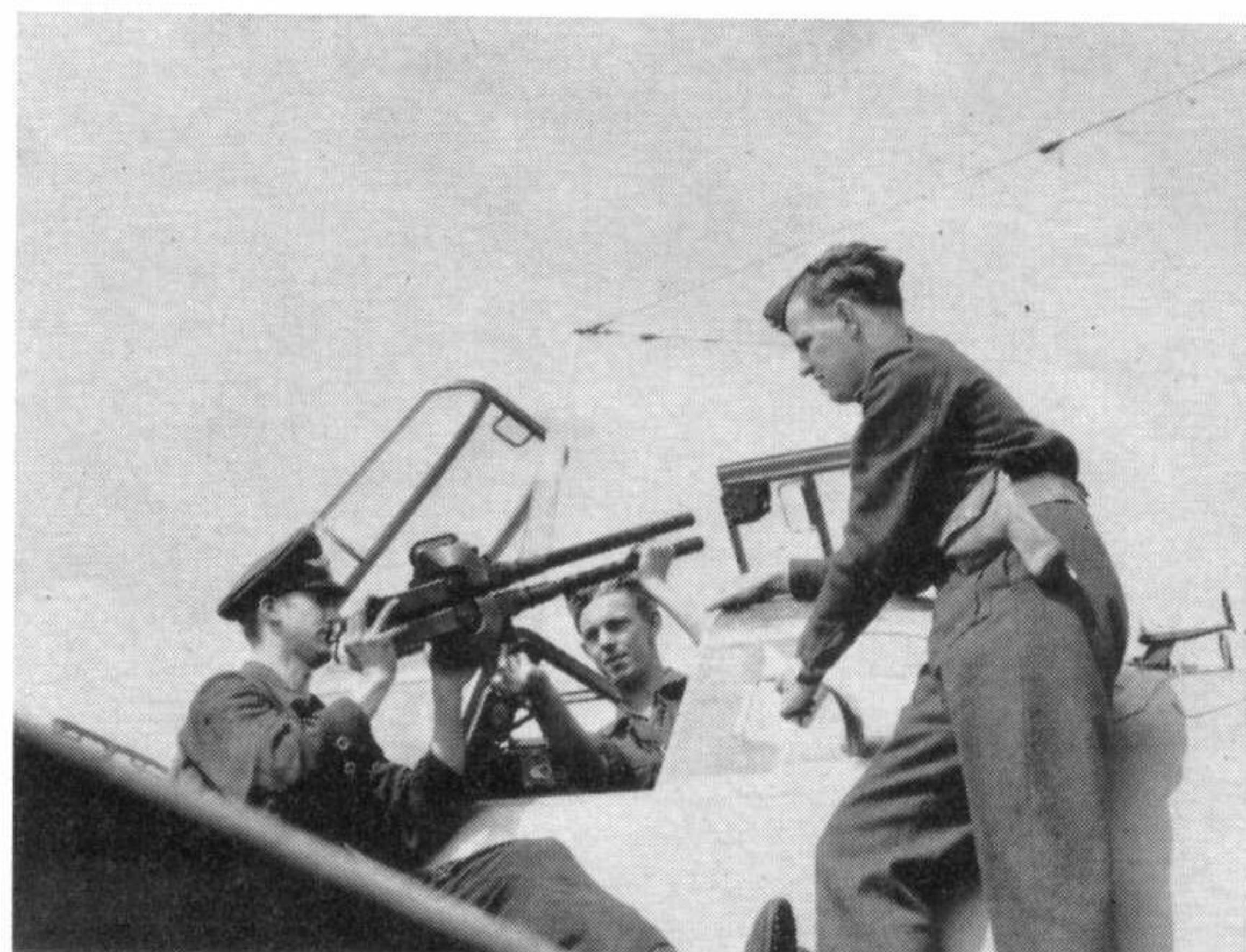
Under entirely new management. (Left) Luftwaffe ground crewmen paint R.A.F. markings on a Bf 110 after the war. (Below) An R.A.F. officer supervises the removal of the rearwards-firing twin-gun MG 81 installation. (I.W.M.)
