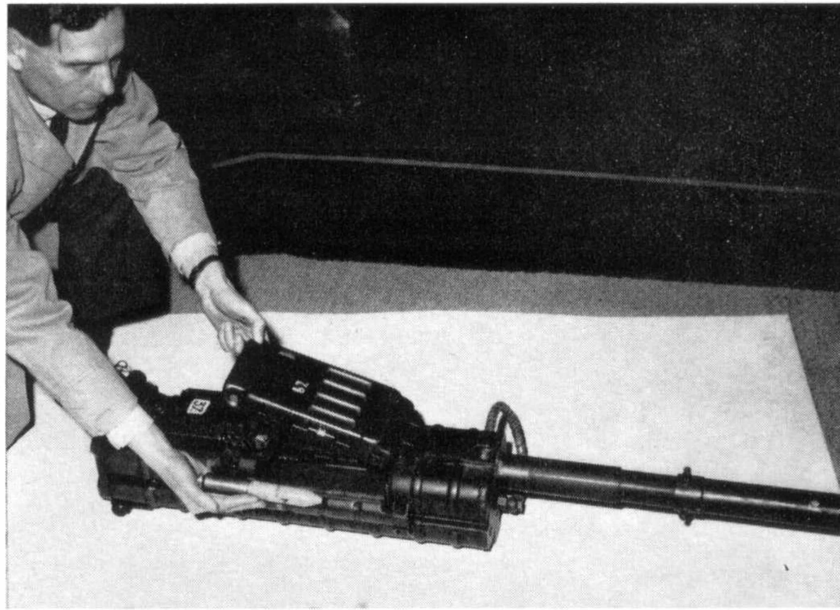
(a) Cause—the 30 mm. MK 108 cannon, seen here with one of the explosive rounds it fired. This weapon was fitted in the upper nose position of the majority of Bf 110s which saw action during the latter part of the war. (b)—and effect. The damage to this Spitfire was caused by a hit from a single explosive round from an MK 108, fired during a test on the ground.
