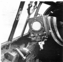
Control unit of the Naxos homing device, which picked up radiations from the British H2S blind-bombing radar set. Note the belt of ammunition, feeding the rear-wards-firing guns.
