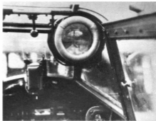
Eye piece of the Spanner infra-red telescope, fitted to a few Bf 110s. The device was intended to enable the pilots to home on to the infra-red emissions from the bombers' exhausts; it did not prove very successful. (Fritz Trenkle)
