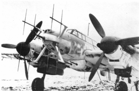
Another view of the FuG 212 and SN-2 aerial; note the under-belly gun pack containing two 20 mm. MG 151 cannon. (Franz Selinger)
