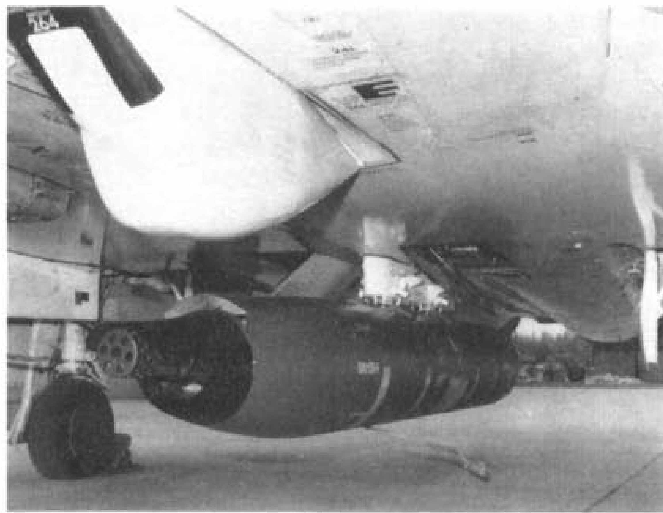
This time located on the centre hardpoint of a R.A.F. F-4M is a SUU-23/A 20-mm. cannon unit, while projecting from the fuselage itself in the foreground is a camera pod. (Photo: Ministry of Defence)
