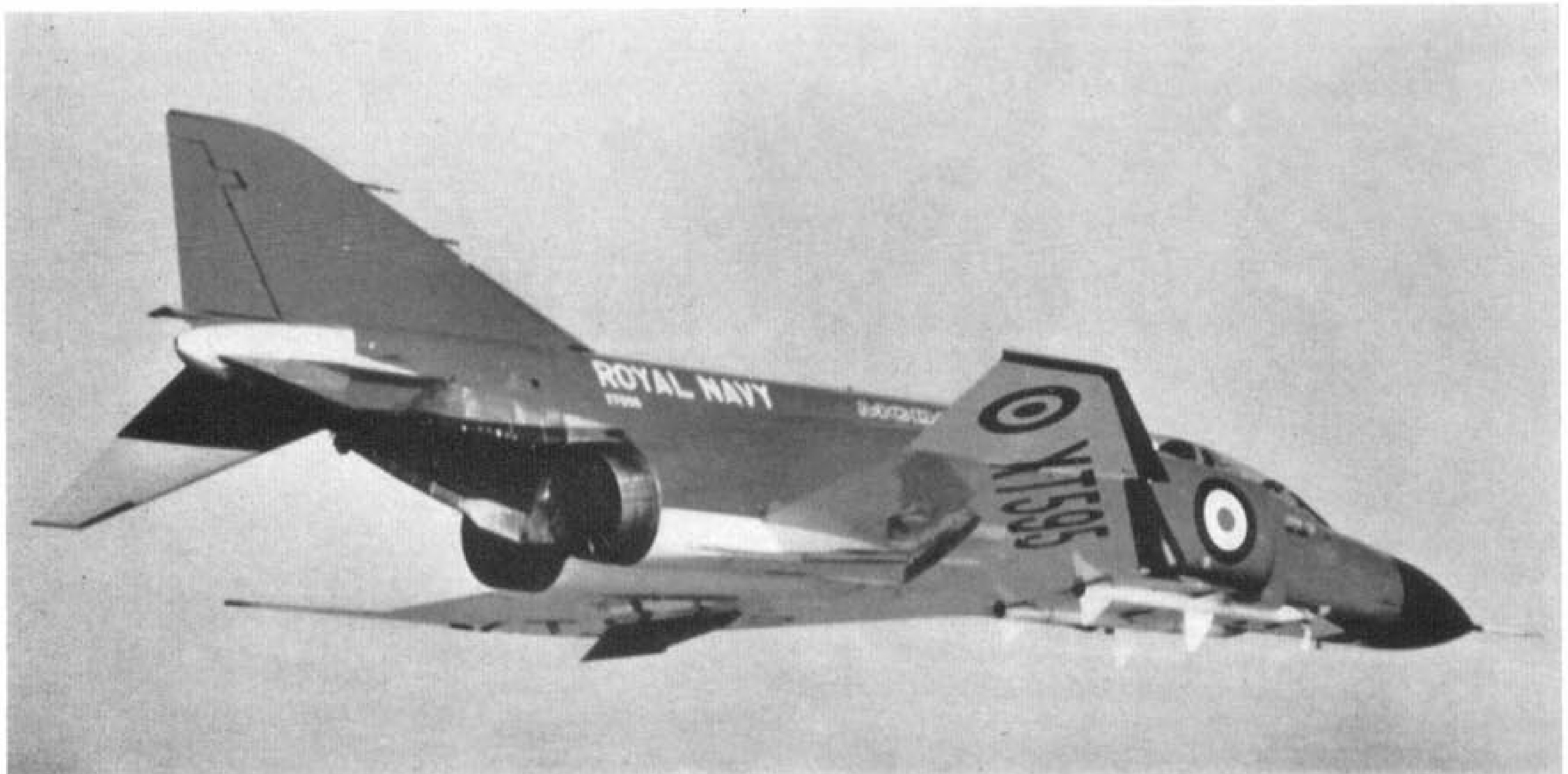
XT595, the first F-4K for the Royal Navy (in fact a YF-4K embodying a high proportion of U.S. equipment) photographed on its first flight on June 27, 1966. Note the protruding leading edge of the outer wing panels (common to all F-4s) and the two Sparrow III radar-guided air-to-air missiles beneath the forward fuselage. (Photo: Rolls-Royce)
