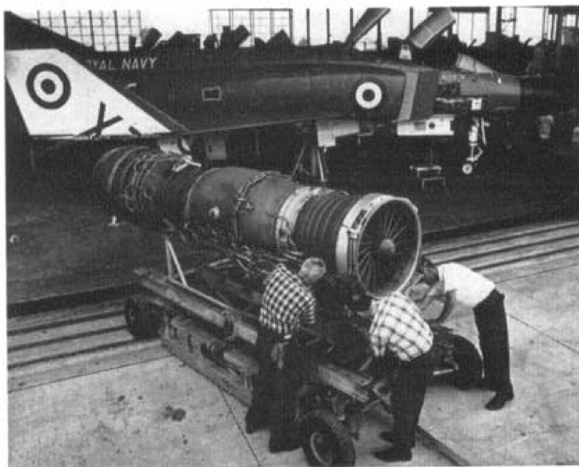
This Rolls-Royce Spey-25R turbofan is about to be installed in a Royal Navy F-4K Phantom at McDonnell Douglas' Lambert Field plant. The new engine required enlarged engine bays and revised air intakes to cope with its greater size and air demands. (Photo: Rolls-Royce)
