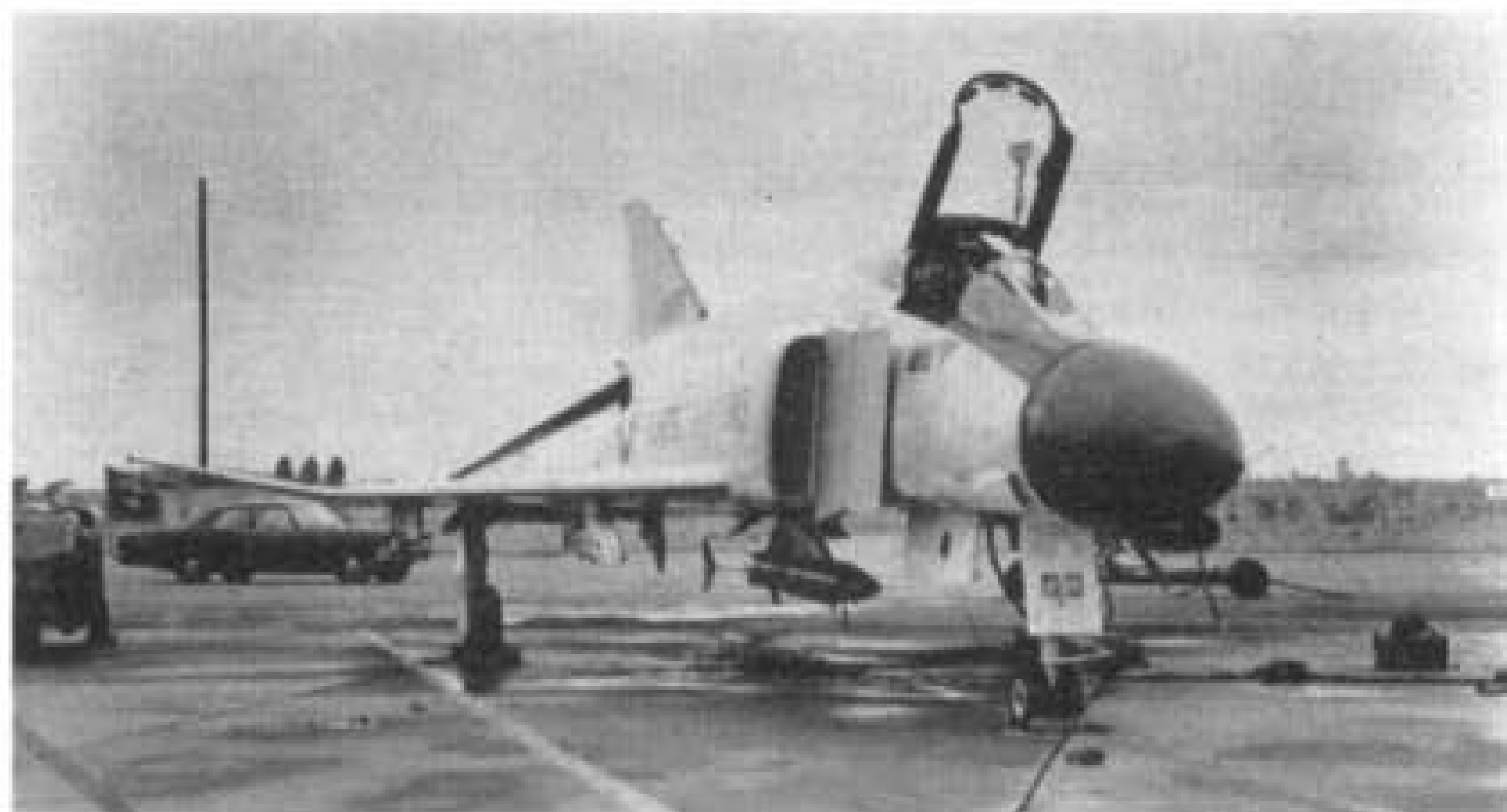
Among the features prominent in this view of U.S.A.F. F-4C (BuA No. 40875) is a Beechcraft "Sandpiper" rocket-powered vehicle, attached to the centre-line stores point. Also clearly visible are the two starboard wing hardpoints, duplicated on the port side. (Photo: via Charles W. Cain)
