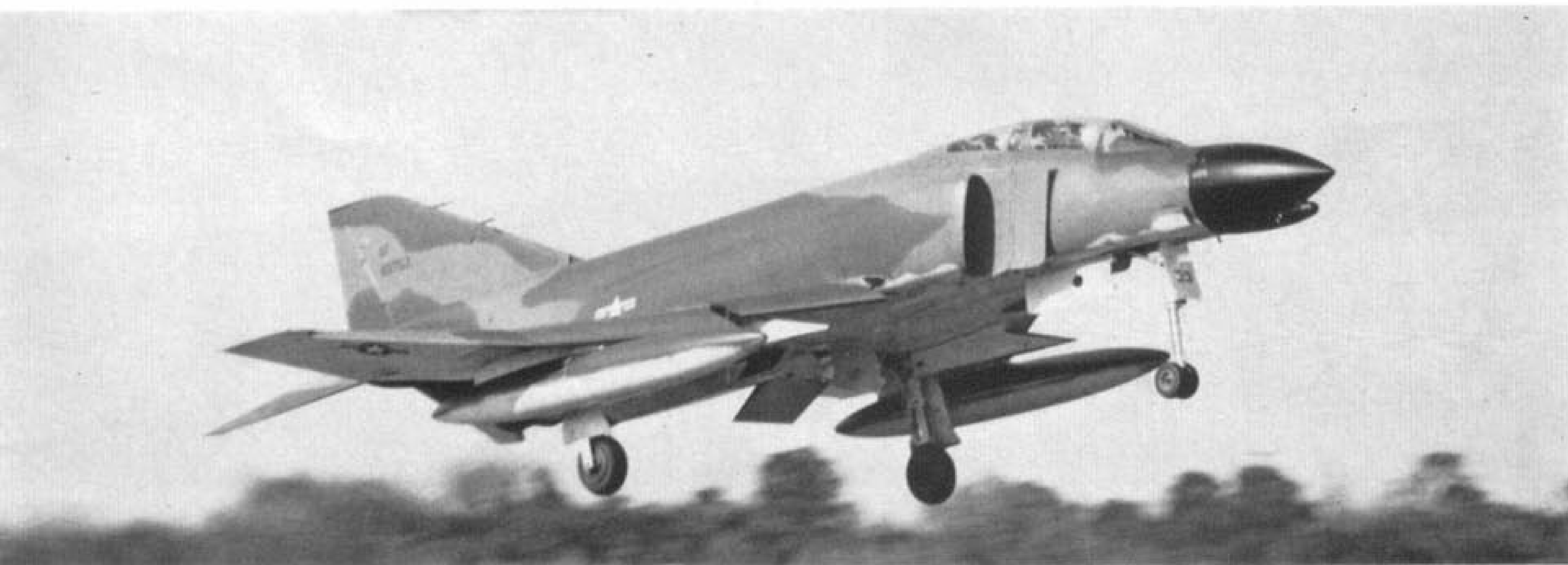
The U.S. Air Force's counterpart to the F-4B, the F-4C Phantom. Seen here with two 370 U.S.-gallon external fuel tanks is U.S.A.F. 40757. (Photo: McDonnell Douglas)
