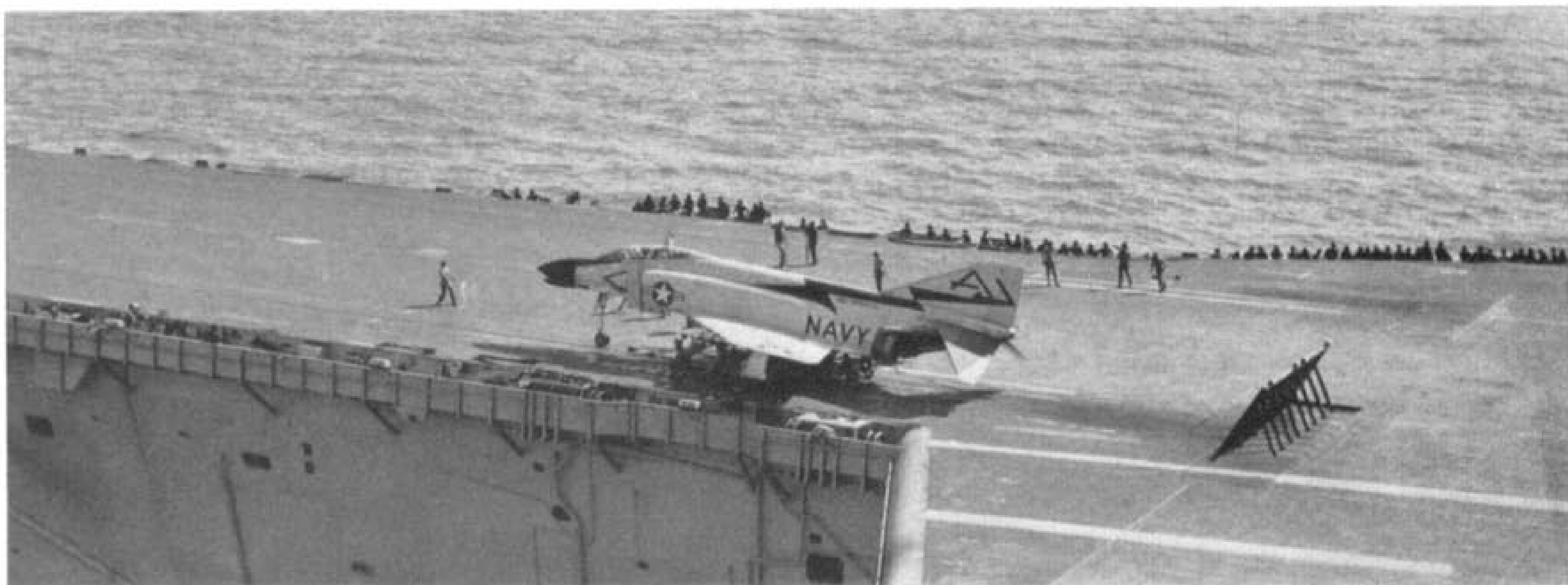
An F-4B Phantom shown aboard the carrier U.S.S. Forrestal and belonging to the U.S. Navy's VF-74 squadron. Just discernable is the aircraft's nose-up angle, effected by the extendible nose undercarriage and very necessary to achieve the correct angle of attack for take-off. (Photo: McDonnell Douglas)
