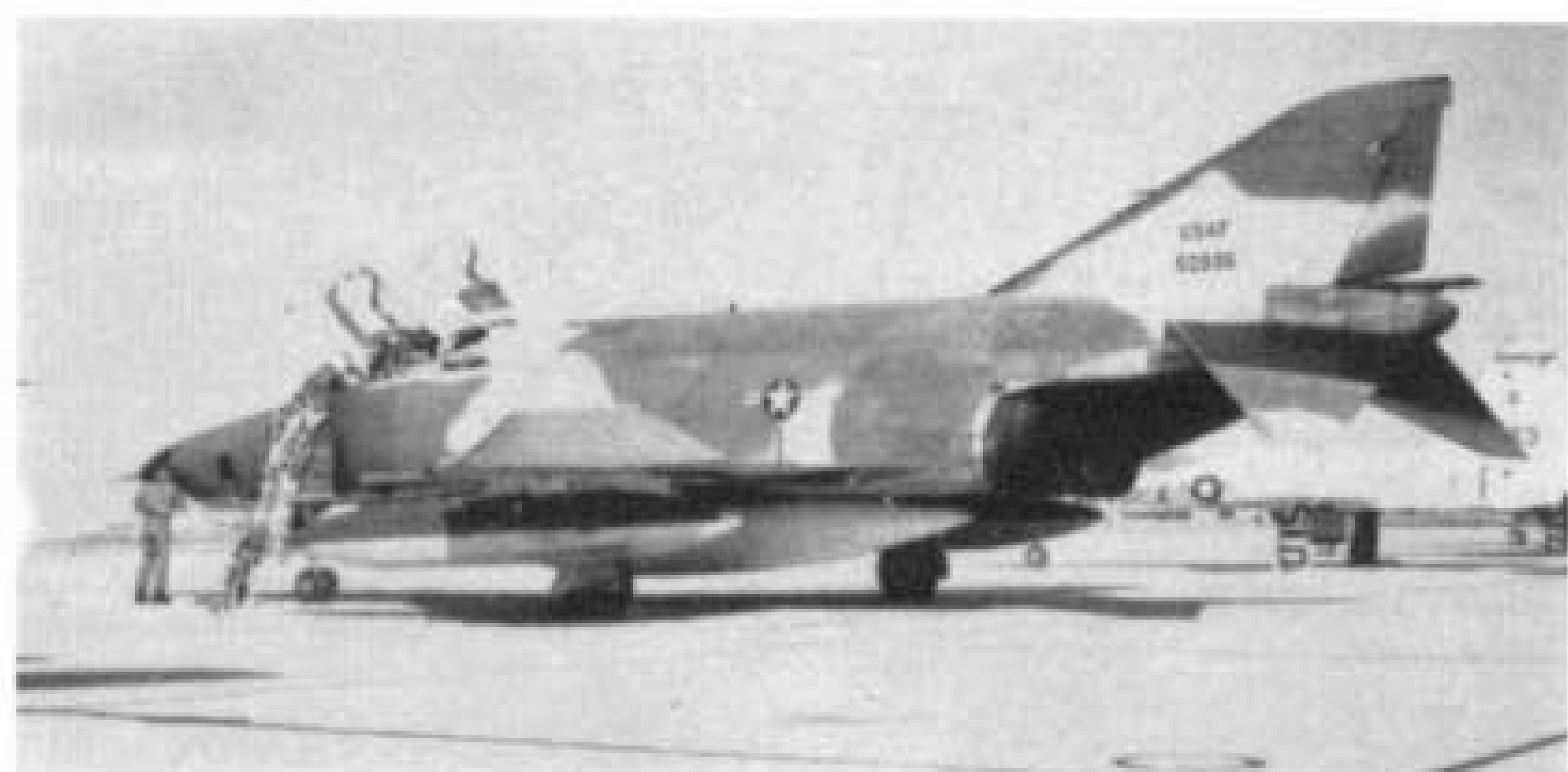
Here seen in U.S.A.F. camouflage markings at the Andrews Air Force Base on October 28, 1967, is another RF-4C (U.S.A.F. 50936). This aircraft has a full complement (two 370 U.S.-gallon plus one 600 U.S.-gallon) of external fuel tanks for maximum area of coverage. (Photo: Dr. J. G. Handelman)
