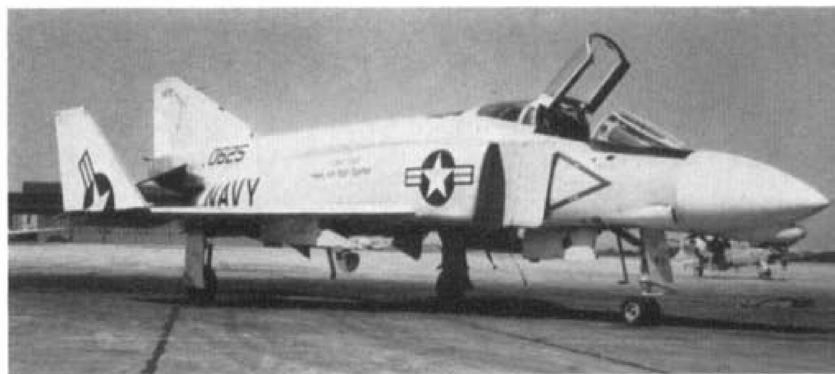
Pictured at the U.S. Navy's Patuxent River, Maryland, Naval Air Test Center is this F-4B, 150625, on August 11, 1965. The prominent variable-geometry engine air intake and folding wing-tips are well displayed in this view, as is the "hardpoint" for fuel tank attachment beneath the starboard wing. (Photo: Dr. J. G. Handelman)
