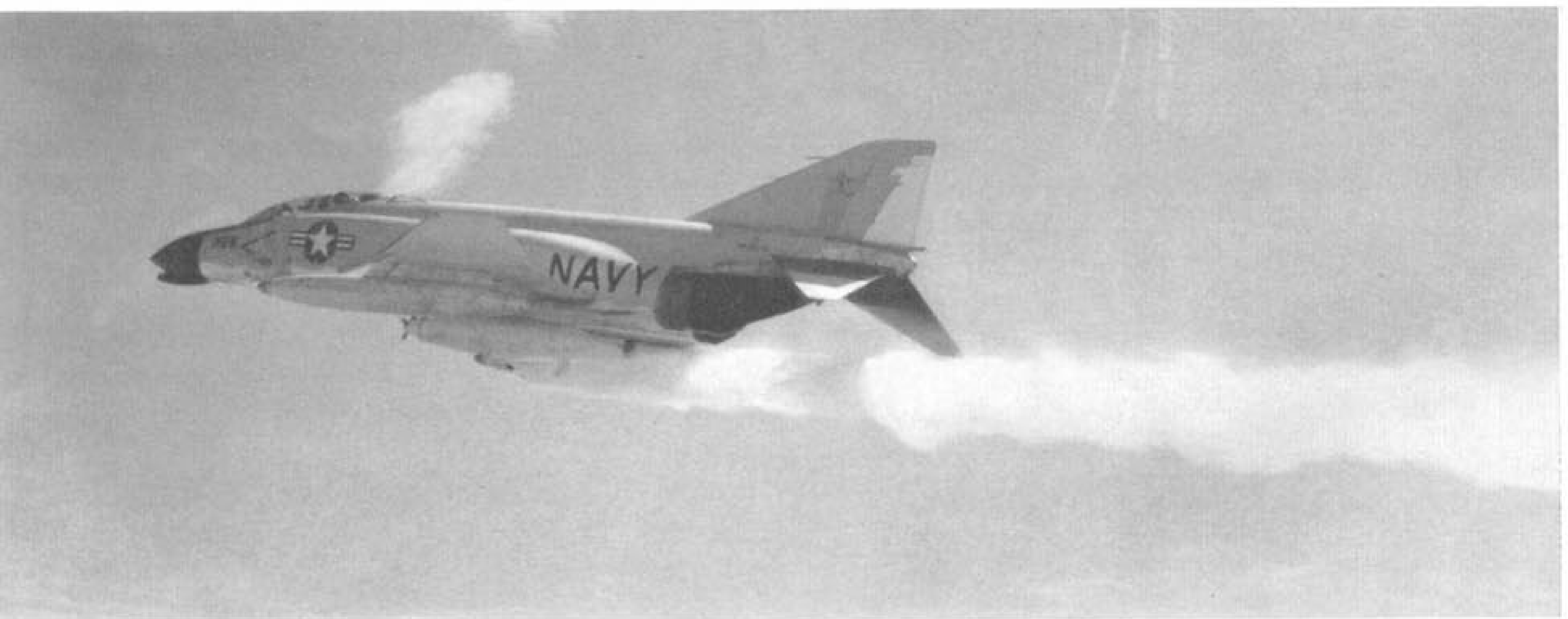
Jettisoning fuel is this U.S. Navy F-4G 150625, seen on August 31, 1964. Externally this version is almost identical to the F-4B. (Photo: U.S. Navy)
