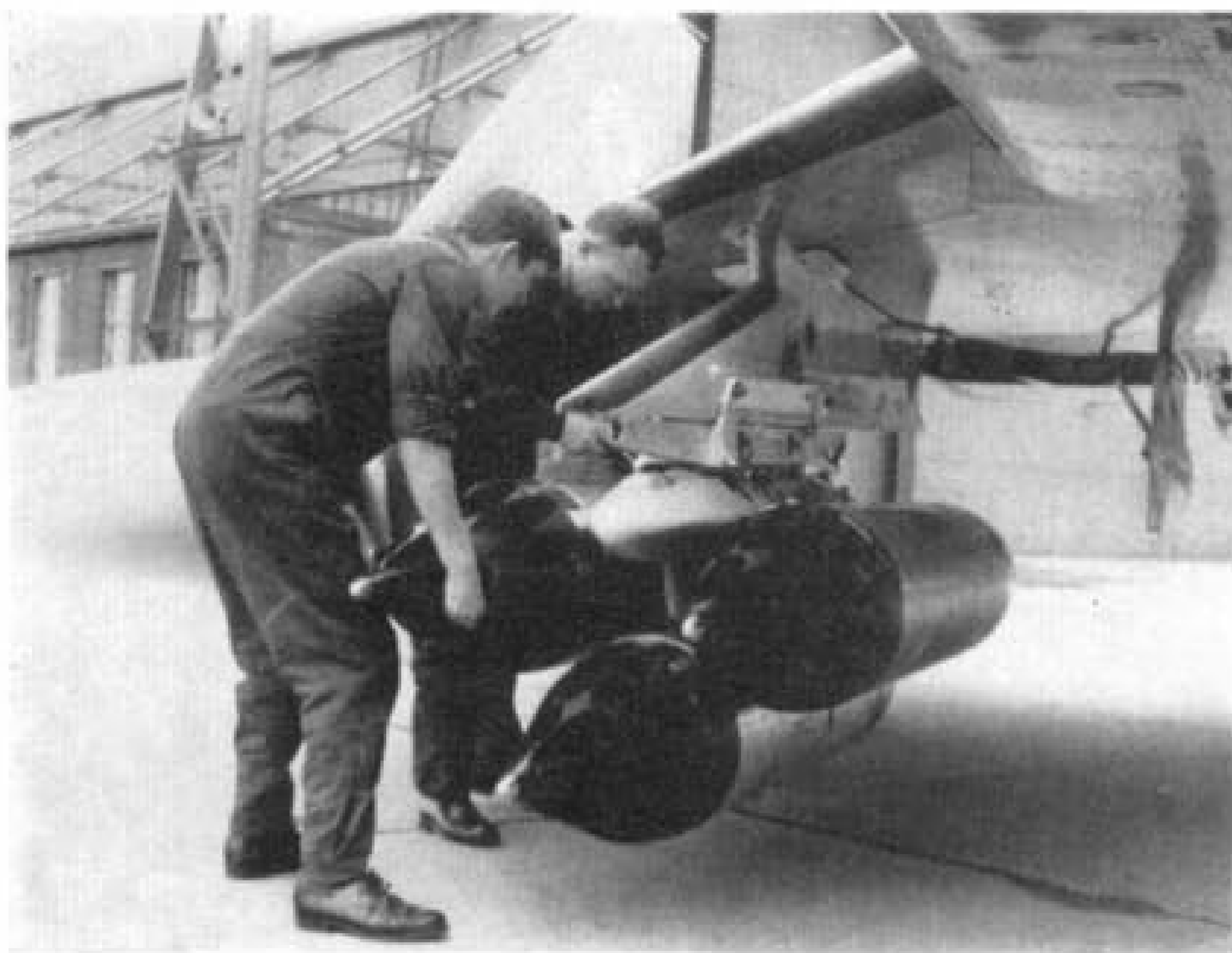
An example of the equipment which may be carried on one hardpoint, in this case belonging to a R.A.F. F-4M Phantom, at Coningsby. Being fixed in place are three Matra 155 rocket launchers. (Photo: Ministry of Defence)
