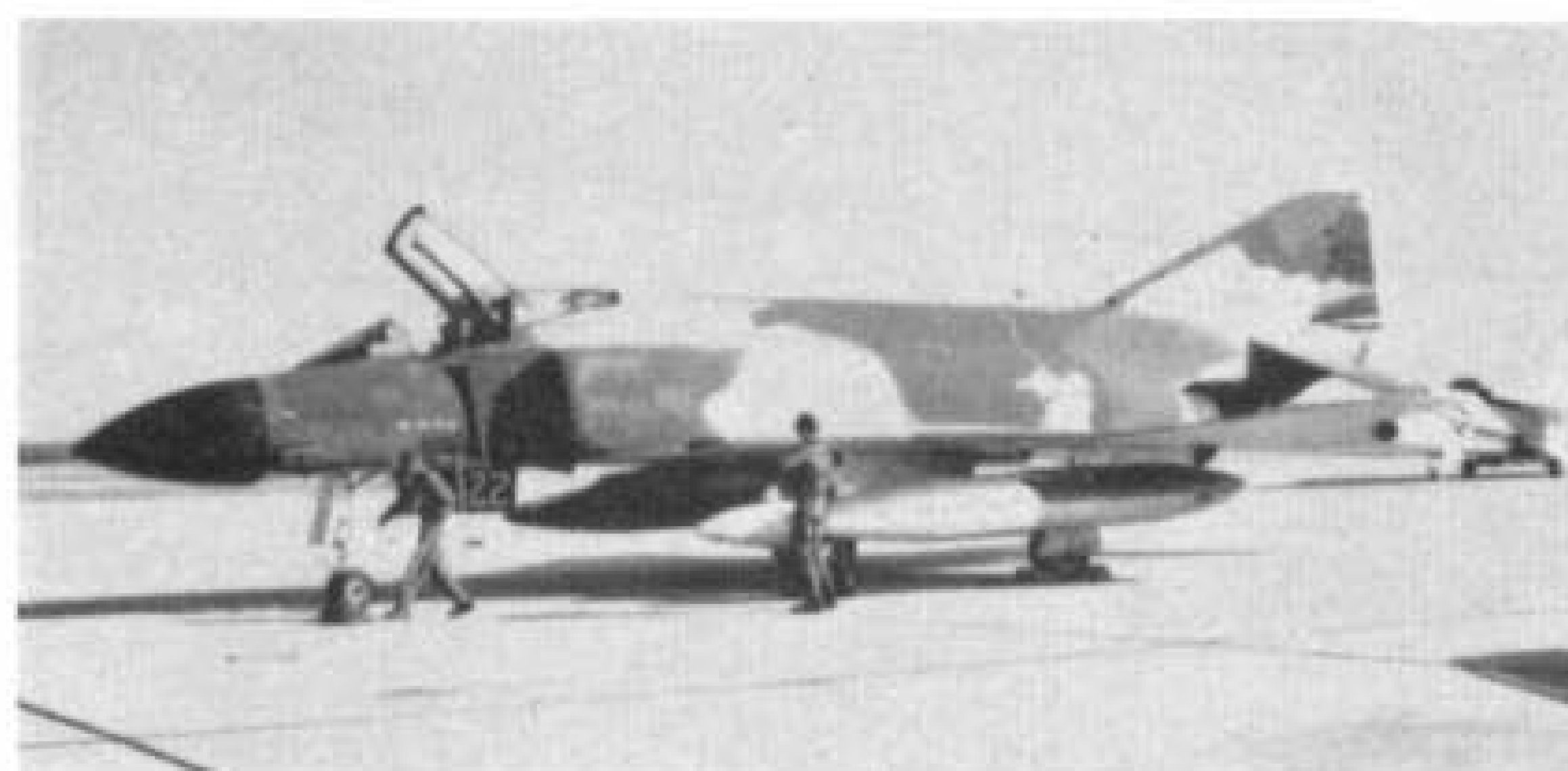
Also at Andrews Air Force Base in October 1967 and bearing three-tone camouflage on side and upper surfaces was this U.S.A.F. F-4D 50622. Successor to, though not replacement of, F-4C, this version differs in appearance through the deletion of the under-nose infra-red heat sensor equipment. (Photo: Dr. J. G. Handelman)
