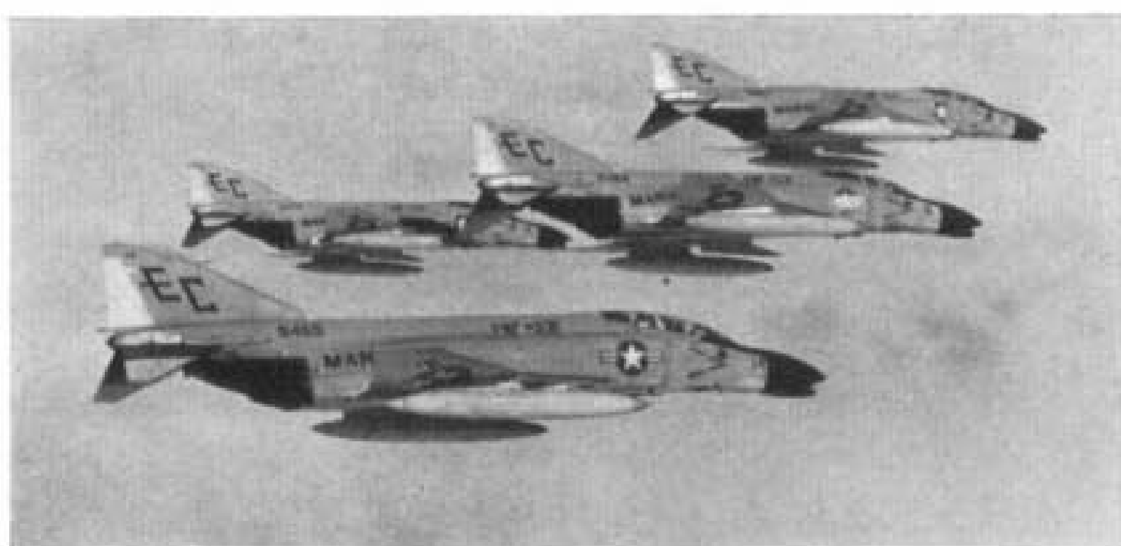
A formation of four F-4B Phantoms from VMF-531 U.S. Marine Corps squadron, each carrying two 370 U.S.-gallon external fuel tanks attached to the undersides of their wings and sporting the standard U.S.N. gull-grey fuselage livery. (Photo: McDonnell Douglas)
