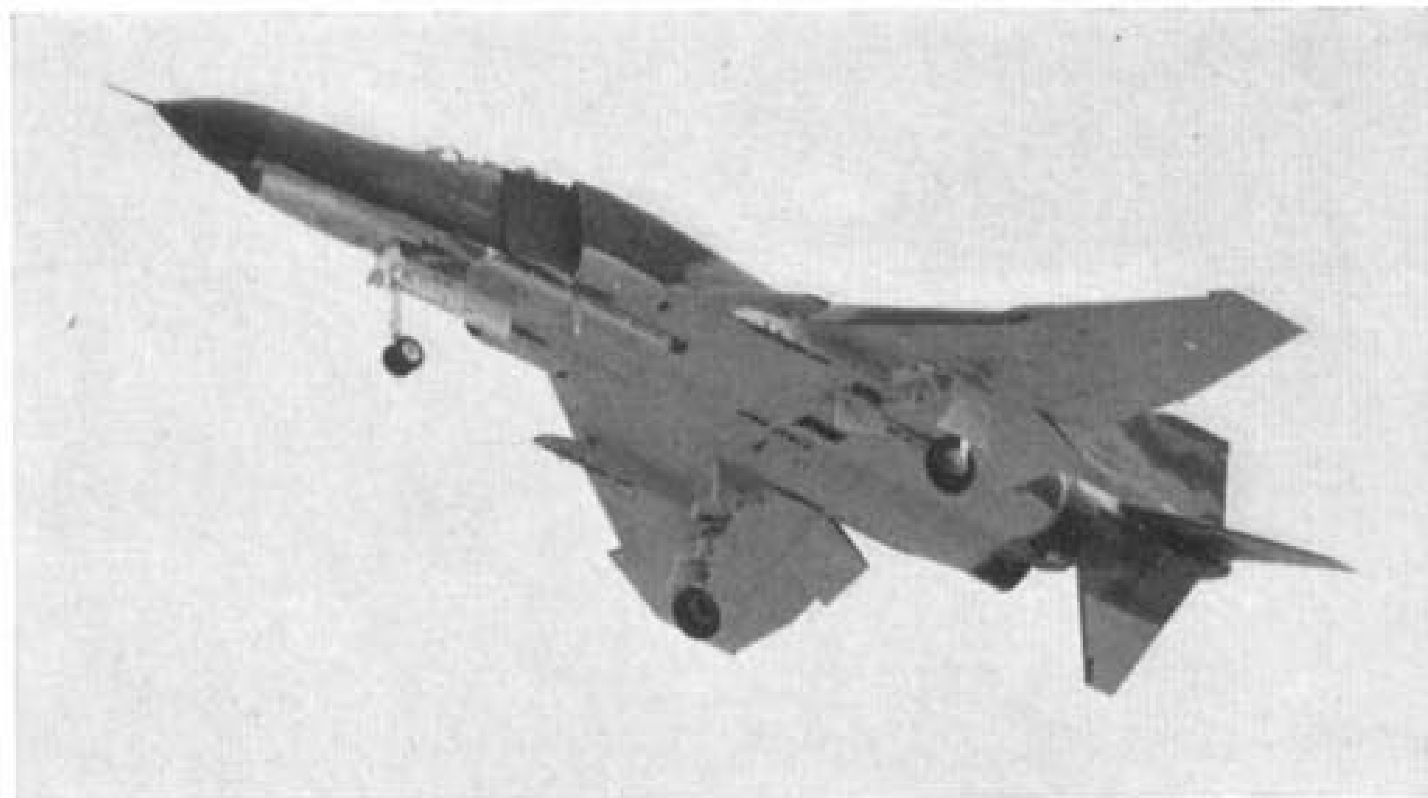
The still more formidable F-4E Phantom, with its integral Vulcan M-61A1 20 mm. Centre-line cannon system, and improved fire-control radar housed in a slimmer radome. Also shown to advantage are the undercarriage units and their stowage bays. (Photo: McDonnell Douglas)
