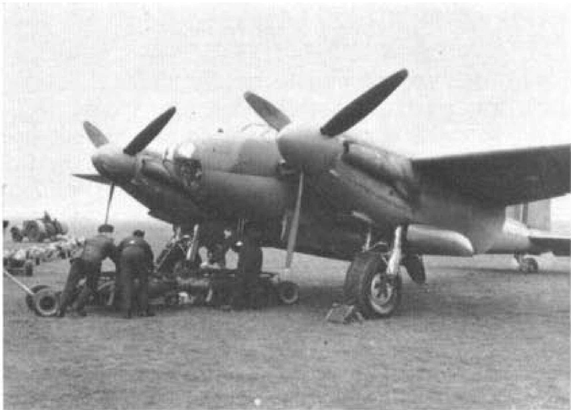
Four 500 lb. bombs with short tails go aboard GB-J DZ367. (Photo: Flight)
