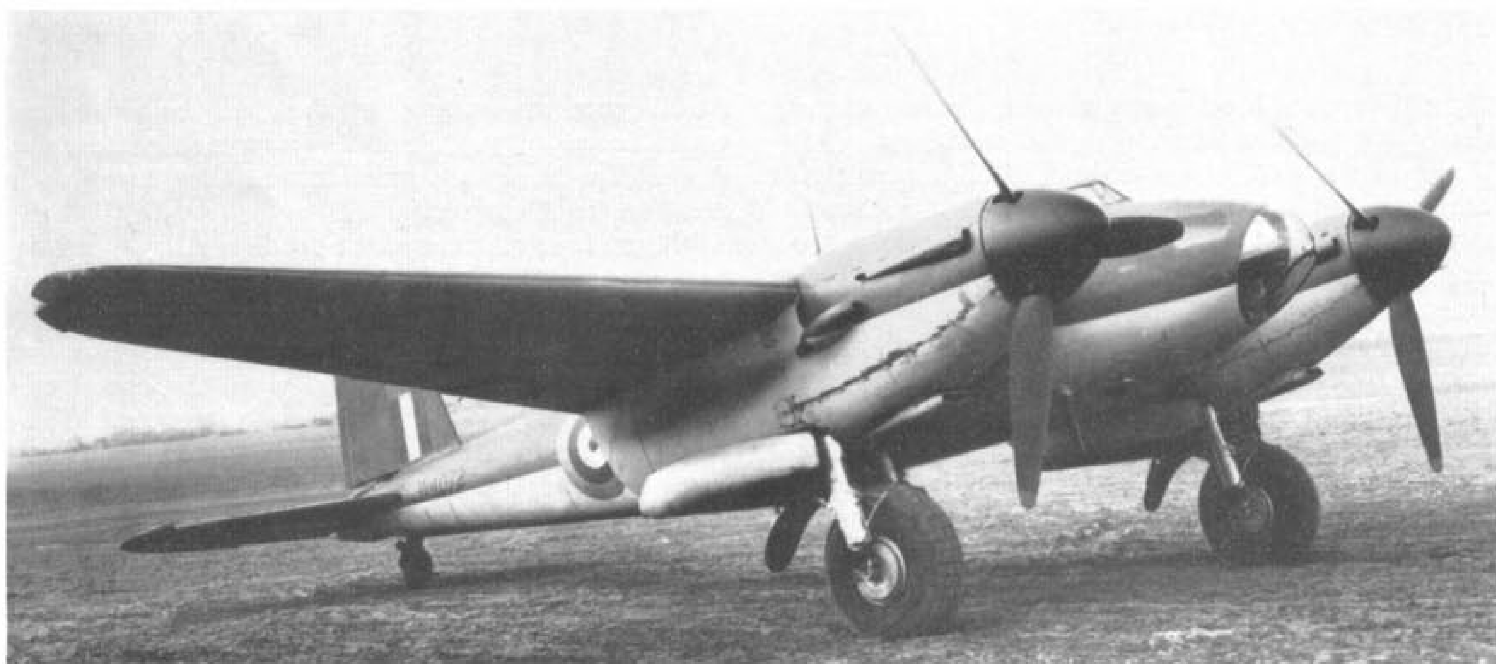
The last of nine B. Mk. IV Srs. i Mosquitos (W4072) shows differences over the first prototype in the detail of the nacelles. Originally, this batch was known as PR/Bomber Conversion aircraft and this Srs. i served with No. 105 Squadron (code: GB-D) in 1942. Later that year it was transferred to No. 1655 Mosquito Training Unit and in 1943 joined No. 627 Squadron (code: AZ-Q). Returning from a raid on Frankfurt on January 9, 1944, Q for Queenie crashed off Bradwell-on-Sea (Essex). The official photographs record the date as being March 1942 and the powerplant as Merlin XXIs. At this period W4072 was being used to evaluate a new type of cavity windshield following normal snag tests. The colour scheme is dark green and dark earth with sky undersurfaces.
