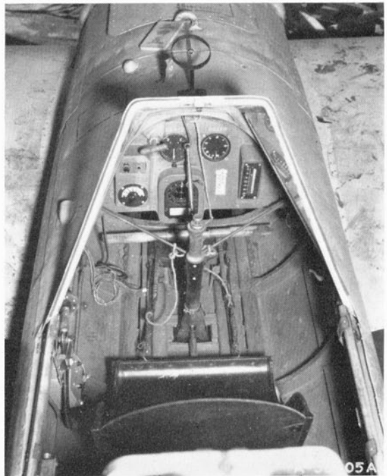
Recalling the simplicity of instrumentation of a World War I scout is this interior of a Model 11. Note the external "ring and bead" sight and the centreline hoisting ring forward of the ringsight. (Photo: U.S.A.F. archives)
