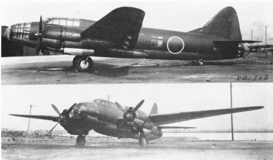
Factory-fresh G4M2a or Model 24. Complete and ready for test flight—except for the spinners—this Navy Type 1 Attack Bomber Model 24 has its distinctive bulged bomb-bay clearly visible in this view. The illusion of a dorsal fin attachment is created by the sloped roof of an assembly hangar in the background. The flap guides are shown to advantage; also the rounded wing tip.
