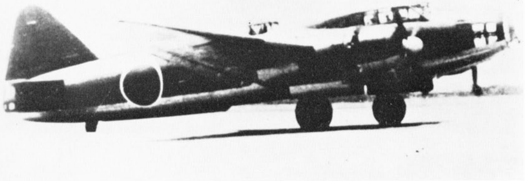
Model 22. One of the 64 Navy Type 1 Attack Bomber Model 22s completed without the bulged bomb-bay doors. (Photo: Real Photographs, No. 3913)
