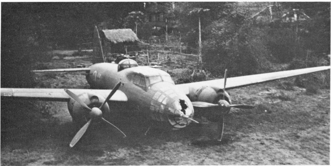
The same Model 24 of the 763rd Kokutai. Damage to the nose above the search radar antenna is visible. (Photo: U.S. National Archives—Navy Dept.)
