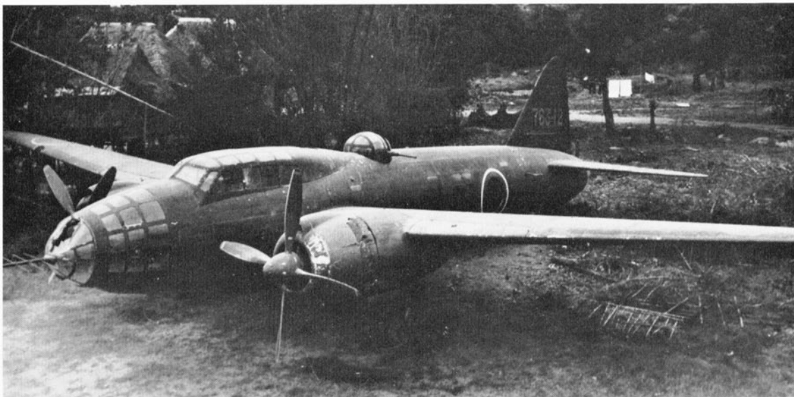
Another view of the Model 24 of the 763rd Kokutai in the Philippines. Presumably it was sufficiently badly damaged to preclude repair before the retreating Japanese forces abandoned the air base. The upper turret mounts a 20-mm. Type 99 Model 1 cannon.
