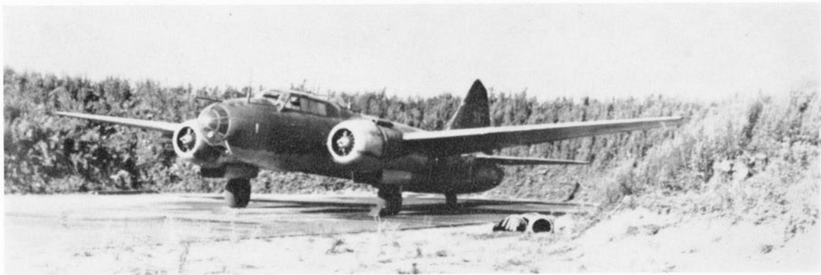
Model 21. A Navy Type 1 Attack Bomber Model 21 with search radar antennae above the nose transparencies and to the rear of the fuselage. This is a post-surrender (August 1945) picture as indicated by the absence of propellers. (Photo: via René J. Francillon)
