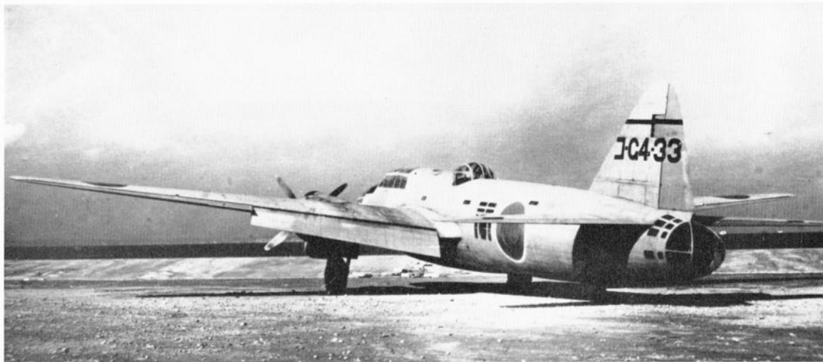
Model 26 in development. Possibly one of the two G4M2c Model 26s—fitted with turbo-supercharged Kasei 25b Ru motors—used as development prototypes for the G4M3 series. (Photo: via René J. Francillon)
