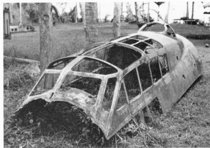
Cockpit and upper amidships gunner's position of the Model 11 was a one-piece fabrication as this photograph—taken in the Philippines as recently as 1965—shows to advantage. (Photo: via René J. Francillon)
