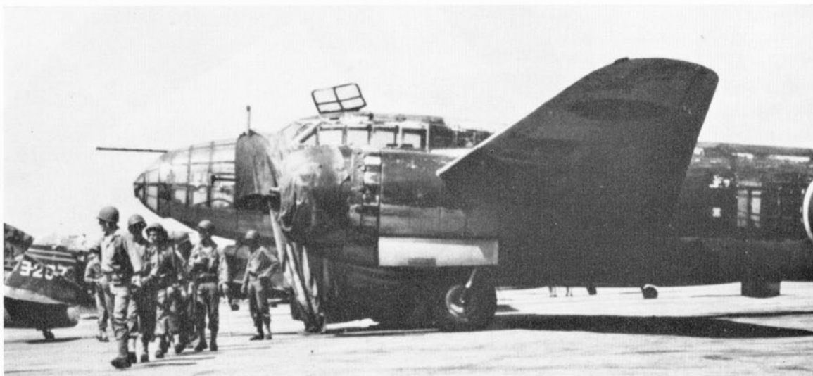
Model 34. After surrender and with propellers removed, a G4M3 Model 34 found at Atsugi in September 1945 by U.S. occupying forces. The kinked nose cone is evident. (Photo: U.S. Navy archives)
