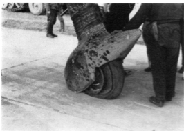
All variants of the Dora suffered from frequent tyre failures, a punctured cover often resulting in a buckled wheel. As the war progressed, the Germans were forced to utilize low-grade materials in their aircraft production programmes. This particular incident shows the effect of overstressing a Ju 87 D-5 main wheel of sheet metal construction. (Photo: Bundesarchiv, ref. 501-133-27)
