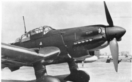
Probably taken during 1942 at the Weser Flugzeugbau factory airfield at Bremen-Lemwerder, this Ju 87 D-1 carries a 66-gallon drop-tank on the outer-wing port bomb-slip. (Photo: Messerschmitt-Bölkow-Blohm GmbH, Archiv ref. 87/42)
