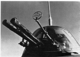
Close-up of the B-Stand or rear-gunner's turret in the Ju 87 D-5. The coupled Mauer MG 81 machine-gun (MG 81 Z) were fitted in a Gleitschienenlafette GSK-K 81 Z flexible mounting giving a 70° traverse to port and starboard, up to 80° upwards and 10°-15° downwards. The long projection on the left of the twin 7.92-mm. gun barrels is the VE 42 gun-right (a development of the VE 22 used in the Ju 87 D-1) and to the right of the MG 81 Z is an instrument to measure deflection. The extensive armour protection for the gunner can be seen under the Plexiglass. (Photo: Bundesarchiv, ref. 446-1935-18)
