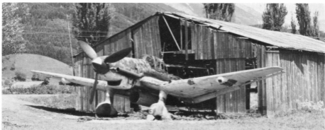
Photographed at an airfield west of Innsbruck, Austria, during June 1945, this Ju 87 D-7 (a refurbished D-3 with Juno 211 P motor) is easily identified by the large flame-dampers exhausting over the wing roots. Used by the Nachtschlachtflieger in substantial numbers, these machines operated against the Allies until the last days of the war. Neither the designation nor the purpose of the cylindrical store carried by this particular aircraft have yet been discovered. (Photo: U.S. Air Force, ref. 57926 AC)
