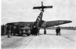
A classic case of the dreaded Kopfstand! In this instance, the crew walked away unscathed and the only damage was a shattered aircrew. The aircraft is a D-3, and the "diving penguin" insignia on the rear of the scout car would indicate that the machine belongs to Stukageschwader 1.
