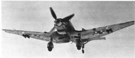
This view of a Ju 87 D-3 taking off on a mission gives an excellent idea of the location and type of offensive load carried. The out-wing bomb carriers on each side could (as in this photograph) accommodate a pair of 110-lb. bombs on individual slips, or a single 550-lb. missile on the inner 500/XIIC carrier. The under-fuselage rack took a 550-lb. or 1,100-lb. shackled to a 500/XIIC slip or a 2,200-lb. or even 3,960-lb. weapon if a special 2000/XIII carrier (replacing the abortive 1000 carrier mentioned in the narrative) was used, though this restricted use of the outer racks.
