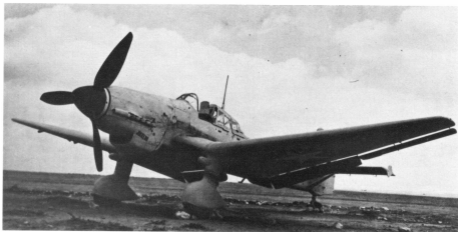
Probably acquired in Tunisia during the spring of 1943, this Ju 87 D-3 troop named Jocelyn is unusual not only in having U.S.A.A.F. markings, but because all excessences including machine-guns, landing-light housings and dive-brakes have been stripped and the wing faired over. (Photo: U.S. Air Force, ref. 26623 AC)
