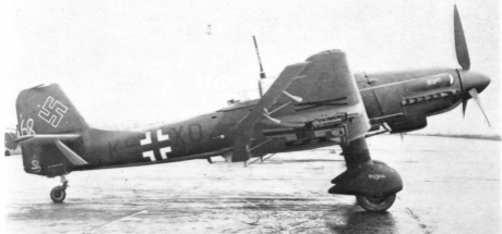
An unarmed early production Ju 87 D-5, probably at Bremen-Lemwerder. The code letters KS+XD on the starboard fuselage are repeated in reverse order under the wings. Reading from left to right—"DX" under the port wing and "SK" under the starboard mainplane. This lettering was retained on operational aircraft, although the fuselage combination was sprayed over and a unit cipher took its place. (Photo: Messerschmitt-Boikow-Blohm Archiv, ref. 87/28)
