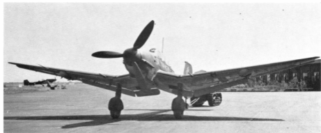
Another Ju 87 D-5 is towed away from the assembly hall by a Kettenfahrzeug—tracked vehicle—to await acceptance testing and delivery to a Luftpark. Once at this Air Park or Maintenance Unit, the Dora would be stored until required by a particular Staffel to replace an aircraft lost in combat or otherwise written off. Before being ferried to the unit, the Luftpark would ensure that all recent detail modifications were incorporated. (Photo: via Egon Krüger)
