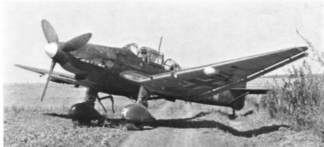
A completely standard Ju 87 D-5. The harness hanging under the forward fuselage was the securing strap of the bomb-crutch, designed to swing the weapon clear of the airscrew during a dive. (Photo: Bundesarchiv, ref. 581-2067-14)
