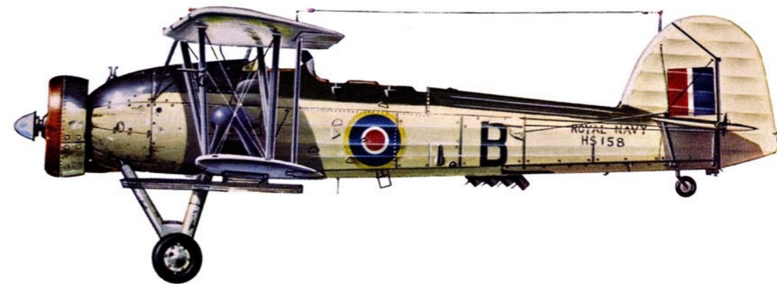
Swordfish II, HS158 of No. 816 Sqdn, 1943; note flare chutes fitted.
