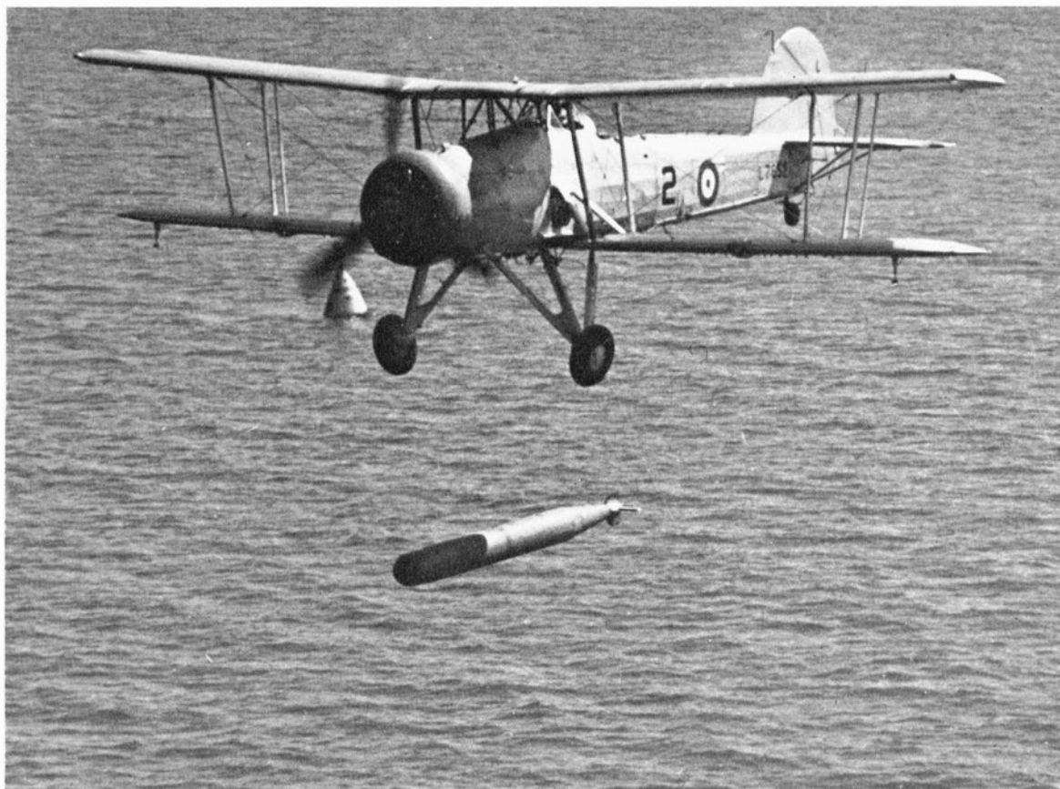
L7652 "2", a Swordfish I of the T.T.U. Gosport, releases its 1,610-lb torpedo.
