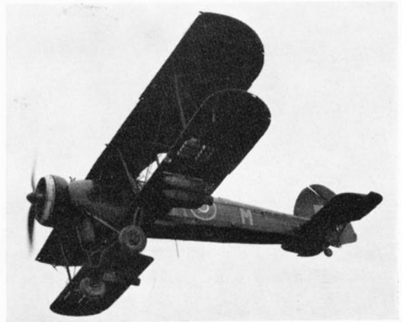
A Swordfish III NF374 "NH-M" of No. 119 Squadron, with a full load of bombs and flares on its wing racks, on anti-shipping patrol near the Dutch coast.
