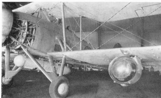
A Swordfish fitted experimentally with a Leigh Light under the port lower mainplane, for night operations. The object between the undercarriage struts is the battery.
