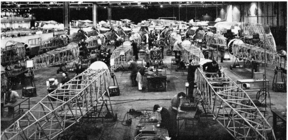
Fuselage frames under construction at the Sherburn factory in May 1944.
