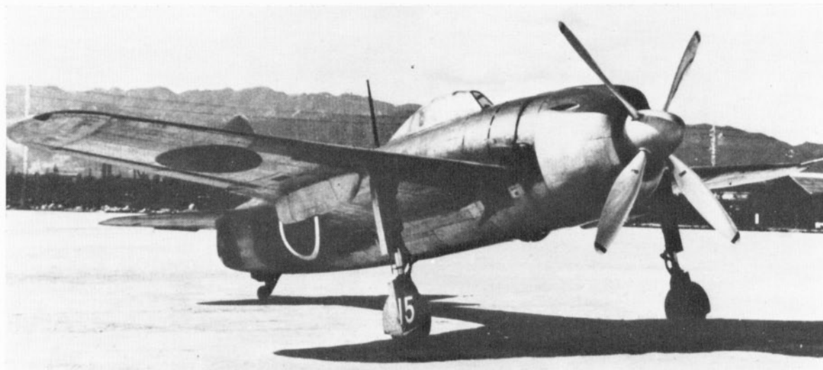
A Kawanishi Model X-1 Experimental Land-based Fighter tested by the Imperial Japanese Navy. Note absence of air scoop on the lower engine cowling lip, a feature which identified the early Model X-1 prototypes.
