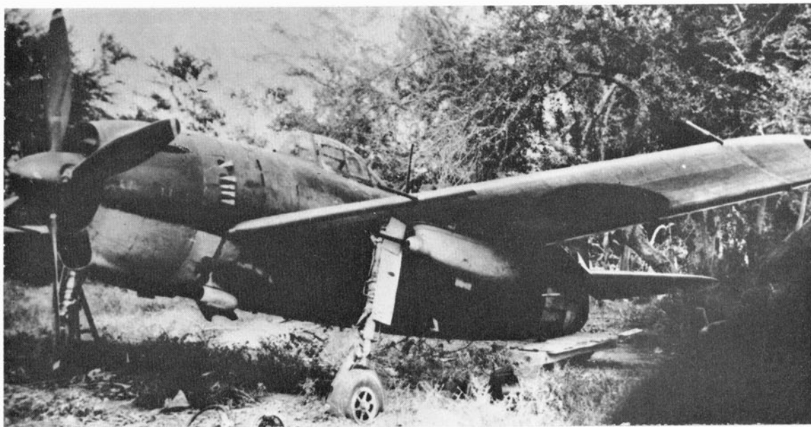
Navy Interceptor Fighter Shiden Model 11 (NIK1-J) of the 201st Kokutai in the Philippines. This particular aircraft bore the tail number 201-53 on its vertical surfaces. Note details of the armament installation.
