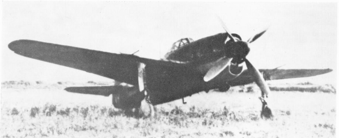
A Kawanishi N1K1-J Shiden Model 11 with underwing gondolas removed. Note external oil cooler protruding beneath the port side of the engine cowling.
