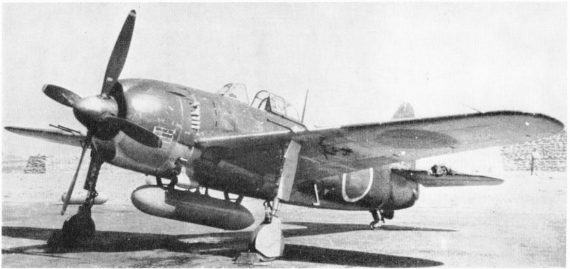
Navy Interceptor Fighter Shiden Model 11A (N1K1-Ja) characterized by the location into the wings of all four 20 mm. cannons. The aircraft is seen fitted with a 400-litre (88 Imp. gal.) drop tank.
