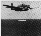
During operations in American waters a Grumman TBF-1 (note mark-10 gun installation in front of cockpit) is photographed moments after releasing its 24-in. torpedo. (Photo: U.S. Navy)
