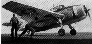
A TBF-1C (note push over wing-mounted eng. which differentiated this version from the earlier TBF-1) about to be launched from the deck of the U.S.S. Franklin (CV-113) in March 1944. (Photos: National Archives)
