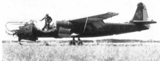
Werk Nummer 140349, an Ar 234 B, probably caught by ground-strafting Allied fighters and burnt-out at Rheine airfield. All salvageable items, including the jet engines and aircraft's tyres were removed by the Germans and the empty shell was used as a decoy.
