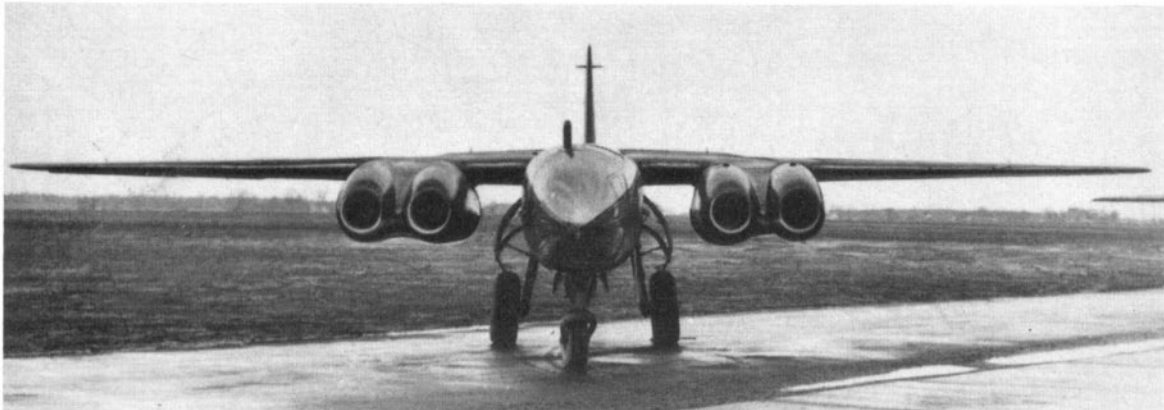
An early prototype Cäsar or "C"-series. Probably in the V-Muster range V 19 to 22, this was the only Luftwaffe four-jet aircraft in production at the cessation of hostilities. (Photo: via Hans J. Ebert)
