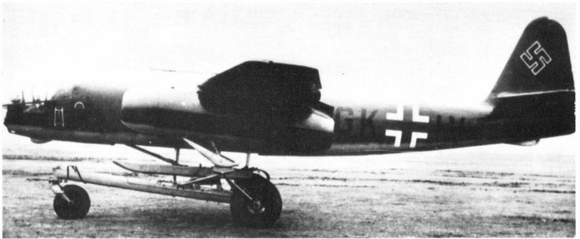
Vying with the Gloster Meteor F.Mk.I and the Messerschmitt Me 262 A for the title of the world's first operational jet aircraft, the Ar 234 V 5 (coded GK+IV), seen here on its jettisonable take-off trolley, was one of a pair of "A"-series prototypes converted for use as reconnaissance aircraft and flown by pilots of the Versuchsverband des Oberkommandos der Luftwaffe over the Allied beachheads in Northern France from late July 1944 onwards. (Photo: via The Royal Aeronautical Society)
