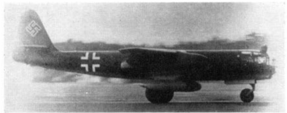
On May 12, 1944, Flugkapitän Eheim flew the Ar 234 V 9 experimentally fitted with under-motor 66-gallon drop-tanks. These tests proved successful and such containers were extensively used by long-range reconnaissance units equipped with the Blitz.
