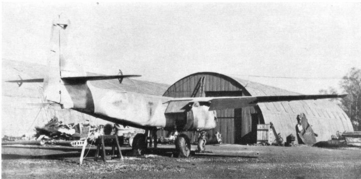
The Segelsdorf Ar 234 B-2, W.Nr. 140173 (F1+ MT) of 9./K.G.76 following re-erection at the Royal Aircraft Establishment. Photographed on March 21, 1945, the aircraft is complete except for a missing escape hatch (jettisoned during the belly landing) and shattered front fuselage glazing. The Jumo 004 Bs have been removed for detailed scrutiny. It was not flown again. (Photo: via Blitz Publications)
