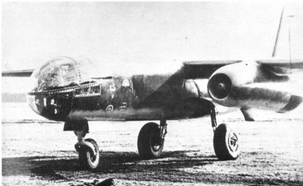
The Ar 234 V 9 is seen here with an experimental bomb/drop-tank carrier under each engine nacelle. During April-May 1944, Flugkapitäne Eheim and Kröger flew a series of trials with this aircraft testing various combinations and calibres of bombs.
