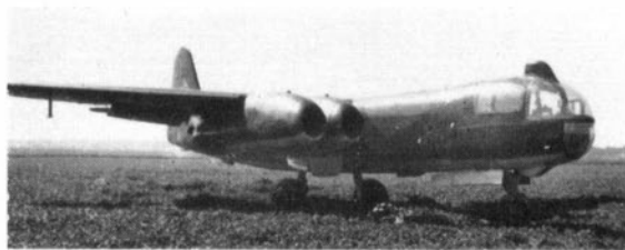
Captured at München-Riem (now Munich International Airport) at the end of April 1945 by American troops, this pre-production Ar 234 C-03 carries the work's number "006". As far as is known, this Cäsar was the only flyable four-jet aircraft to fall into the hands of the Western Allies. Apart from the paired jet motors, the revised contour of the nose section, reduced glazing and a more streamlined periscope all characterize this excellent design. Less obvious are the modified ailerons and smoother wing skinning which improved the aerodynamic characteristics of the type. The C-3 was just going into production when the war ended.
