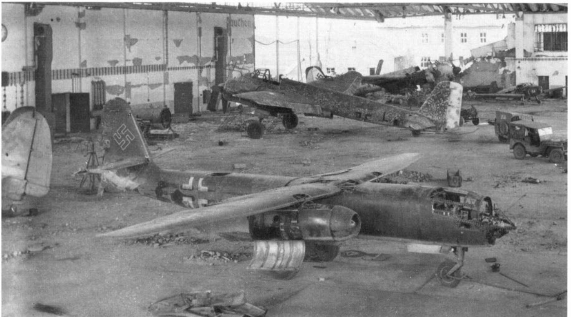
A battered and dusty Ar 234 B-0, W.Nr. 140114 (coded GM+BN), stands in a damaged hangar at Manching airfield. In the background are Ju-88 G night-fighters used in the defence of München (Munich). This Blitz was one of several pre-production Ar 234s flown from the Erprobungsstelle Rechlin. On September 14, 1944, when the aircraft was ferried to Burg near Magdeburg for modification in order to flight test an automatic pilot, the airframe time totalled only 7 hours 11 minutes. (Photo: U.S. Army ref. SC 195630)
