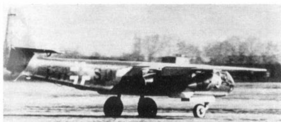
The Ar 234 V 9 taxiing to take-off with a pair of Walter Ri 202 b (109-500) rocket A.T.O. motors slung under the wings outside the Jumo 004s. These rocket engines went out of production before the Blitz was firmly established in service and attention was focused on using more powerful motors (such as the Schmidding SG 34 for the Ar 234 C) in their place.
