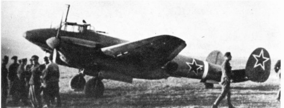
Another subject for a colour side view on page 124, this is a late production, VK-105RF-powered Pe-2 in Autumn 1944 at Tri Duby airfield during the Slovakian national uprising. (Photo: via Zdenek Titz)
