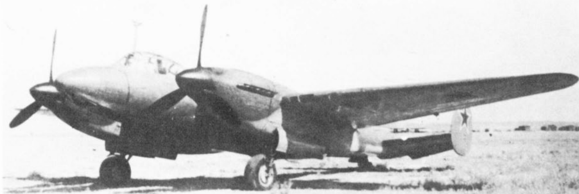
Final development of Pe-2 production, the Pe-2I ("Istrebitel"; "Fighter") powered by VK-107 As in slimmer cowlings and with individual exhaust stubs. (Photo: via Vaclav Nemecek)
