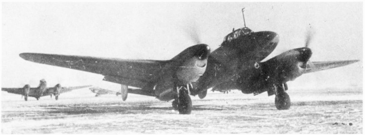
The definitive Pe-2 with VK-105RFs cleaned-up engine cowlings and aerial mast removed to the forward position. The oil cooler intakes are revised, too. (Photo: via Imperial War Museum, ref. RUS4750)
