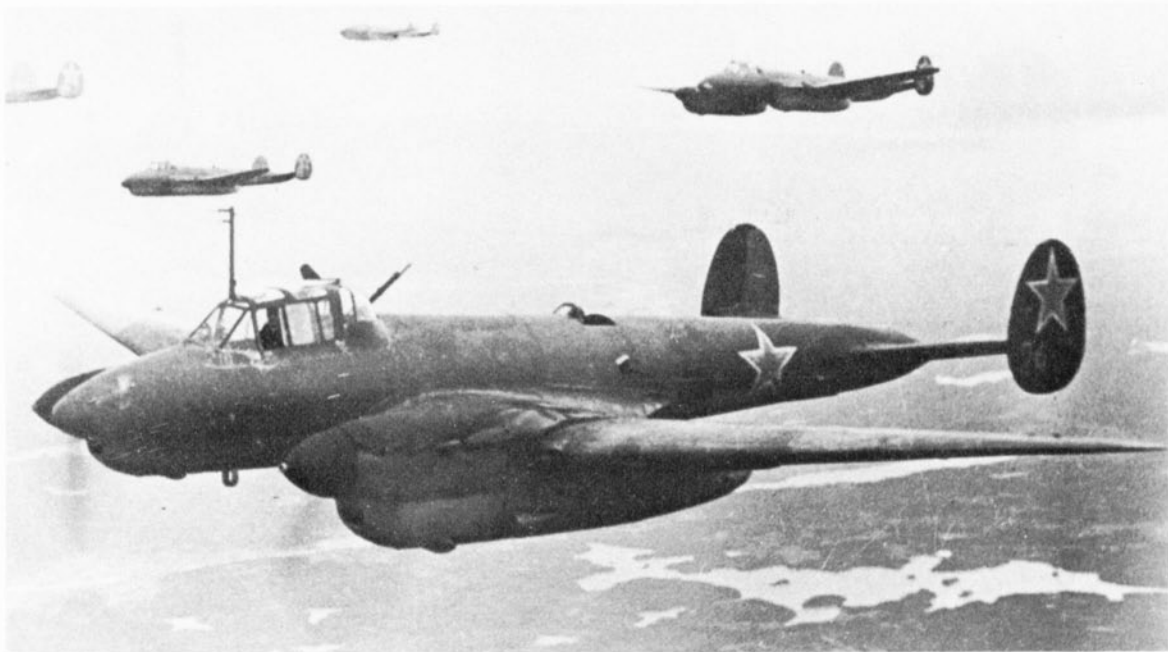
The definitive Pe-2. Period, Autumn 1944. Above the wing root can be seen the open hatch—complete with windshield—and the head of the radio operator/ventral gunner. The porthole gun just below this hatch appears to have been censored. (Photo: via Air-Britain archives)
