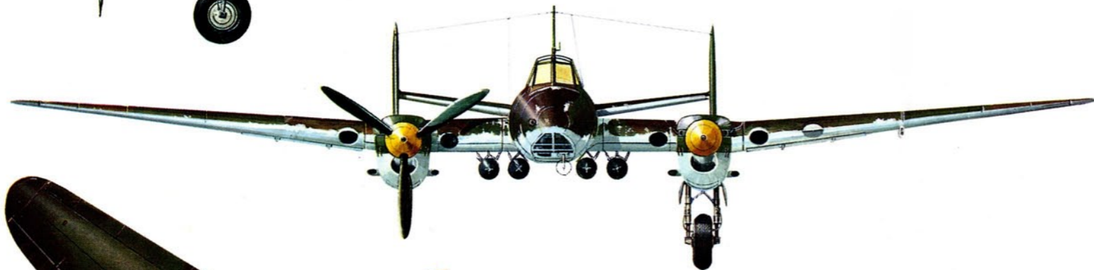
A typical first-line Soviet Bomber Air Regiment "Peshka" (familarly, the chess pawn) in early 1945 colouring; the "Front-line" dive-bomber Pe-2 with two VK-105RF inlines.
