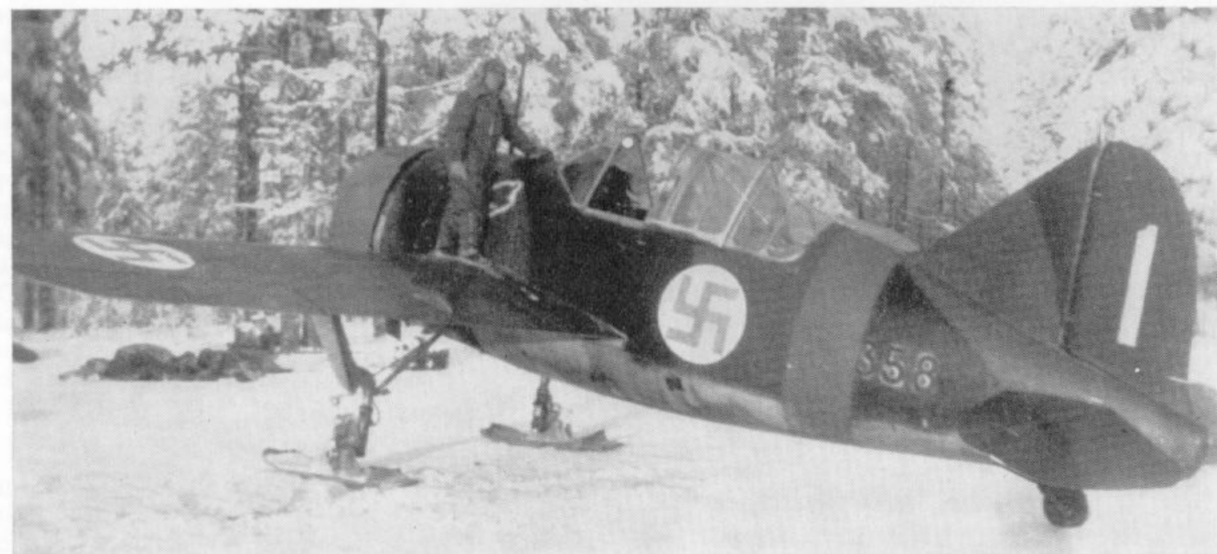
Brewster 239 BW-358, of 2nd Flight/HLeLv 24 fitted with skis for winter operations from Tiiksjärvi airfield, January 1942. (Photo: via Kalevi Keskinen)
