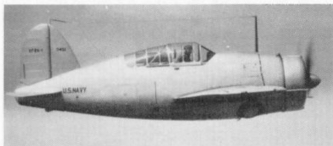
Prototype Brewster XF2A-1 in flight; note original lower-profile cockpit canopy. (via C. Macomber)
