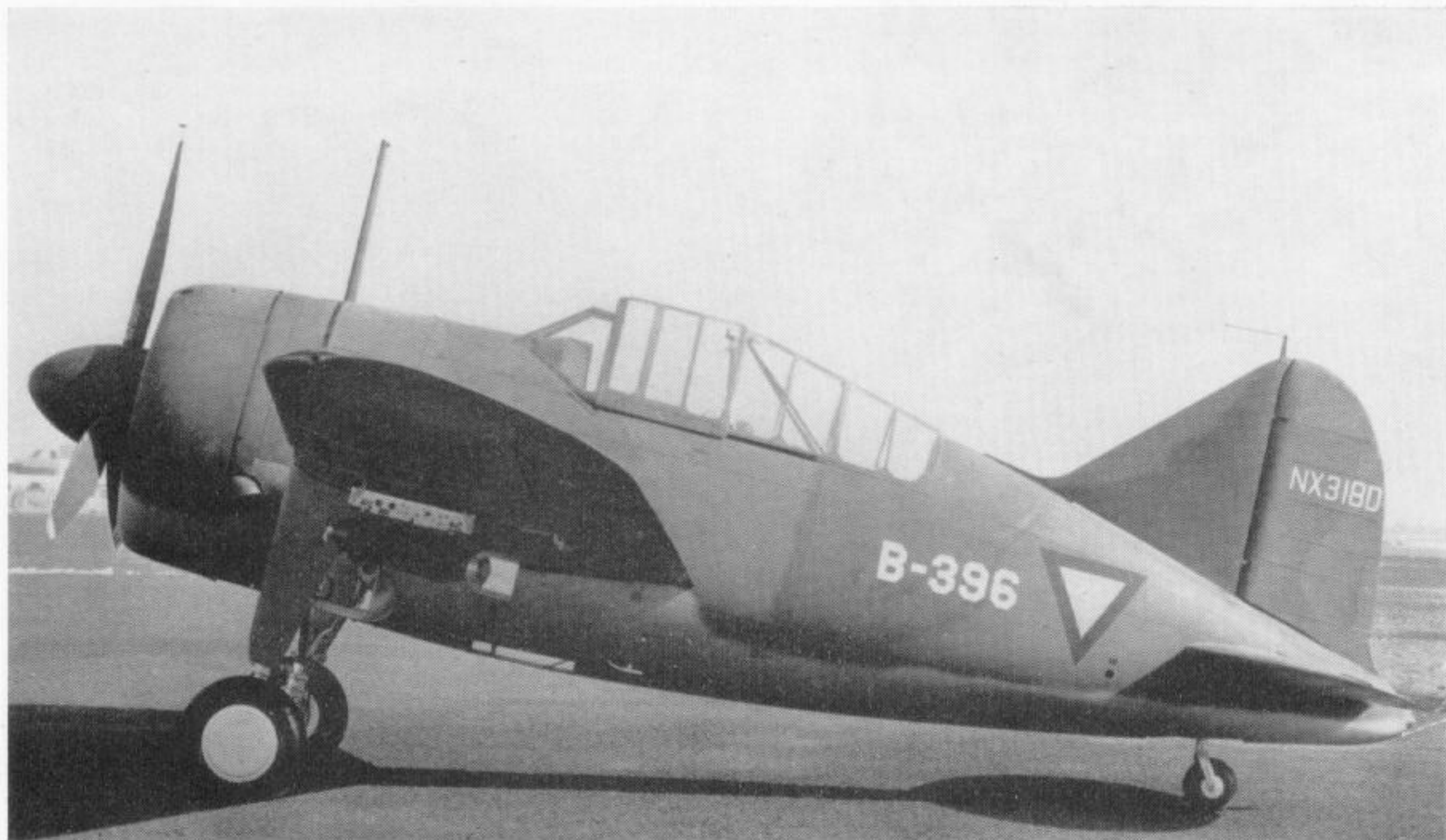
Above: Third air force to take the Brewster fighter into action was that of the Netherlands East Indies. This B-339D, fitted with underwing 50 kg. bombs, is awaiting shipment from the U.S. (Note U.S. serial on rudder.)
