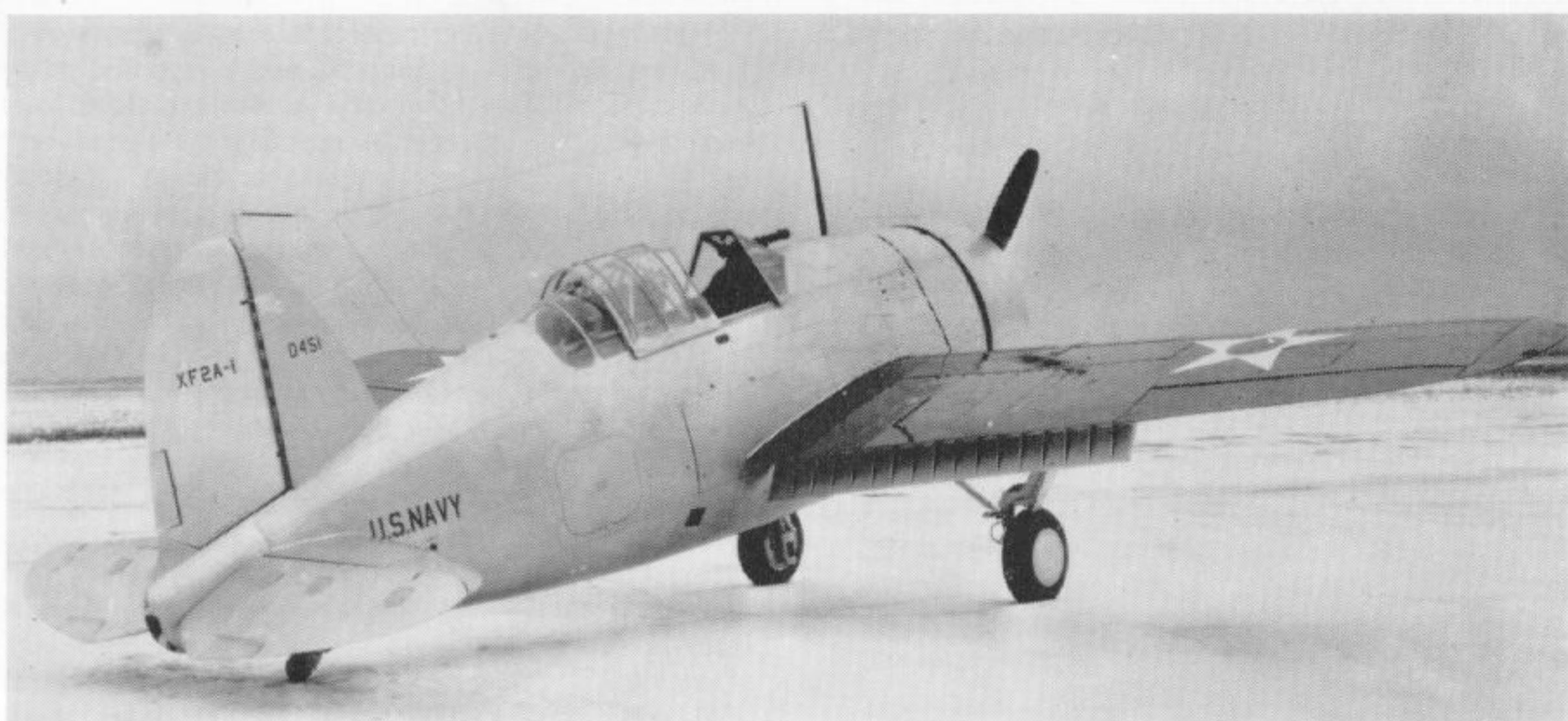
Prototype Brewster XF2A-1 with original low cockpit canopy. Apparent dark paint on wing upper surfaces is chrome yellow as rendered by early type films. (via C. Macomber)
