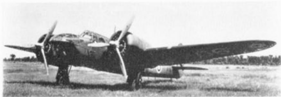
The Canadian prototype Bolingbroke Mk. IV-C (9074) with apparently oversize cowlings housing the single-row Wright Cyclones. It flew for the first time in June 1942. (Photo: Bristol T149/71)
