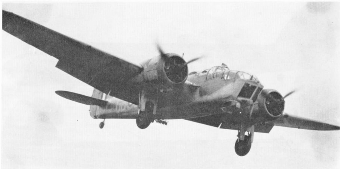
A late-production Blenheim Mk. IV (V6389) of No. 105 Squadron, built by Rootes Securities at Speke. The extra nose armament of a free-mounted Vickers K can be seen, as can the light bomb carrier on the rear fuselage. A small rear-view mirror is above the windshield. (Photo: via the author's collection)
