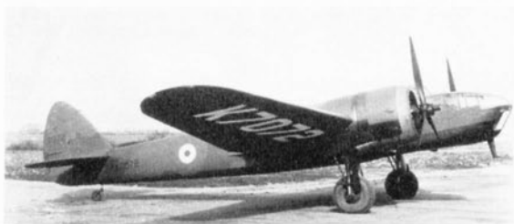
Above: Two views of K7072, the Bolingbroke prototype, at Filton on December 28, 1937, with the revised and symmetrical nose permitting stepped-down pilot's windshield—superficially reminiscent of the Bristol Beaufort torpedo-bomber. The use of Orthochromatic film gives false reading of outer yellow ring to fuselage roundel. (Photos: Bristol T149/17 & /16)
