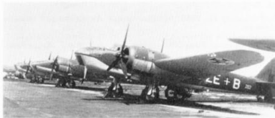
Above and below: Portuguese Air Force Blenheim Mk. IVs sandwich a Mk. V. The markings are more colourful than those of their Navy compatriots and ZE:B has the serial 262 while ZE:G is designated 267. These are late production Blenheims. The Mk. IV below, unlike those above, does not have a desert Vokes air filter under the cowling.
