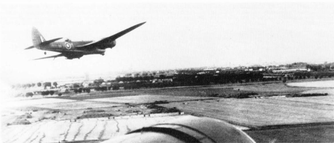
Blenheim Mk. IVs of Nos. 18 (Burma) and 21 Squadrons took part in a low-level anti-shipping strike at Rotterdam on July 16, 1941. Shown here, from a Blenheim dorsal turret is a No. 18 Squadron Mk. IV (coded WV:H) low over the outskirts of the Dutch port. Note the exhaust flare muzzle-type extensions under the engine nacelles.
