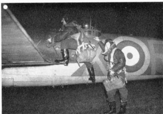
That's how they clambered aboard, using the fuselage foot cavities. This unidentified night fighter squadron's Blenheim is a Mk. IVF—the ventral 4-gun pack is just visible, extreme left. IFF ("Identification—Friend-or-Foe") is fitted as evidenced by aerial wire to position on white circle of roundel. Upper and lower surfaces paint demarcation is unusual. (Photo: Imperial War Museum CH1585)
