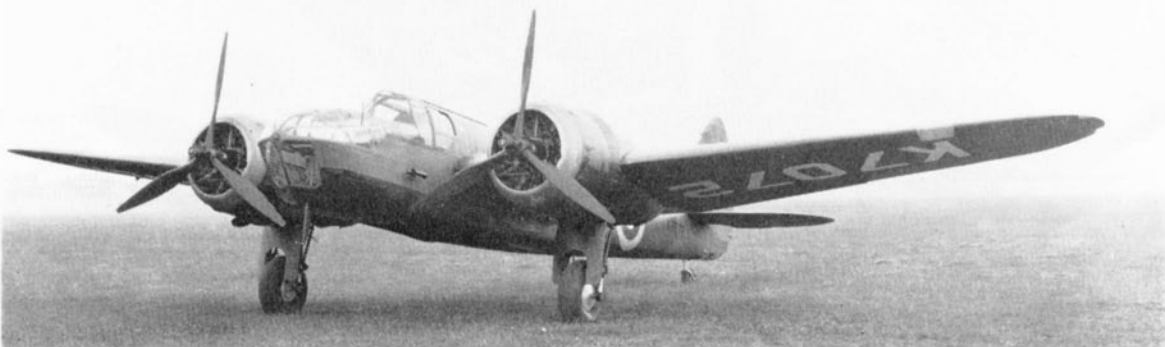
Below: Again at Filton, K7072 is photographed on June 22, 1938 with the definitive asymmetric "long-nose" transparency. At this stage the radio mast was not installed. (Photo: Bristol T149/20)
