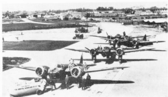
Two of a kind. Left-hand photograph, taken at Filton in April 1939, shows four N-serial Mk. IVs (from Bristol's second production batch). Nearest Blenheim still lacks propellers. Right-hand photograph of nine Mk. IVs was taken in mid-1940 at the Rootes' factory, Speke. Two more Mk. IVs are in the background. (Photos: Bristol T142M/223 and C. H. Barnes collection)
