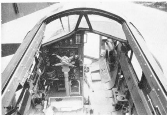
The cockpit of an early production Mk. IV at Filton, May 29, 1939. Instrumentation is sparse and ring-and-bead sight for the port wing 0.303-in. Browning machine-gun is equally basic. (Photo: Bristol T149/55)
