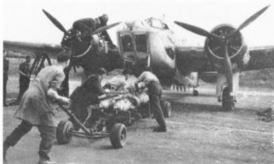
A Blenheim Mk. IV, June 1941, being prepared for an offensive sweep by R.A.F. Bomber Command, as armourers trolley-in a load of 4 x 250-lb. bombs. It appears that the cable-cutting devices on the wing leading-edges have been removed. (Photo: via C. H. Barnes collection)
