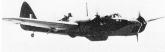
A Blenheim Mk. IVF fighter of late-series production, possibly Rootes-built, as used for "trade protection" and by the anti-shipping strike squadrons of R.A.F. Coastal Command. The four-gun pack is well silhouetted.
