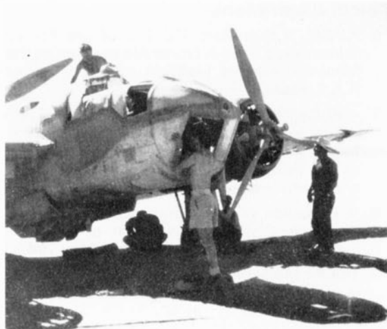
A close-up of the rediscovered Z7513 in 1959. The front panel had been removed because the fuselage contained an extraordinary field mod.—a long-barrel 20-mm. cannon. Eight Mk. IVFs were issued to the squadron. (Photo: Bristol via the author)
