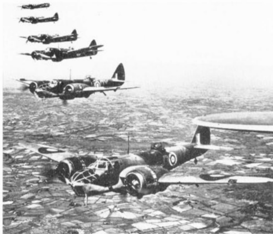
Blenheim Mk. IV fighters of No. 235 Squadron (coded DY) circa 1941. These are mid-production standard with single drum-fed Vickers K in the dorsal turret and a tray of four 0.303-in. Brownings under the bomb compartment.
