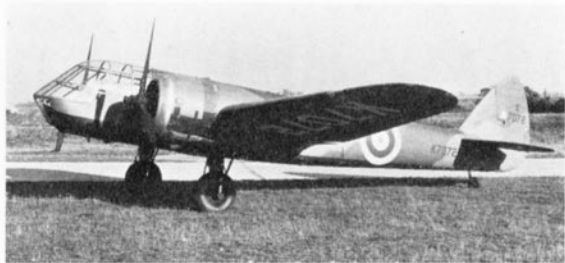
Above: From mock-up to reality in K7072, the workhorse prototype of the Type 149 Bolingbroke (later renamed Blenheim Mk. IV). These photographs, taken in October 1937, show the original "long-nose" application. The close-up of K7072, originally a Type 142 Blenheim Mk. I, reveals the early "snake's head" type of pitot extension and the subtle twin bulges in the amidships bomb-bay doors, against which the then "big" 500-lb. G.P. bombs would apply their self-opening bulk after carrier release. (Photos: Crown Copyright 9251 and Bristol T149/8)
