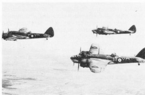
Mark IV Blenheims of No. 40 Squadron (coded BL and based at Wyton, Huntingdonshire) in formation, early March 1941. No. 40 Squadron returned from duty with the A.A.S.F. in France in December 1939 and re-equipped from Fairey Battle single-engine bombers. All have the under defence gun in the nose but the Blenheim second from the right has an unusually large rear-view mirror above the windshield. (Photo: Imperial War Museum CH786)
