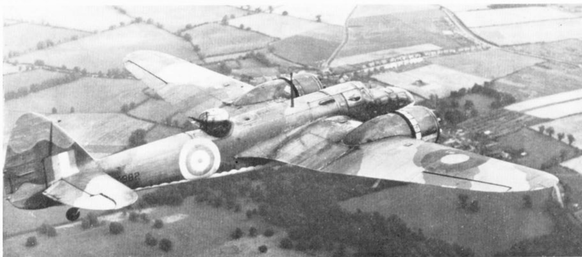
A Rootes-built Blenheim Mk. IV (V5382) flying over England in the late summer of 1941. The scallop-edging paint line is non-standard. The cockpit side panel blister for better oblique vision shows clearly. (Photo: via the author's collection)
