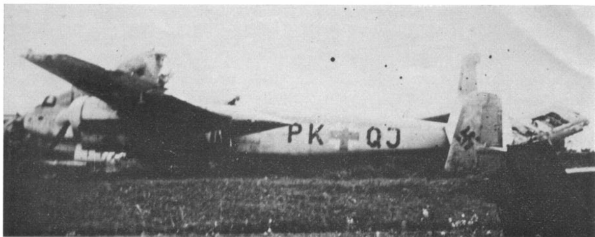
Used for exhaust flame-damper trials, the He 219 V 17 (coded PK + QJ), is seen here badly damaged after suffering main undercarriage failure. (Photo: via Ing. Fred Haubner)
