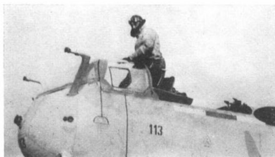
A test pilot climbs into the semi-open cockpit of the He 219 prototype, DV+DI, used for ejector-seat trials. Initially ballast, then dummies were fired from this aircraft. Later, Wilhelm Buss, one of Germany's most experienced parachutists carried out live ejections from the He 219. The main masts for the nose-mounted radar antennas are retained on this Uhu.
