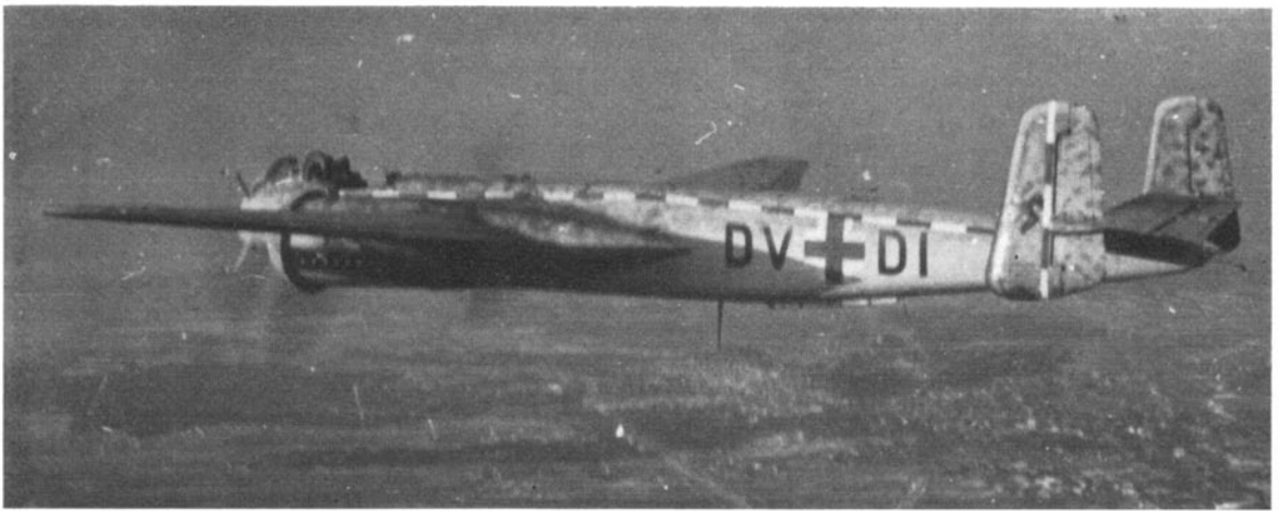
Two He 219 prototypes (the V 4 and V 6) were used at the Erprobungsstelle Rechlin for compressed-air ejector-seat trials during 1943–1944. One of these machines (coded DV + DI), with main canopy removed, is seen in standard night-fighter camouflage but with the addition of red and white checks running the length of the fuselage. Similar coloured checks are painted vertically on the fin. This paint scheme was designed to assist in-flight kinetheodolite measurements of the ejected seat's trajectory. (Photo: via the author)
