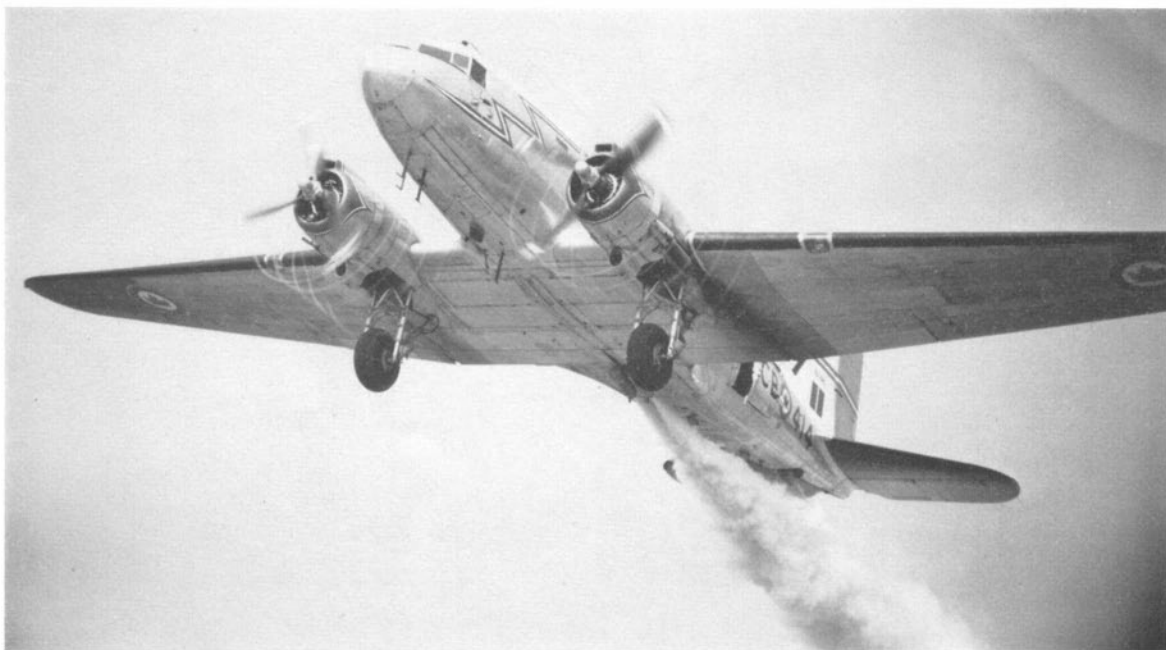
Action photo of Dakota Mk. III KG414 CB-414 C-47A-10-DK 42-92627 c/n. 12449 using RATOG bottles for take-off. KG414 served with the R.A.F. with No. 48 Squadron as "12-UG" during World War II, sold to the R.C.A.F. in August 1946 and one of eight Dakotas donated to the Indian Air Force in November 1962. (Photo: Canadian Armed Forces PL-88448)
