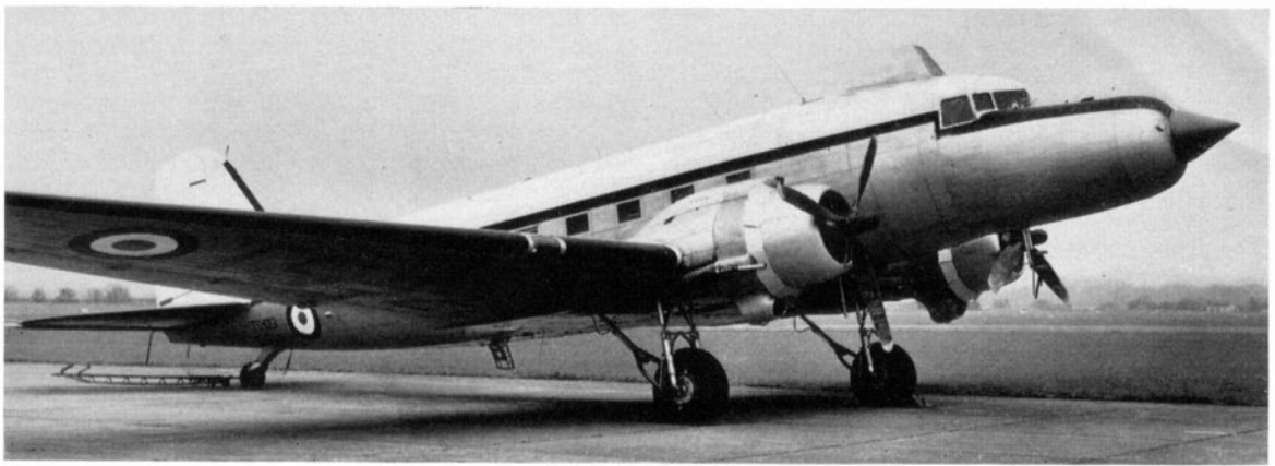
In 1952 the nose profile of TS423 was again altered to accept a bullet shaped structure to carry an Airpass radar. The "Hen Coop" above the cockpit was designed to carry a forward looking camera and also used for visual observation. (Photo: Ferranti 158D)
