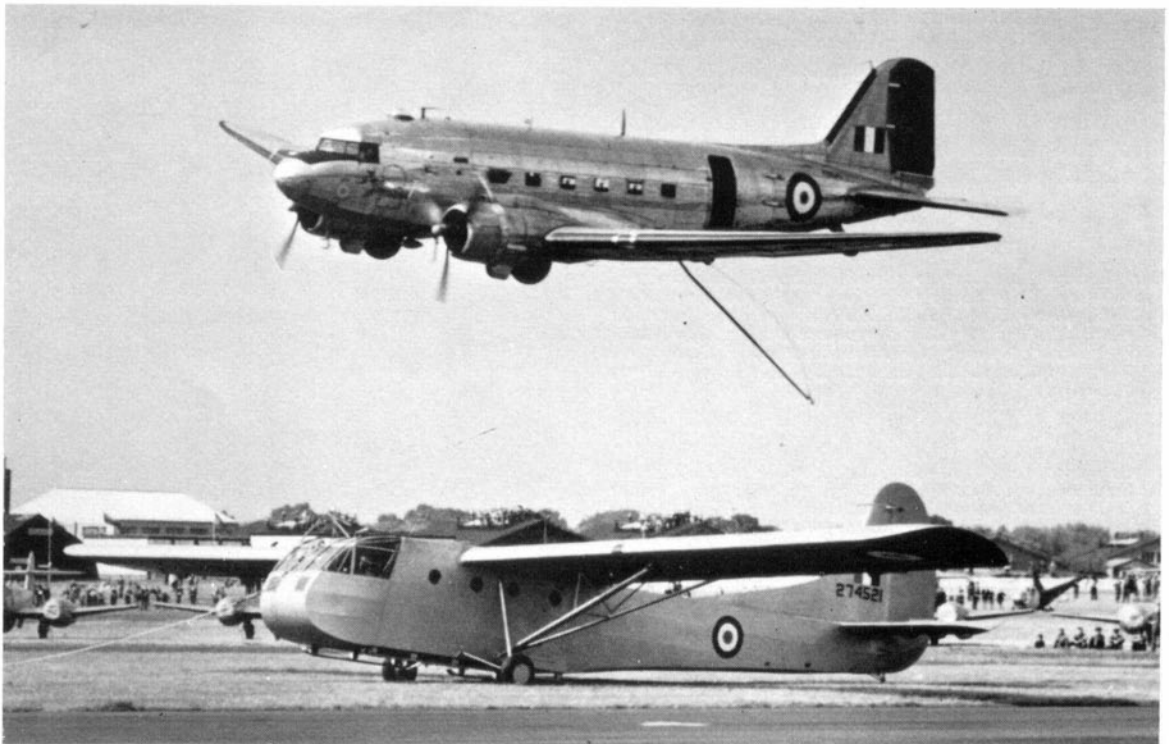
Formed at Ibsley after World War II the Glider Pick-up Flight operated with Dakotas modified for glider-tug snatch with Waco Hadrian gliders. The system was demonstrated to the public at the R.A.F. Display, Farnborough in 1950 as seen by the photo. The Hadrian still retains its U.S.A.A.F. serial 274521.
