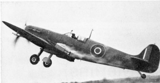
Supermarine-built Seafire Mk. IB. MB307 taking off with R.A.T.O.G. Note revised fuselage and fin markings. (Photo: Flight)
