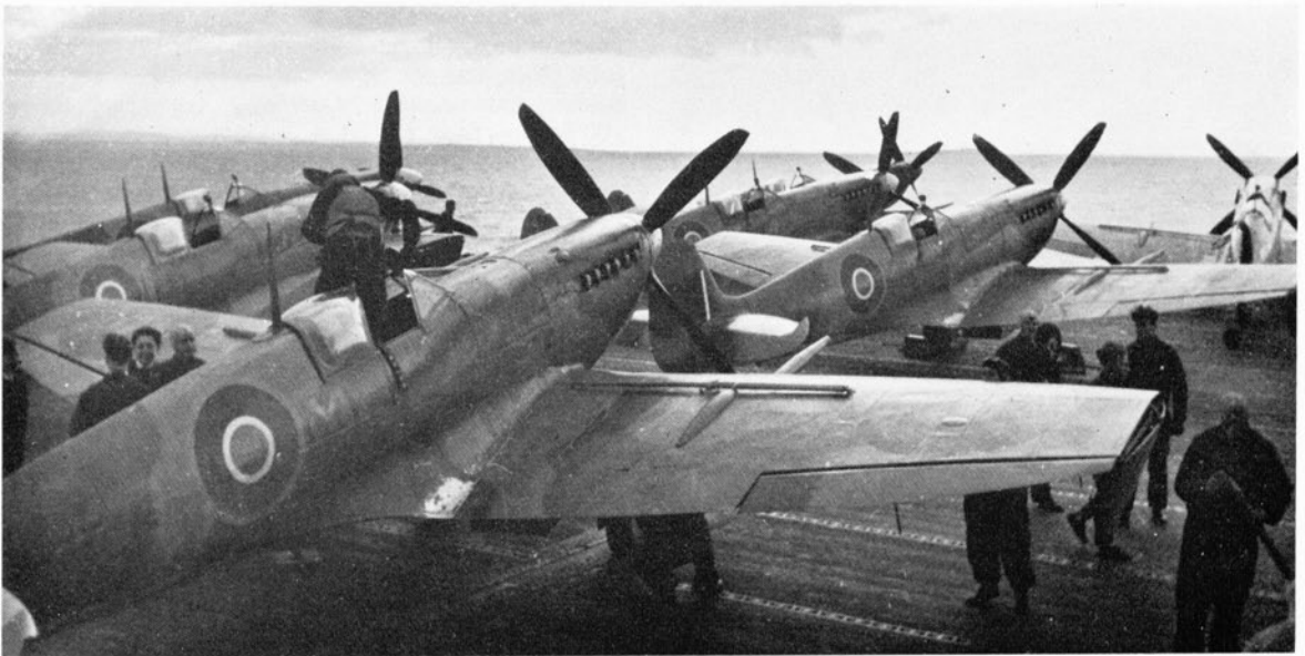
Seafire Mk. IIIs of No. 899 Squadron aboard H.M.S. Khedive. Note wing tips folding down to facilitate deck parking. (Photo: L. J. Kelly via M. Garbett)
