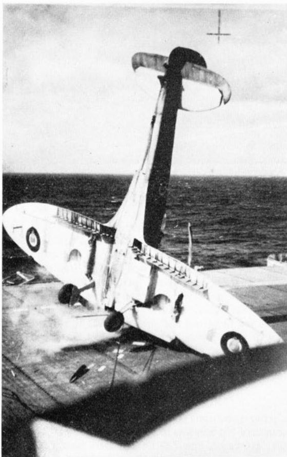
Another landing sequence, this time aboard H.M.S. Hunter working-up in Irish Sea, early 1944. Seafire Mk. III LR717 "H-J", of No. 807 Squadron loses its engine. Note hook has momentarily swung back into the normal retracted position—in the first photograph—due to the braking force of impact. (Photos: G. E. Thomas via M. Garbett)
