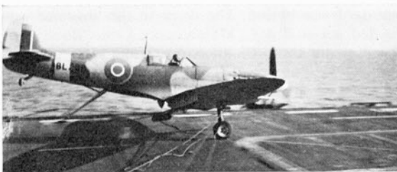
Hooked Spitfire BL238 making a heavy landing on the Training carrier H.M.S. Ravager. Note port undercarriage leg has already collapsed. Aircraft still retains the "sky" fuselage band. (Photo: C. Vale via M. Garbett)
