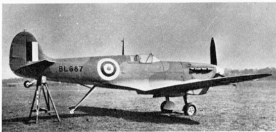
Hooked Spitfire Mk. VB BL667/MB329 resting on trestle, clearly showing the arrester hook in lowered position. (Photo: Real Photographs, Liverpool)
