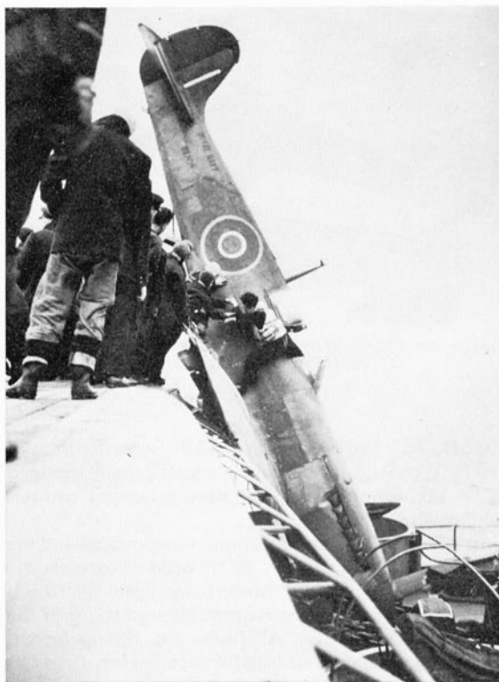
Another mishap aboard H.M.S. Ravager with the pilot extricating himself from hooked Spitfire F. Mk. VB. BL818. Note signs of repair to rear fuselage section and that the engine has six exhaust manifolds. (Photo: C. Vale via M. Garbett)
