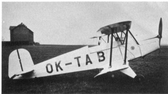
The first Czechoslovakian licence-built Tatra T-131 (licence Bü 131 B) OK-TAB. Colour scheme was light grey overall with black struts and registration letters. The nose flash was red. Forward of front cockpit is the Tatra badge. (Photo: via Vaclav Nemecek)
