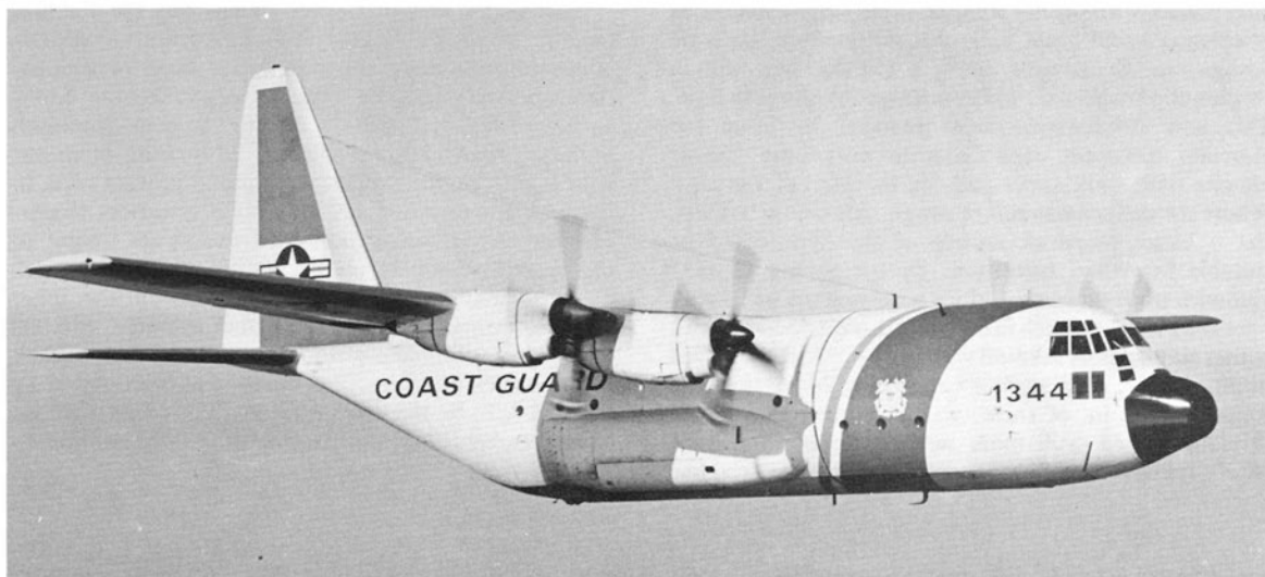
The SC-130B Hercules, seen here in its striking red, blue and white livery, was the first turbine-engined aircraft to equip the US Coast Guard when introduced in early 1960. Note the 4-bladed propellers. (Photo: U.S.C.G.)
