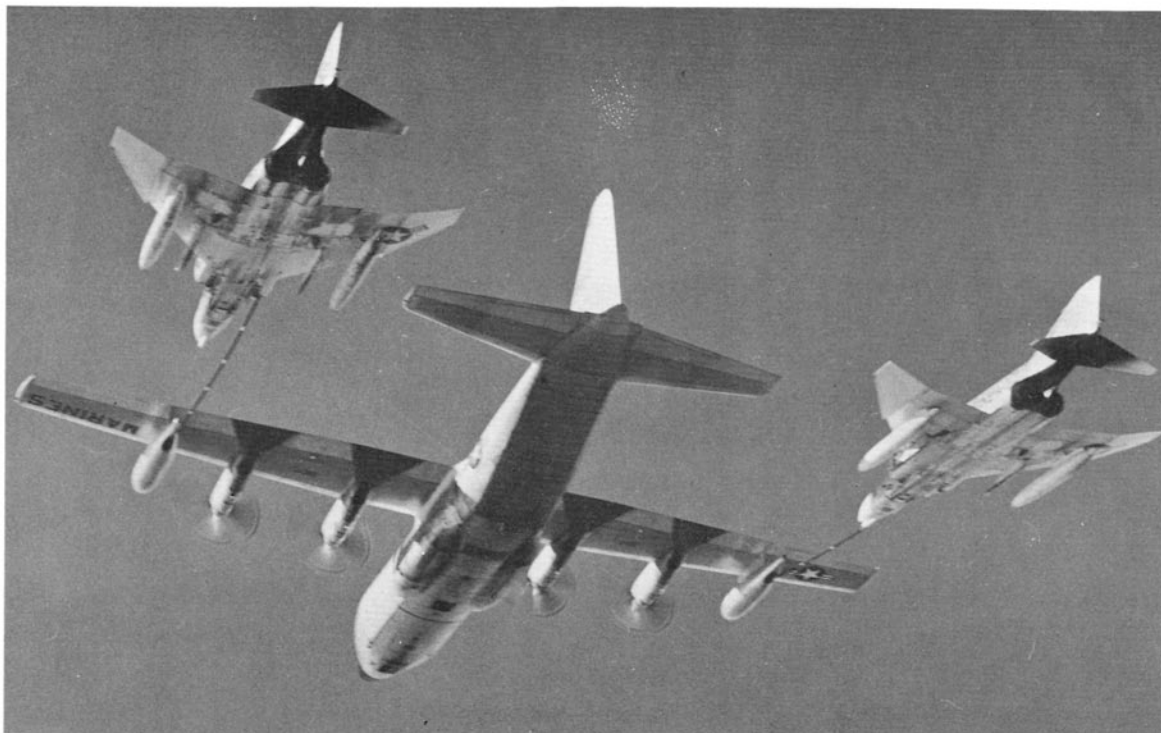
Two US Marines F-4 Phantoms take on extra fuel from a KC-130F (GV-1) Hercules, also of the US Marines.
