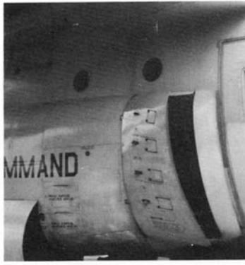
On closer inspection, (left) HC-130H (65-0975) shows the recovery "Yoke" at rest, (centre) the double-slotted Lockheed-Fowler mainplane flaps and (right) tandem-wheel undercarriage bulge also housing four vertical sited windstream deflectors used when airdropping parachute troops. (Photos: G. Pleasance)
