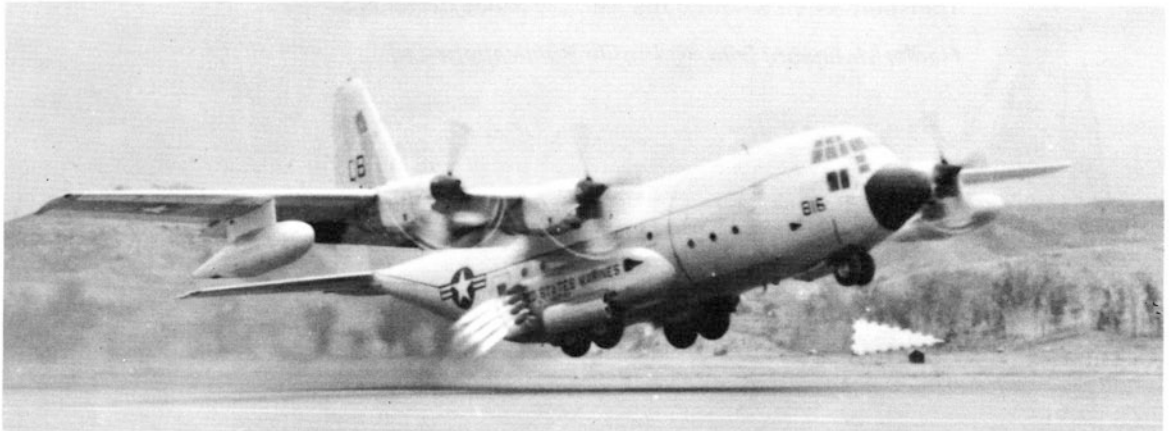
This KC-130F of US Marines Squadron VMGR 352 is boosted into the air with the aid of eight 1,000 lb thrust rocket units, located on the rear of the main undercarriage blisters. Note the large, tandem wheels on each main undercarriage unit. (Photo: U.S.M.C.)
