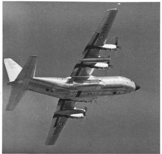
Another Hercules tanker, this time the HC-130P of the USAF, for in-flight helicopter refuelling. (Photo: Lockheed)
