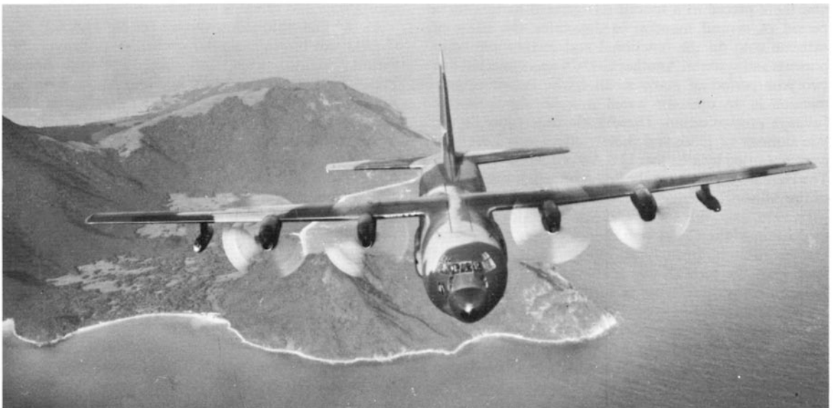
This USAF C-130A, depicted off the coast of South Vietnam in December 1966, sports full camouflage and two 450 U.S. gal underwing tanks mounted on pylons. (Photo: U.S.A.F.)
