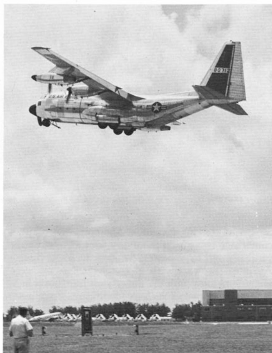
"BLC"—the Boundary Layer Control Hercules was tested in 1960 to meet U.S. Army requirements for a heavy transport with STOL—(Short-Take-Off-and-Landing) capability. Initially the C-130C, this converted C-130B became the NC-130B. Noticeable differences are the extra outboard turbojets and increased rudder and aileron chords. Note airflow tufts on rudder. (Photo: Lockheed, via David A. Anderton)
