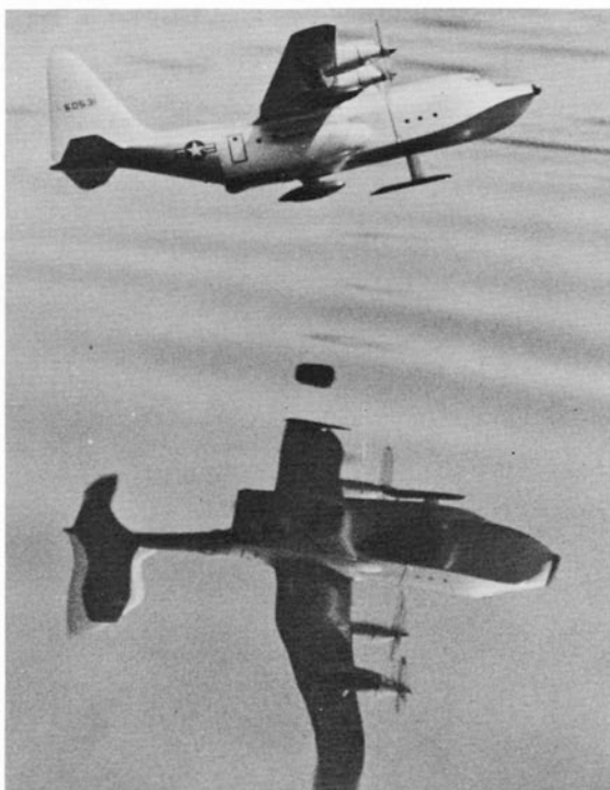
"HOW"—the "Hercules-on-Water" project was U.S. Navy Air Systems Command-sponsored in 1968 for hydroski feasibility studies. Lanier Industries of Gainesville, Ga., was sub-contracted to build 8 ft. 3 in. wingspan boat-hull/tip floats' model for tests on Lake Lanier using radio-control. Jet engine intakes were to be inverted as on Lockheed L-188 Electra. (Photo: Lockheed, via David A. Anderton)
