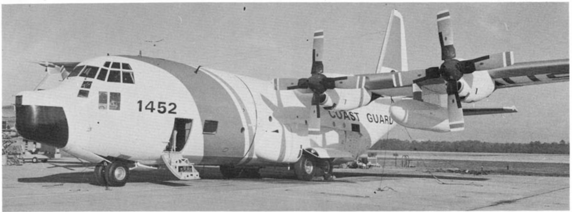
One of the three HC-130H Hercules of the US Coast Guard, with more powerful 4,500 eshp engines and an extended nose with provision for the "Yoke" recovery system. (Photo: Lockheed)
