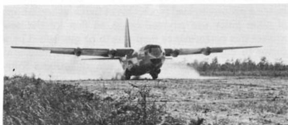
One of the YC-130A prototypes demonstrates its ability to take off from a soft, rough airstrip, merely a sod stretch hastily cleared of the scrub vegetation. (Photo: Lockheed)
