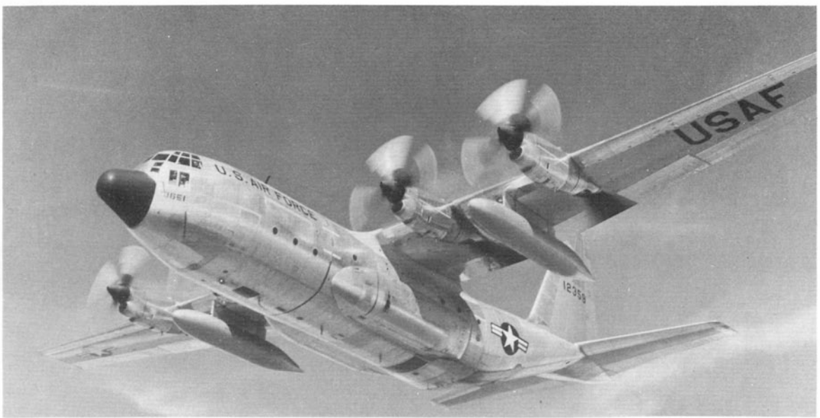
One salient feature of the C-130E, seen here in USAF markings, is the 1,360 US gal supplementary fuel tank under each wing. (Photo: Lockheed)
