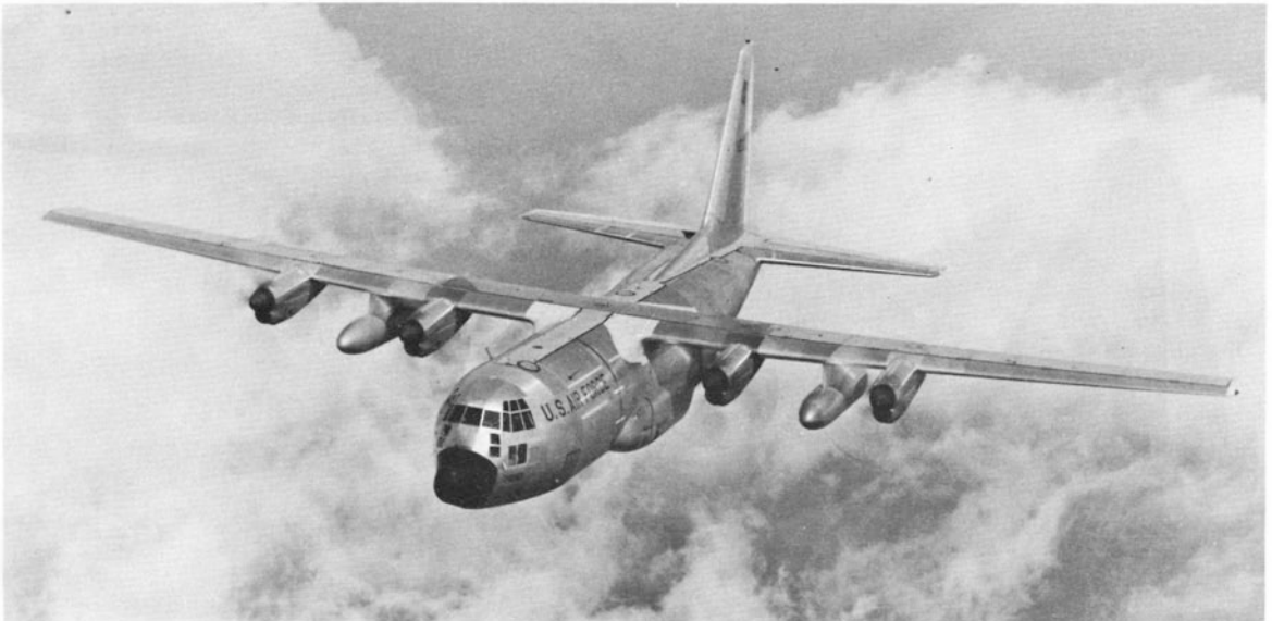
Another view of the same USAF C-130E as that shown in the previous picture, illustrating the compact installation of its 4,050 eshp T56-A-7 A turbo-props. (Photo: Lockheed)
