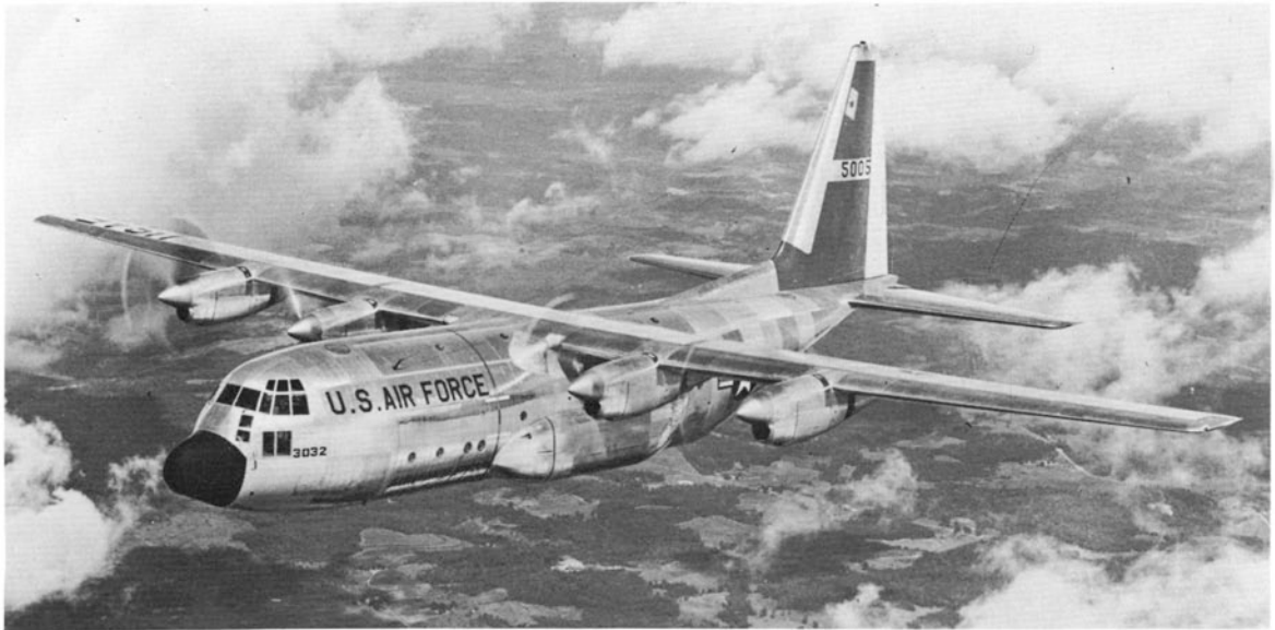
An early USAF C-130A. Note the extensive cockpit glazing, with windows extending down to floor level, and the enlarged nose radome which distinguishes production aircraft from the prototypes. (Photo: Lockheed)
