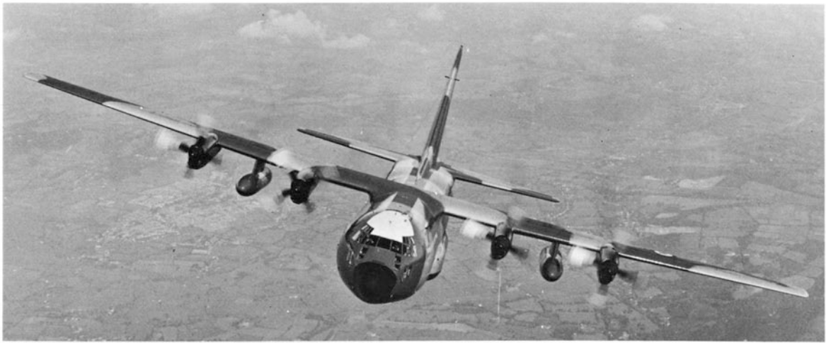
Head-on view of another RAF Air Support Command C-130K. Like the C-130Es, these aircraft feature 1,360 U.S. gal underwing fuel tanks. (Photo: R.A.F.)
