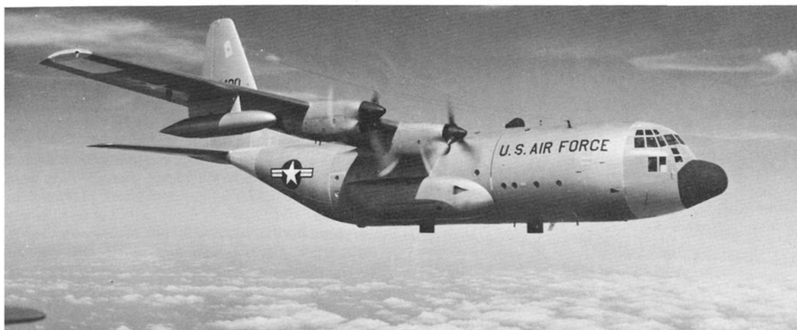
Seen over Florida on October 19 1962 is this uncamouflaged USAF C-130A, with auxiliary wing-mounted 450 U.S. gal fuel tanks. Prominent in this view are the large main undercarriage blisters, and the parallel cross-section of the single cargo hold. (Photo: U.S.A.F.)
