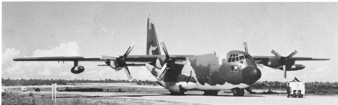
A USAF C-130A takes its rest at a base in Southeast Asia, in 1965. Note the three-bladed propellers which distinguish this series from later variants, and the slight wing anhedral. (Photo: U.S.A.F.)
