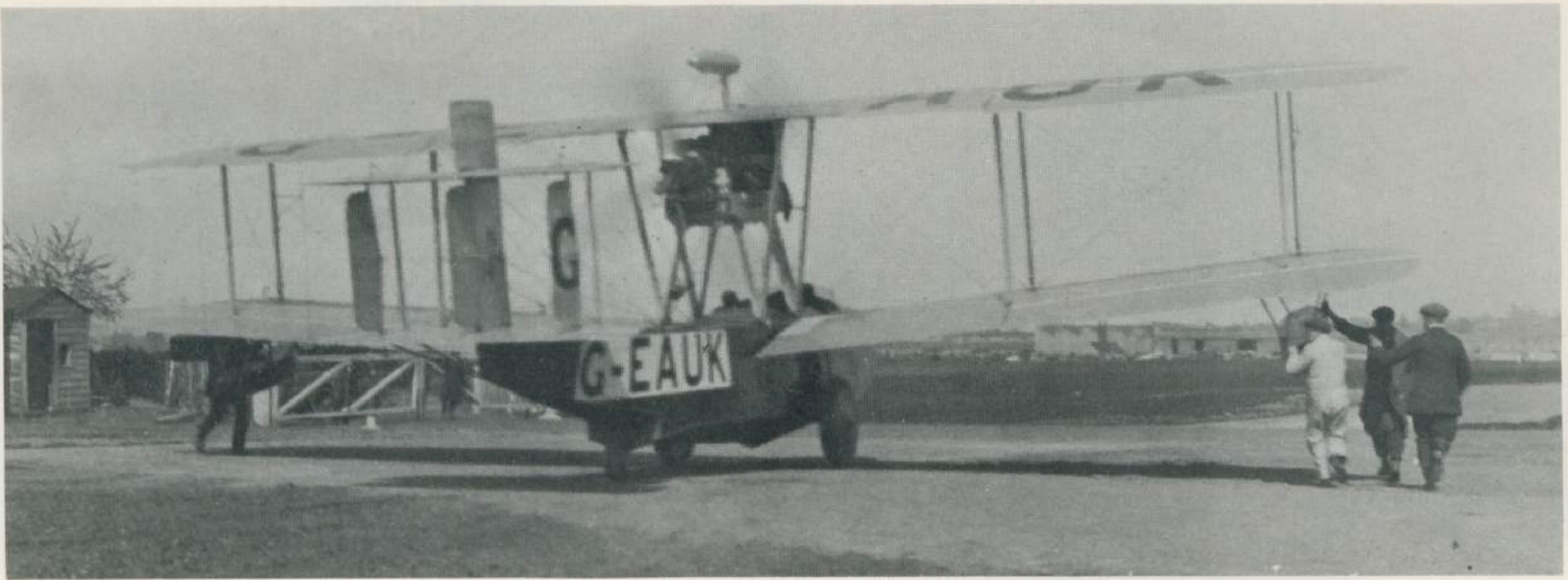
Father: Vickers Type 59 Viking III G-EAUK , seen crossing the railway level crossing at Plough Lane, Croydon, in September 1920 (see page 28). Pilot, Captain S. Cockerell. The slab-sided hard-chine hull contrasts with the more aesthetic rotundity of the Seal/Seagull.
