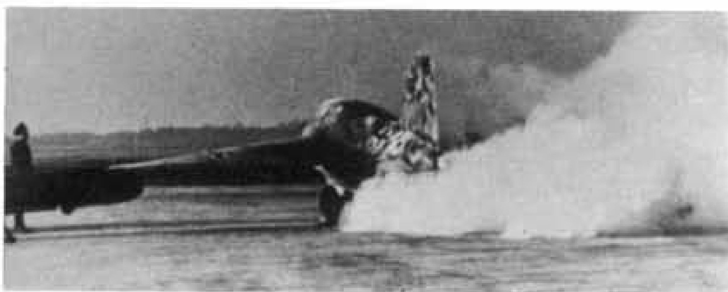
Clouds of steam billow from beneath an Me 163 B of J.G.400 as its pilot goes through the start-up procedure. T-Stoff was 80% hydrogen peroxide and apart from its main function as a fuel propellant, was also used to initiate a cycle that produced steam to power the turbine driving the two main fuel pumps. (Photo: Herr Husemann)
