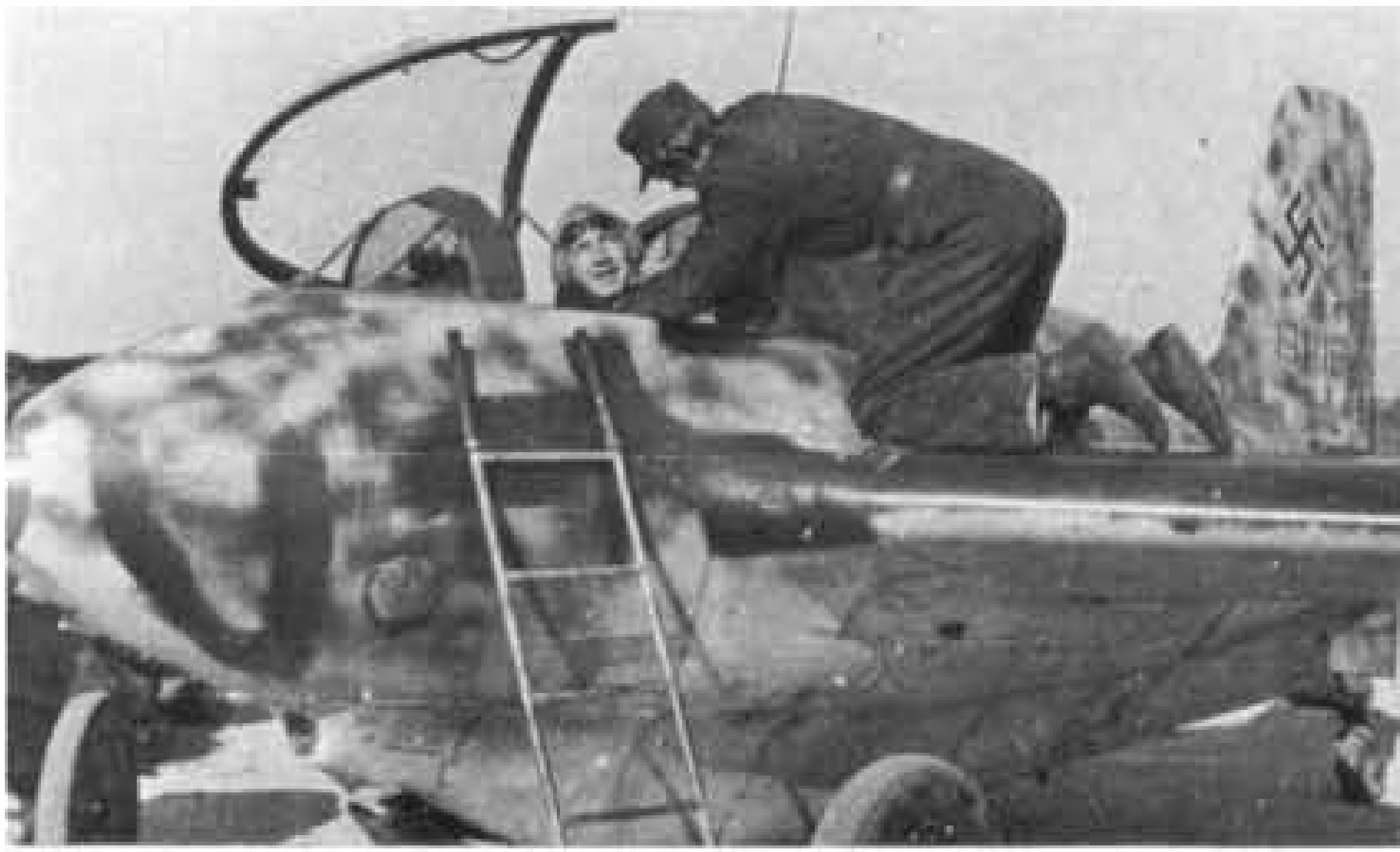
A mechanic helps a pilot of Jagdgeschwader 400 to adjust his straps prior to start-up in Me 163 B-1, W.Nr. 191116. Aircraft of this Geschwader carried a wide variety of camouflage finishes and it would appear that this Komet has not fired its 30-mm. MK 108 cannon since the application of additional doping. The thick plate of bullet-proof plexiglas forward of the cockpit was not integral with the canopy and was sprung in order to lessen the-chance of splintering if hit by enemy fire.
