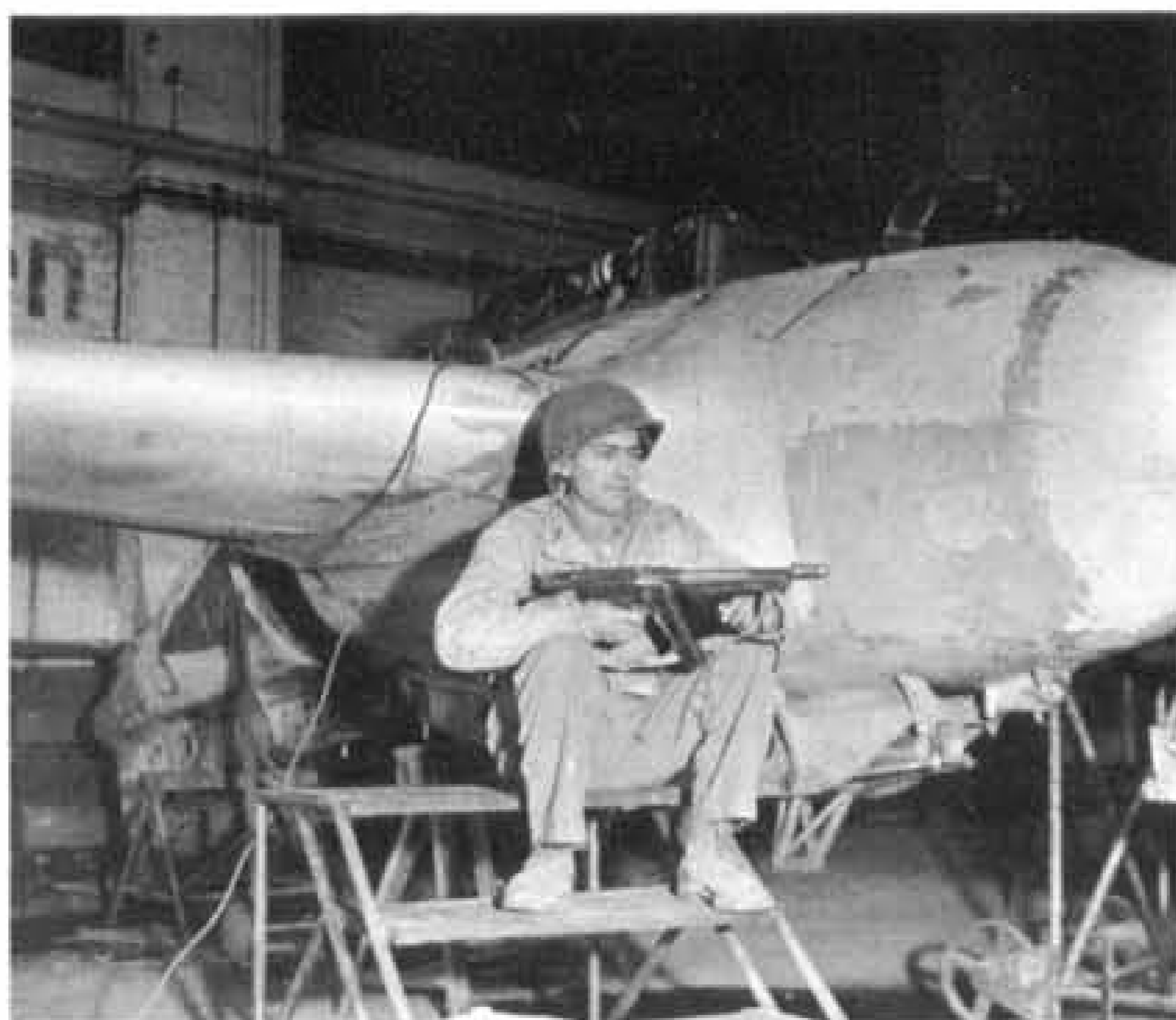
Probably relegated to a ground instructional rôle, the Me 163 B V 13, seen here in a hangar at Polzen on April 19, 1945, guarded by a private of the U.S. First Army's 9th. Armoured Division, was still flying at Lechfeld during August 1944. On the 18th. of that month, it underwent a rocket motor change: a Walter 109-509 A-0 being removed and a new A-1 engine (W.Nr. 3487) being installed in its place.
