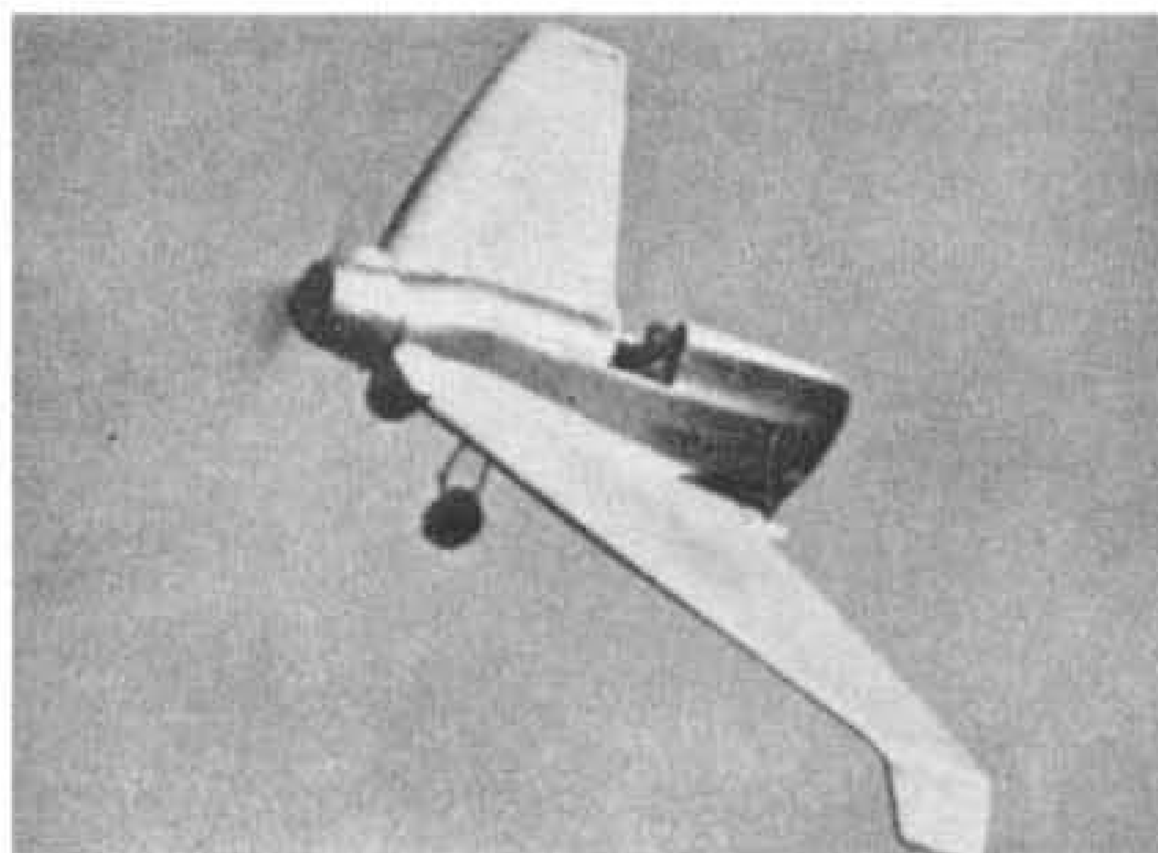
The all-wing, tractor-powered D.F.S. 39 Delta IVd with marked anhedral on the wing-tips. (Photo: via Air-Britain archives)
