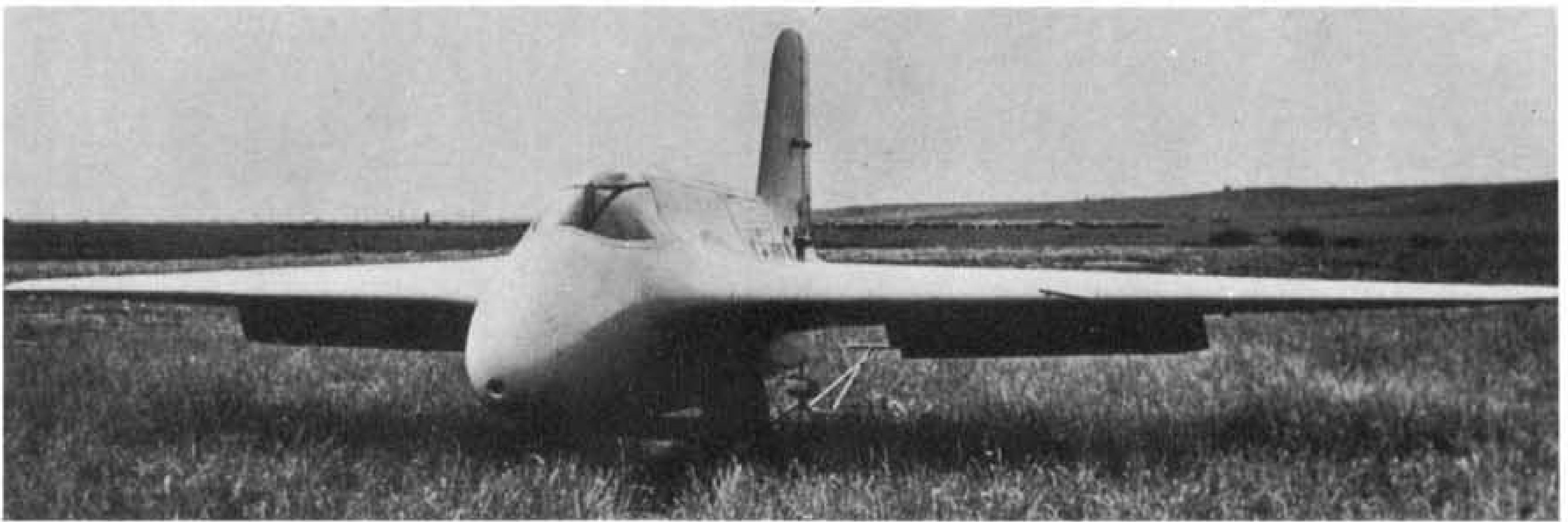
A refined version of the DFS 194, the Me 163 AV 1 (first prototype), KE+SW, resting on its take-off trolley with a wheeled tail-mounted cradle attached for ground-handling. Taken at Augsburg, this view shows the large-area landing flaps in the lowered position.
