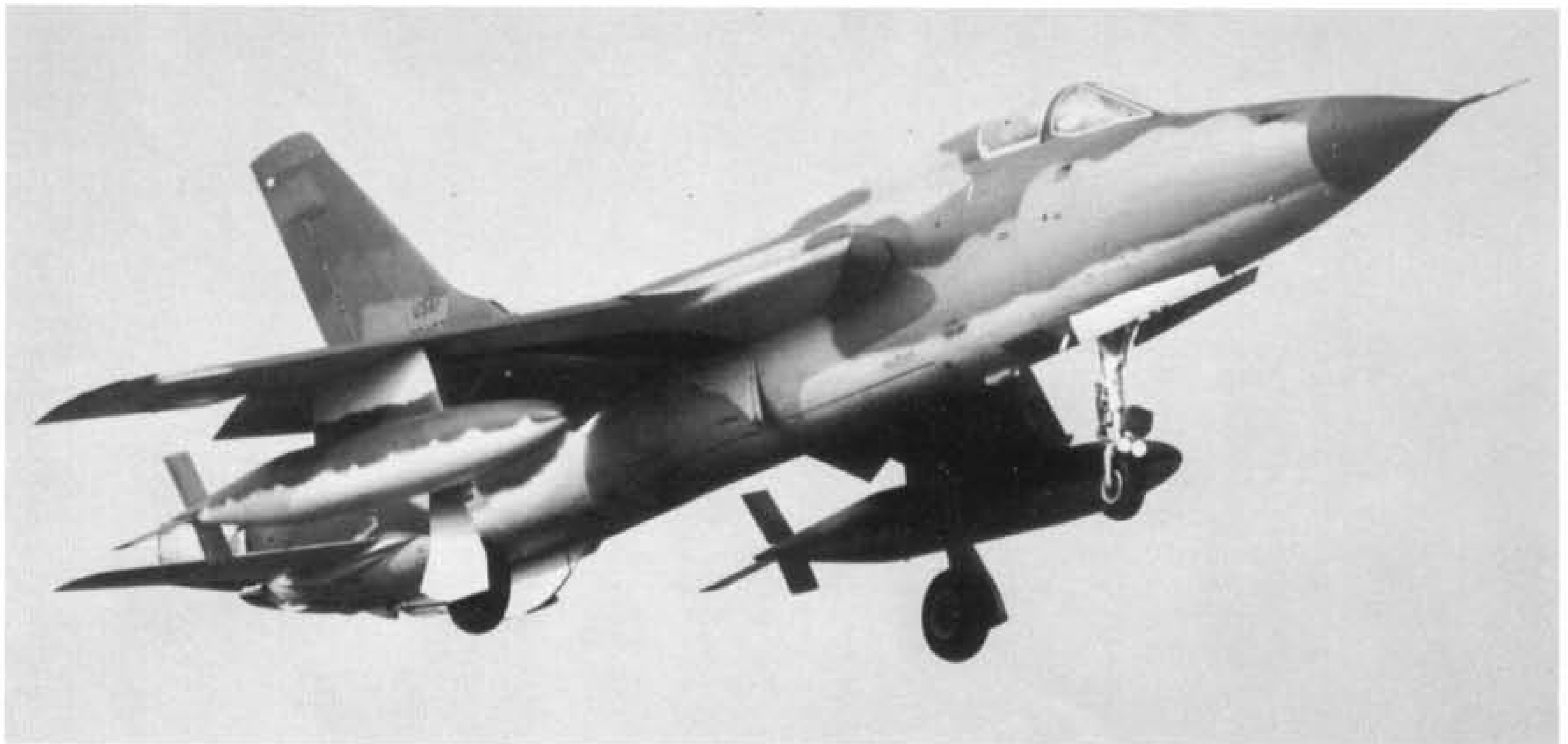
Yet another camouflage variation, even extended to pylon fuel tanks. Photographed in Japan in 1966, USAF: 60-0427 was the first of the 121 F-105D-10REs ordered. The slightly stepped-down twin landing lights between the nosewheel and radar reflector are revealed to advantage. (Photo: "Aireview", Japan)
