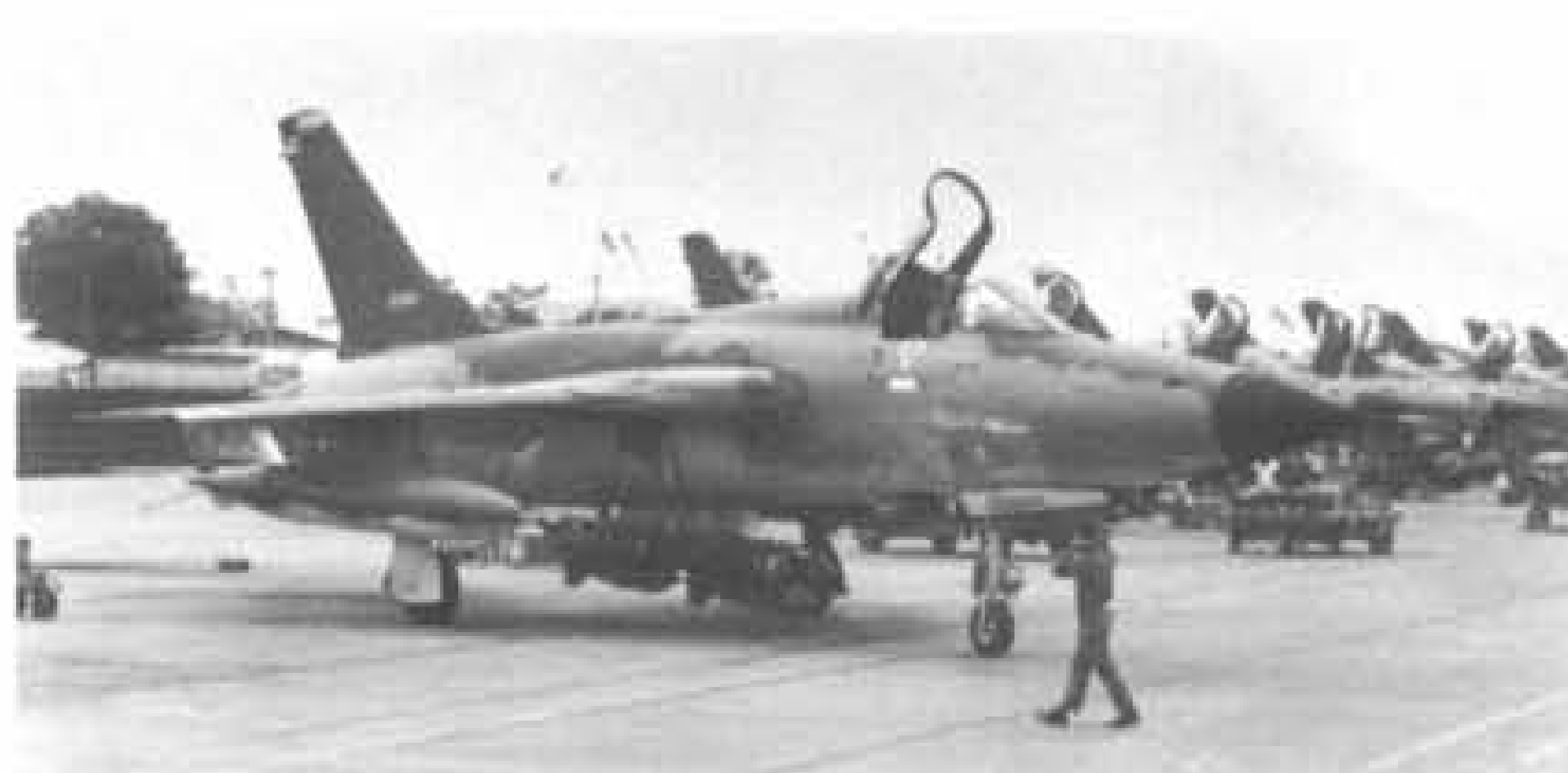
At Takhli Air Base, Thailand, 1968, an F-105D-31RE (62-4364) is being readied for another sortie and is armed with 6 x 750-lb M-117 bombs. By late October 1968, the 355TFW's "364" had become one of the first four Thunderchiefs to log 3,000 flying hours. (Photo: F.H. Republic ref. B-16290)
