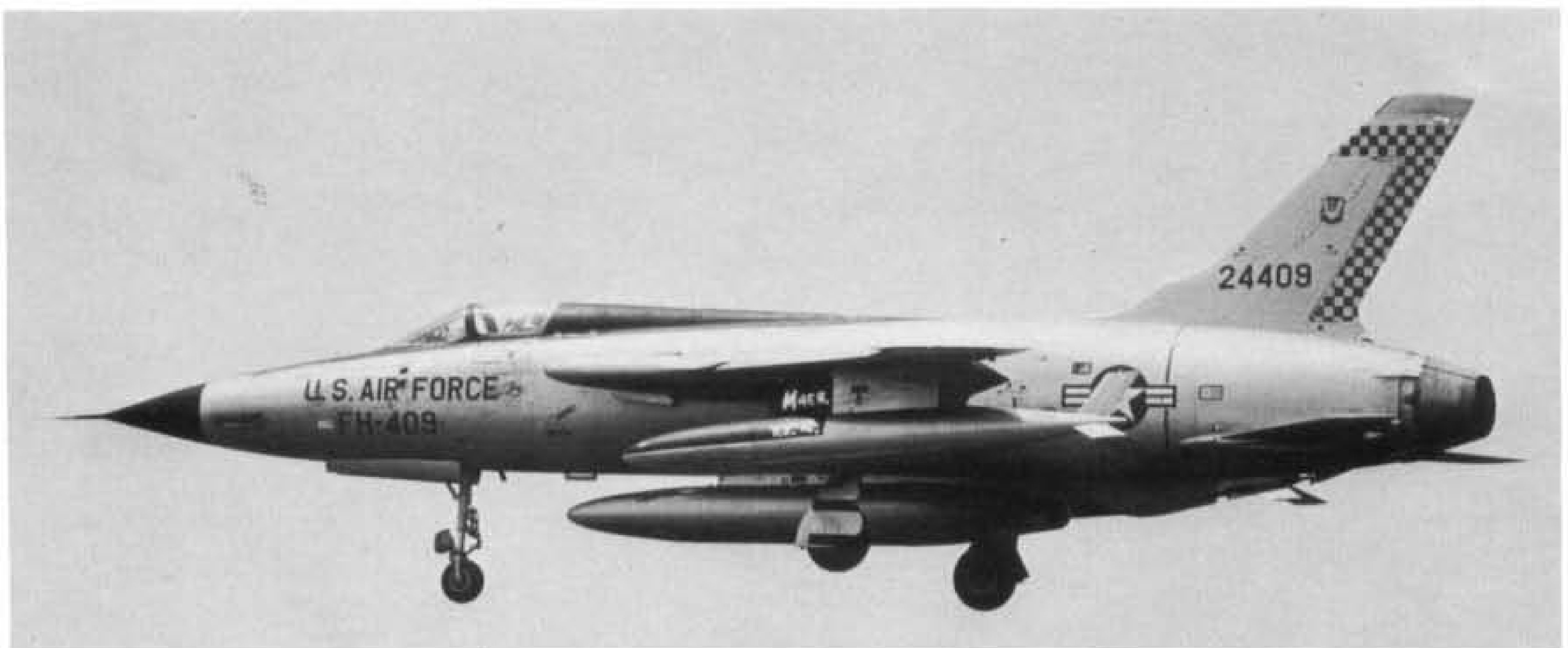
An F-105D-31RE out from Yokota AB, Honshu, Japan, in late 1964, in the colours of the 561TFS/23TFW whose home base is McConnell AFB, Kansas. This may account for the hurried scrawled "MAFB" on the outer wing pylon. Emblem on the fin is that of TAC. Nosewheel strut radar reflector shows clearly. (Photo: "Aireview", Japan)
