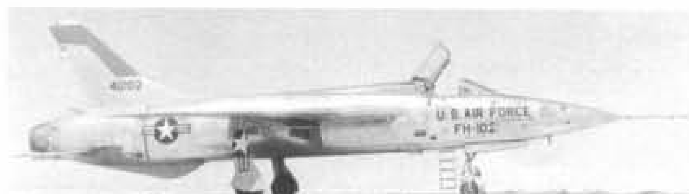
Two views of 54-0102, the third of four F-105B-1REs and the fifth Thunderchief to be built. In the first photograph, "102" has been set up for a publicity photo-call with correct "Buzz No." of FH-102 ignored in the interests of the more obvious "F-105". The centreline tank holds 650 US gals. of fuel and the wing pylons mount dummy 3,000-lb and 750-lb stores. The later photograph shows FH-102 at the Air Force Flight Test Center, Edwards AFB, California on June 20, 1958. Transparency behind canopy is evident on this development "Bravo Chief". (Photos: Fairchild Hiller Republic ref. B-2680 & USAF ref. 4526-AC)
