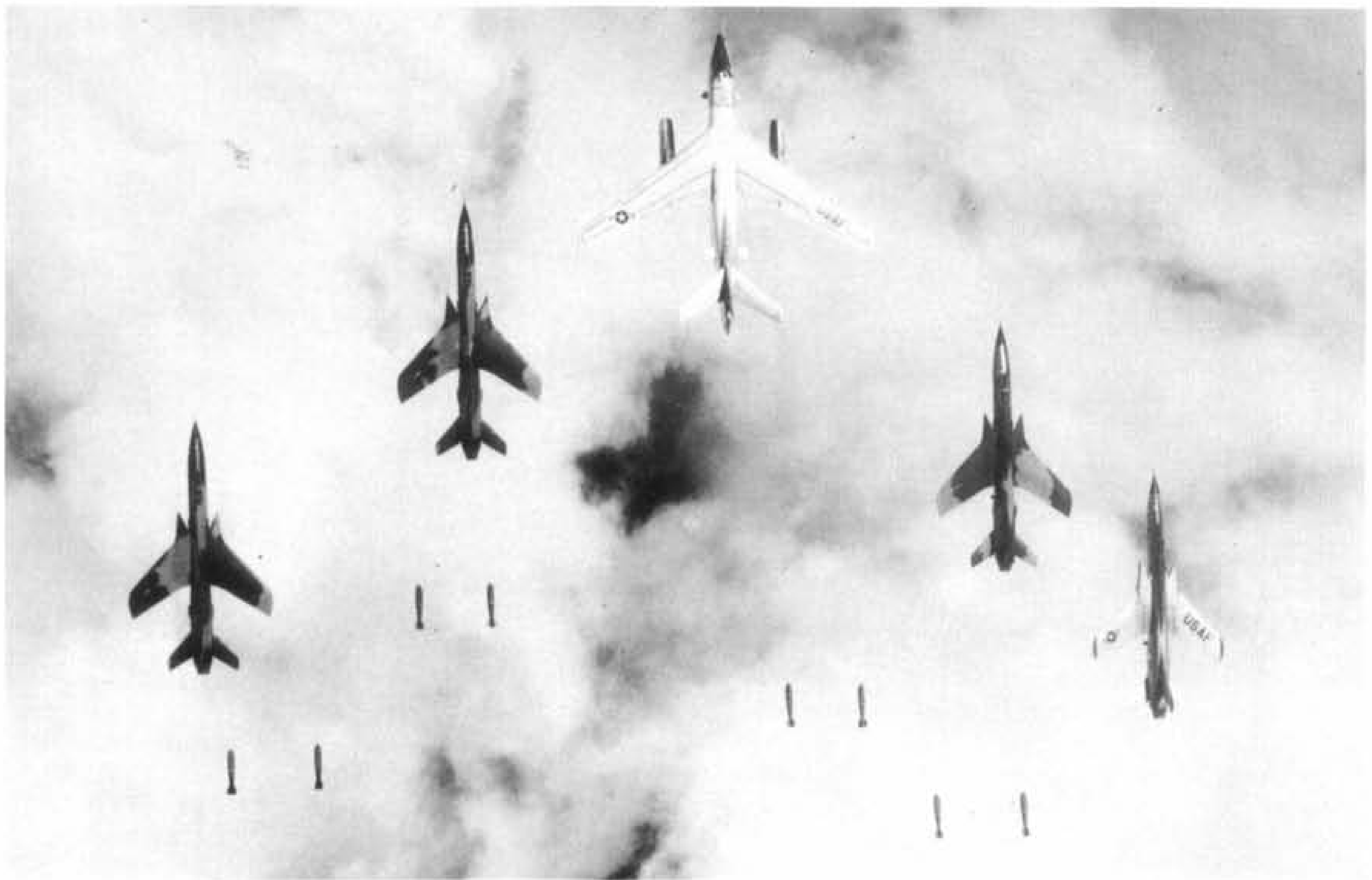
Study in planforms as a jet "pathfinder" Douglas EB-66 Destroyer provides four Tactical Air Command F-105Ds with radar control through 8/8ths cloud cover over the "southern panhandle" of N. Vietnam on June 14, 1966. On the three camouflaged F-105s, the remarkable "sawtooth" wing leading-edge air intakes stand out more clearly than on the all-silver Thunderchief. All four F-105s have just released their two 3,000-lb M-118 wing pylon-mounted bombs, a load 50% greater than Boeing B-17G Flying Fortress of World War Two. This incident was recorded by a shadowing photo-reconnaissance McDonnell RF-101C Voodoo of TAC. (Photo: USAF ref. 96182)
