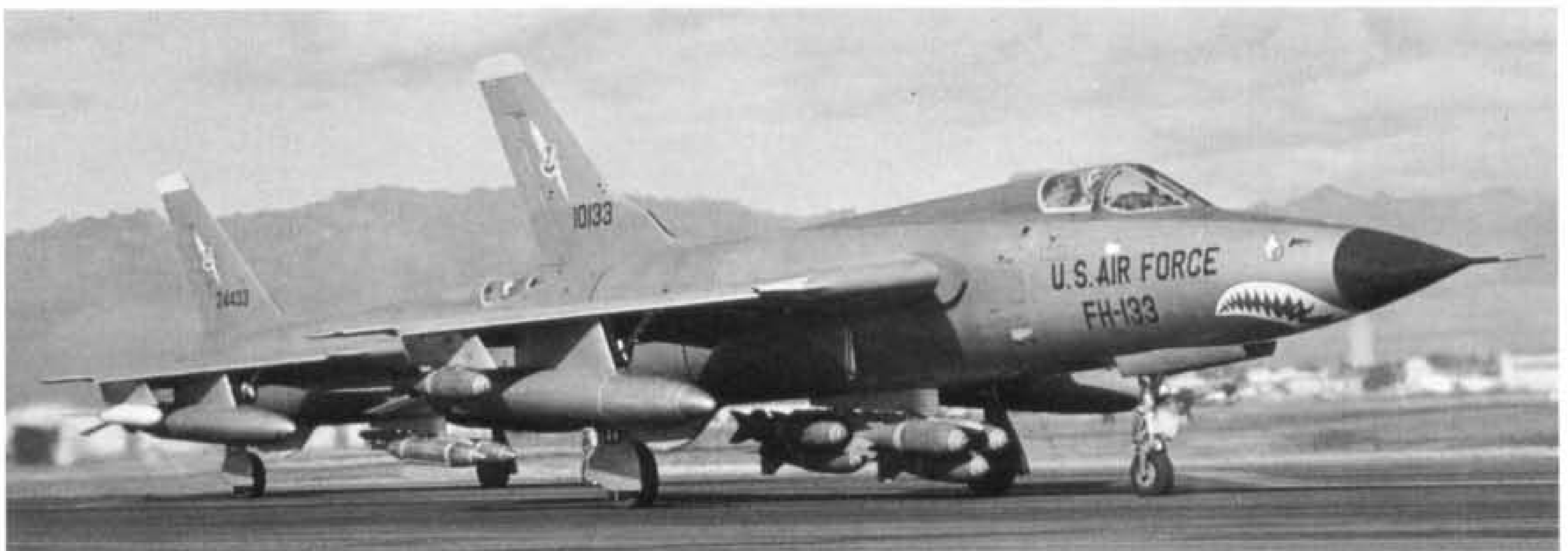
The "Flying Tigers" tradition of the 23rd Fighter Group (activated 1942) lives on in this photograph taken in the mid-1960s at the 23TFW's South Vietnam base of Da Nang Airport. "FH-133" is an F-105D-20RE armed with six 750-lb M-117s on the centreline MER (Multiple Ejector Rack), and one pylon-mounted M-117 bomb on each wing. A pair of 450 US gal. fuel tanks complete the external load. On the MER of the F-105F-1RE to the rear are a pair of fire bombs (napalm). MER-cluster ground clearance is impressively economical! (Photo: USAF Official)
