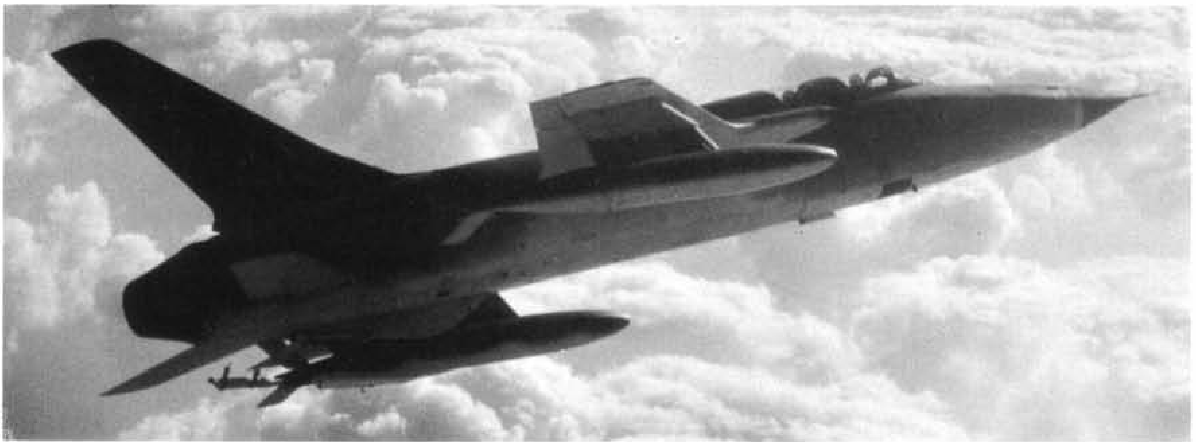
The clouds remember. An evocative study in near silhouette of F-105F-1RE (63-8268) of the 12TFS/18TFW in November 1967 when based at Kadena AB, Okinawa. From the outer port wing pylon is the launch equipment for the high-speed dart trailed for air gunnery training. The dart gear is illustrated on page 79. (Photo: "Aireview", Japan)
