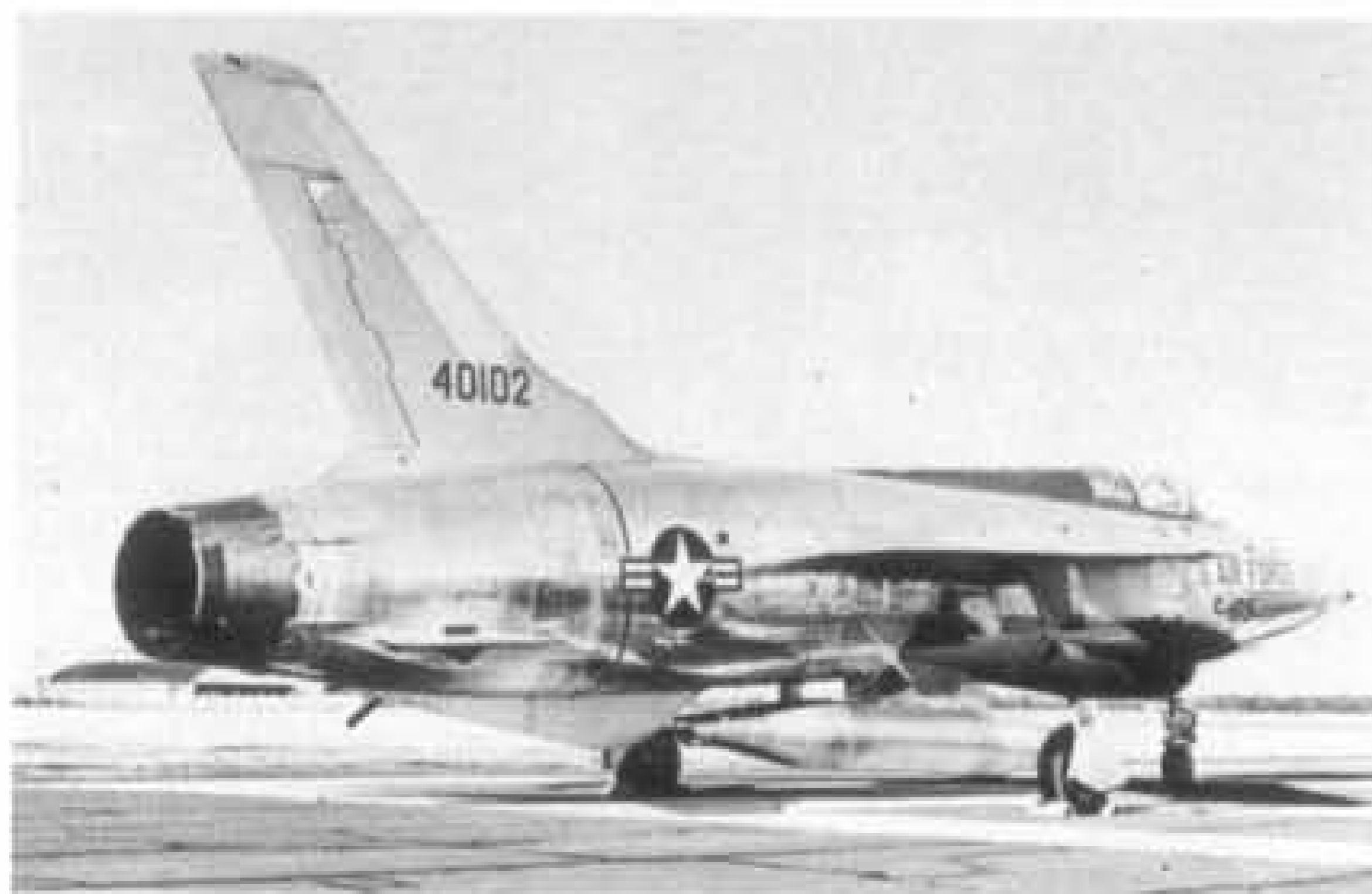
Two views of 54-0102, the third of four F-105B-1REs and the fifth Thunderchief to be built. In the first photograph, "102" has been set up for a publicity photo-call with correct "Buzz No." of FH-102 ignored in the interests of the more obvious "F-105". The centreline tank holds 650 US gals. of fuel and the wing pylons mount dummy 3,000-lb and 750-lb stores. The later photograph shows FH-102 at the Air Force Flight Test Center, Edwards AFB, California on June 20, 1958. Transparency behind canopy is evident on this development "Bravo Chief". (Photos: Fairchild Hiller Republic ref. B-2680 & USAF ref. 4526-AC)
