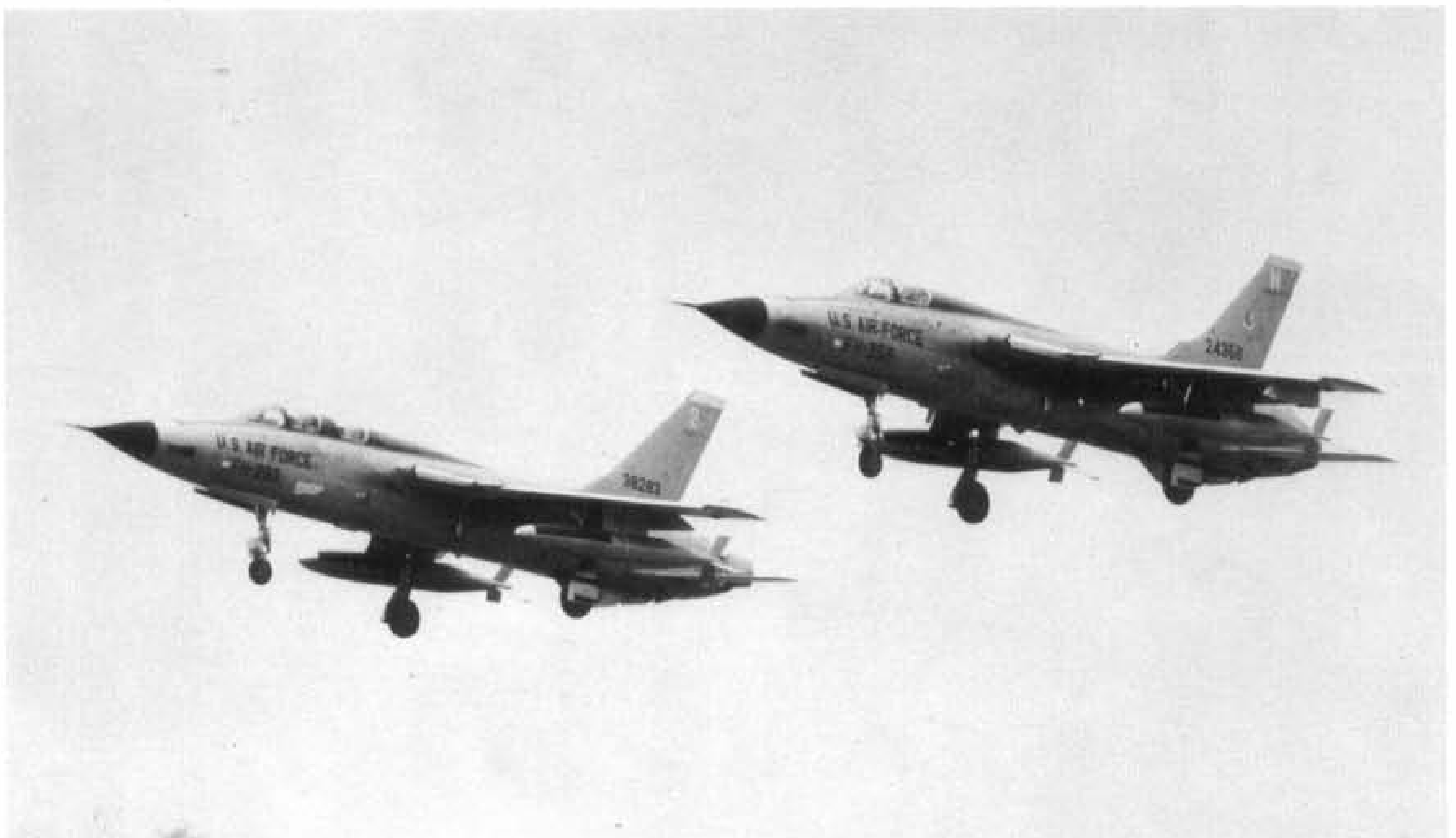
Study in development, "Foxtrot" and "Delta" Thunderchiefs. The tandem-seat "FH-283", an F-105F-1RE (62-8283) comes in to land at Yokota Air Base, Honshu, Japan, alongside "FH-358", an F-105D-31RE (62-4358). Both, at this time (1964) were allocated to the 6441TFWing. The approx. 8% increase in length of the F-105F is hardly noticeable but the ventral tail fin clearly shows the outline of the arrestor hook applied to all F-105Ds and 'Fs and late-production F-105Bs. (Photo: "Aireview", Japan)
