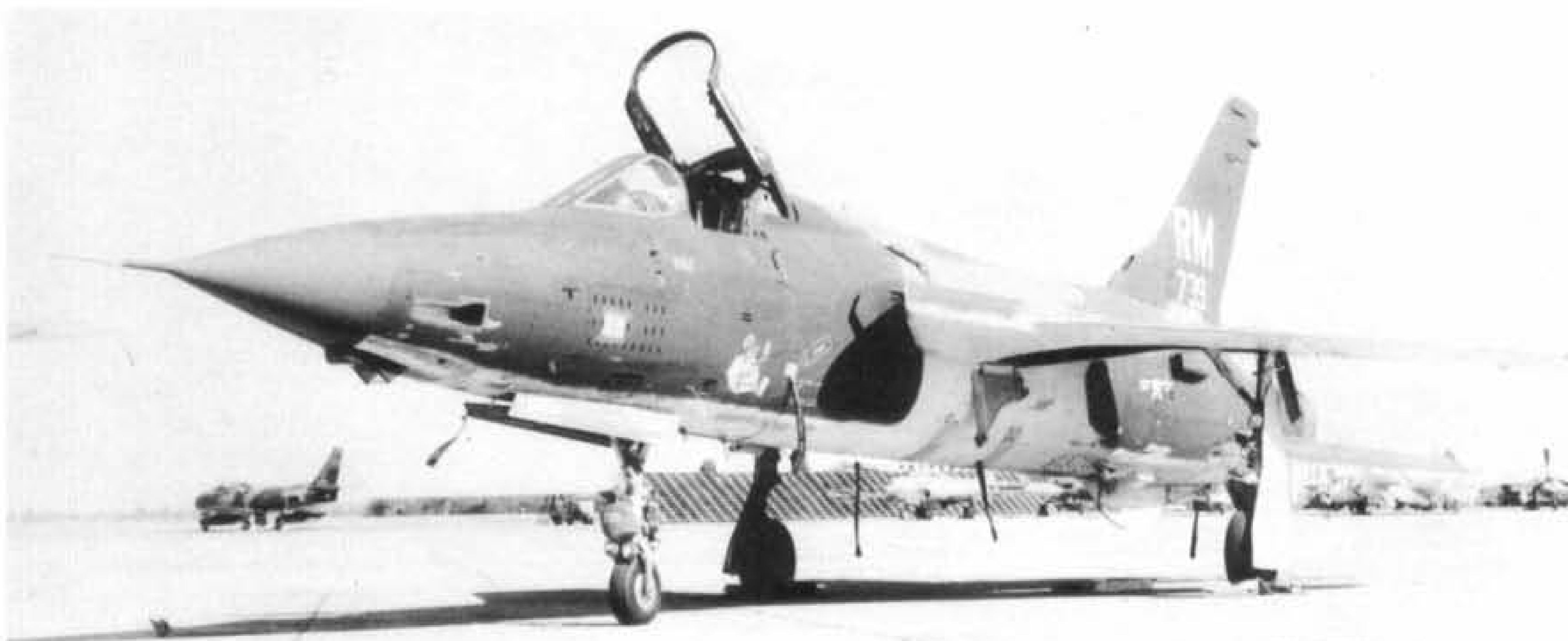
The subject of No. 8 of the colour artwork side views, "RM 739" is another F-105D-5RE (59-1739) of the 354TFS/355TFW, seen here at McClellan AFB, California, in June 1969. The triple row of eight louvres to exhaust the gases from the six-barrel 20-mm M-61 Vulcan cannon stand out clearly just above the nosewheel doors, as does the boundary-layer fence at the wing root and the strike camera immediately behind the radar nose cone. The F-105D's "last three" appears in white on the nosewheel radar reflector. In the background, a camouflaged North American F-86 Sabre.
