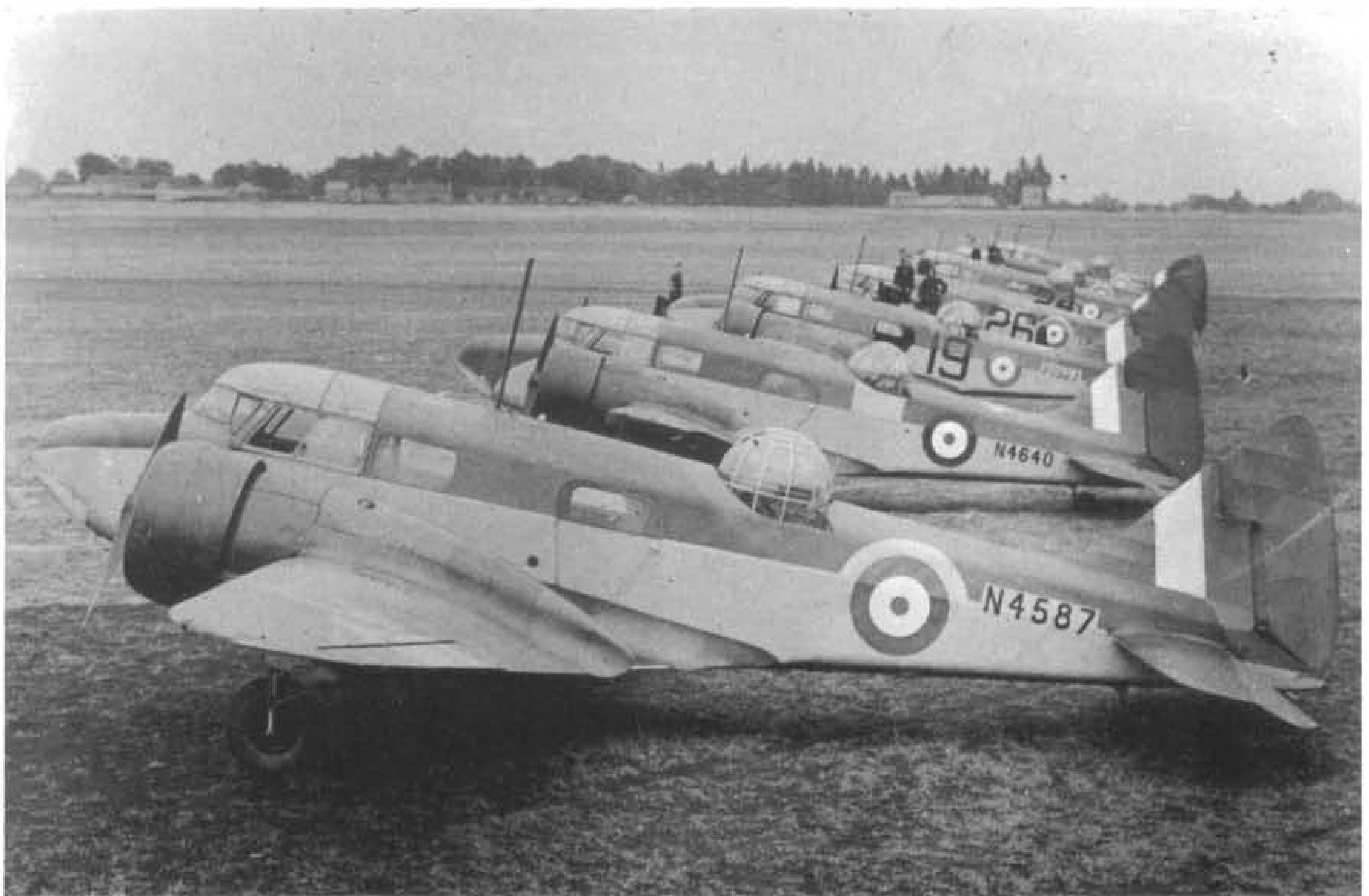
Morning line-up at Cranfield in the summer of 1940. One aircraft is turretless, others show variation in nose camouflage and have a coloured patch below the turret housing. The unit is No. 14 S.F.T.S. (Photo: I.W.M. CH1094)
