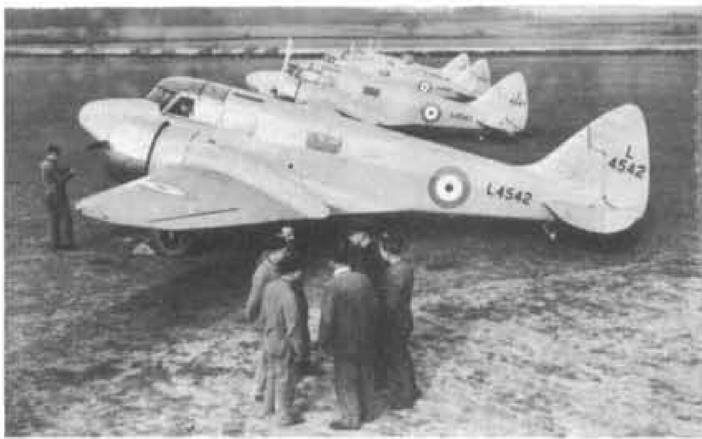
This early line-up outside the factory at Portsmouth was taken in March, 1938. The aircraft are painted yellow overall with natural metal cowlings and only the farthest aircraft, L4544, has a dorsal turret although they are all Mk. Is. (Photo: "Flight" 15455S)
