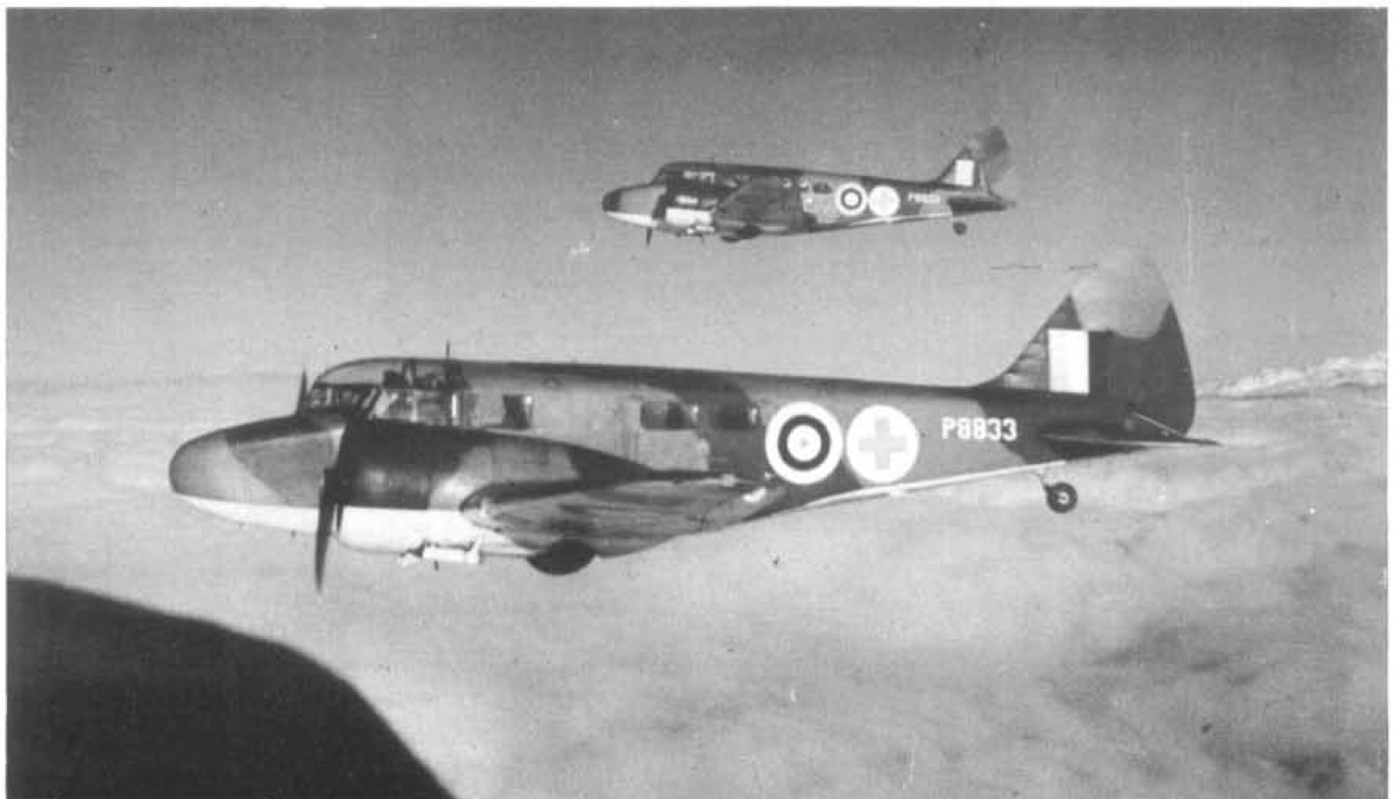
The two ambulance Oxfords, P8832 and P8833, flying from Portsmouth just before delivery. External differences were the larger freight-type doors with two windows.
