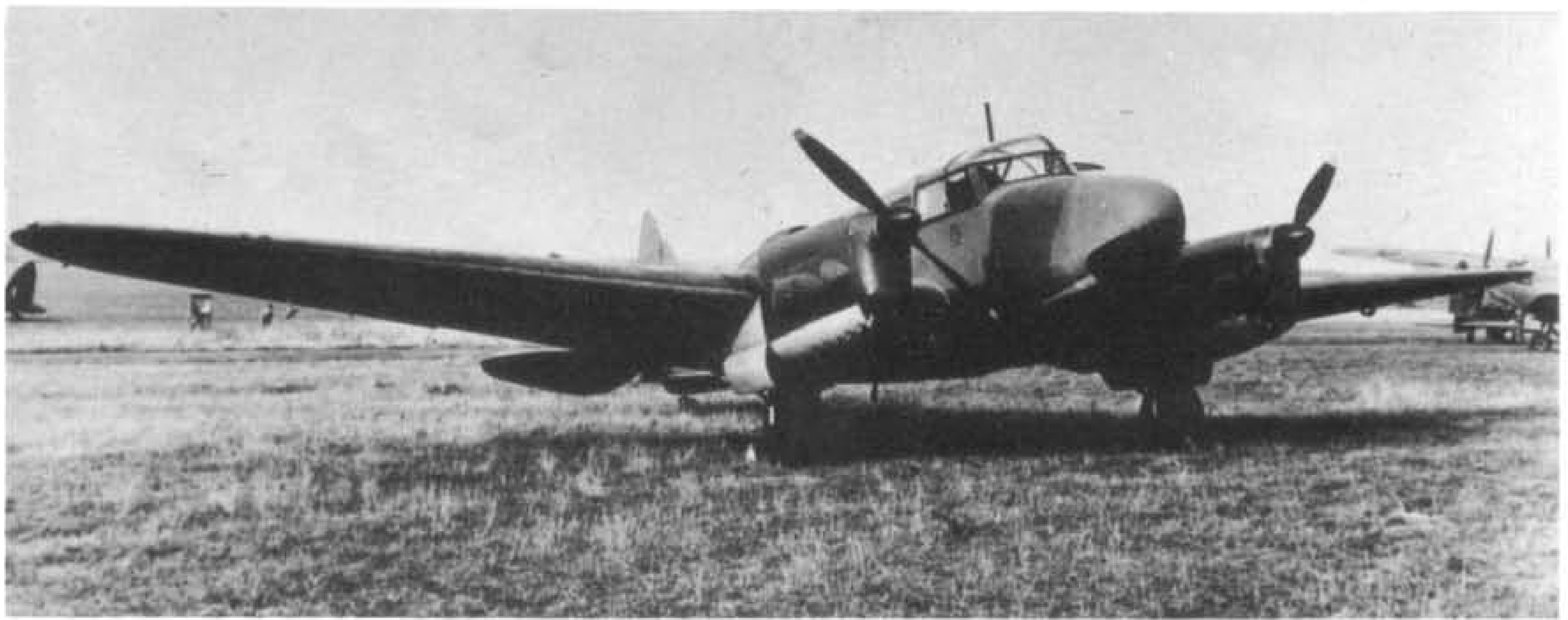
AS504 was the sole Oxford fitted with Gipsy Queen IV engines. This photograph is of interest in that, when it was released publicly during the war it "leaked" the Mosquito, whose tail can be seen under the starboard wingtip and which, at that time, was still secret.
