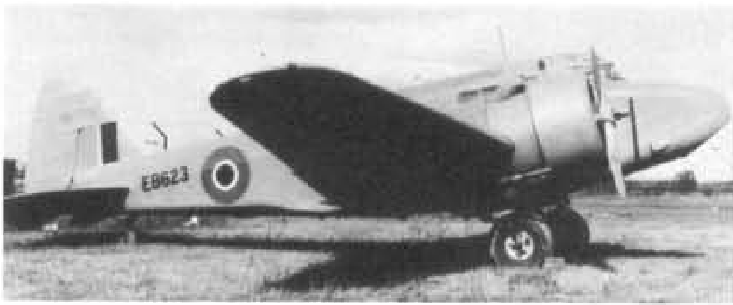
Most of the Oxford Vs were shipped overseas as airframes and fitted with Wasp Juniors in Canada. Here is one of them in Canada at the end of the War. (Photo: Howard Levy)
