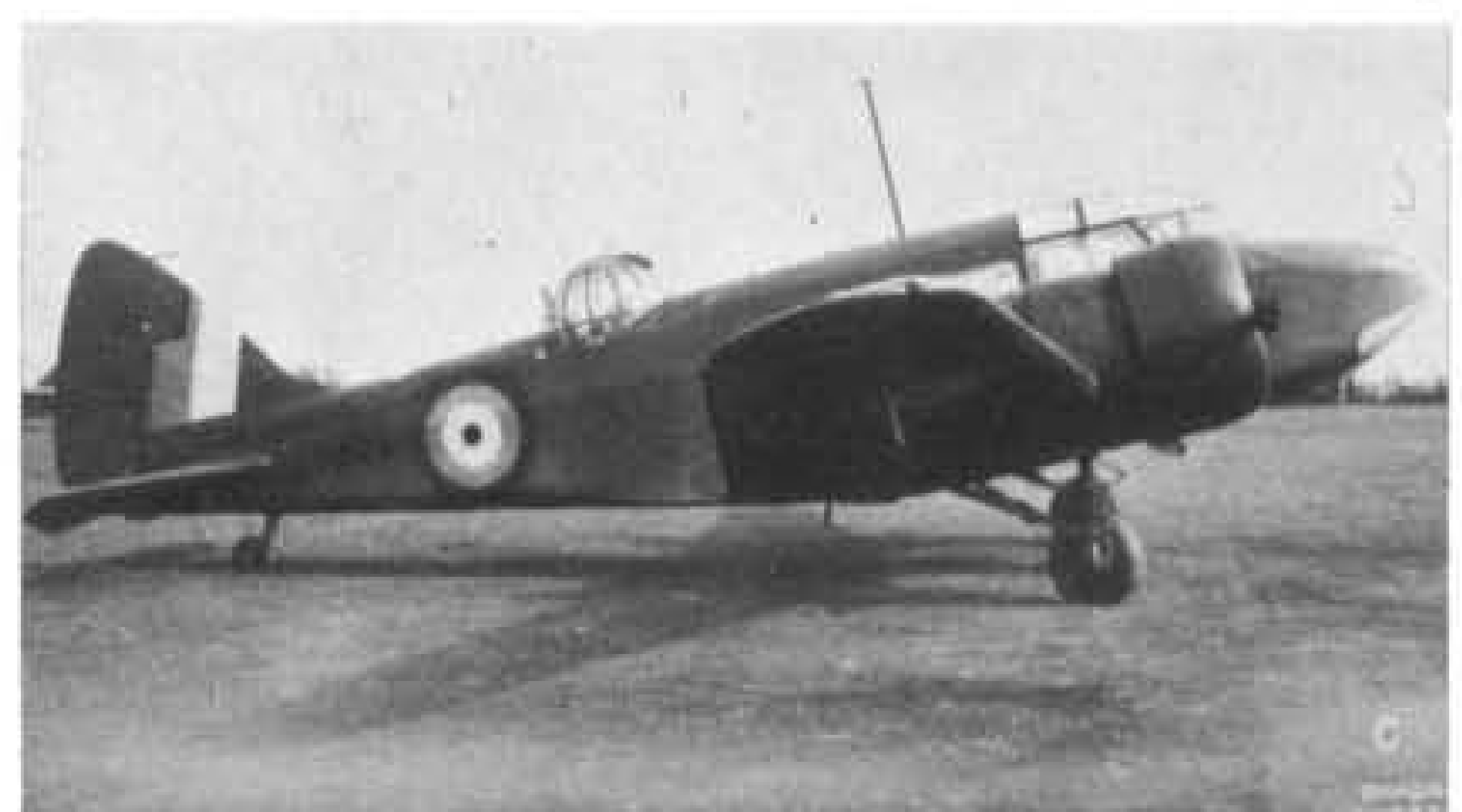
The fifth production Oxford I, L4539, was used by Heston Aircraft to test the Maclaren swivelling undercarriage for landing out of wind.
