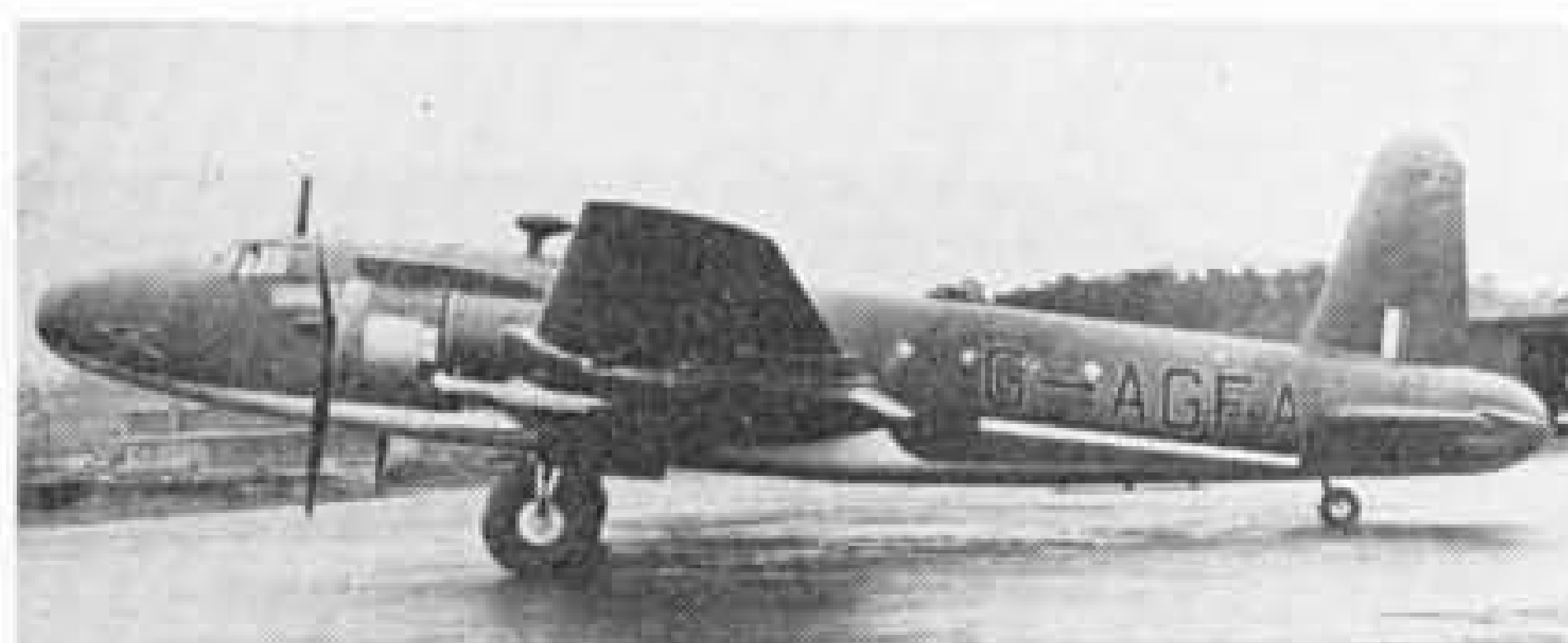
Fourth of the 14 Warwick C.Mk. Is of BOAC (G-AGFA, ex-BV246), at Brooklands in February 1943; showing to effect the passenger windows, exhaust-stack flame dampers and faired-over gun turret positions that characterized this conversion from the B.Mk. I bomber airframe.
