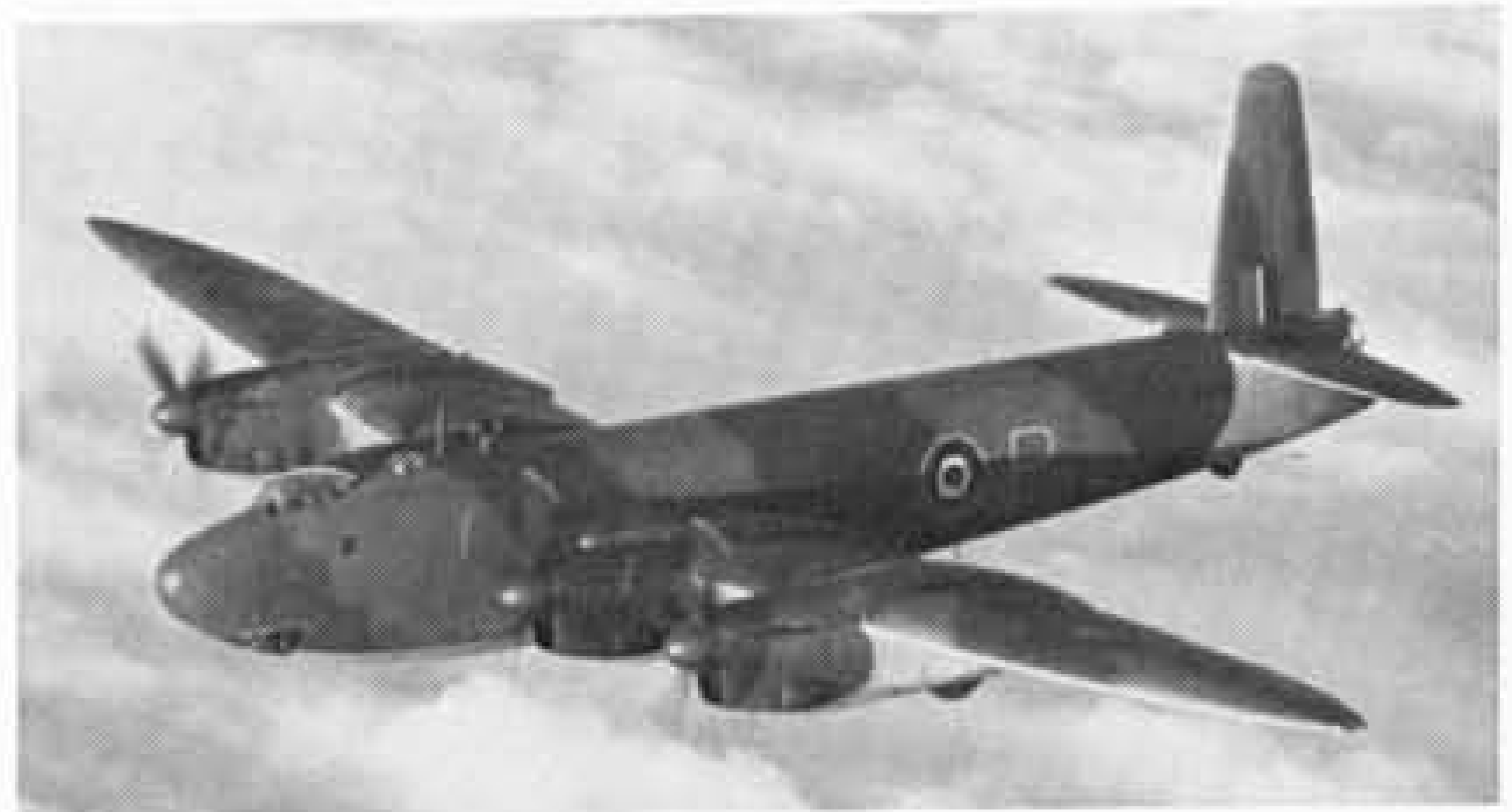
The original B.1/35 second prototype (L9704) seen airborne in 1944 during development of remotely-sighted armament for the Windsor—twin barbette guns in the rear of the engine nacelles and the sighting position replacing the tail gun turret.
