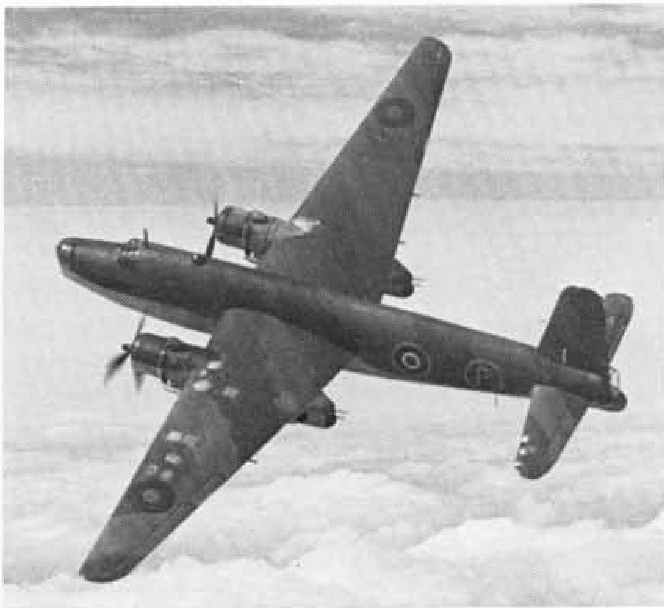
The original B.1/35 second prototype (L9704) seen airborne in 1944 during development of remotely-sighted armament for the Windsor—twin barbette guns in the rear of the engine nacelles and the sighting position replacing the tail gun turret.
