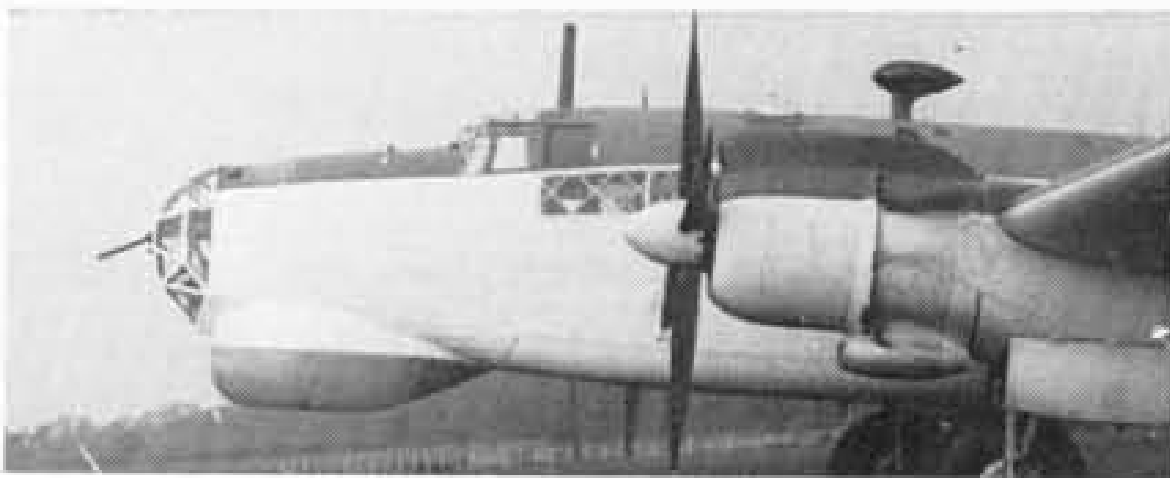
Details of the special ASV radar installation with 6-ft. diameter scanner mirror on Warwick ASR. Mk. V PN796 which was converted at Weybridge and delivered to T.R.E. (Telecommunications Research Establishment) Defford, on March 17, 1945. Note also the revised, multi-faceted, nose turret fitted to all general reconnaissance Warwicks (Mks. II and V).
