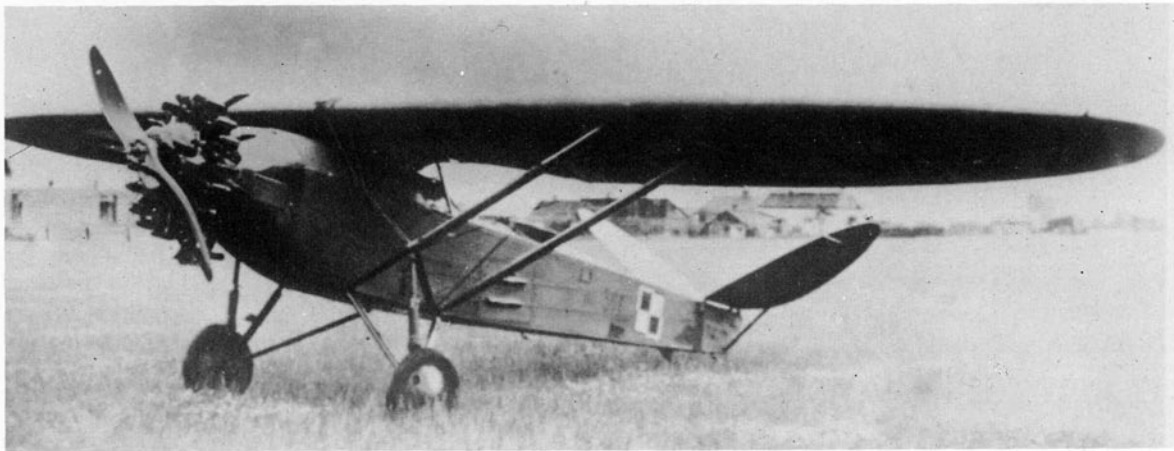
The original R-XIII prototype, c/n. 56.1, after the conversion to the R-XIX configuration, in the summer of 1932. The R-XIX was the world's second aircraft to fly with Rudlicki V-tail. (Photo: Jerzy S. Rudlicki)
