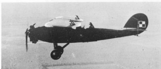
A military R-XIIIC V.I.P./liaison monoplane without a gun-ring installation in the second cockpit.
