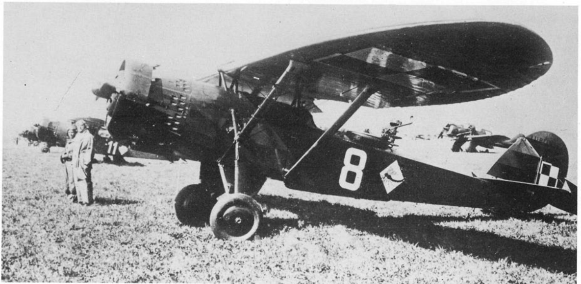
R-XIIIDs of No. 36 Observation Squadron of the 3rd Air Regiment, taking part in a military aviation display at Warsaw-Okecie airfield in the summer of 1938. A late production D, c/n. 56.150, with P.Z.L.-type wheels, is nearest to the camera.
