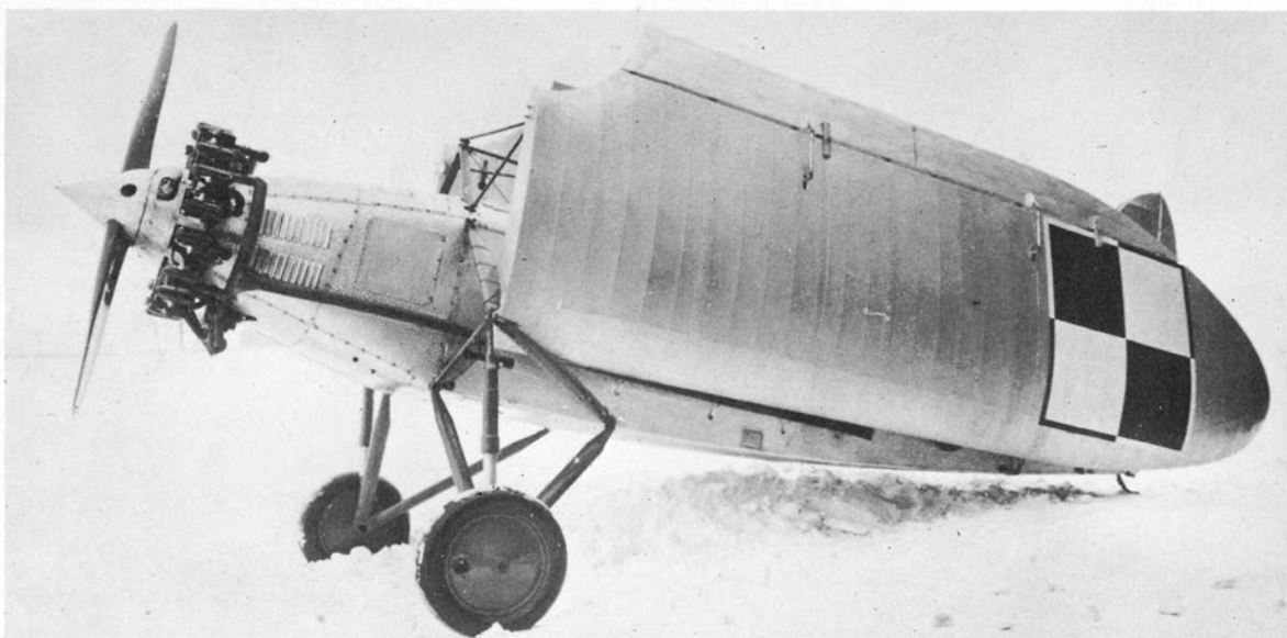
The first prototype Lublin R-X, c/n 52.1, soon after completion, with wing panels detached and tailplane and elevators folded up alongside the vertical tail surfaces, in which form the aircraft could be towed behind a car. (Photo: W. B. Klepacki)
