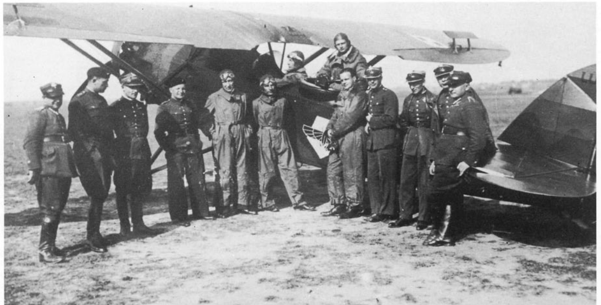
A hybrid R-XIIIC of No. 43 Observation Squadron, featuring a Townend ring engine cowling. The aircraft, call-number 52-T (which appeared on the wing undersurfaces), was otherwise similar to the standard C series and did not possess the head-plate cowling associated with the later D series model. (Photo: A. Glass)
