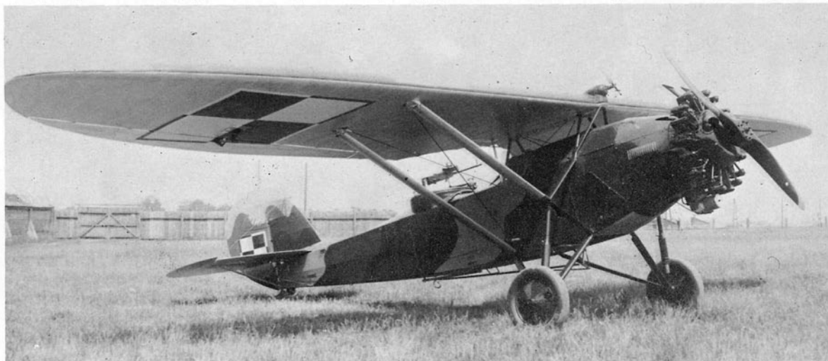
A newly completed R-XIIIB, equipped with a Lublin-produced R-2 gun-ring, before entering service with one of the observation platoons.
