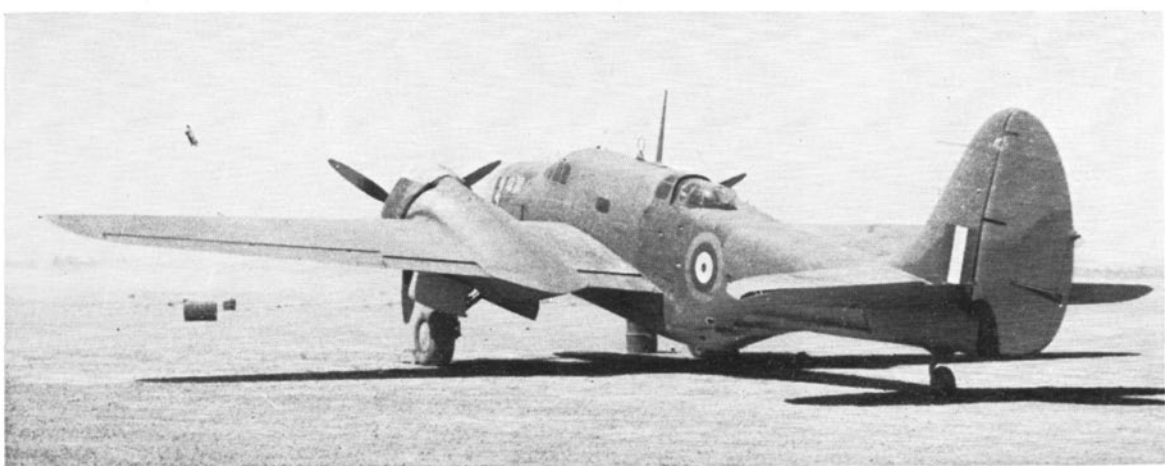
Long-range photo-reconnaissance Baltimore of No. 69 Squadron R.A.F., at Luqa, Malta, summer 1942. The aircraft is either a Mark I or II; note lack of powered dorsal turret. (Photo: via R. C. Jones)
