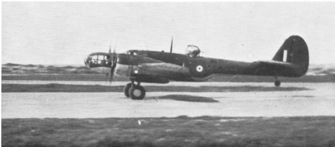
The first R.A.F. unit to operate Marylands was No. 431 Flight at Luqa, Malta. Here is one of the Flight's aircraft, believed to be AH261, during its take-off run. Like several of the initial Marylands to be received, this one is equipped with an Armstrong Whitworth manually-operated dorsal turret. (Photo: Newton via R. C. Jones)
