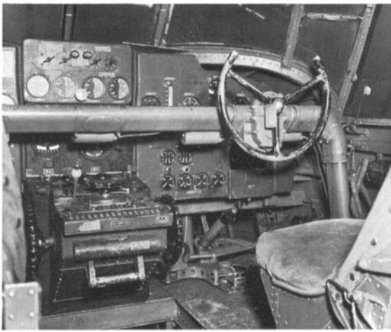
A close-up of the right-hand pilot's seat on the H8K2. (Photo: U.S. Navy via Major Robert C. Mikesh)
