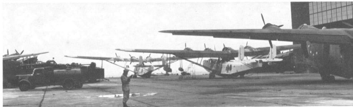
A mixed group of H6K2-L and H8K2-L Transport Flying Boats found on the Dai Nippon Koku slipway at Yokohama in September 1945 by the U.S. Forces. The H8K2-L in the foreground is minus its inboard propeller and wingtip float. The two H6K2-Ls are painted with white surrender markings on the rear hull only, with green surrender crosses on the hull and superimposed on the upper wing (Photo: U.S. Air Force via Major Robert C. Mikesh)
