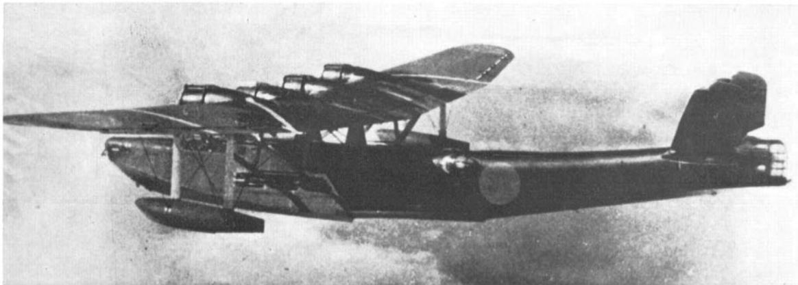
An H6K4 in flight with bombs attached to the wing support struts. The drab Pacific War colour scheme was introduced in mid-1942 for all combat aircraft of the IJNAF.
