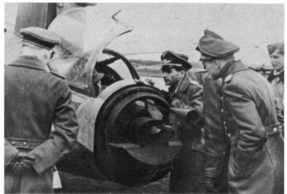
A further view of the rear gun position, showing the entry/escape hatch open; the 20-mm. cannon is not fitted. (Photo: Otto von Ballasko)
