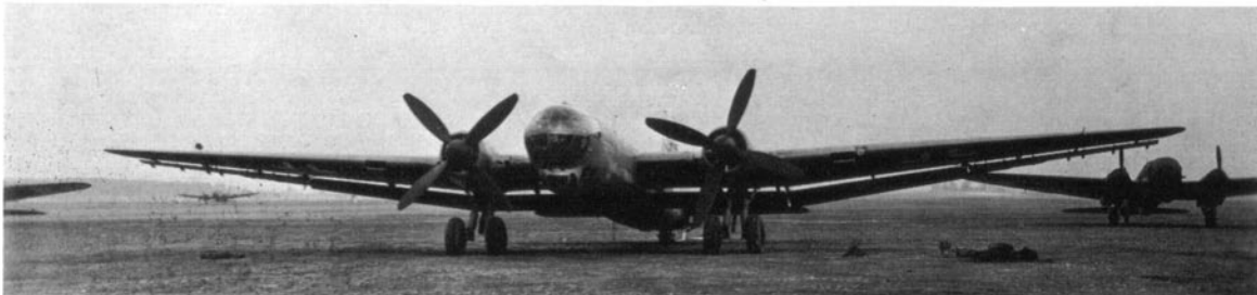
The second prototype of the He 177, pictured at the Heinkel works at Rostock-Marienehe. Note the full-span Fowler flaps, a feature of the early versions of this bomber. This example broke up in mid-air during diving tests. (Photo: via Edgar Petersen)
