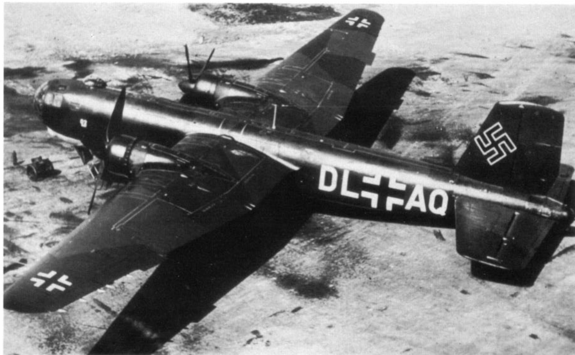
The second aircraft in the pre-production batch. Designated the He 177 A-0, this version featured a conventional gun turret immediately aft of the nose cabin. (Photo: Imperial War Museum HU 2861)
