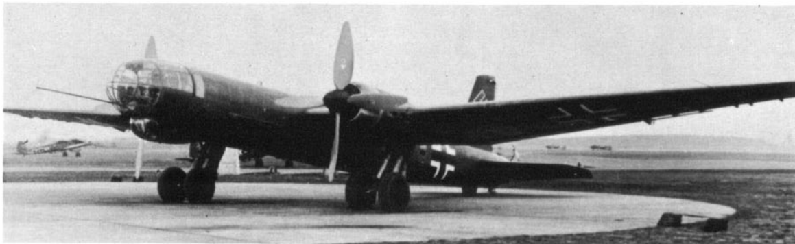
The first prototype of the He 177, which made its first flight on November 19, 1939; the flight lasted only twelve minutes, before test pilot Francke had to return with overheating engines. The problem of unsatisfactory engines was to remain with the He 177 throughout its life.
