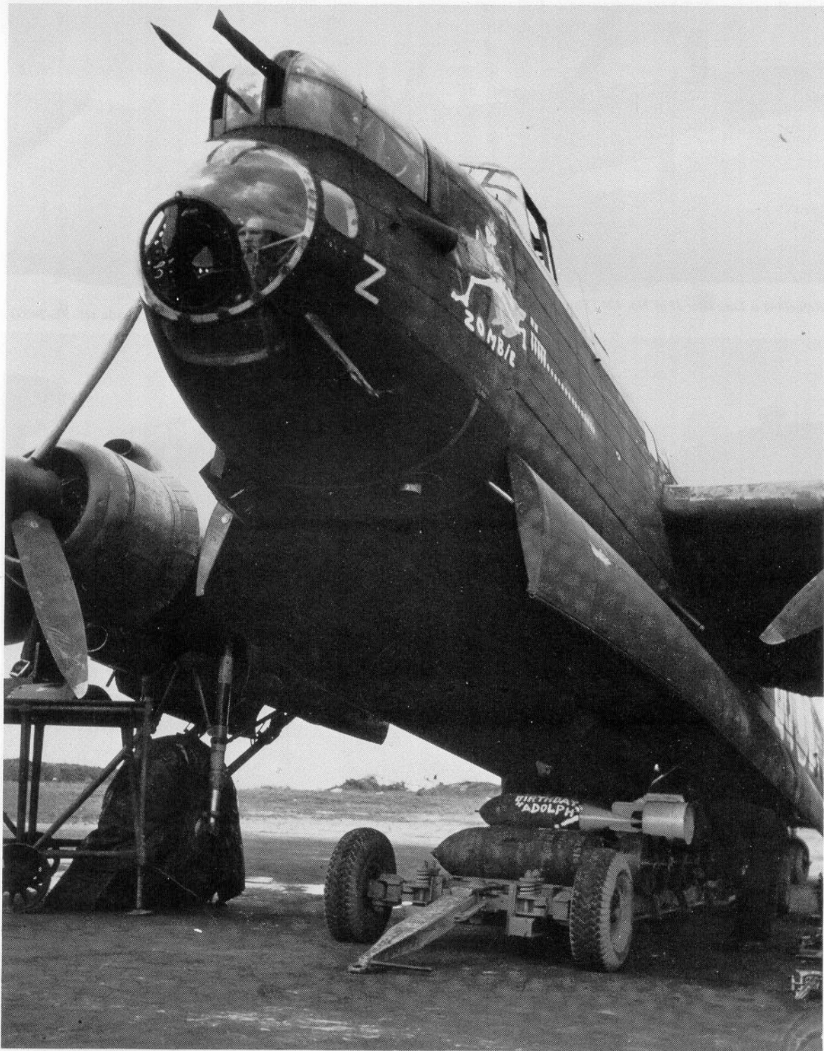
Another view of Zombie showing the bomb aimer's position and window with its circular glycol spray rig for de-icing, and further under, just in front of the bomb bay, the F-24 camera aperture can be seen. The louvre in front of the Zombie painting is the cabin heating outlet. In this case, the front guns have protective sleeves over the barrels. (Photo: Public Archives of Canada ref. PL-29072)
