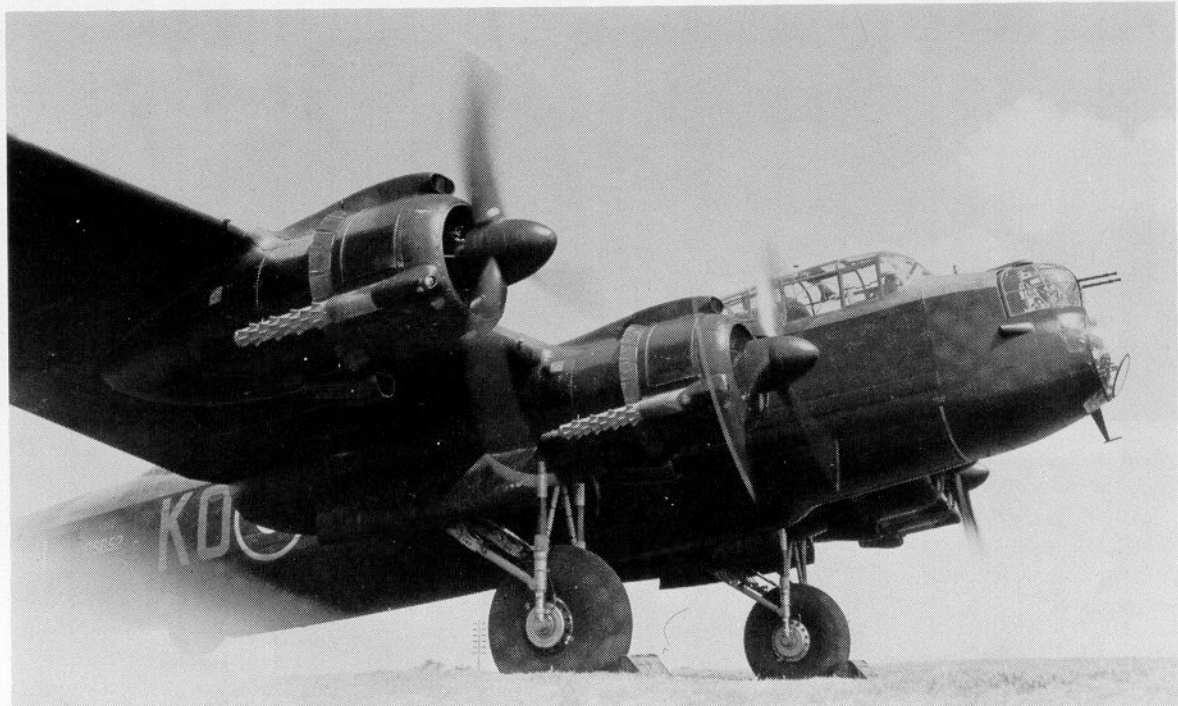
Lancaster II (DS652) of No. 115 Squadron, R.A.F., which was fated to crash near Udem, the night of June 12-13, 1943 while attacking Bochum. Two of the eight cable cutters fitted to each wing can be clearly seen in this photograph protruding from their inset containers. (Photo: Imperial War Museum ref. CH19792)
