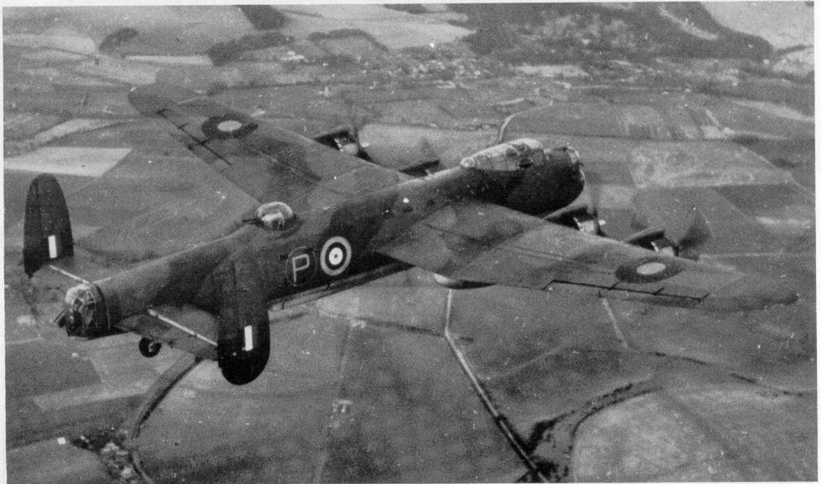
The Mark II prototype (DT810) after modification with bulged bomb doors. Most of its flying life took place at A. & A.E.E., Boscombe Down; being employed on performance trials, flame damping and fuel system trials, before being scrapped in April 1944. (Photo: A. & A.E.E., Crown copyright)
