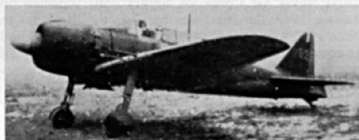
A rarely illustrated aspect of the Zero-Sen, Model 52—with undercarriage and flaps 'down'. This bare-metal A6M5 has the marking TAIC on the fin but the individual number is hidden by the starboard wingtip. (Photo: Koku Fan)
