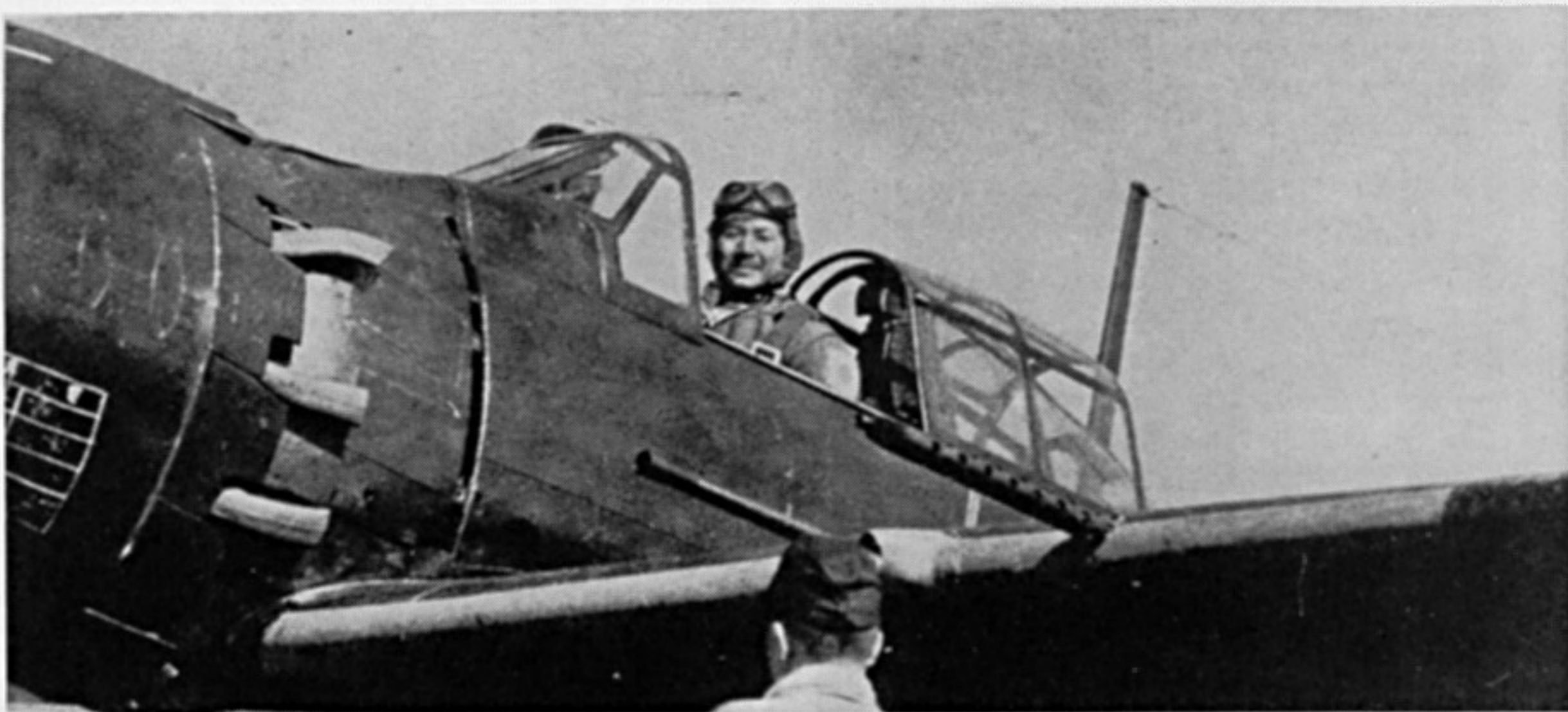
A striking close-up of a Zero-Sen, Model 52c (A6M5c) clearly illustrating the complex curves of the welded-steel exhaust stubs and cut-out gills of the Nakajima Sakae, Model 21 two-row radial. Behind the stencil-marked cowling can be seen the characteristic hump (embracing the windshield) which formerly housed two machine-guns. In the Model 52c, only one 13-mm. Type 3 heavy machine-gun was installed. But the wing armament was increased by two more heavy-calibre m-gs., each being situated outboard of the 20-mm. cannon.
