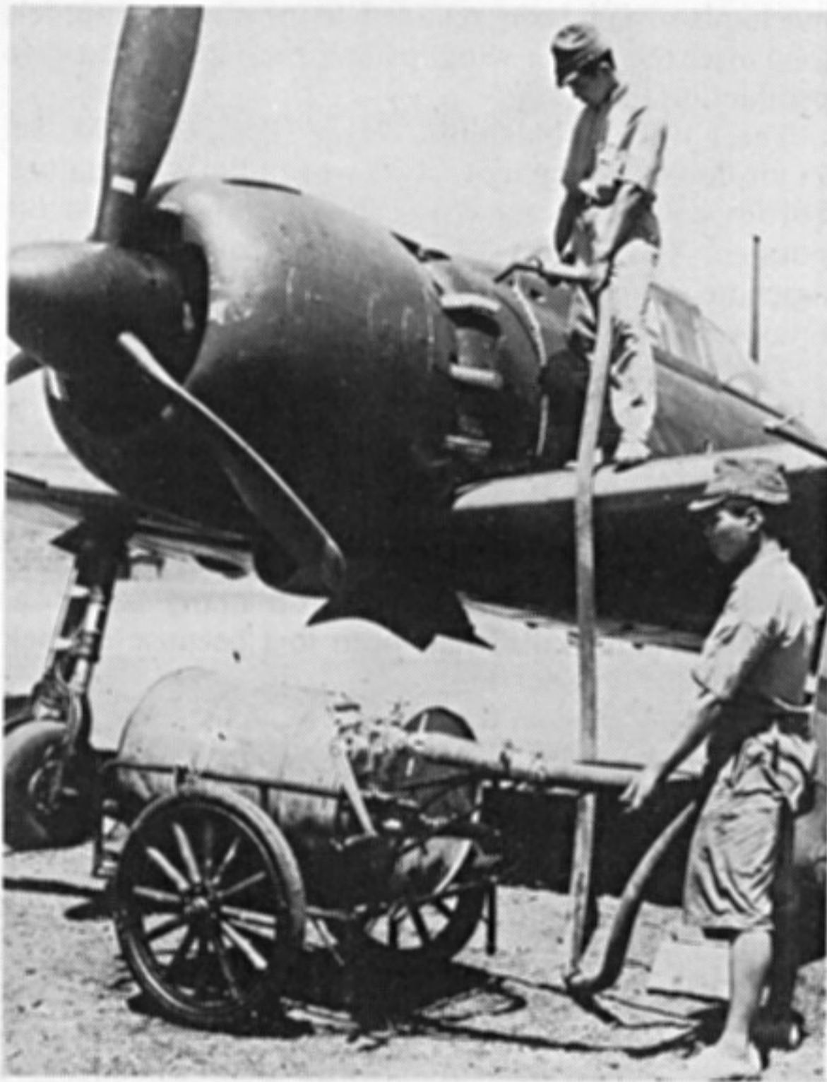
A crudely simple but effective 'in-the-field' mobile refueller for the Zero-Sen, Model 52. (Photo: US Navy Dept., National Archives, ref. 80-G-169292)
