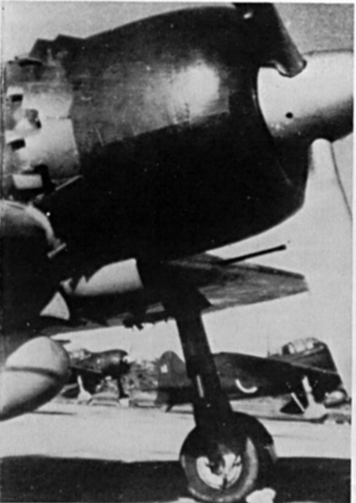
1. Cowling scoops, propeller and main undercarriage details show up well in this frontal view of a Zero-Sen, Model 52b. (Photo: Koku Fan)
