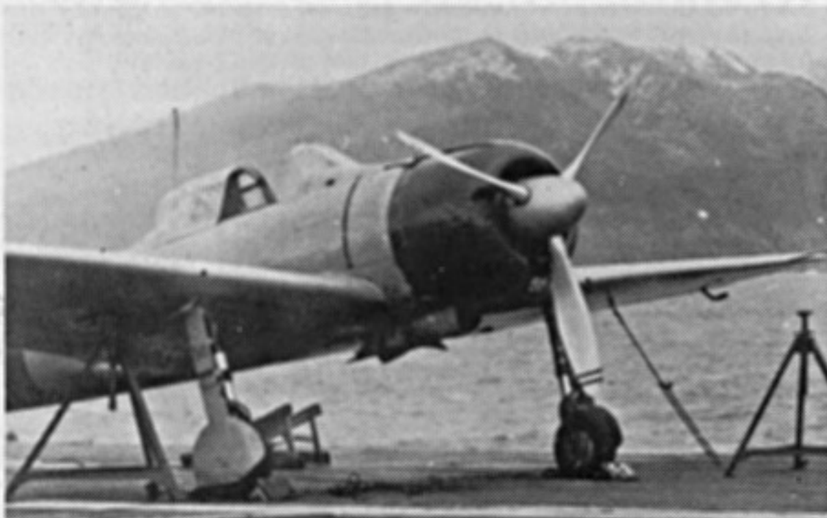
Study in refinement. (Left) The shape of 1941, just prior to the attack on Pearl Harbor. A Zero-Sen, Model 21 (A6M2) on the flight deck of IJN Akagi anchored in Hitokappu Bay, Japan. The ‘last-two’ of the aircraft’s number (in full, A1-158) appears both on the motor cowling ventral intake and on the main undercarriage covers. This early variant’s aileron mass balance is well in evidence. (Right) A Model 52c (A6M5c) in late 1944 shows the revised engine cowling, gills, exhaust stubs and the increased wing armament of two 20-mm. cannon and two (outboard) 13-mm. machine-guns. (Photos: via Takeshi Miyawaki)
