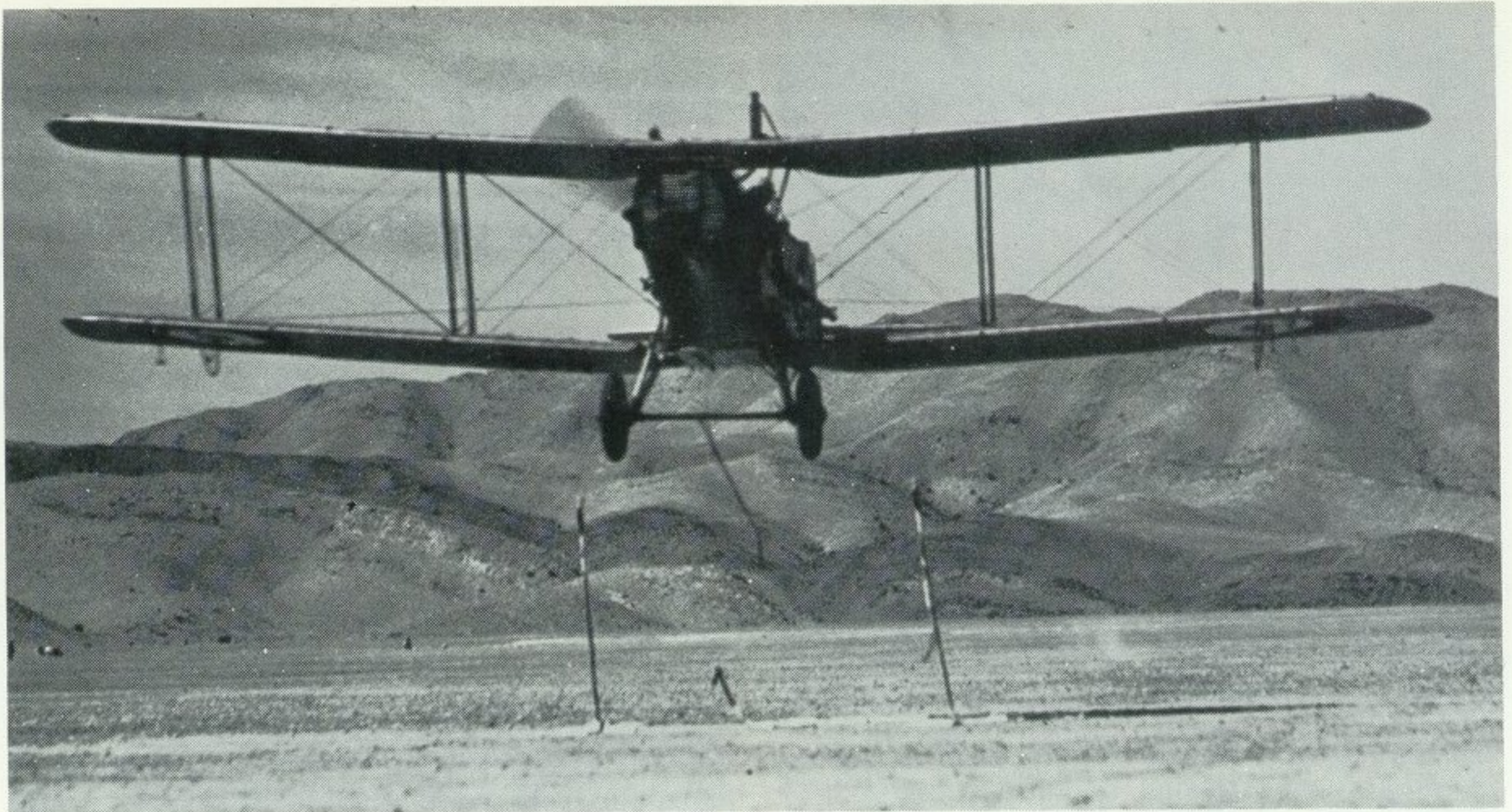
The "Hook-up" technique for retrieving ground messages. An F.2B about to collect a message, suspended between two poles, by use of the standard under-fuselage "hook"—a procedure which could prove highly dangerous for aircrews when attempted among the hills and mountains of India. (Photo: Ministry of Defence (Air))
