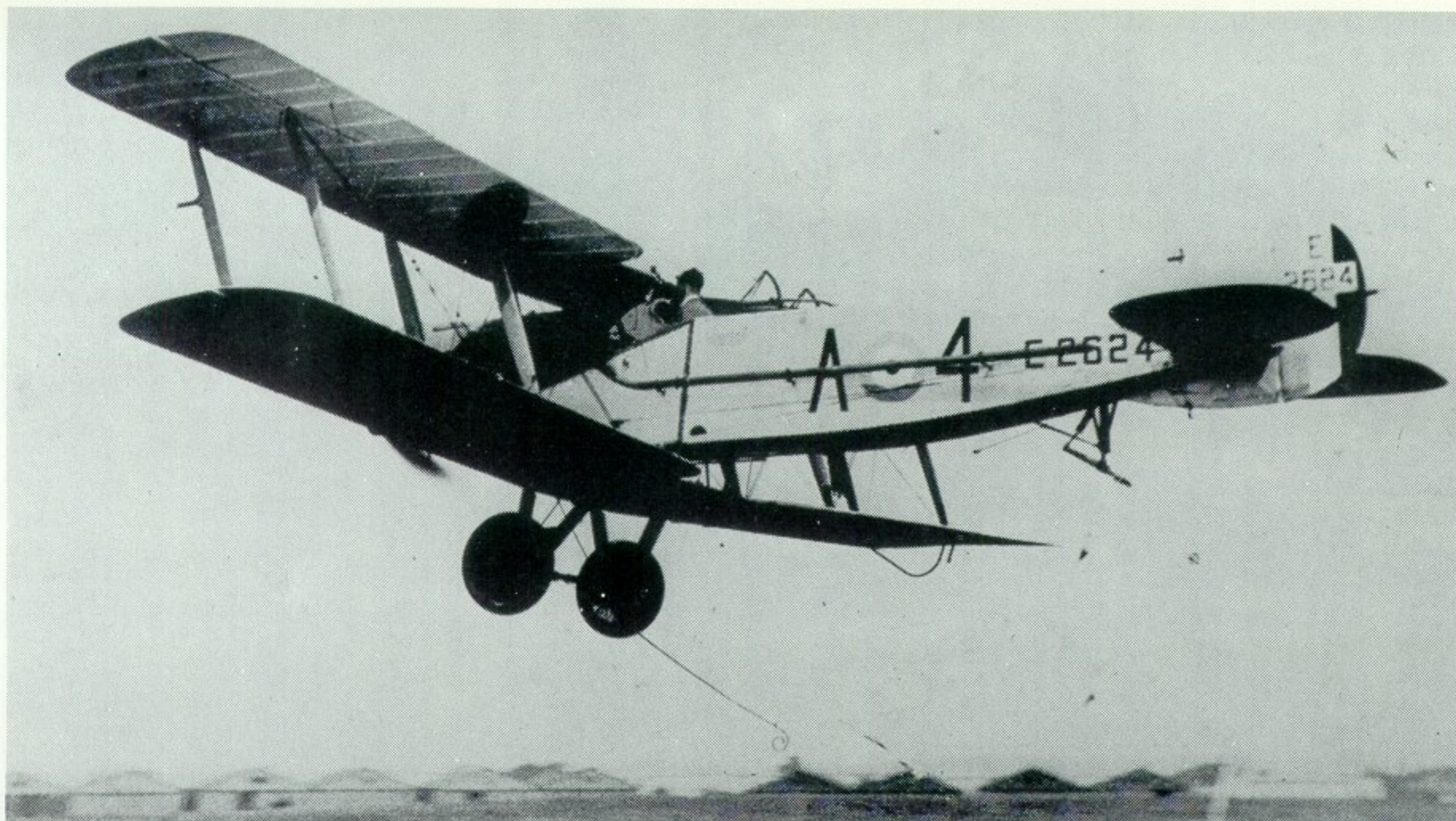
E2624, "4" of A Flight, No. 4 Squadron demonstrating the hook-up method of retrieving messages from the ground—the main procedure in use in the 1920s and early 1930s by all RAF Army Cooperation aircraft. (Photo: Author's Collection)
