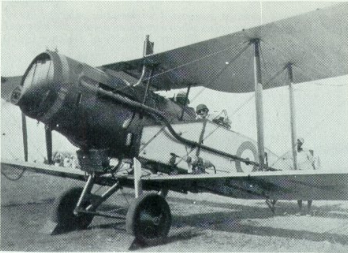
"A" of 28 Squadron preparing for take-off at Secunderabad India, on January 17, 1931. Of particular interest are the "desert" tyres, tropical radiator and upper wing centre-section cooling outlet piping. (Photo: courtesy No. 28 Squadron, RAF)
