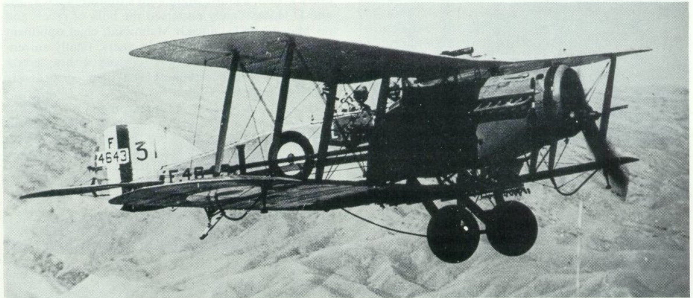
F4643, "J" of 31 Squadron, taken on June 1, 1928, in India. Protrusion showing above upper wing is "barrel" of a Hythe Camera-gun. (Photo: Author's Collection)
