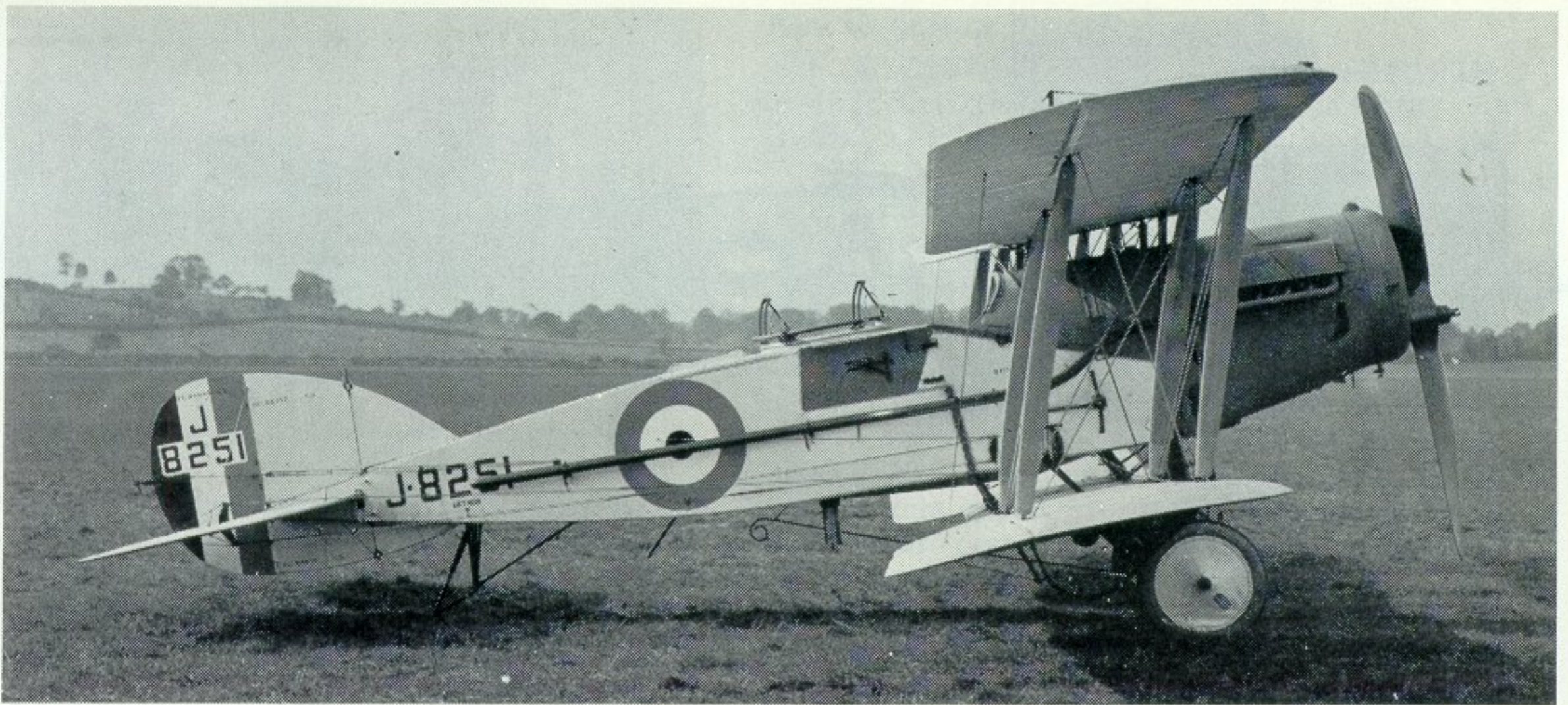
The first production Mk. III Bristol Fighter, J8251 (Type 96), fitted with Rolls-Royce Falcon III engine. Flight tests were flown on October 7, 1926. Clearly visible are under-fuselage pick-up hook and redesigned tail skid. (Photo: via C. H. Barnes)
