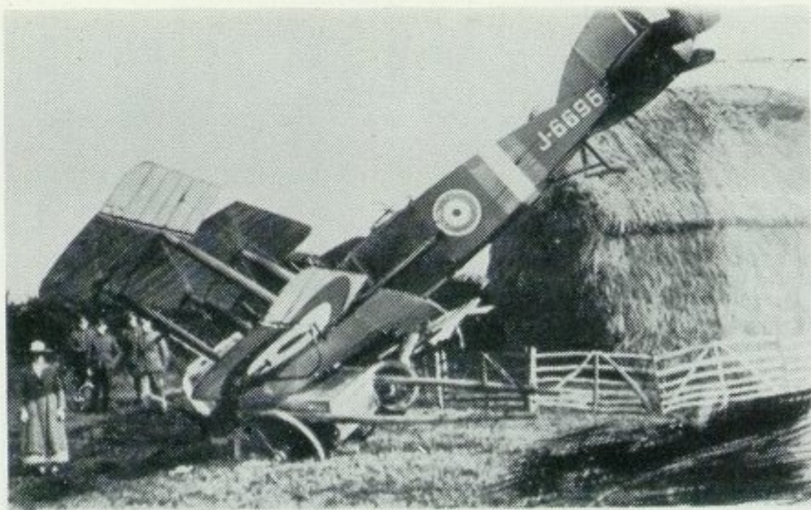
J6696 of A Flight No. 2 Squadron, which ran into a "farming machine" (sic). Of interest is the 1918 overall style of markings and 2 Squadron's unofficial squadron/flight insigne, comprising (here) two outer red bands and centre-band of white around rear fuselage. (Photo: P. M. Jarrett)
