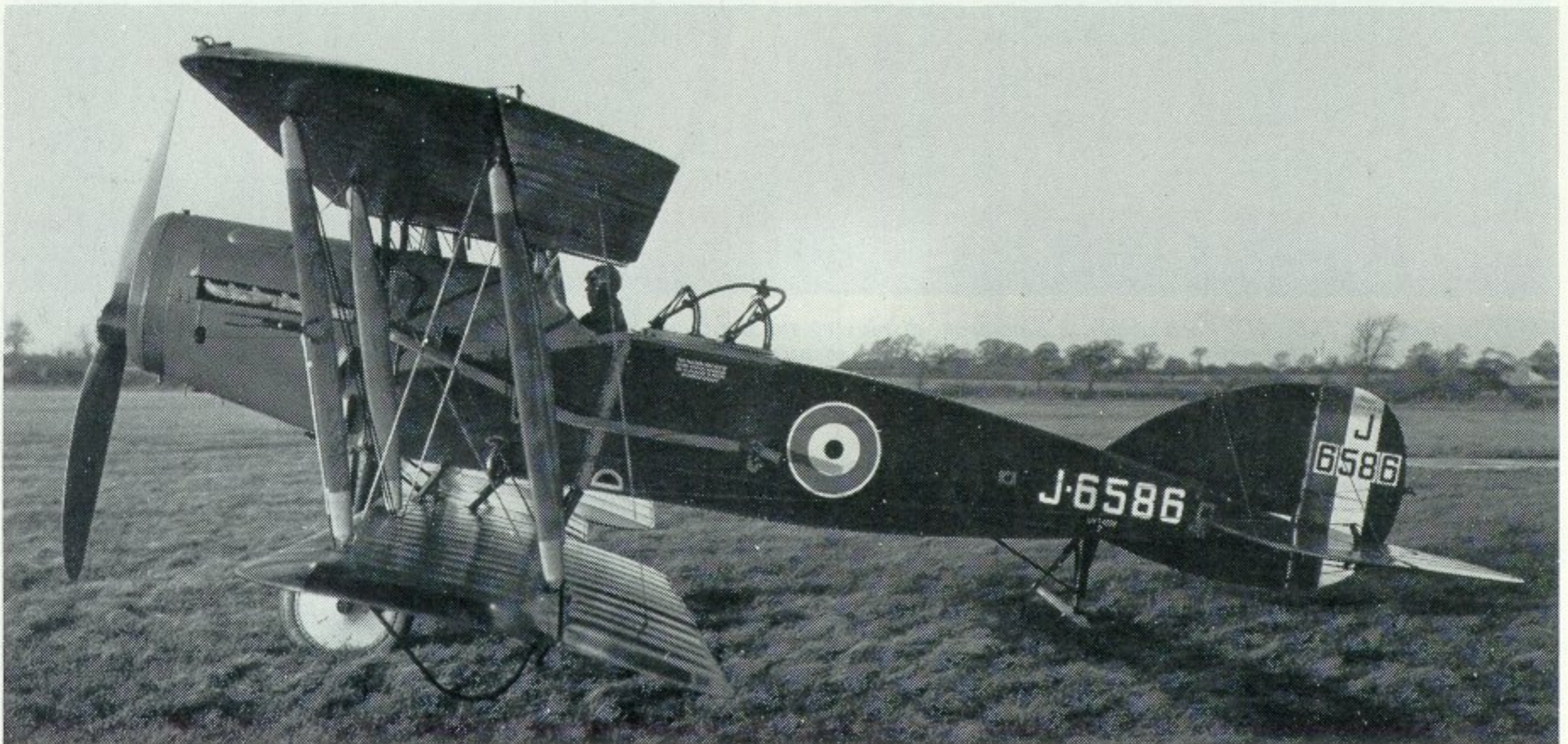
Two views of J6586 (Rolls-Royce Falcon III). This was the first of an eventual batch of 215 F.2Bs (J6587-J6800), built to a new, post-1918 contract. J6586 was widely tested with a range of desert equipment—including tropical cooling system—for use in India and Iraq, 1921. (Photos: via C. H. Barnes)
