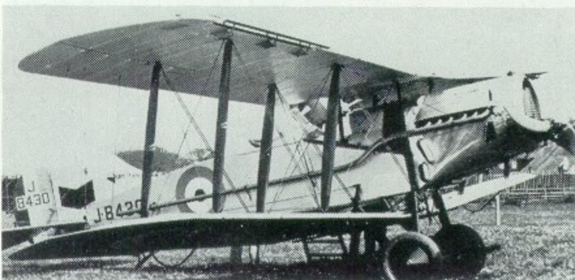
J8430 was the second F.2B built of a batch, J8429—J8458, specially converted to two-seat, dual control and completed between January and June 1927. This particular F.2B was further modified to include large rear cockpit windscreen and upper-wing auto-slots. Wheel covers were doped in red; while aircraft was brought onto the strength of No. 24 Squadron for maintenance purposes, as a personal transport for the use of Edward, H.R.H. The Prince of Wales, later H.M. King Edward VIII. (Photo: via C. H. Barnes)
