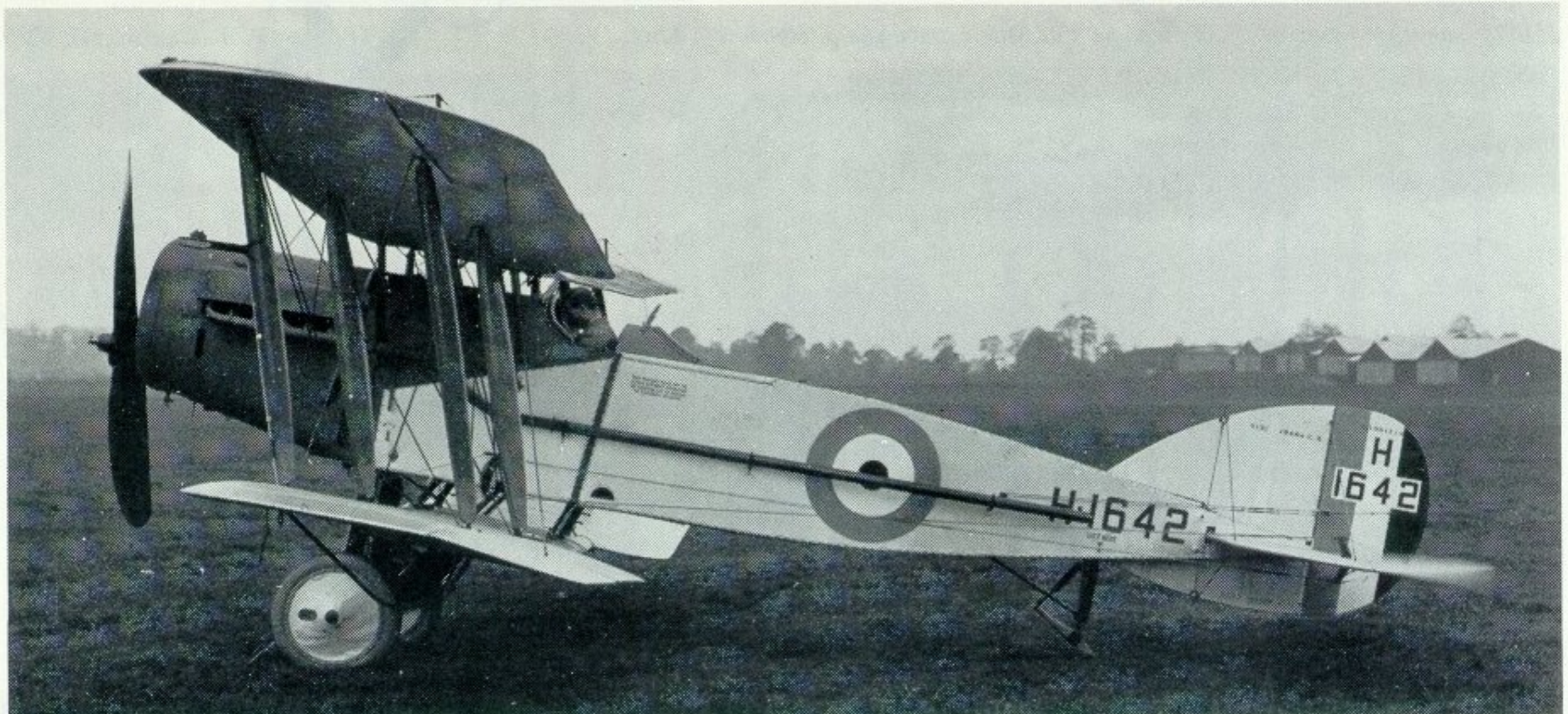
A straight-from-the-factory example of the dual control/seat version of the F.2B supplied to the RAF Cadet College, Cranwell in 1925. This particular aircraft (H1642) was reconditioned to "J" (or "Mk. II") standard in October 1925.
