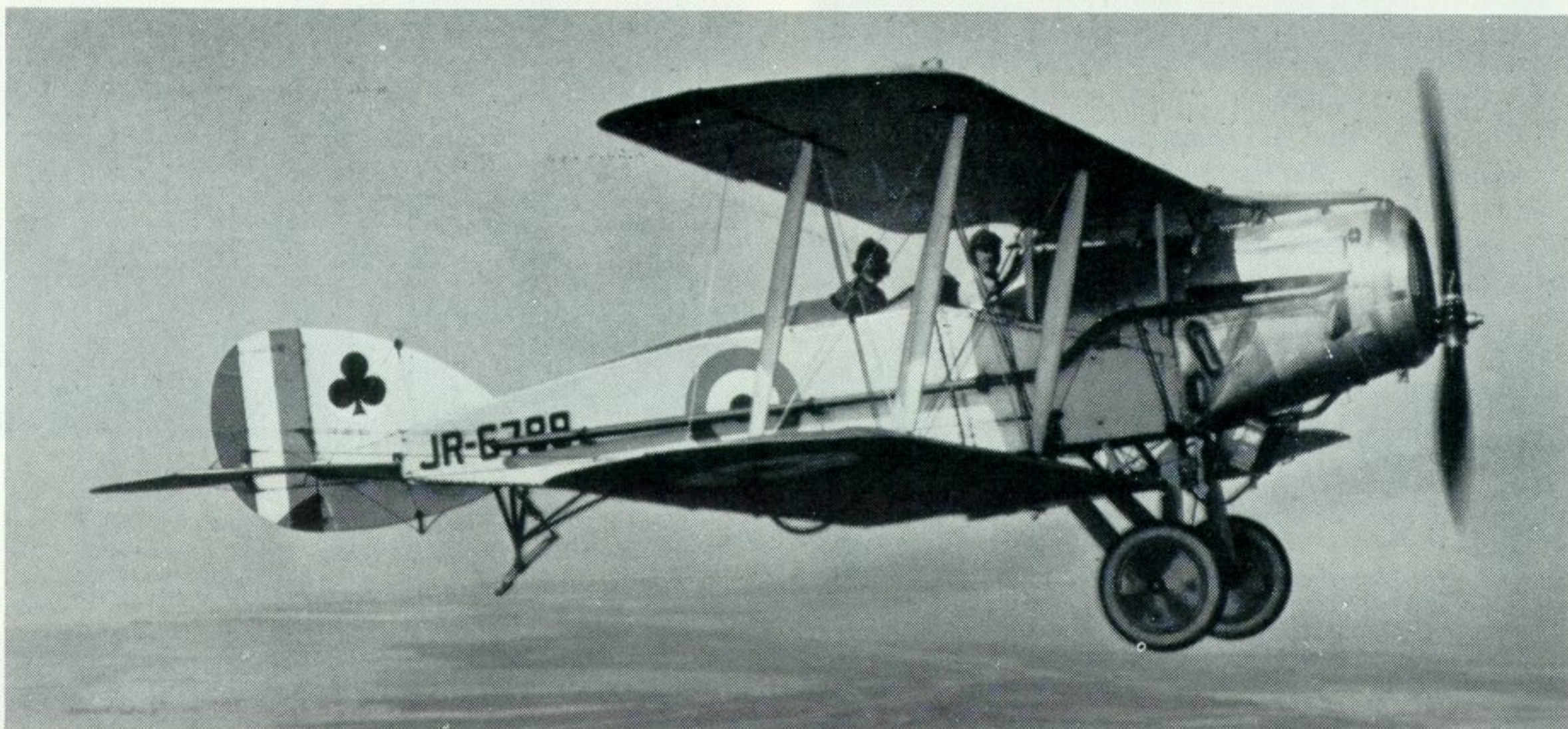
Rebuilt F.2B, JR6788 of 208 Squadron, flying over Suez Canal area. This particular aircraft has been locally modified by removing the gunner's Scarff ring and fairing over the rear fuselage, possibly for use as a unit "hack" communication vehicle. The Flight markings of a black "Club" on a white circle (denoting A Flt.) was doped on fin, upper centre section and under starboard lower wing. (Photo: Wing Commander J. H. Halliwell, OBE, RAF, Ret'd.)
