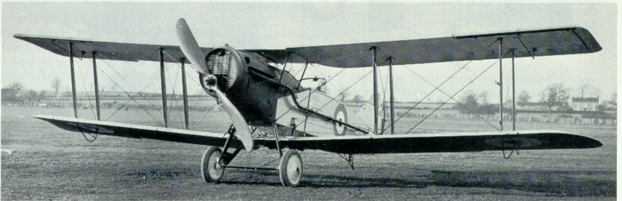
Type 96A, Mk. IIIA (H1417) in March, 1926. This F.2B became the prototype Mk. IV F.2B and had square-cut upper wing tips, due to convenience of affixing wing auto-slots (linked to ailerons). Originally converted to "Mk. II" standard on November 15, 1924; H1417 is seen here with the characteristic Mk. IV larger fin and horn-balanced rudder. (Photo: via C. H. Barnes)
