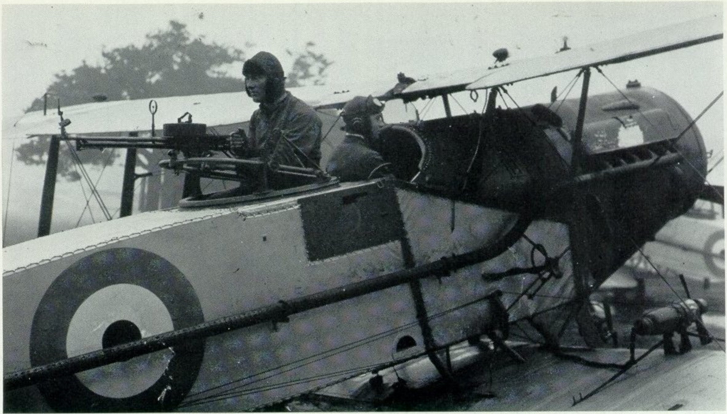
Back-to-Back—the classic fighting arrangement for the two-man crew of a Bristol Fighter.
