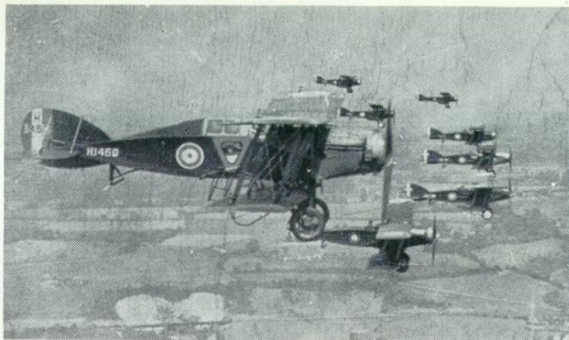
Another formation of 24 Squadron F.2Bs, July 1919. Nearest F.2B (H1460), was one of the first "Coupe" versions, converted for passenger transport and general communications. (Photo: J. M. Bruce/G. S. Leslie Collection)
