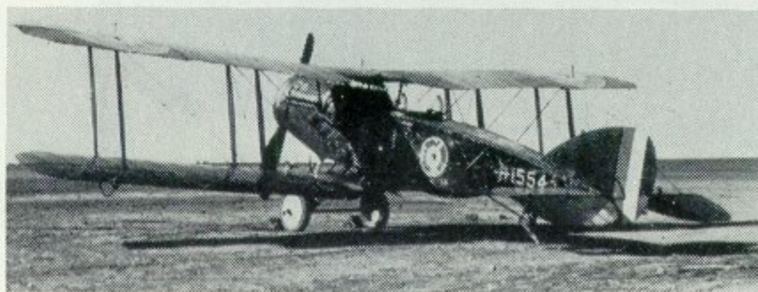
An early example of 28 Squadron's F.2Bs in 1921. H1554 shows graphically the effects of blistering sun and dust erosion on its fabric.
