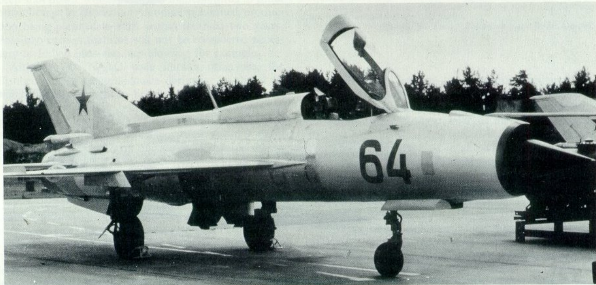
A Soviet Air Forces' MiG-21PFM (late-model "Fishbed-D") seen during a courtesy visit to Sweden during 1968. It features a new broad-chord vertical tail and relocated braking parachute, in an "acorn" fairing at the base of the fin, but differs from the "Fishbed-F" in retaining the forward-hinging cockpit canopy. (Photo: "Contact", Kokkedal, Denmark)
