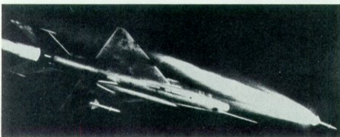
Night view of a "Fishbed-C" firing a K-13 missile (NATO: "Atoll"). The "Fishbed-C" is basically a fair-weather aircraft and much of the MiG-21's development since introduction to service has been aimed at improving its all-weather capability. (Photo: Soviet Official)
