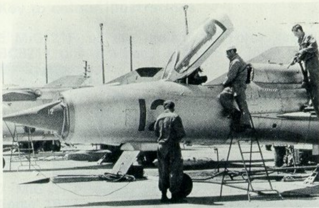
MiG-21PFs of the Soviet Air Forces being serviced on the flight-line. The crewman on the wing at the right may be refuelling the aircraft's auxiliary motor, which gives the aircraft self-starting capability. (Photo: M. Toda, "Koku-Fan")
