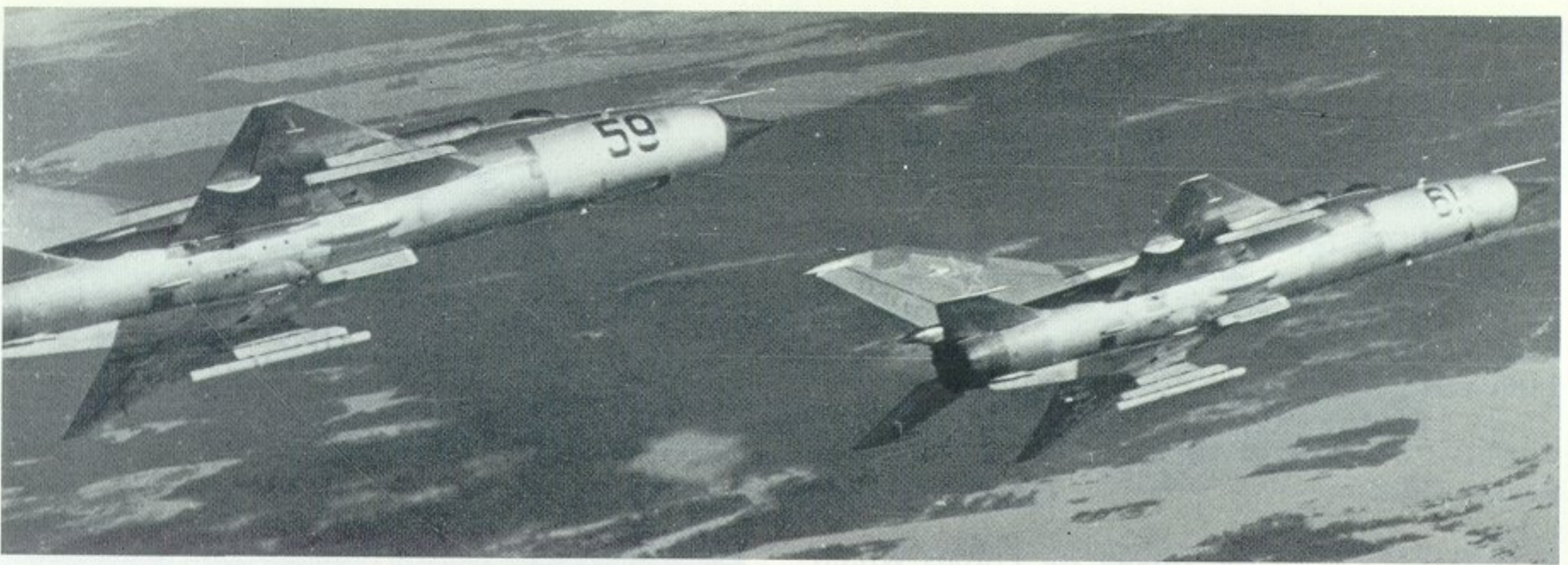
This "para" (pair) of late-model "Fishbed-D" interceptors shows to advantage the ventral and underwing stores' pylons. (Photo: Tass, November 1969, ref. 746773)
