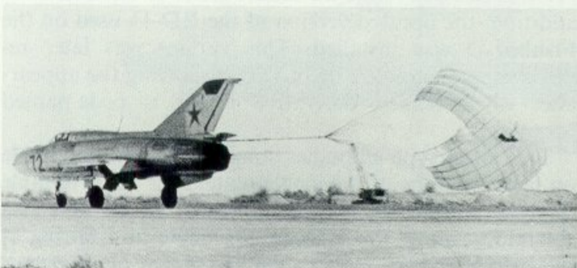
Soviet MiG-21PFMs—this time "Fishbed-F" aircraft—taking-off with jettisonable rocket-assist gear and landing with the aid of a later-type braking parachute. (Photos: Tass and M. Toda, "Koku-Fan")
