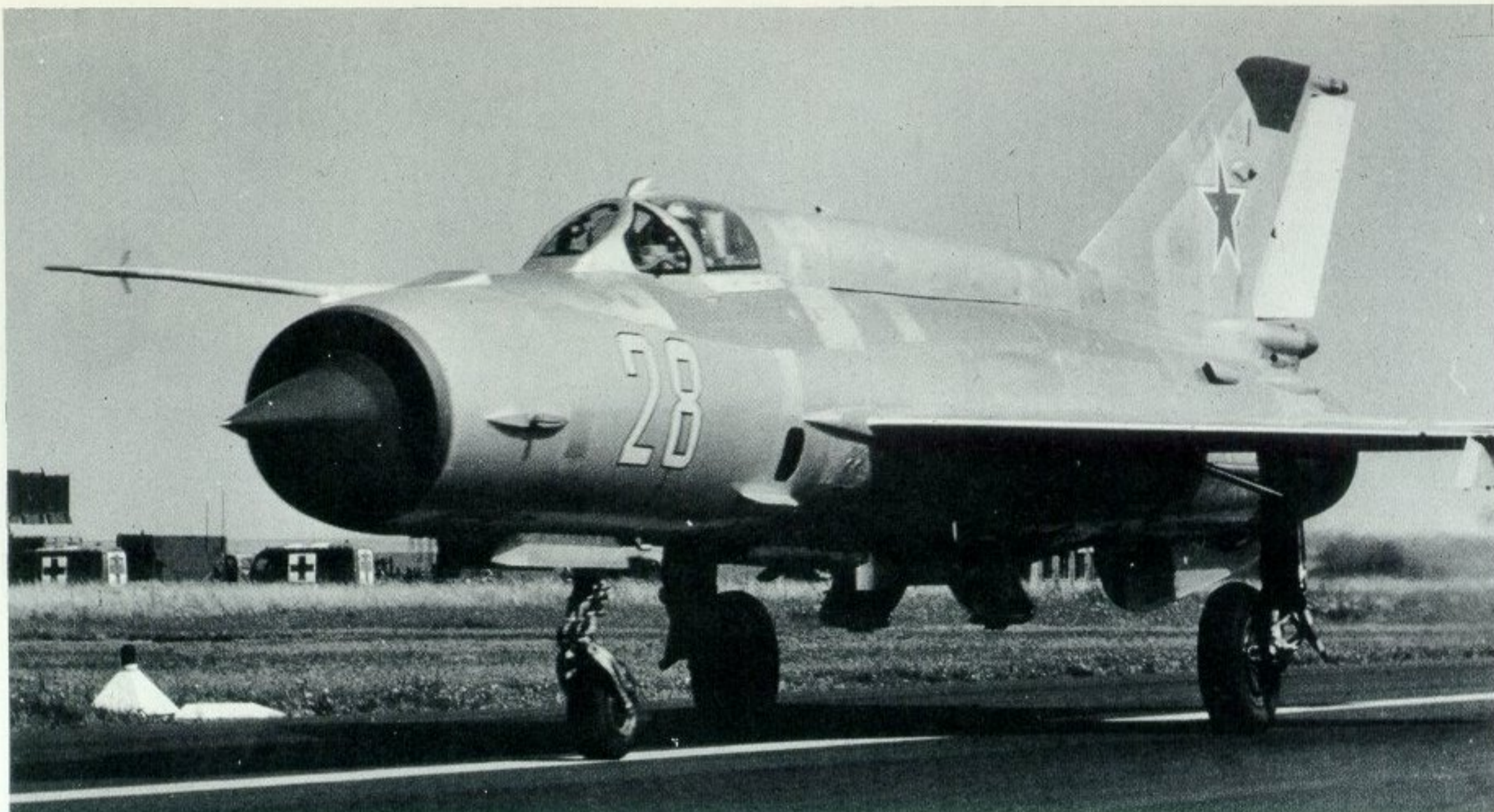
One of the Mig-21MF ("Fishbed-J") aircraft which visited Rheims in September 1971. This version has provision for two short-barrel 23-mm. cannon under the fuselage between the nosewheel and the ventral pylon. (In the photograph, they are below the suction-relief doors ahead of the wing.) Also noteworthy are the rear-view mirror and the deepened dorsal fairing aft of the cockpit. (Photo: SIRPA-Air, Paris, France, ref. 33184)
