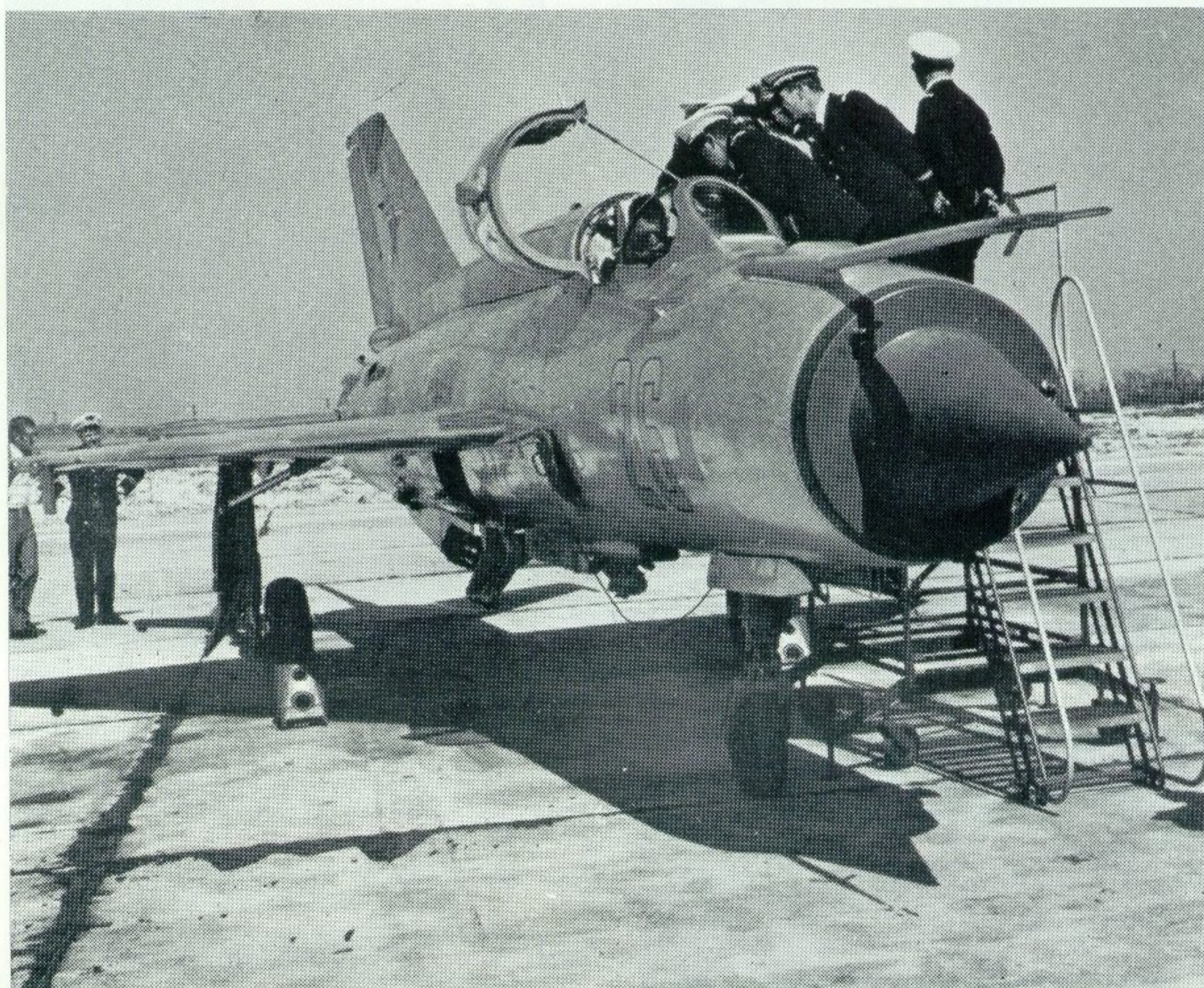
French Air Force personnel examining a MiG-21MF at Rheims; they commented favourably on the aircraft's general flying capabilities. The air intake blank and cockpit canopy prop are of note. (Photo: ECP-Armées, Fort d'Ivry, France, ref. F71360)
