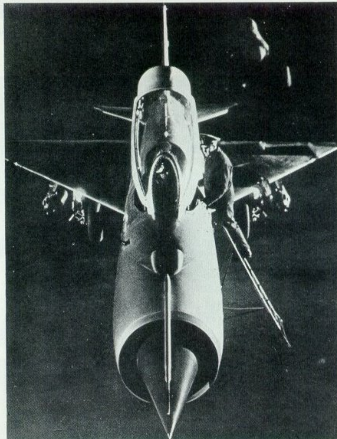
Two views of MiG-21PFMs ("Fishbed-D") in Soviet service, both carrying underwing UV-16-57 rocket pods (housing sixteen 57-mm. missiles). The landing view shows the deployed airbrakes and the nose-down attitude as the aircraft decelerates, while the night scene illustrates the cockpit access and servicing ladder.
