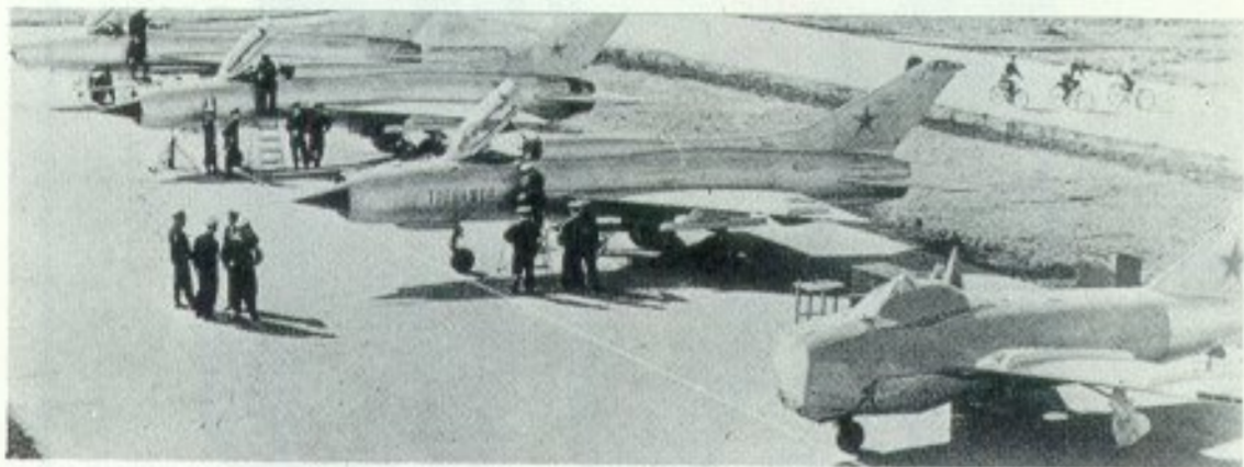
This incomplete but unusual view illustrates three MiG-21s and a MiG-17 lined-up at a Soviet airfield. The aircraft in the background is a MiG-21F ("Fishbed-C"), next to it is a late-model MiG-21PF ("Fishbed-D") with a broad-chord fin and rudder. The nearest MiG-21PF, with the inscription "Trenazher" (or Trainer) on the nose in Cyrillic characters, has an early-style narrow-chord fin and rudder.
