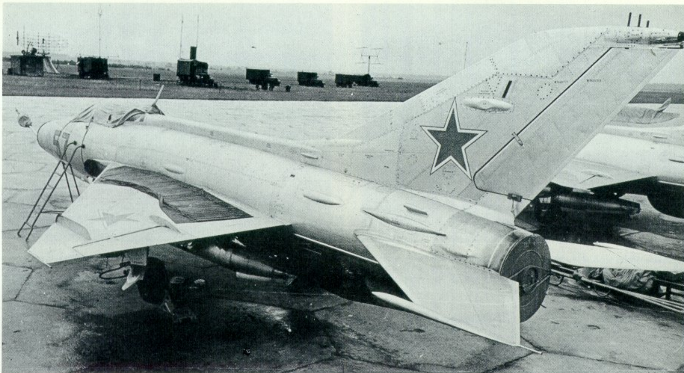
Superbly clear photograph of a MiG-21F covered-up for protection against the elements with canopy cover, exhaust blank and control locks. The airfield air traffic control and surveillance radar vehicles are noteworthy. (Photo: Tass, Moscow, USSR, November 1969, ref. 746772)
