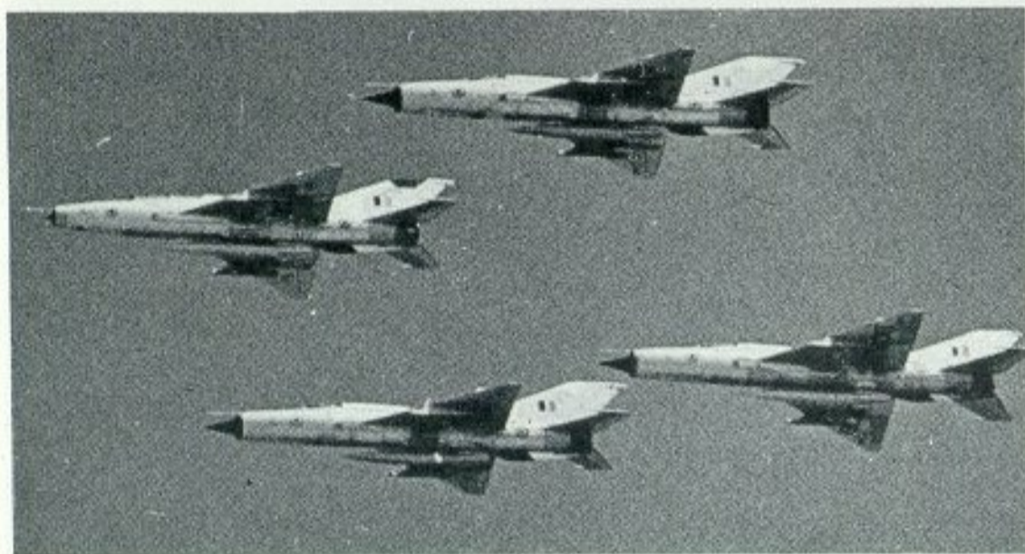
A formation of four MiG-21PFs of the Indian Air Force. This variant is built under licence by Hindustan Aeronautics and was active in the December 1971 conflict between India and Pakistan. To make up for this version's lack of built-in cannon armament, the Indians use a twin 23-mm. cannon gunpack which can be fitted in place of the ventral auxiliary tank. (Photo: Indian Official)
