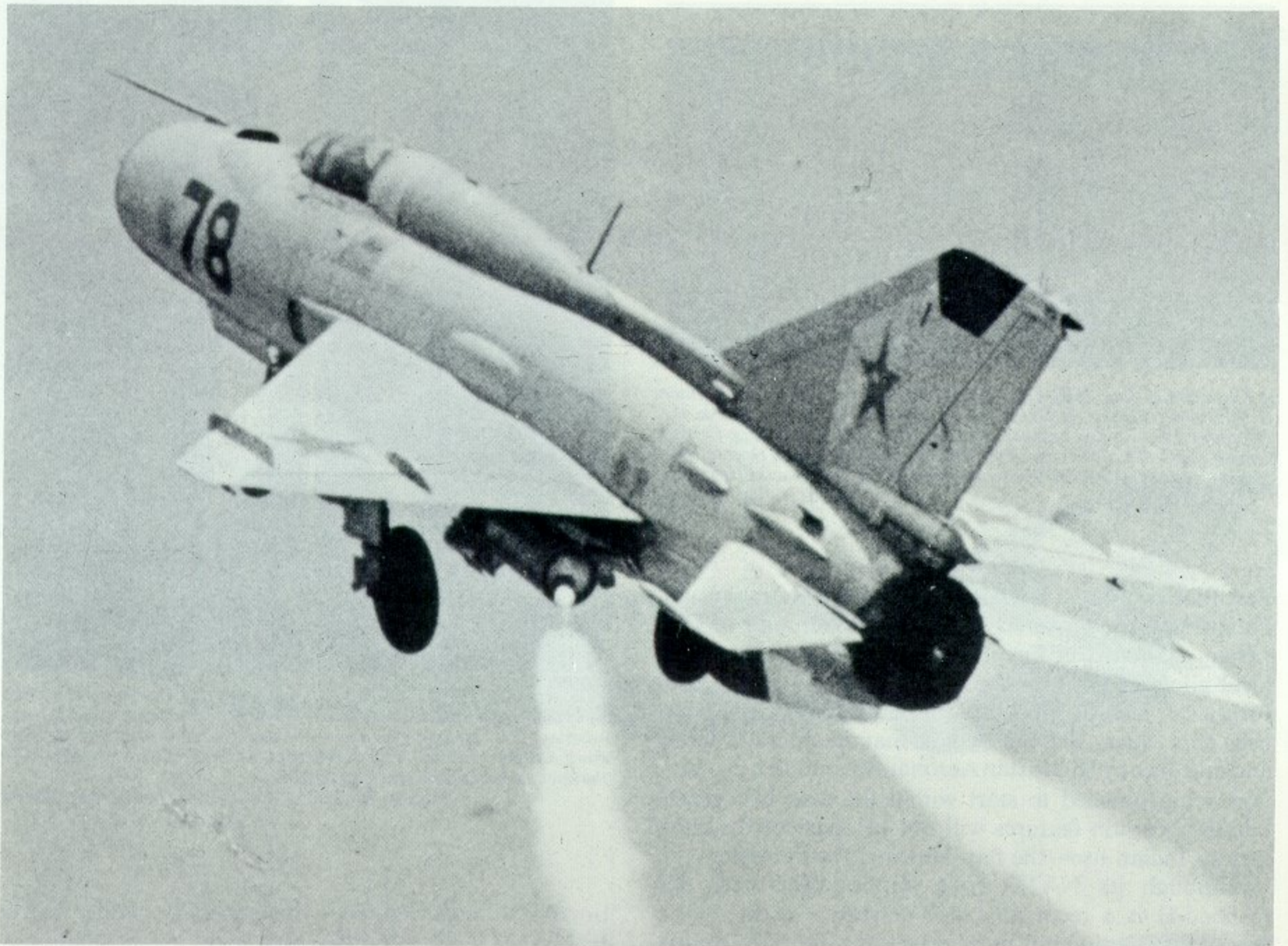
Soviet MiG-21PFMs—this time "Fishbed-F" aircraft—taking-off with jettisonable rocket-assist gear and landing with the aid of a later-type braking parachute. (Photos: Tass and M. Toda, "Koku-Fan")
