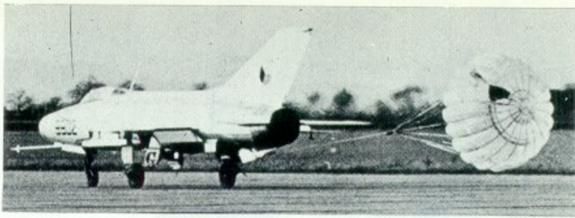
This view of a Czechoslovak Air Force MiG-21F shows it trailing its braking parachute. On this variant the chute is housed in the port rear fuselage (the open door is just aft of the port flap) and is streamed from the rear of the ventral fuselage fairing.
