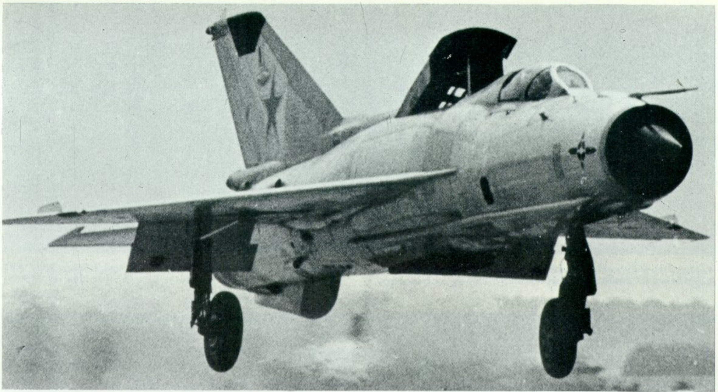
An experimental STOL version of the MiG-21 (NATO "Fishbed-G"), was demonstrated at the Soviet air display held at Moscow's Domodedovo Airport in July 1967. The main modification was the insertion of an extra fuselage section housing two lift engines. The main undercarriage was fixed, but the nosewheel was retractable to avoid stability problems. (Photo: Tass, March 1969, ref. 728084)
