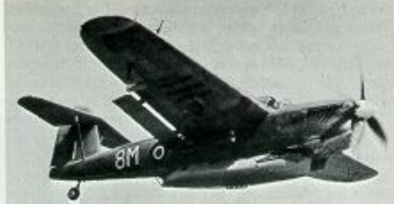
BV727, a Blackburn-built Barracuda II of the Naval Air-Sea Warfare Development Unit, seen during trials with the Airborne Lifeboat adapted for carriage by the Barracuda. The trials were entirely successful and the lifeboat was put into limited production, for carriage by either the Barracuda II or the Barracuda III. (Photo: Imperial War Museum, ref. A29658)
