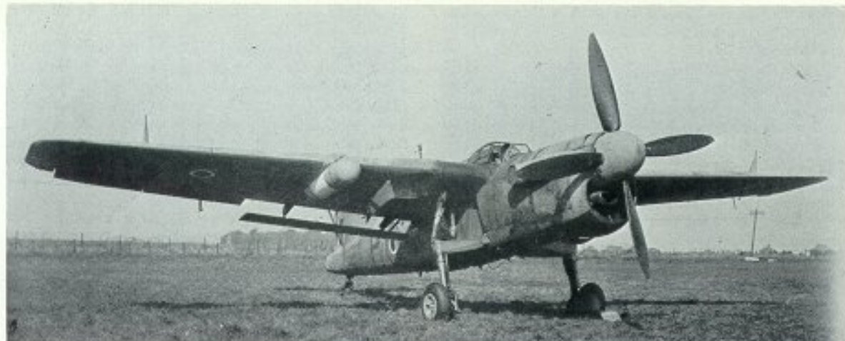
PM940, the first true Barracuda V prototype, with extended fin and wing-tips. The ASH radar nacelle was subsequently moved to the underside of the port wing. (Photo: Crown copyright, ref. 15205B)
