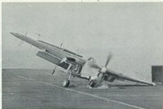
3A 767 Squadron Barracuda comes to grief during a deck-landing training session aboard the escort carrier Rajah, landing with too much sideways "drift" and causing the port oleo to collapse. The cloud of sawdust immediately in front of the aircraft has been thrown up from the wooden deck, under the impact of the propeller blades. (Photo: via author)
