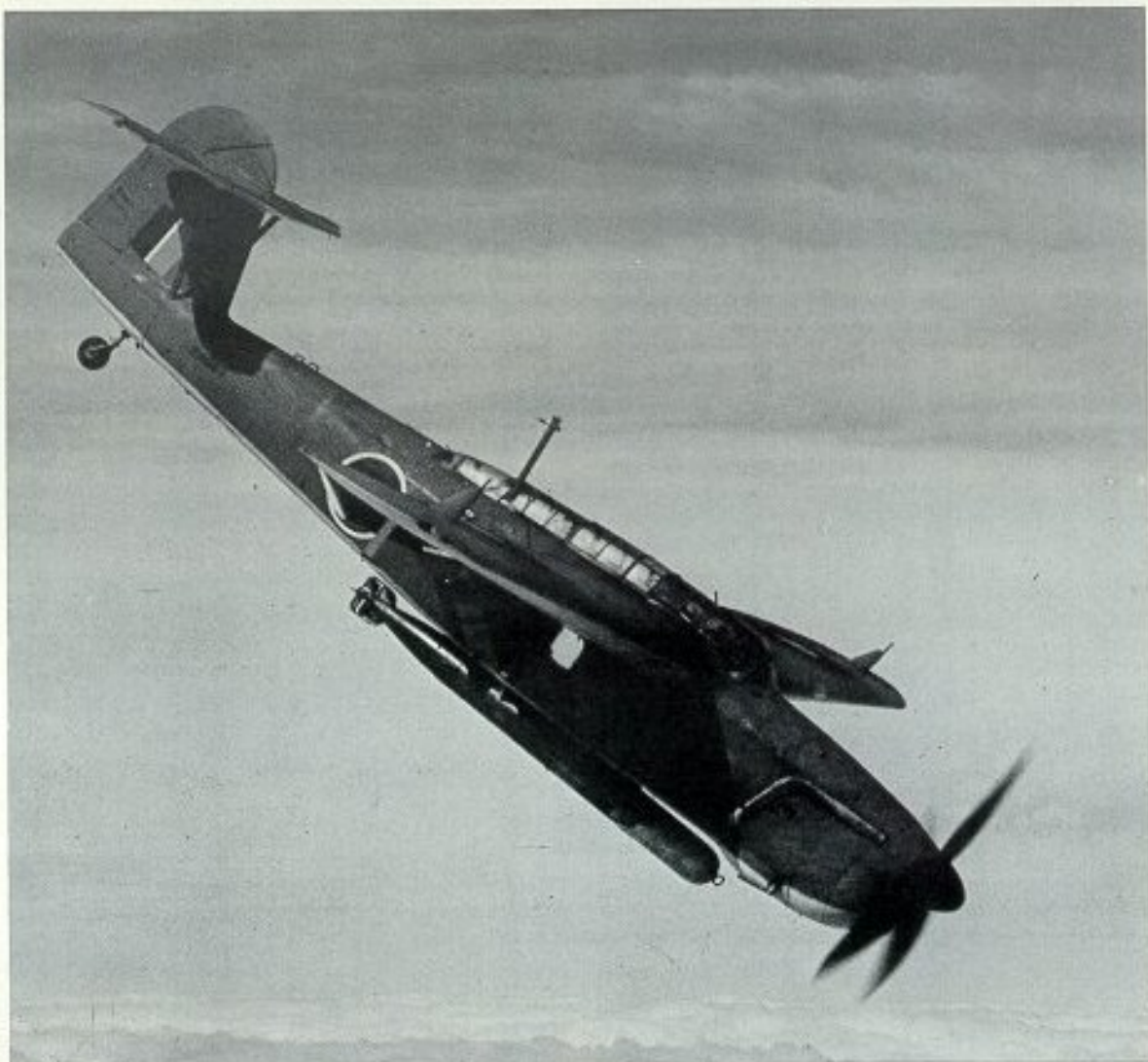
P9667, the first production Barracuda II, seen in a 40° dive, with the flaps at a negative incidence. The monoplane air tail usually fitted to the Mk. XII torpedo has been omitted as its existence was a secret at the time. (Photo: Charles E. Brown)
