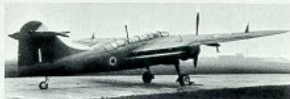
19976, the initial Griffon-Barracuda, a Mark II from the first production batch modified to accommodate a Rolls-Royce Griffon VIII engine, and with an extended dorsal fillet to compensate for the opposite (to the Merlin) propeller rotation and the extra length of the engine cowling. (Photo: Imperial War Museum, ref. ATP.13576D)
