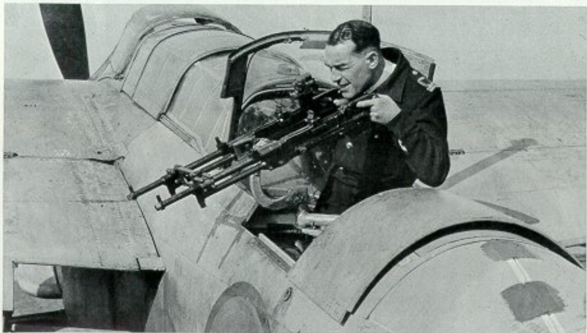
An Observer of 787 Squadron, the Naval Air Fighting Development Unit, demonstrates the twin Vickers machine-gun mounting in the Telegraphist-Air-Gunner's cockpit of P9788. The ammunition drums are not fitted to the guns. Note the dinghy lanyard wire, held over the standard white diagonal stripe by patches of doped fabric. (Photo: via author)
