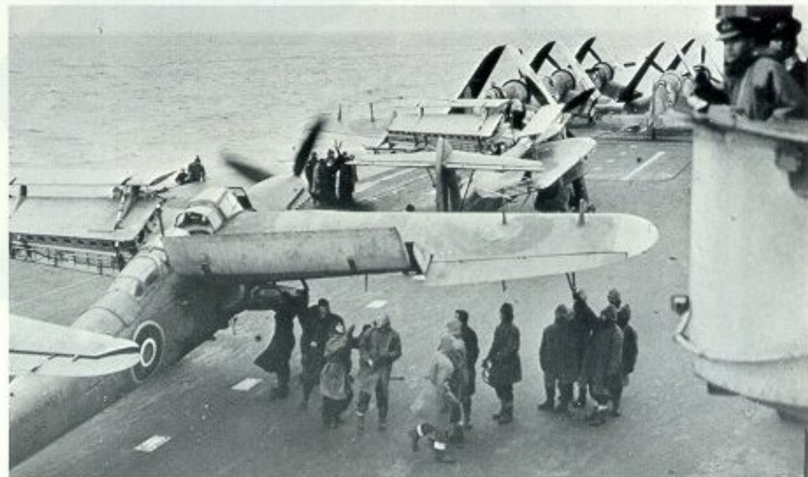
"4A" (LS550, the flagship of No. 52 TBR Wing (829 and 831 Squadrons), folds its starboard flap and inboard trailing edge preparatory to the wings being folded. Note that the TAG's lower window has been removed and replaced by a "solid" panel. (Photo: Imperial War Museum, ref. Q23038)
