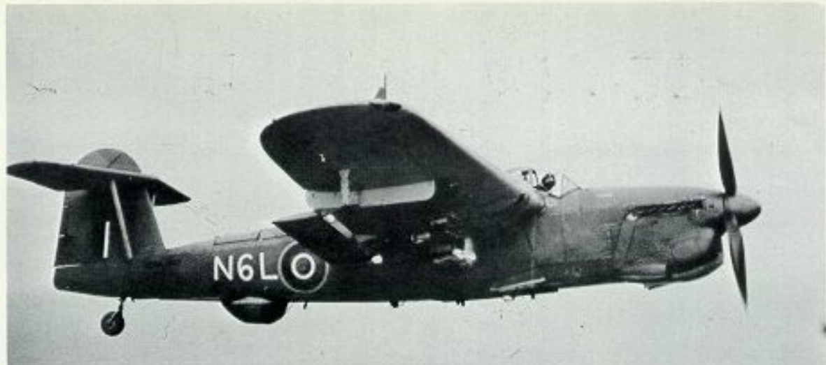
A superb air-to-air view of a Barracuda III of 810 Squadron, seen flying over the Irish Sea. The Squadron was at this time operating from Machrihanish, working up prior to embarkation in HMS Queen in August 1945. Note that this aircraft retains the three bomb-racks of the Mark II, a multiple carrier on the inboard rack carrying three practice bombs. (Photo: C. W. H. Morton)
