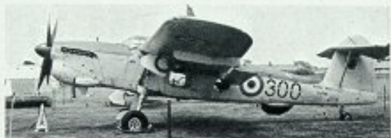
A Barracuda III of 750 Squadron (Observer School) from St Merryn , seen at the Daily Express Exhibition to mark 50 years of flying, in 1951, at RAF Hendon. The discoloration aft of the code number is the doping over the patches on the re-aligned dingy lanyard. (Photo: Charles W. Cain)
