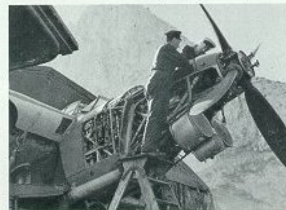
A Barracuda II of the front-line Reserve Aircraft Pool held at Gibraltar for carriers operating in the Mediterranean. The "drums" below the cantilevered Merlin 32 are the engine radiators and the oil cooling radiator (below). Surprisingly, the engine, with accessories and propeller, was nearly as heavy as the remainder of the fuselage structure. (Photo: Imperial War Museum, ref. 21927)
