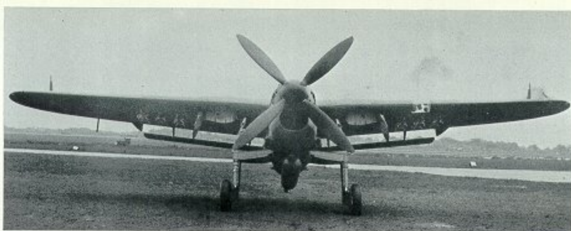
P9647, the prototype Barracuda II, showing the four-blade propeller needed to absorb the extra power provided by the Rolls-Royce Merlin 32 engine. Under the fuselage can be seen the 116-gallon auxiliary fuel tank, and outboard of the wing bomb-racks are the "lee-boards"—boundary-layer fences to prevent the spanwise spread of vortices set up when the flaps were used as dive-brakes. (Photo: Imperial War Museum, ref. 10996A)
