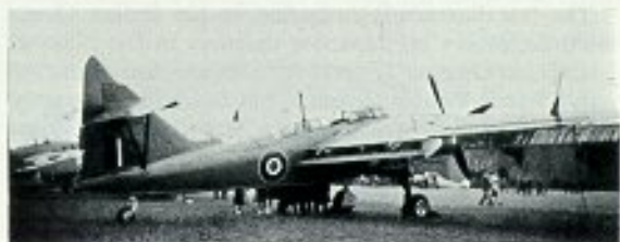
Yet another variation in the shape of the Barracuda V's empennage: RK335 with an extended rudder. (Photo: Charles W. Cain)
