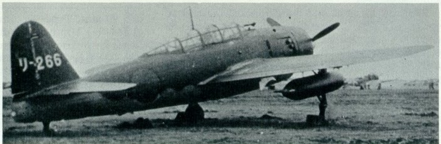
A D4Y3 of the 601st Naval Air Corps, this exceptionally clear view shows to good effect the bulky radial which was installed on the slim fuselage of the Suisei .
