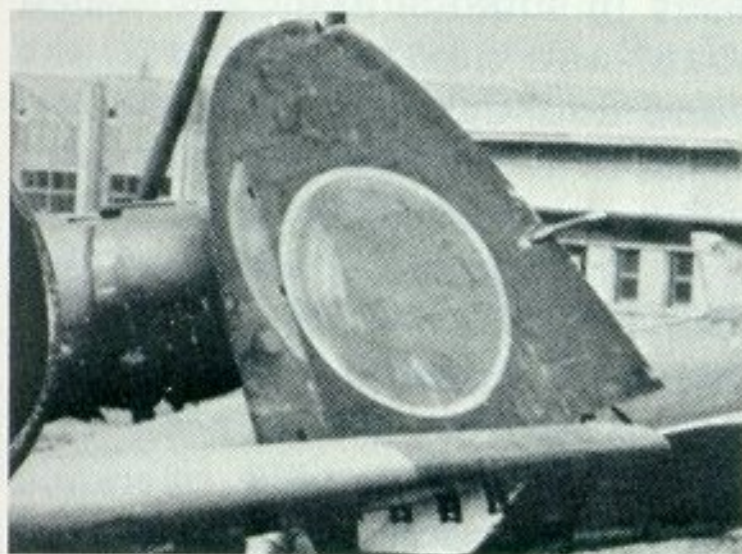
Wing tip folding detail of D3A1 (upper) and D3A2 (lower). The latter, at the Atsugi Air Base, Japan, on September 5, 1945, seems to have port aileron from another aircraft.
