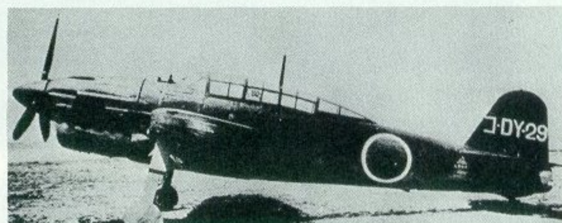
A D4Y2 prototype. The tail legend reads: D=Carrier Bomber; Y=Yokosuka as the designers of the aircraft; 2=second Model; and 9=ninth Prototype. The first letter ko (like mirror "C") indicates that the aircraft is being tested at the Yokosuka Naval Air Technical Arsenal. (Photo: via Major Robert C. Mikesh)
