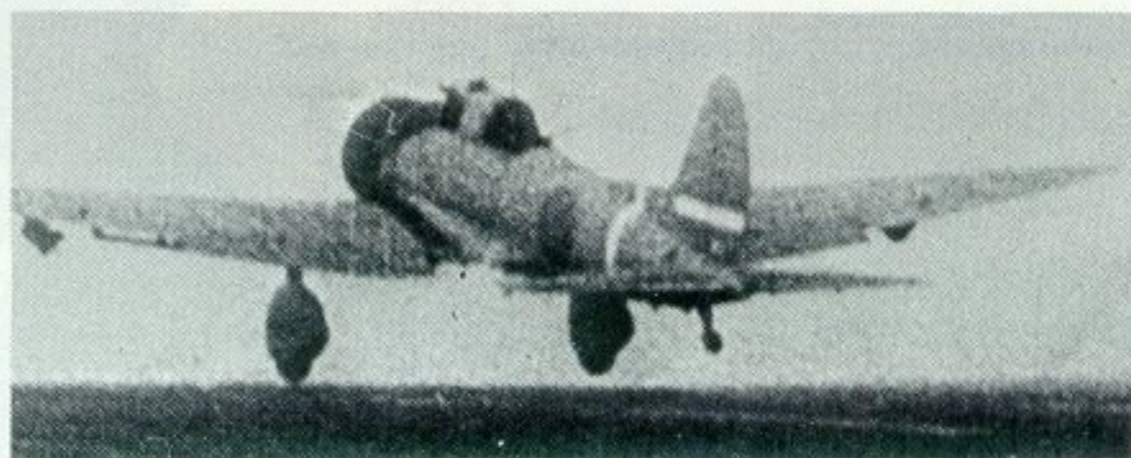
A D3A1 taking-off from a carrier of the IJN in the early months of the Pacific War. The overall light grey paint scheme is in evidence. This aircraft has under-wing bombs attached.
