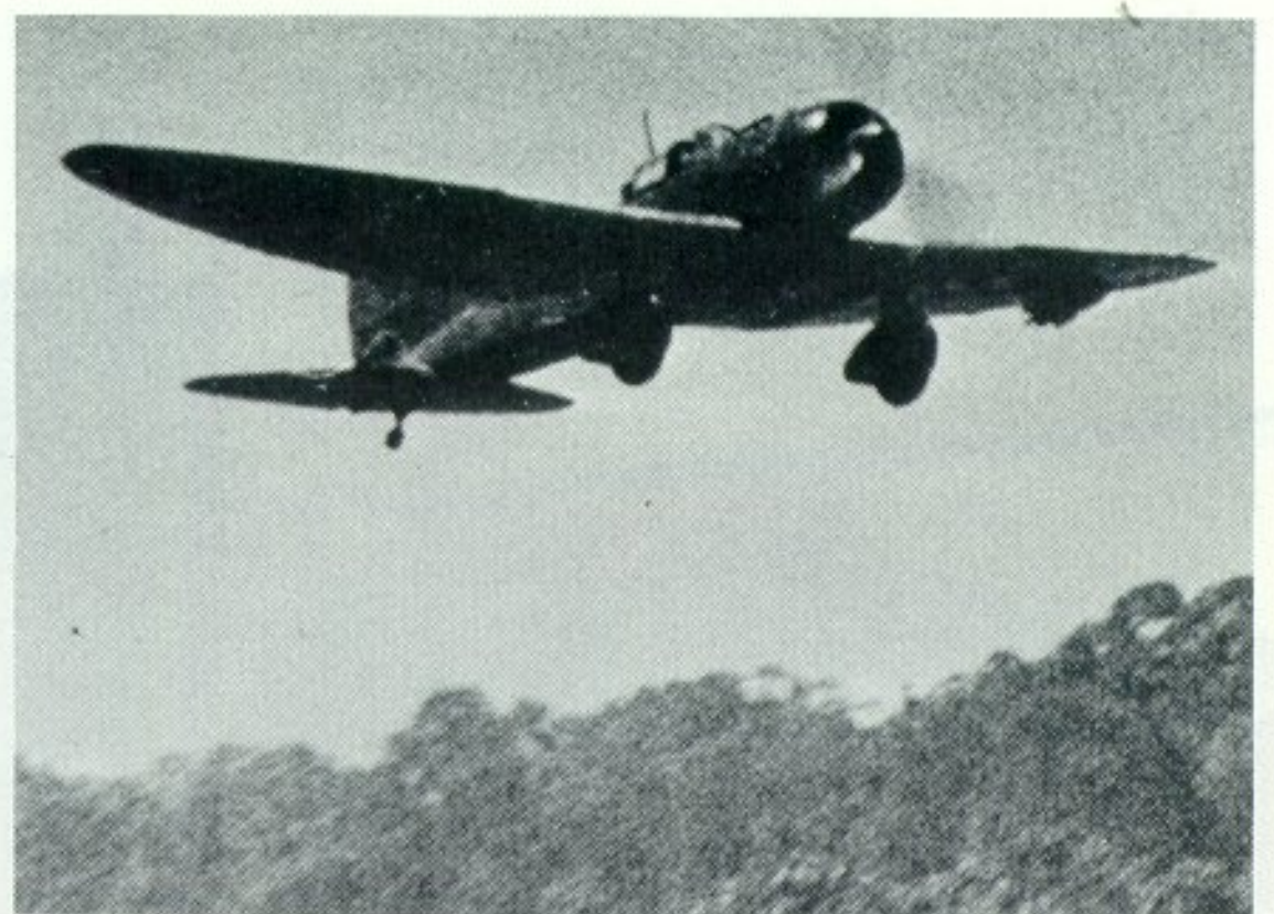
A D3A2 taking-off from one of the four airfields at Rabaul in 1943. Bomb carried under port wing is noticeable.
