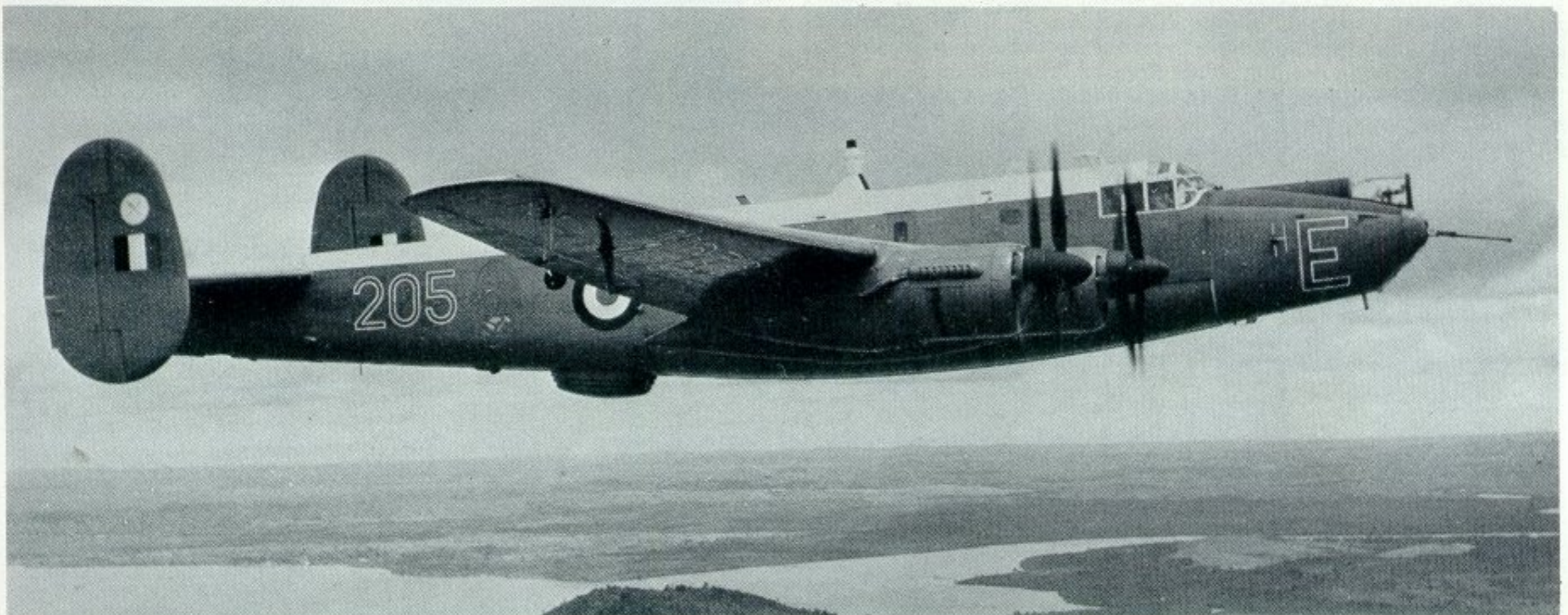
A Mk.2 Phase 2 aircraft, WG532/E, of No. 205 Squadron flying along the Malayan coast in 1967. ECM head fitted, but HF radio posts still old position. No. 205 Squadron never adopted the new colour schemes, and retained their squadron number on the rear fuselage until disbanded at the end of October, 1971. Note engine exhausts from Mk.3 aircraft. Dark blue spinners. (Photo: Roger Brooks)
