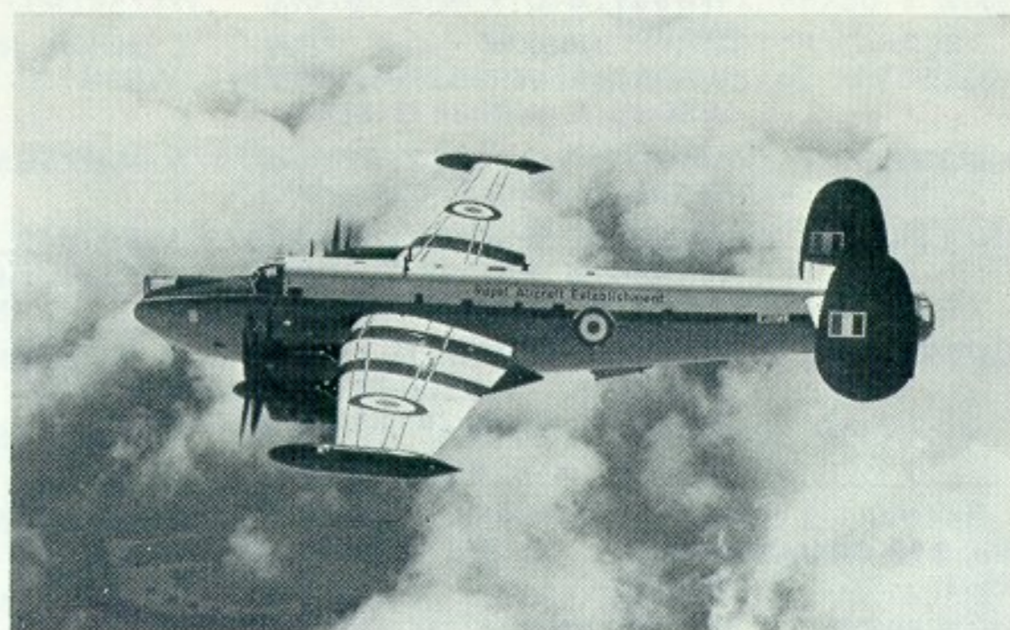
WR972, a Mk.3 Phase 2 aircraft without ECM, purchased by the Ministry of Technology in March, 1959 for the Royal Aircraft Establishment. Note rear fuselage observation position. Colour scheme dark blue and white, grey fuselage.
