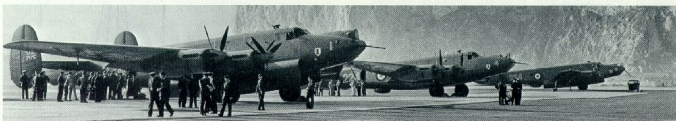
WB828 of No. 120 Squadron photographed at Bovingdon on April 23rd, 1956 displaying the newly-adopted standard scheme of aircraft letter on the nose, and squadron number on the rear fuselage, both in red outlined in white. Note coloured spinners.
