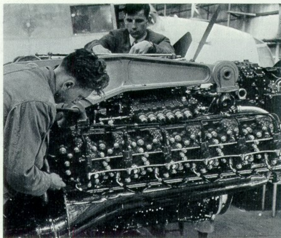
A real Napier Nomad E.145 engine fitted in the starboard outer nacelle of Shackleton VW131 at Napier's Luton hangar ready for trials to start. See text.
