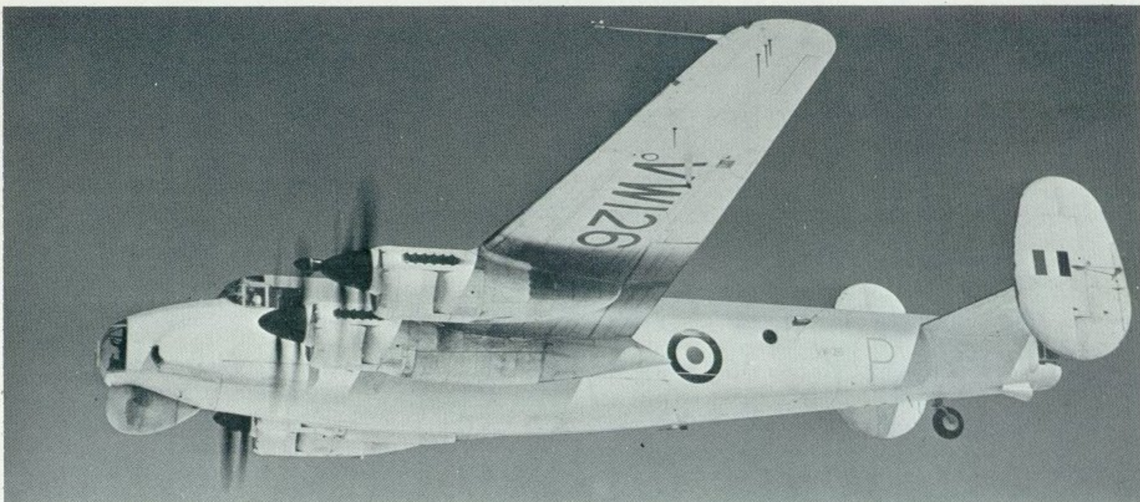
Top The first flight of the prototype Avro Shackleton VW126 at Woodford on March 9th, 1949. The aircraft, piloted by Mr. Jimmy Orrell, was airborne after a 14-second run. (Photo: A. V. Roe) Bottom Another view of VW126 showing the nose turret barbettes, the tail turret, and the flight refuelling pick-up under the tail. The housing for the radio d/f loop can be seen above the cockpit roof, and the three aerials under each wingtip are for sonobuoy homing. (Photo: Harry Holmes)
