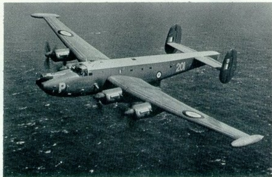
XF707 201/P, the first Mk.3 Phase 1 aircraft, seen soon after delivery. The long whip aerials of the VHF radio homer on the nose identify the Phase 1 aircraft, but note also the SARAH aerials on the nose sides just aft of the letter, and the 'snifter' intake just below them.
