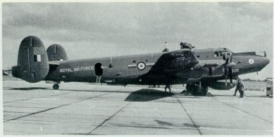
WL756, a Shackleton AEW Mk.2 of No. 8 Squadron, seen at R.A.F. Wattisham in June, 1972. Note squadron badge on nose (Arabian dagger on white circle) and last two numbers of serial repeated on fin. Turret deleted from nose, and most of "maritime" equipment removed. (Photo: M. Brewer)
