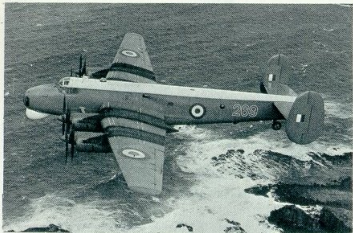
VP291 of No. 269 Squadron in March, 1958 over Irish Coast. During the period 1957 to 1960 aircraft from Ballykelly did not carry aircraft letters. Note intake for 'snifter' equipment on nose side, mounted lower on Mk.2 aircraft. (Photo: Flight)
