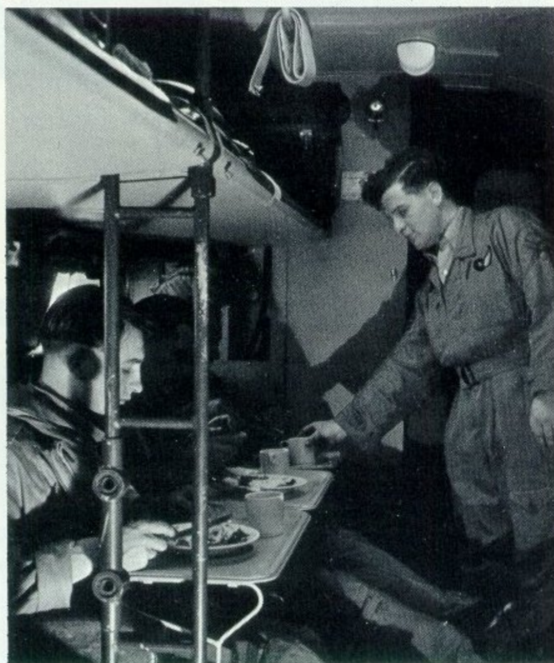
Lunchtime for some of the crew of Mk.3 Phase 1 XF730 206/C in the rest room during a flight to Gibraltar on November 14th, 1960. There are two tiers of three bunks, but the centre ones have been dropped down to form backrests, and trays clipped on for mealtime use. Note rexine lining over soundproofing, and access door to rest room over signallers left shoulder.
