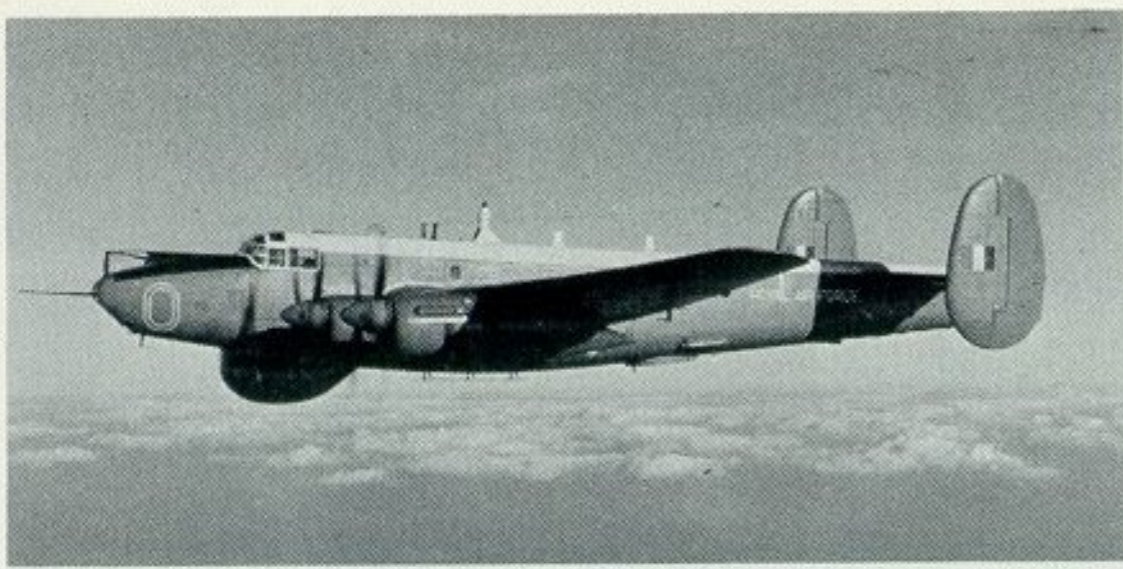
WL745, the prototype Shackleton A.E.W. Mk.2, on its maiden flight of September 30th, 1971. Radome from Fairey Gannet 3 aircraft faired into forward bomb-bay, normal radome removed, and extra aerials of transmitters along roof. All the twelve aircraft to be converted will be ex-Phase 3 aircraft. (Photo: Hawker Siddeley)
