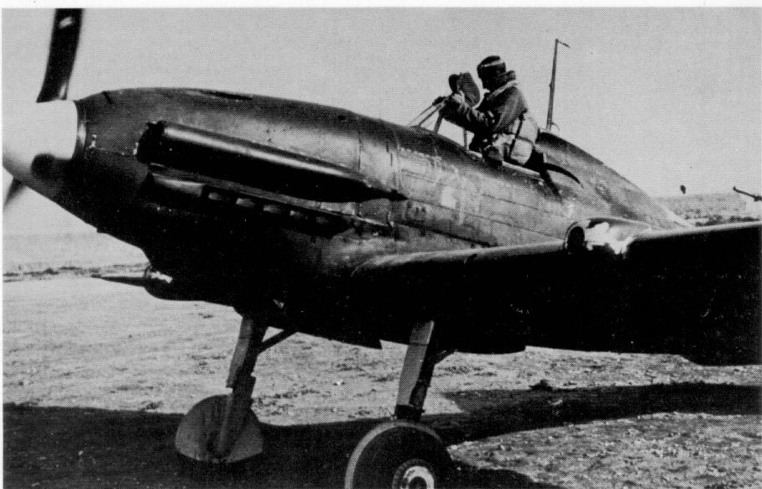
The photo-reconnaissance version of the Caproni Reggiane Re 2001. Note the leading-edge camera housings.
