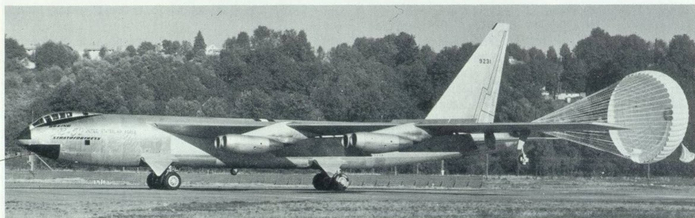
The YB-52 deploys the 44-foot braking parachute during a landing. Observe that the prototype has sufficient forward speed here to have lift on the wings, as evidenced by the height of the wingtip protection wheels above the ground. (Photo: Boeing)
