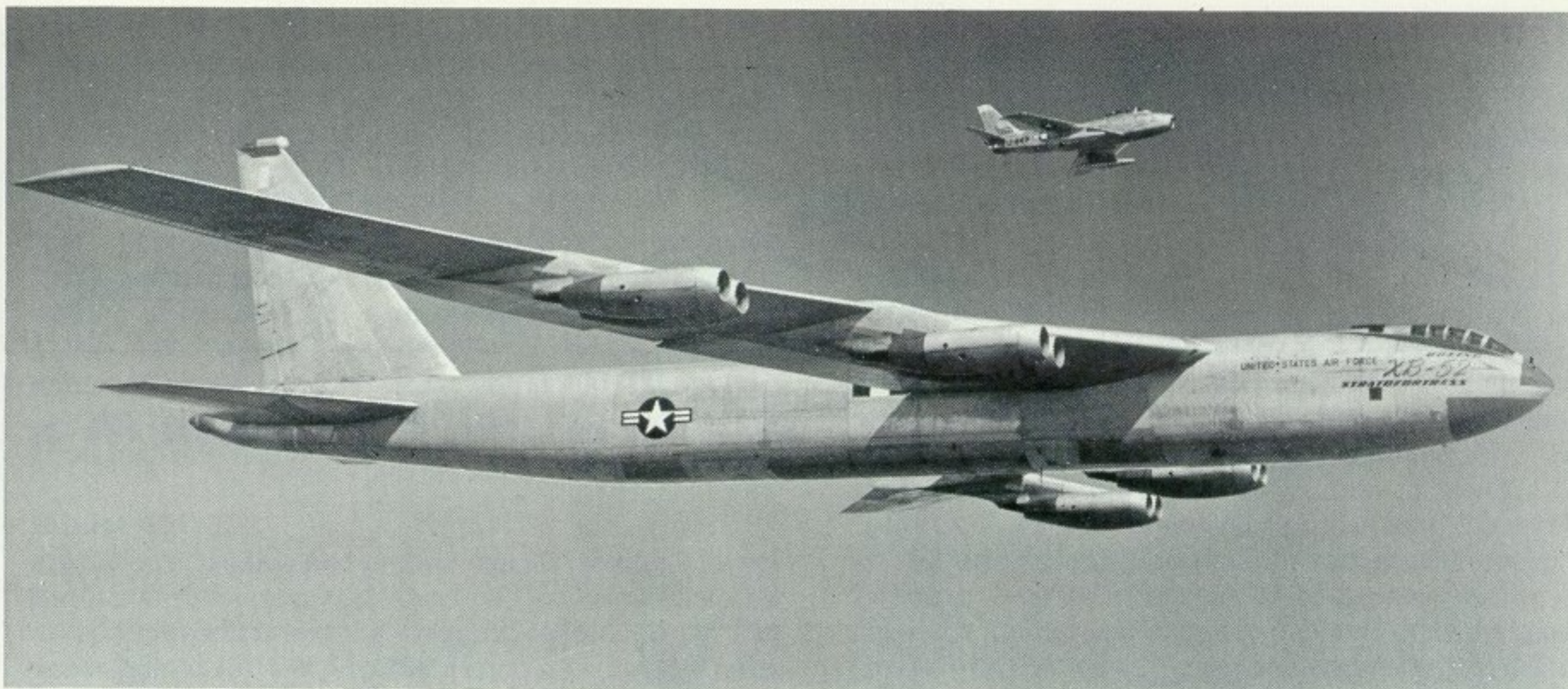
The prototype Boeing XB-52 (USAF serial number 49-230) on an early test flight accompanied by a North American F-86 Sabre "chase plane". The device at the top of the vertical fin is part of the test equipment. (Photo: Boeing)
