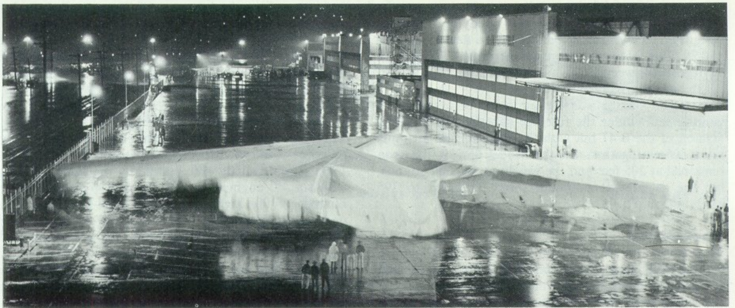
The completed XB-52 was transferred from the Boeing factory to the flight test hangar under wraps and in great secrecy on the night of November 29, 1951. The fold-down vertical tail was a feature of all subsequent B-52s. (Photo: Boeing)
