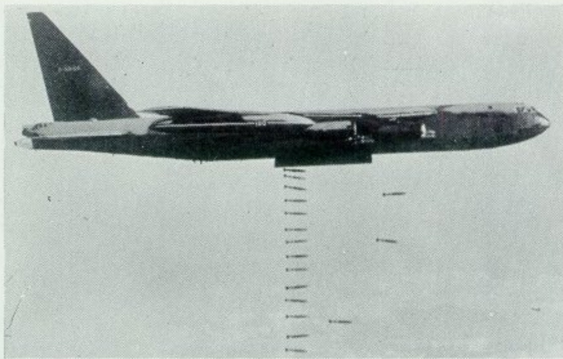
A Seattle-built B-52D (USAF: 65-100; here as 0-50100), dropping 500-lb "Iron Bombs" in train. Eighty-four of these bombs are carried in the bomb-bay with an additional 24 bombs, either 500- or 750-pounders, carried on two wing pylons. (Photo: USAF via Boeing)
