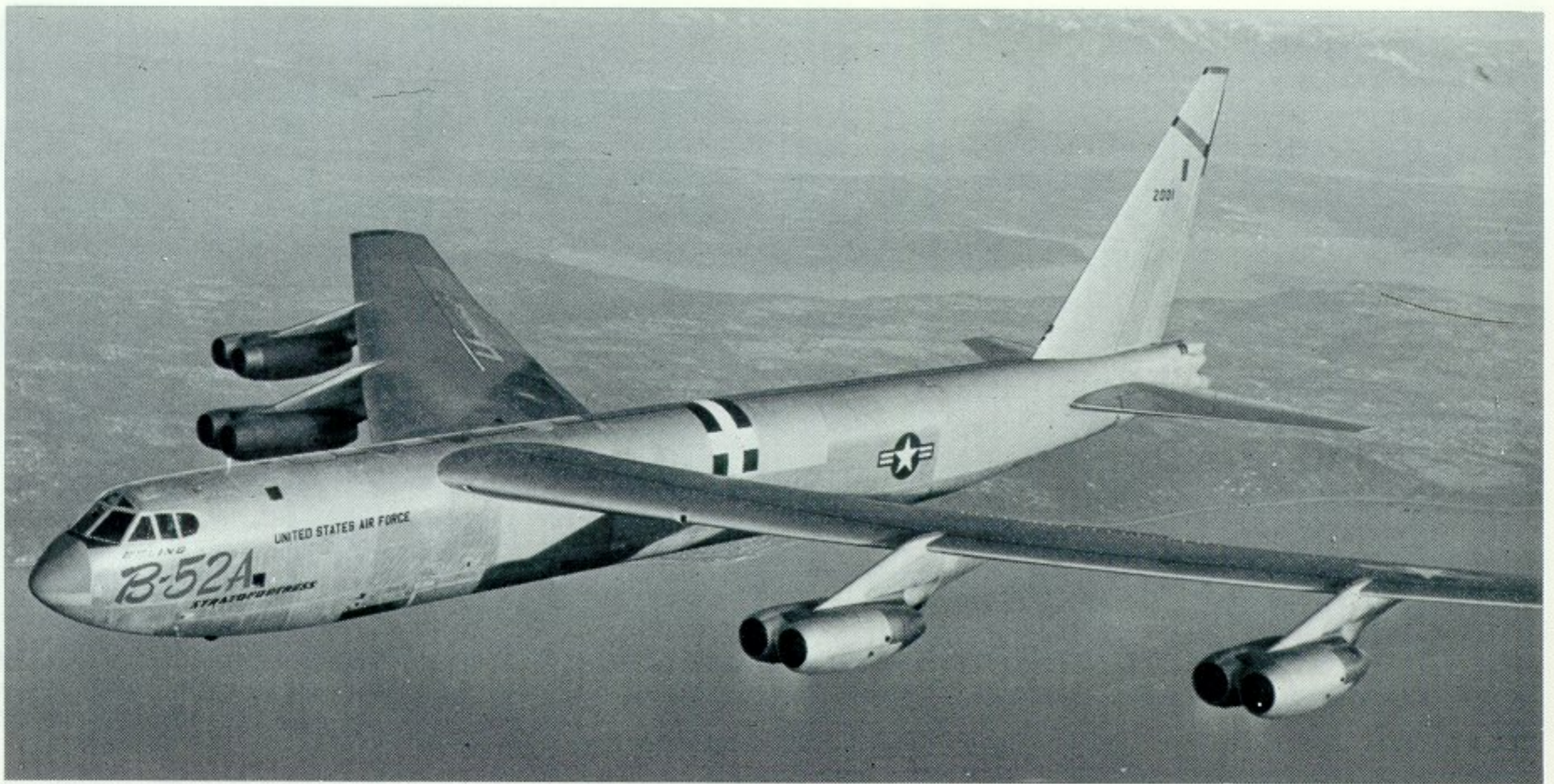
The first production B-52s were the three B-52As, differing outwardly from the prototypes in having a revised nose design for side-by-side crew seating. This is the first B-52A (serial no. 52-1; shown on tail as 2001) on an early test flight. (Photo: Boeing)
