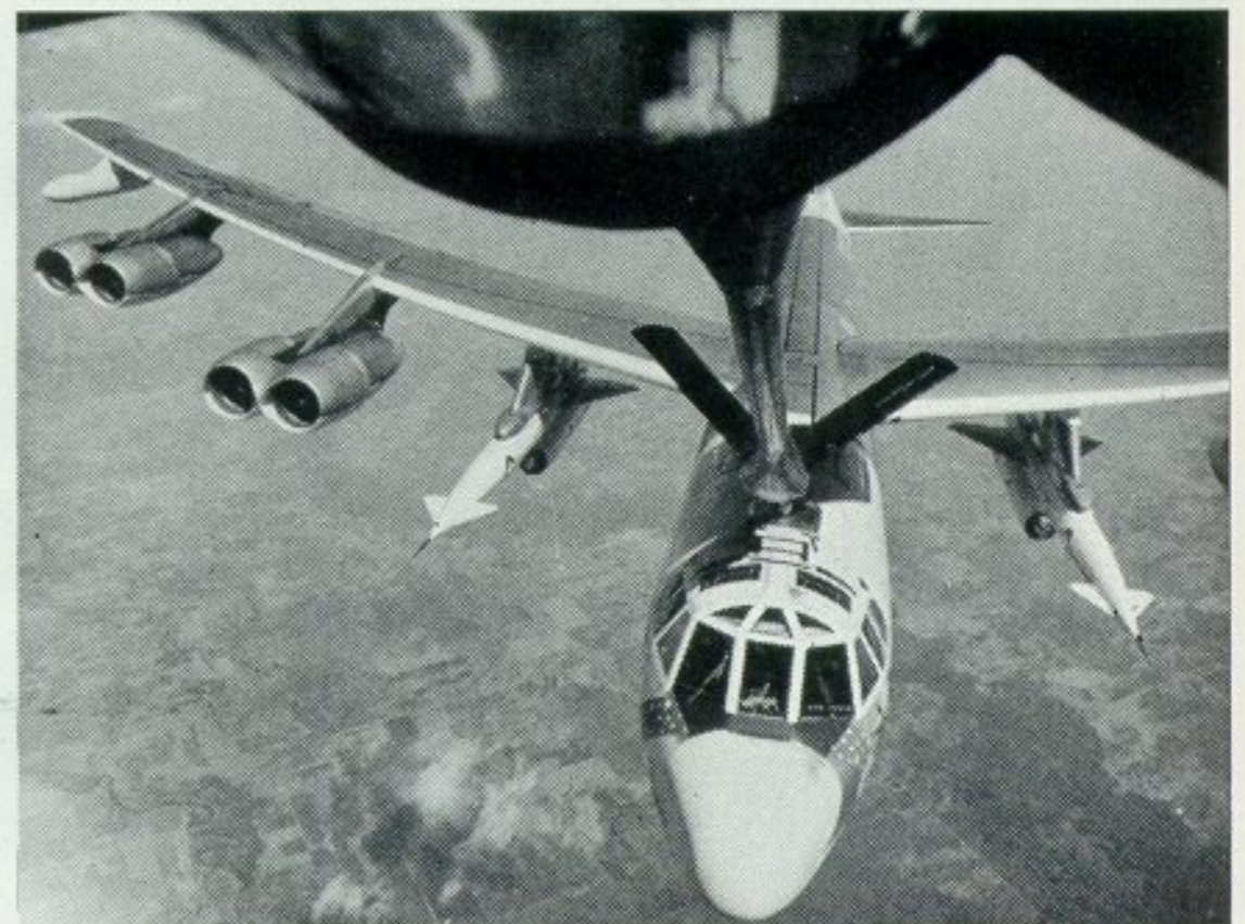
Test model of B-52H (with AGM-28 Hound Dog missiles) in process of aerial refuelling. (Photo: Boeing)
