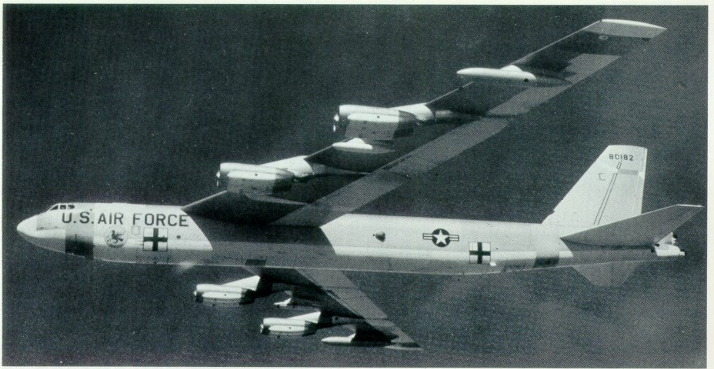
A B-52G with 700-gallon (U.S.) drop tanks being used by the Air Force to test electronic countermeasures pods that can be seen under the wings between the inboard and outboard nacelles. Note the double theodolite target markings fore and aft on the fuselage. (Photo: USAF via Boeing)
