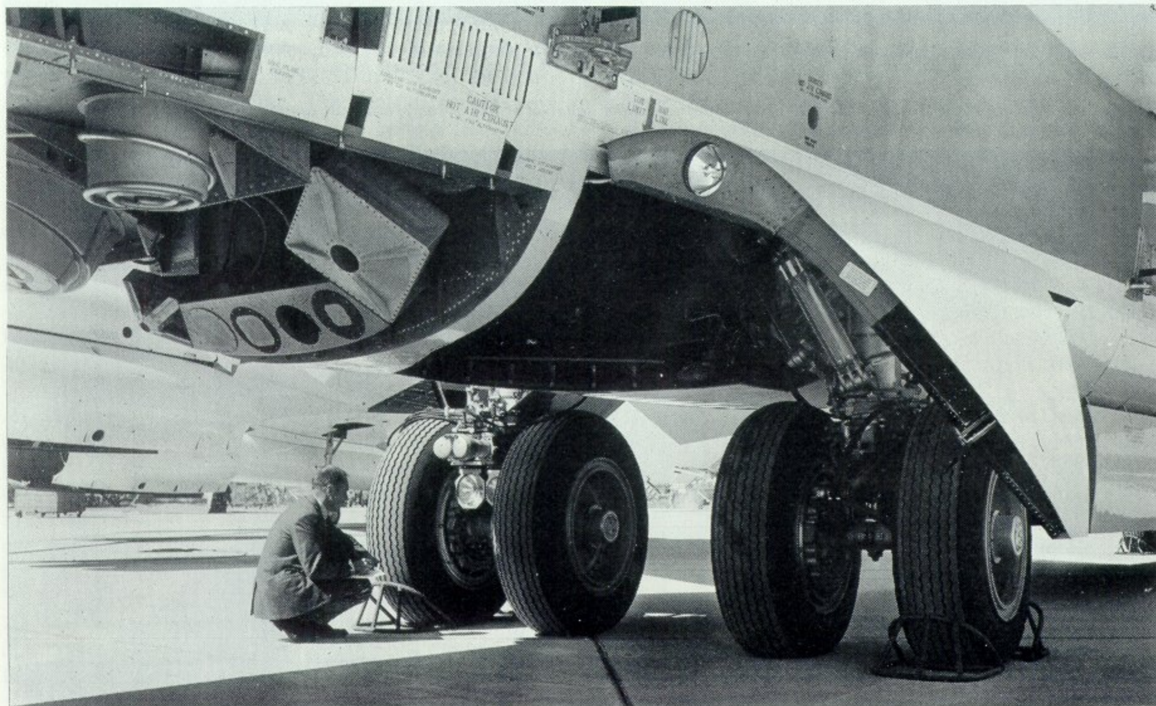
Forward landing gear units of a B-52B revealing that the landing lights are built into the wheel well doors. The lower radome has been removed to show some of the radar installation. (Photo: Boeing)
