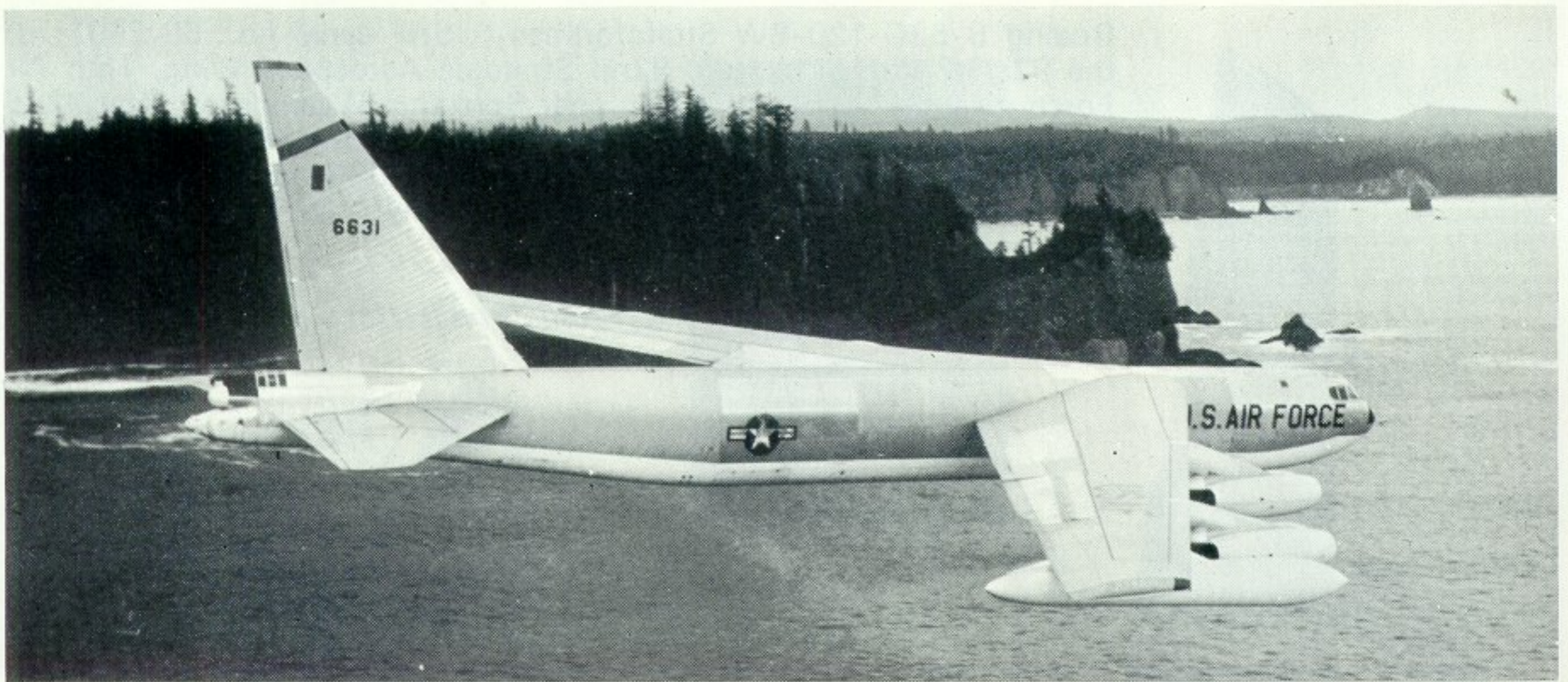
With a reinforced airframe, the first Seattle-built B-52E (USAF: 56-631) was used to develop low-altitude penetration techniques whereby the bomber could approach the target undetected by flying below the defensive radar screen. (Photo: Boeing)
