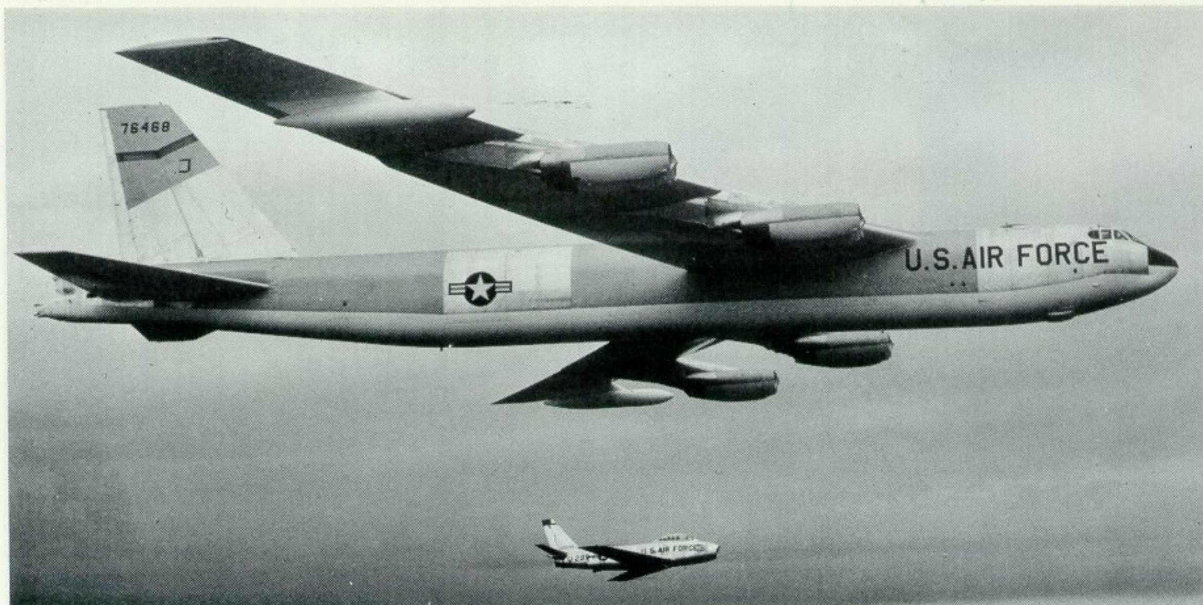
The first B-52G (USAF: 57-6468) on an early test flight accompanied by a "chase" F-86 Sabre. Principal external identifying feature is the shortened vertical tail. Seattle B-52 production ended with the B-52E; all subsequent B-52 models were built only at Wichita. (Photo: Boeing)
