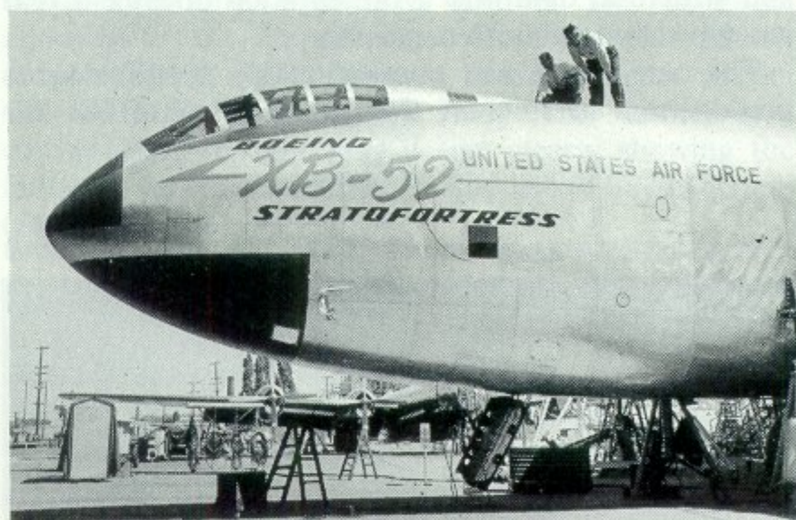
Nose of the XB-52, showing the tandem canopy for the crew and the entry hatch under the belly. The dark areas are moulded non-metallic structures to cover radar equipment. A B-29 Superfortress is jacked-up in the background. (Photo: Boeing)
