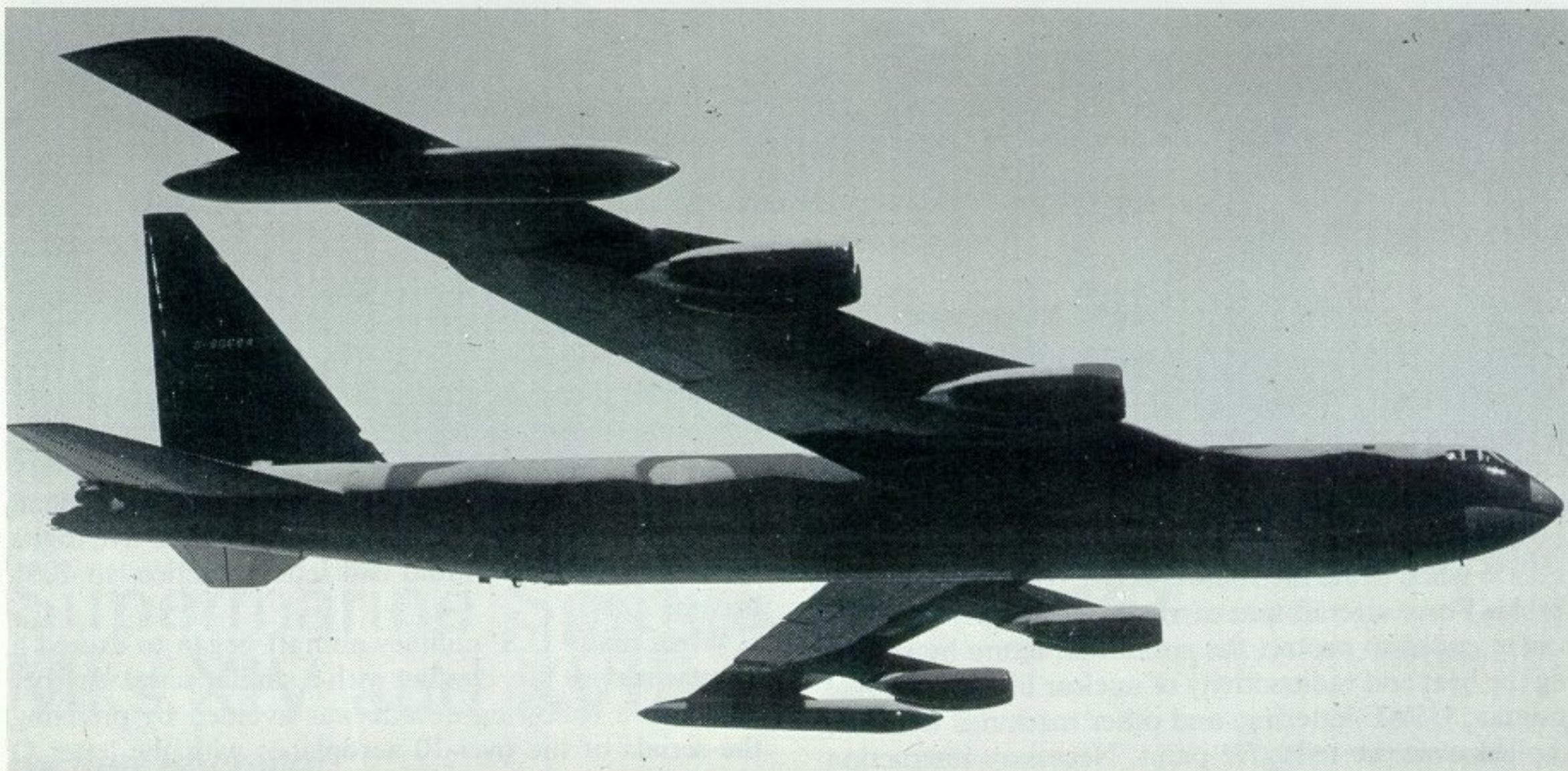
A Wichita-built B-52D (USAF: 56-684; as 0-60684 on the fin) in camouflage. Black undersides and vertical fin are used in Viet Nam operations. Serial number in red on the black fin. (Photo: Boeing)
