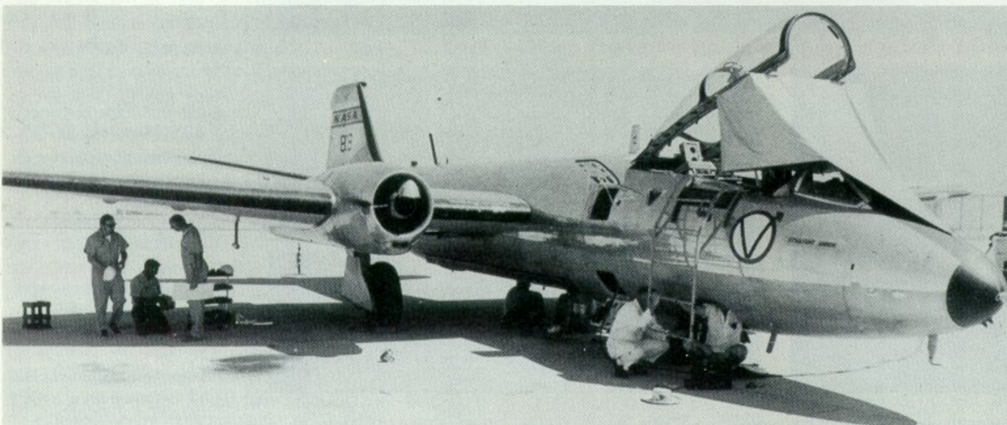
A sunshade shields the cockpit from the desert sun on the flight line at NASA's Flight Research Center, Edwards, Calif. This B-57B, registered NASA 809, is used for tests of the Viking Mars-lander parachute, and for probing the upper atmosphere for clear-air turbulence.
