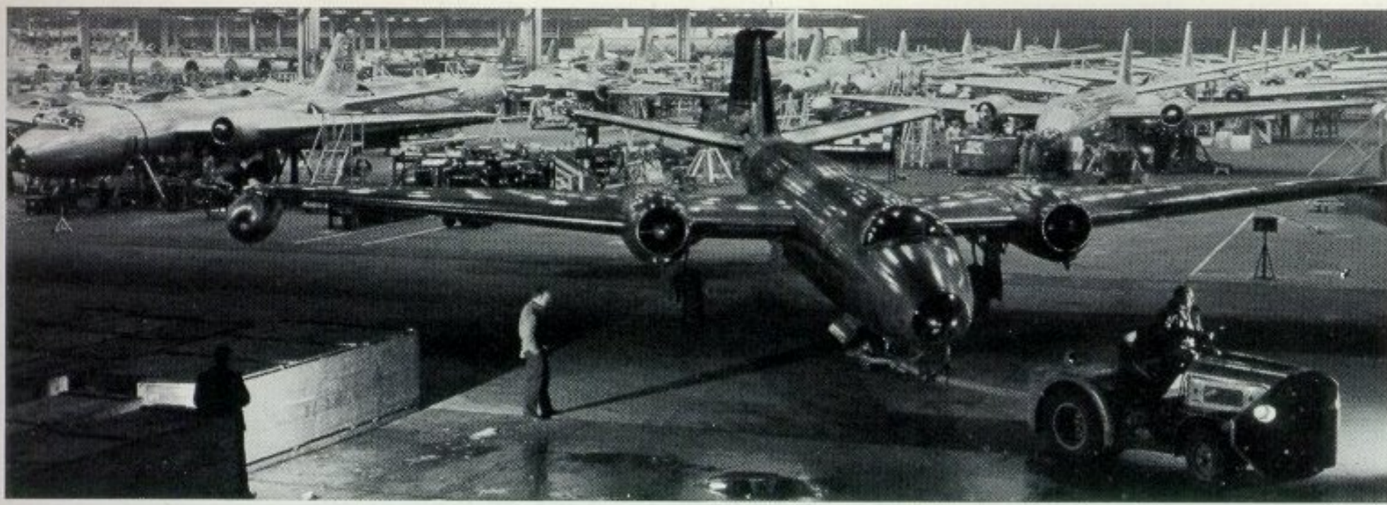
In early 1954, the Martin B-57 assembly area in Plant 2 was crammed with aircraft; about 20 are shown here in final assembly, plus a large number of fuselages in jigs to the left. Aircraft 5, B-57A (52-1422) is at the forward position on the line to the left; the aircraft under tow is presumed to be B-57A No 4. (Photo: Martin, ref. P-50228)
