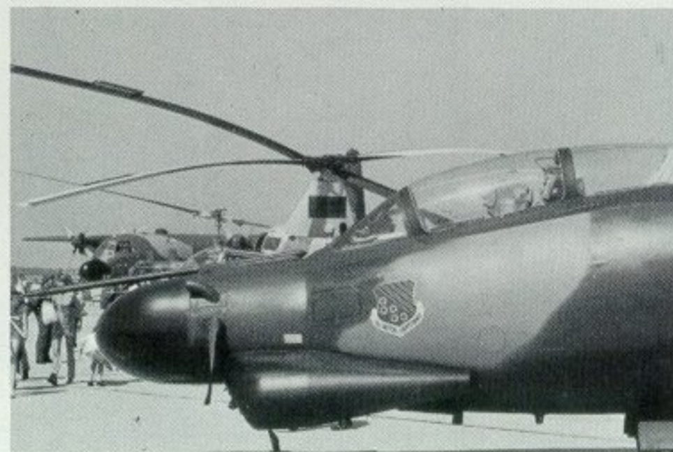
Nose details of B-57G (53-3906) assigned to the 1st Tactical Fighter Wing, emphasize the shape of the jowl fairings added to house the special sensors. Note that the nose is also extended as well as modified in contours; the bay behind the radome was necessary to mount the extra installations. Long boom protruding forward is an accurate pitot head. (Photo: Ken Buchanan)
