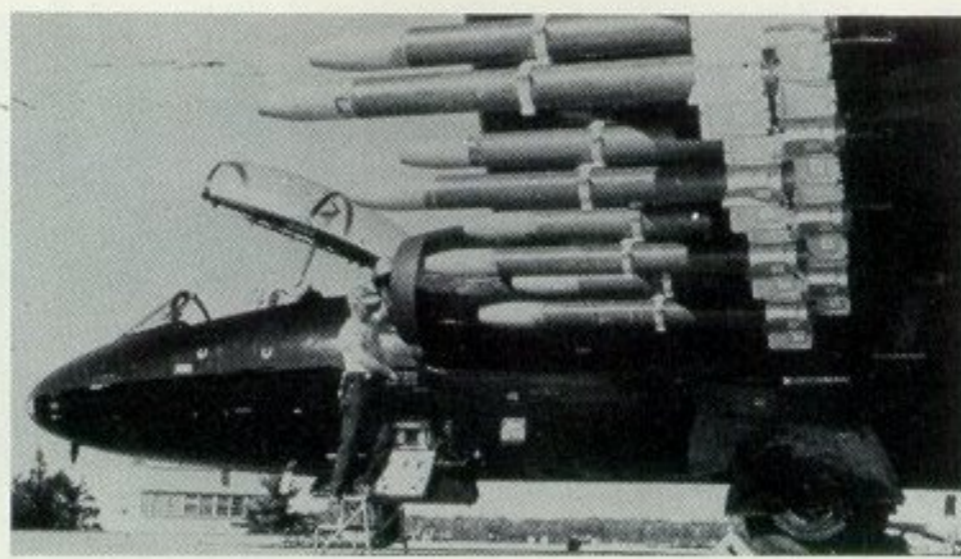
Ready to drop, this B-57B carries nine 500-lb. bombs on its rotary bomb door plus four more on underwing pylons. Smoke stains on underwing are from gunfire. Dark circular area below US insignia on rear fuselage is Shoran antenna. (Photo: USAF 98346)
