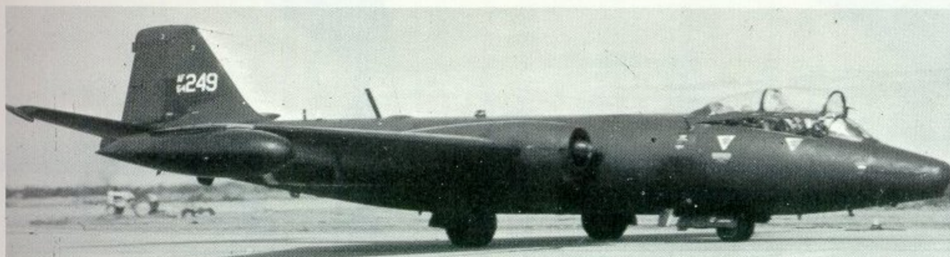
One of the Patricia Lynn aircraft, B-57E (55-4249), returns to Tan Son Nhut AB, Viet Nam, after a mission on December 14 1970. Note the elongated nose which housed a forward-looking Fairchild KA-1 camera. Aircraft is in flat black finish with flat white tail codes; it was assigned to Det. 1, 460th Tactical Reconnaissance Wing.
