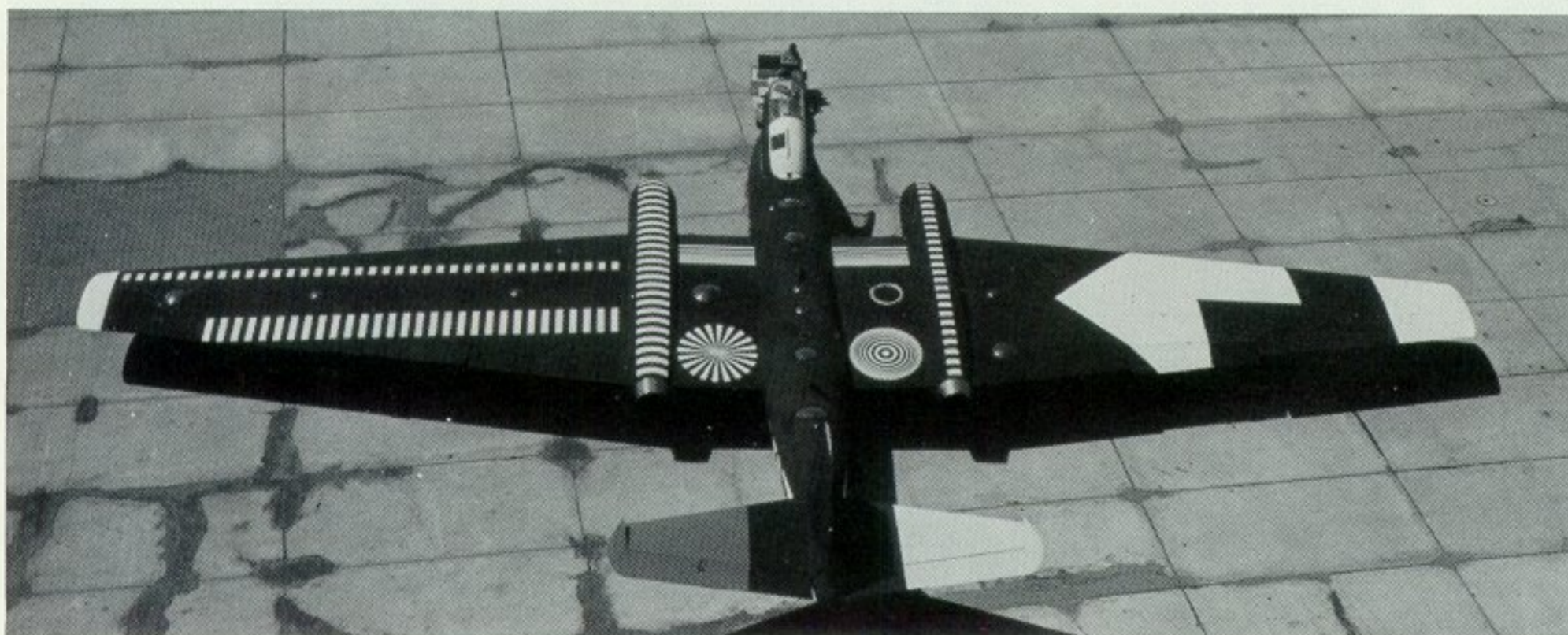
The unusual markings on this RB-57D at Wright-Patterson AFB were done to test the quality of lenses and film emulsions in Project APRE (Aerospace Photographic Reconnaissance Experiments). Neutral grey area on left horizontal tail is photographic standard for color reproduction. A dozen convex mirrors are positioned on fuselage and wing upper surfaces. Aircraft was flown below a balloon carrying the camera on test, and photographed as it passed within the camera's field of view. (Photo: USAF)
