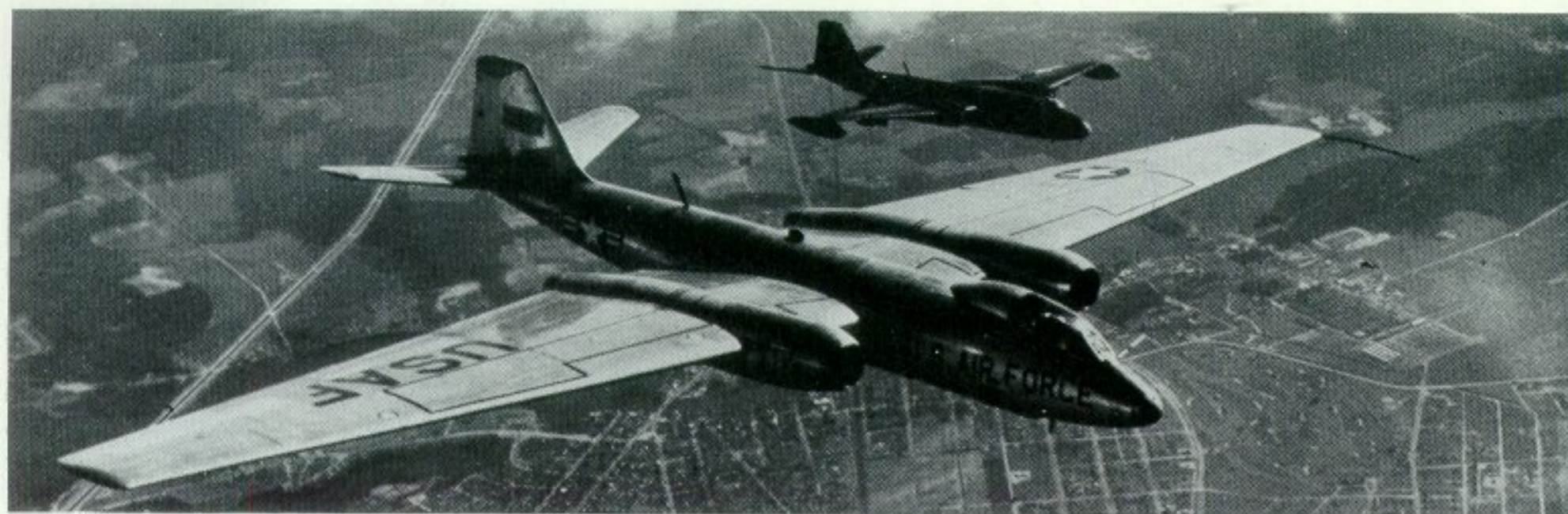
The first RB-57D, serial 53-3977, was accepted by the USAF in November 1955. Assigned to Strategic Air Command for day photo reconnaissance, the aircraft was one of a batch of six designed for the job. Note the break in the belly contour under the cockpit, where cameras were mounted. This aircraft later served with the Air Weather Service and then was converted to an EB-57D and assigned to ADC for defence systems evaluation, where it was based at Hill AFB, Utah. It was in storage at MASDC in May 1972.
