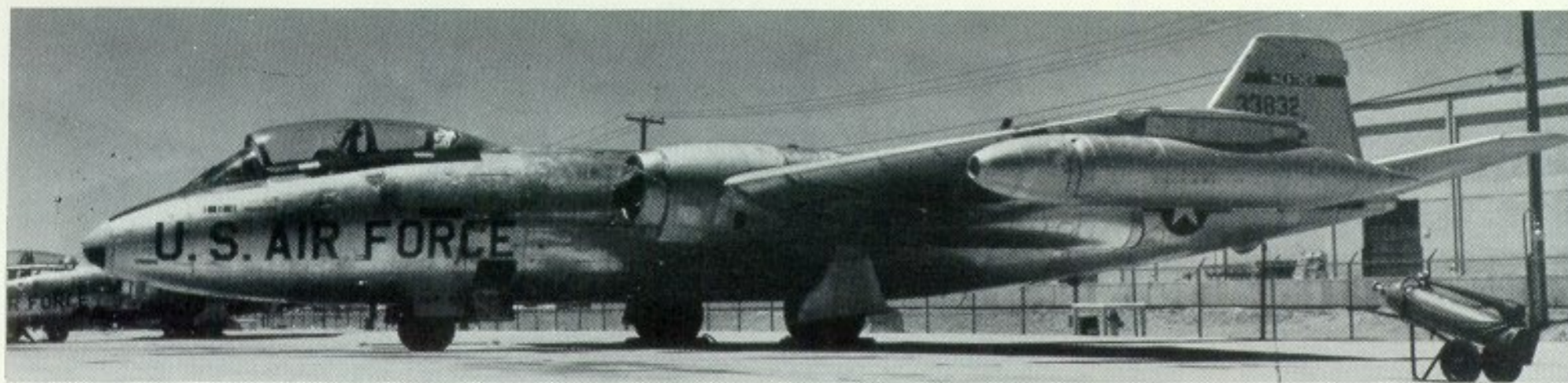
Wingtip pods for capture of airborne debris from nuclear weapons tests are carried by this RB-57C (53-3832) of the Air Weather Service photographed in May 1965. Pods have removable paper filter elements, were developed by the Los Alamos Scientific Laboratory. Aircraft is now designated WB-57C and was still assigned to the 58th WRSq in April 1972. (Photo: via Gordon S. Williams)
