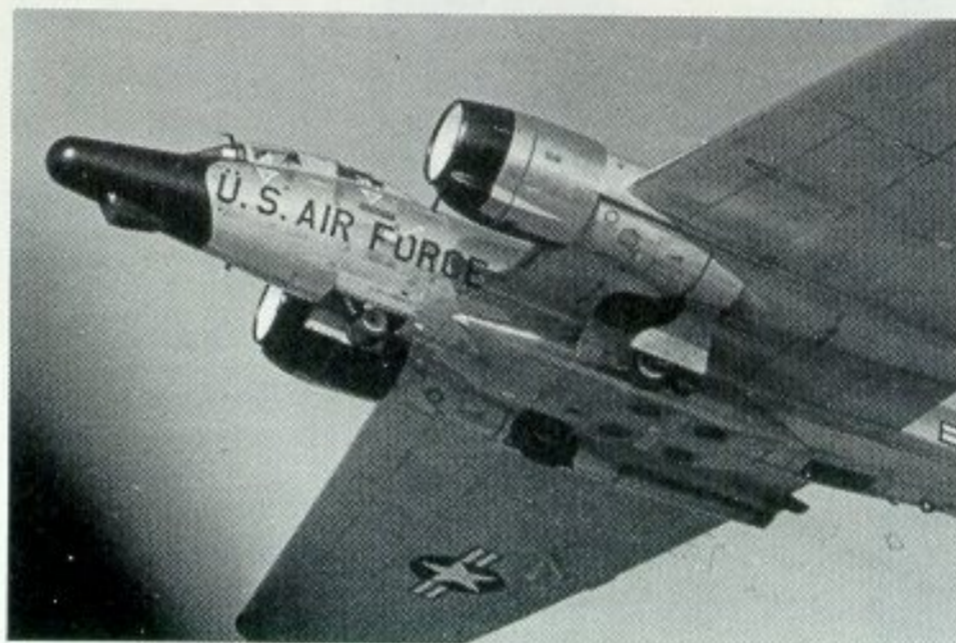
The camera pallet under the fuselage of this WB-57F was developed for the corn blight experiments, and is typical of the installations that will be used in support of NASA's ERTS (Earth Resources Technology Satellite) programme. (Photo: NASA)
