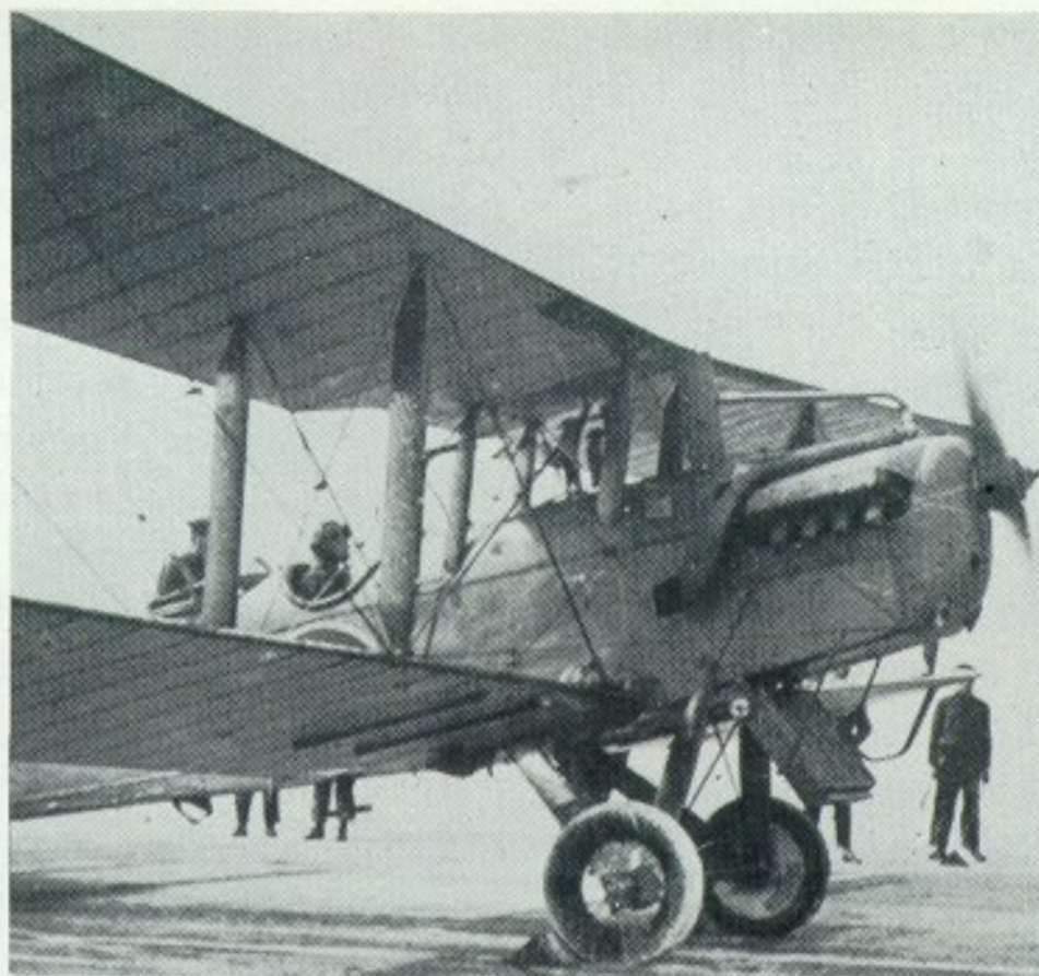
D.H.9A, E752, fitted with Napier Lion, warming up for take-off during deck-landing trials aboard the aircraft carrier, HMS Eagle in 1920. (Photo: via R. C. B. Ashworth)
