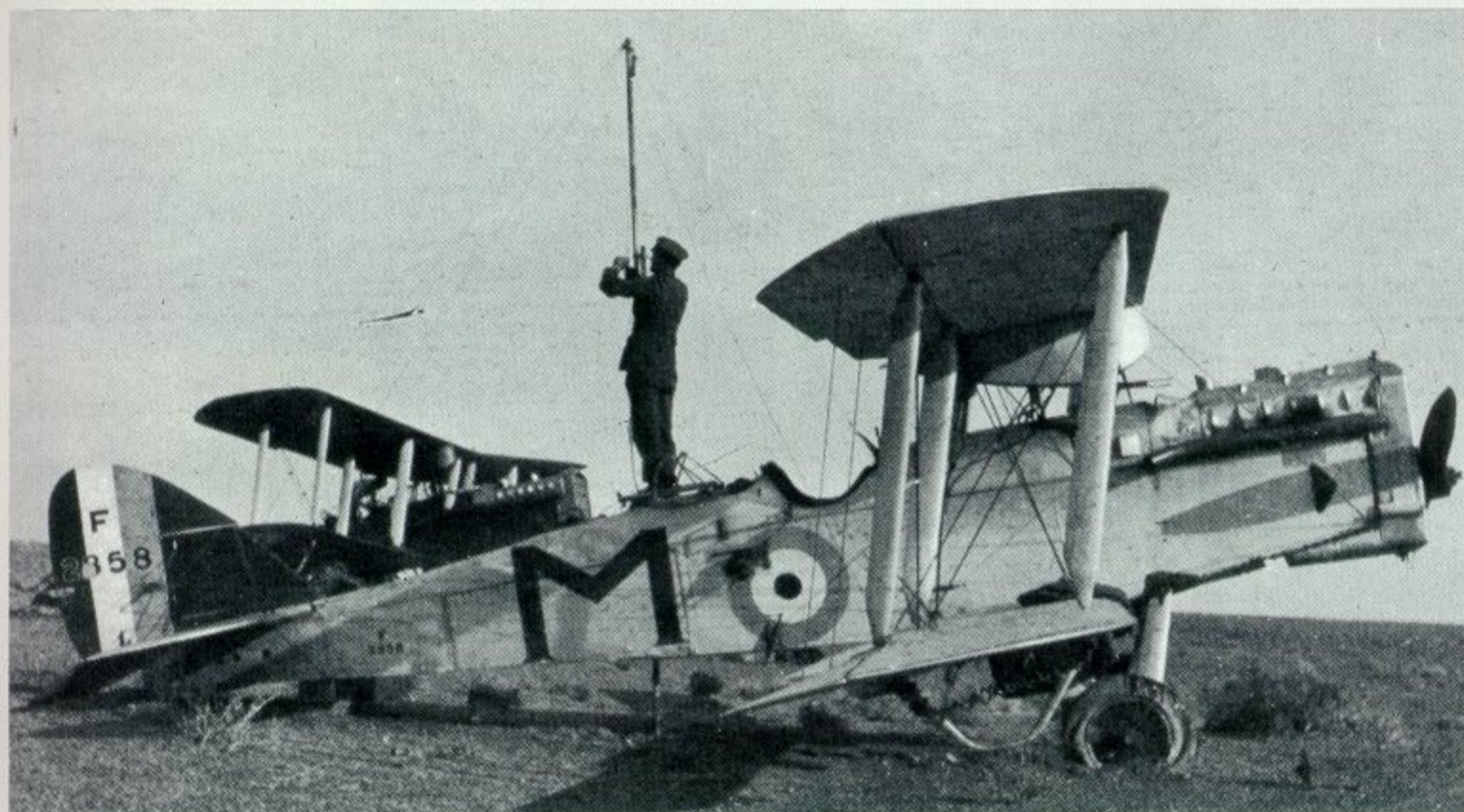
F2858, 'M' of B Flight, No. 8 Squadron (subject of the 5-view colour centrespread) after a forced landing in lava country, Palestine, 1924. The airman is raising the W/T aerial for communication. (Photo: Wing Commander N. H. F. Unwin, MBE)
