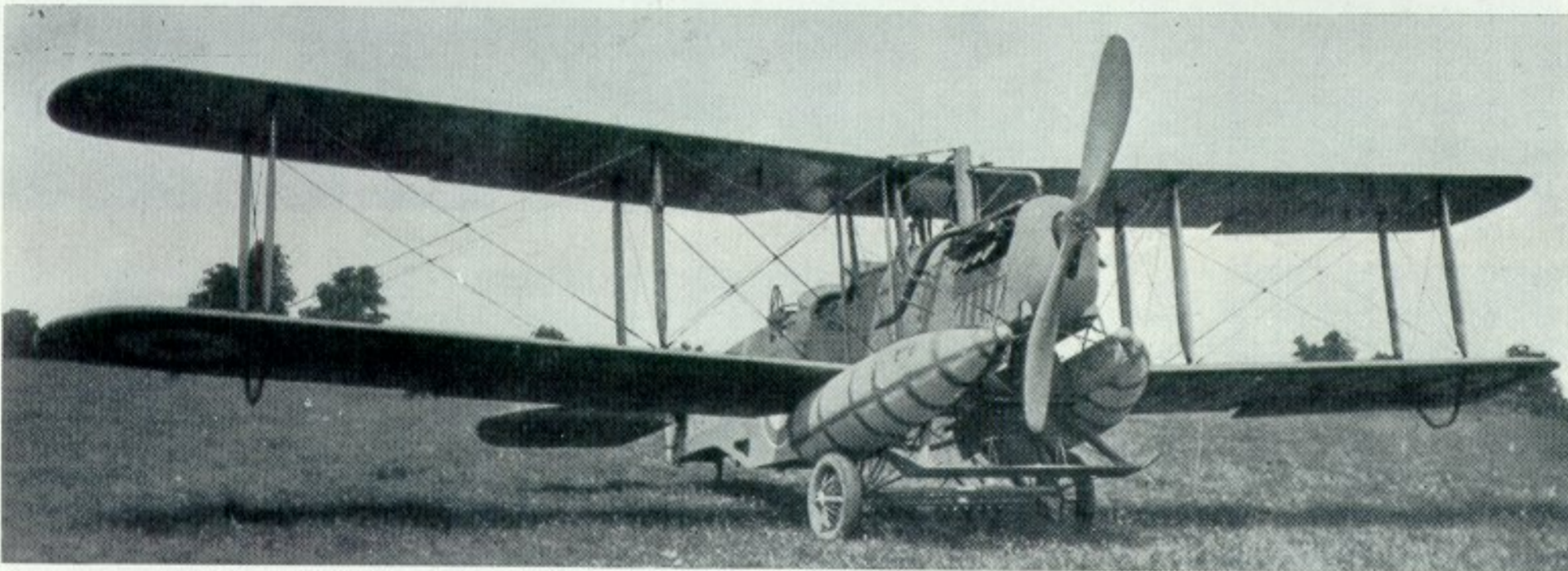
The Ugly Sister—Westland's Walrus version, a three-seat Ninak with prone Observer's under-compartment, flotation bags (shown inflated), Napier Lion engine and forward hydrovane extended; it was not a success. (Photo: Westland Aircraft Limited)
