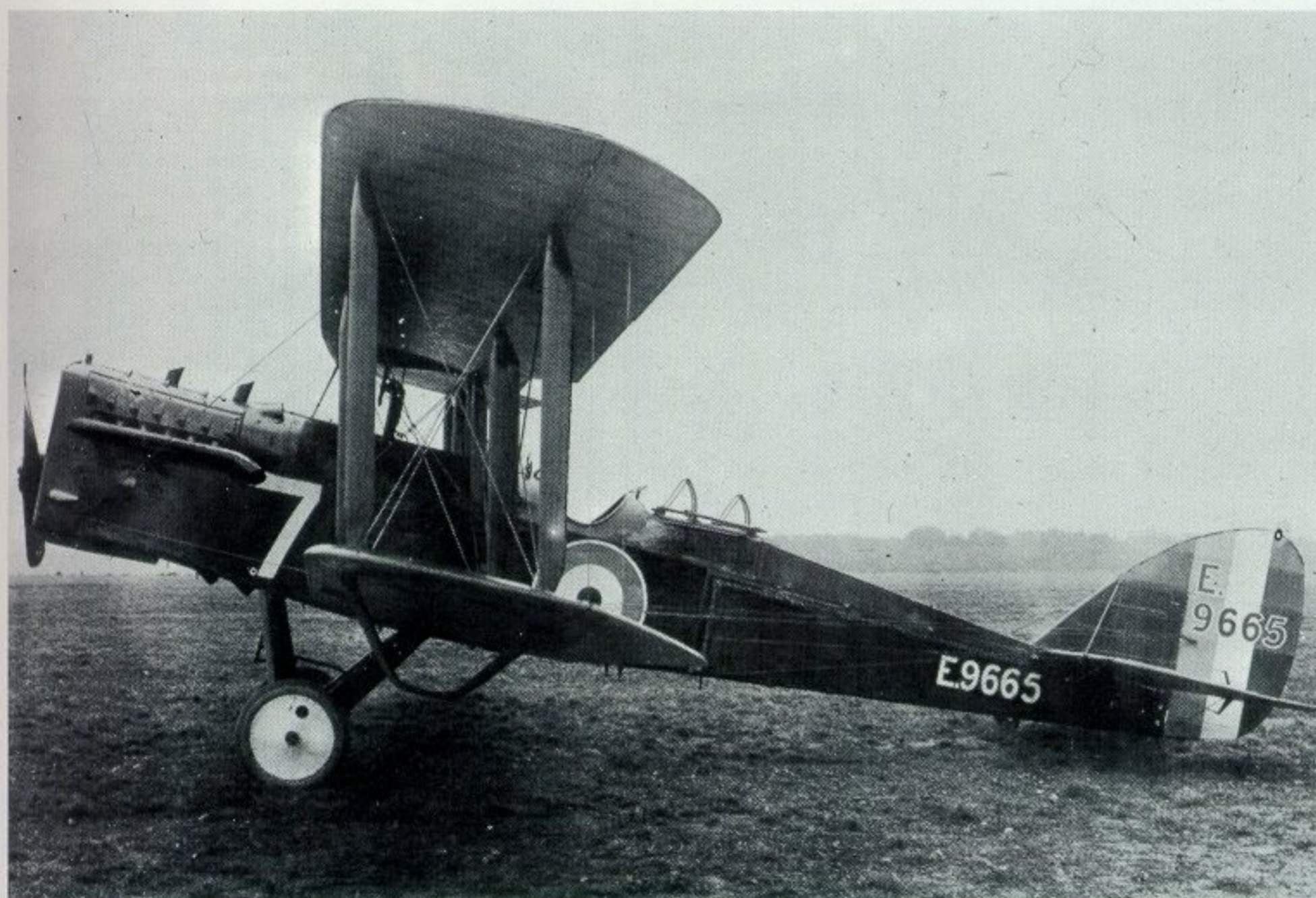
Fine side elevation of E9665, a Ninak of typical 1918-19 construction—in this case by Mann, Egerton of Norwich.
