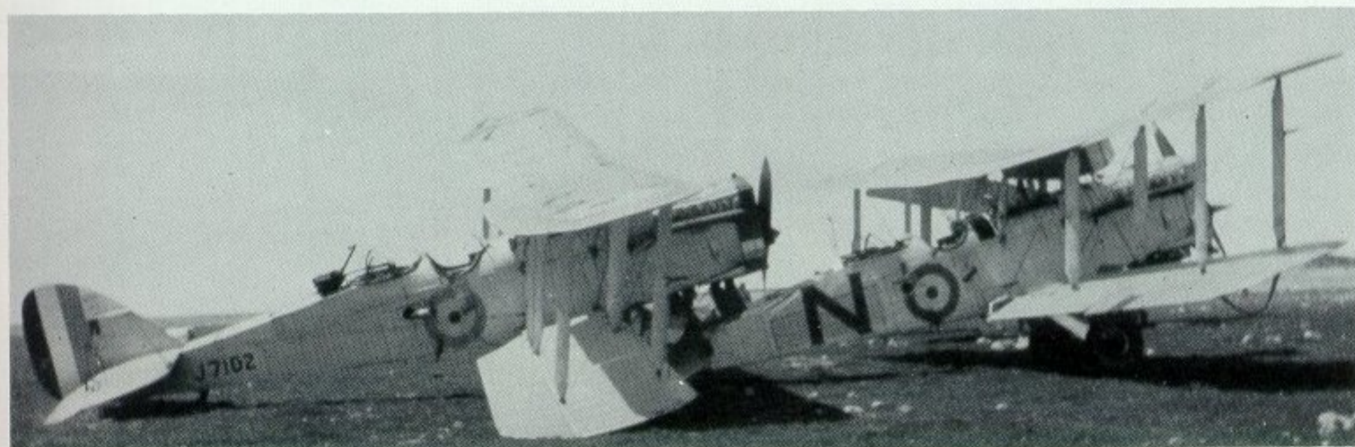
Before and After. A landing accident between J7321 (N) and J7102 of No. 8 Squadron on the southern frontier with Nedj territory during anti-Ibn Saud operations. Despite being deep in hostile country, both aircraft were hastily but effectively repaired by a working party airlifted in a Vickers Vernon and both Ninaks eventually flew back to base . . .
