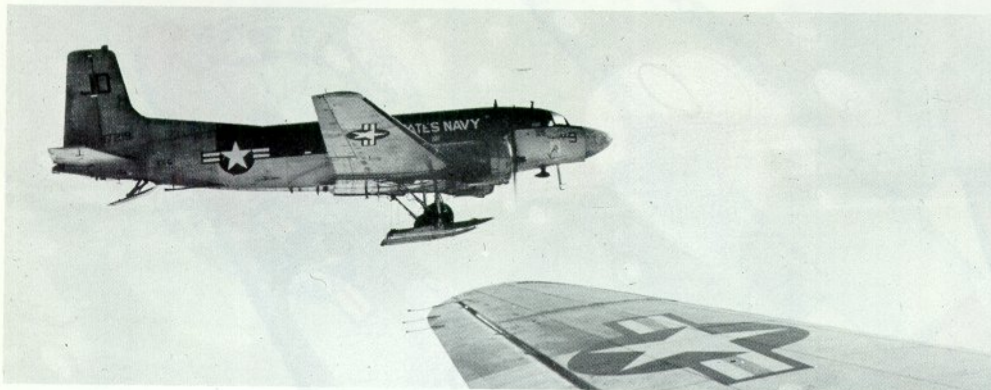
Seen at Detroit, Michigan during April 1956 this R4D-6S (BuNo. 99840) is from VX-1 (Experimental) Squadron. Note the 'thimble' radar nose and tail probe. (Photo: Bill Balogh)
