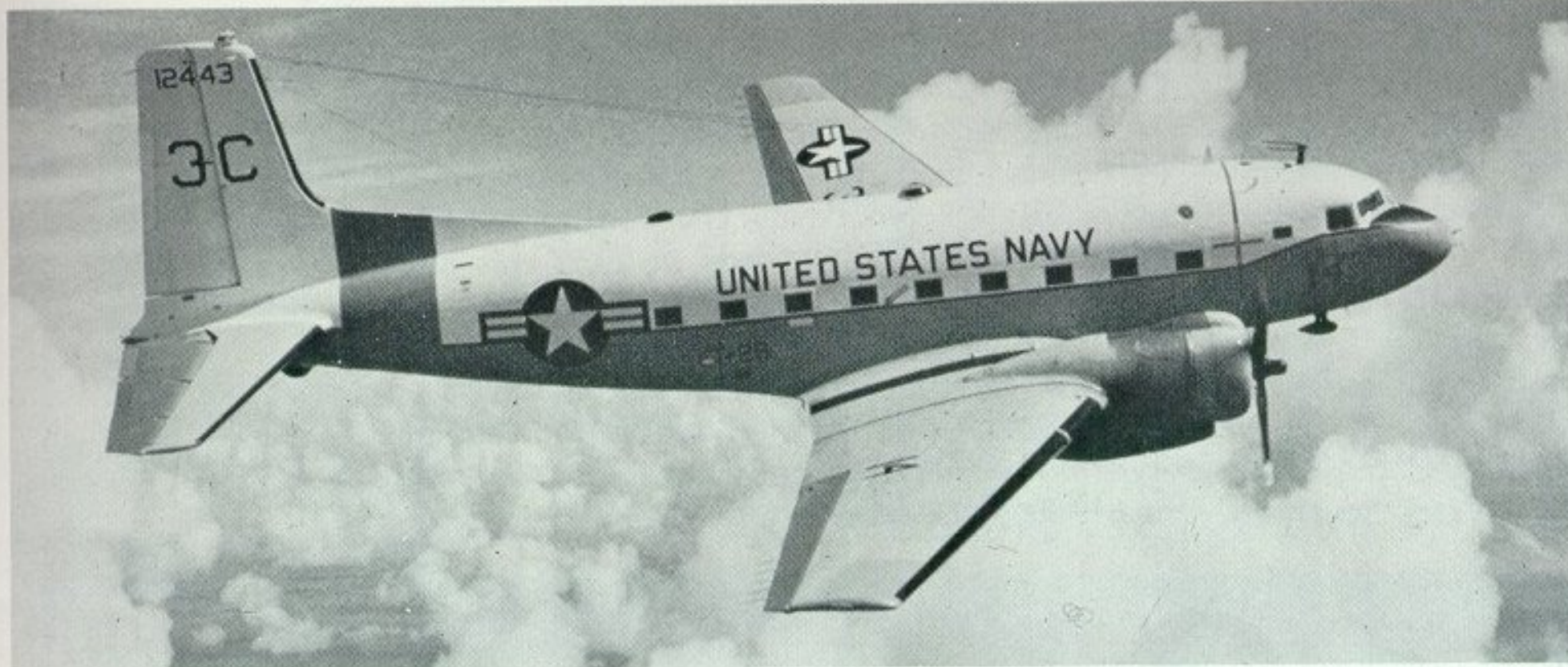
Fine air to air study of R4D-8 (BuNo. 12443) of VT-29 Squadron showing the new lines introduced with the conversion to Super DC-3. Originally an R4D-5 (with c/n. 9781) this transport also had a USAF serial 42-23919. (Photo: US Navy)
